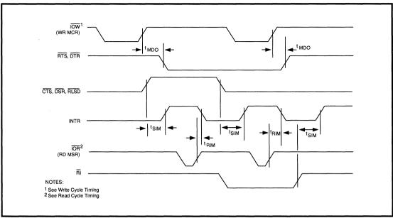
Figure C-3. MODEM Control Timing
