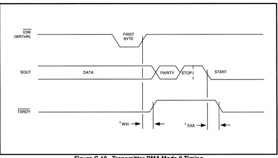
Figure C-10. Transmitter DMA Mode 0 Timing (FCR0 = 0 or FCR0 = 1 and FCR3 = 0)
