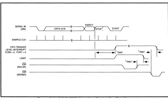
Figure C-6. RCVR FIFO Signaling Timing For First Byte
