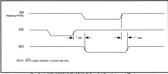
Fig. C-14. WD16C551/WD16C451B Parallel Port Interrupt Timing
