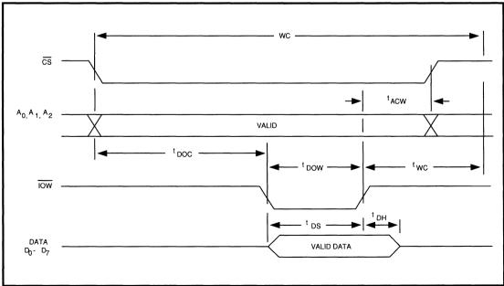
Figure C-5. Write Cycle Timing
