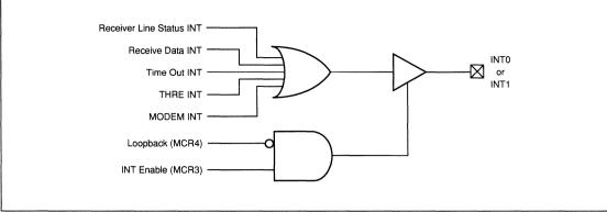
Figure 3. Interrupt Signal Logic
