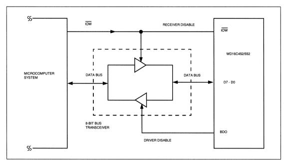
Figure 4. Typical Interface for a High-Capacity Data Bus
