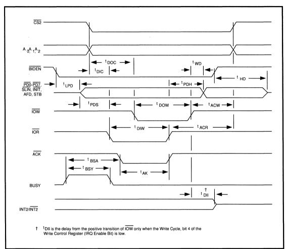
Figure C-12. Parallel Port Timing
