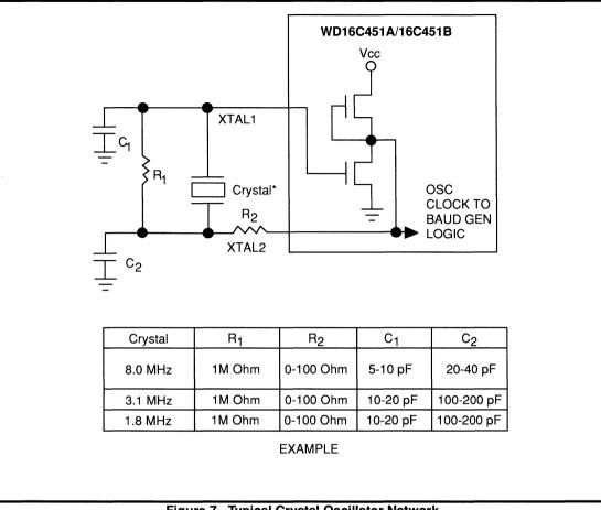
Figure 7. Typical Crystal Oscillator Network
