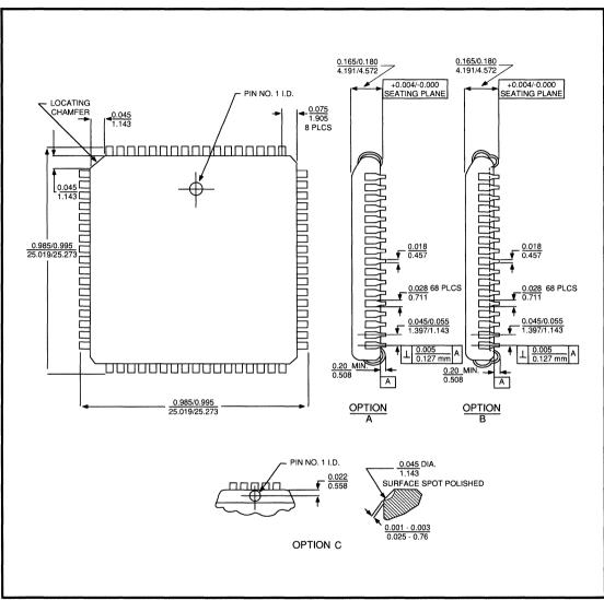
Figure D-1. 68-Pin QUAD Plastic Package
