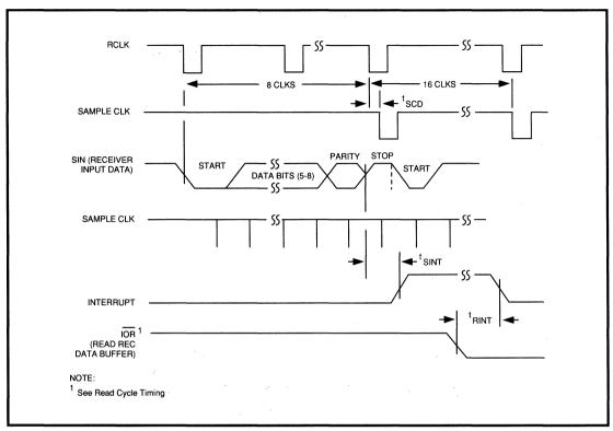
Figure C-1. Receiver Timing
