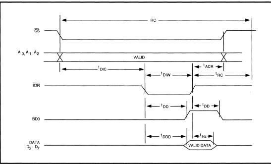
Figure C-4. Read Cycle Timing
