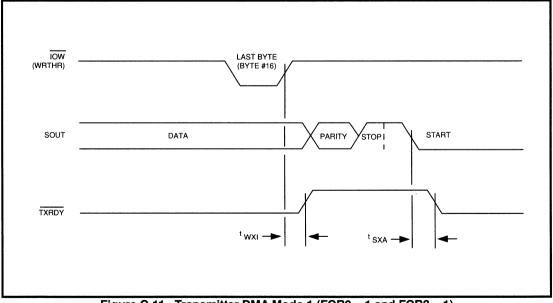
Figure C-11. Transmitter DMA Mode 1 (FCR0 = 1 and FCR3 = 1)
