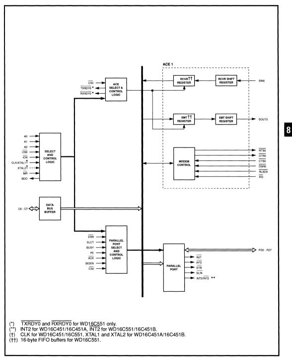
Figure 2. WD16C451/WD16C55A Block Diagram
