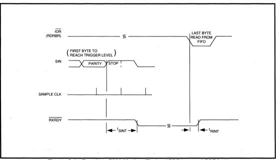
Figure C-9. Receiver DMA Mode 1 Timing (FCR0=1 and FCR3=1)
