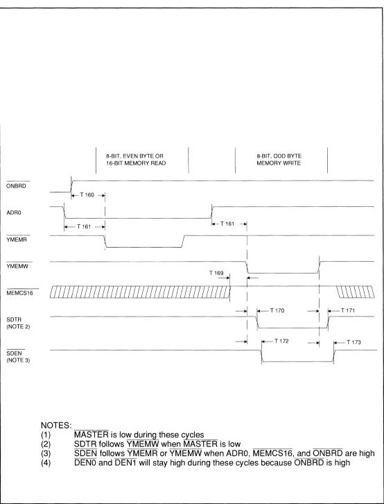
FIGURE 7-25. MASTER MODE TIMING: OFF-BOARD MEMORY READ/WRITE
