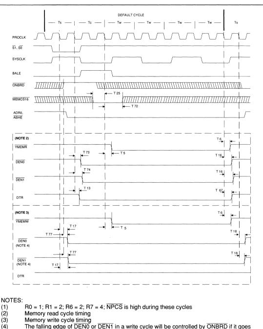
The falling edge of DEN0 or DEN1 in a write cycle will be controlled by ONBRD if it goes high in the last half of the processor Ts state, or by PROCLK if ONBRD goes high earlier
