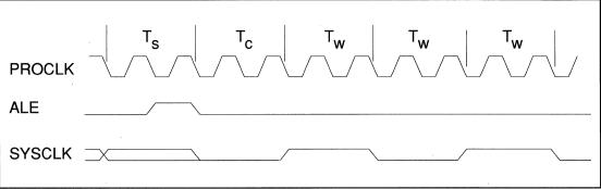
FIGURE 2-1. SYSCLK TIMING DURING HIGH SPEED OPERATIONS
