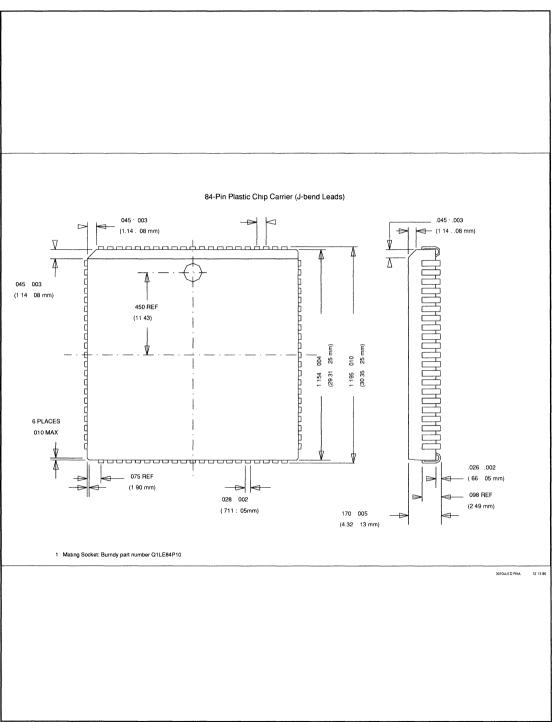
FIGURE 7-27. 84-PIN PLCC PACKAGING DIAGRAM
