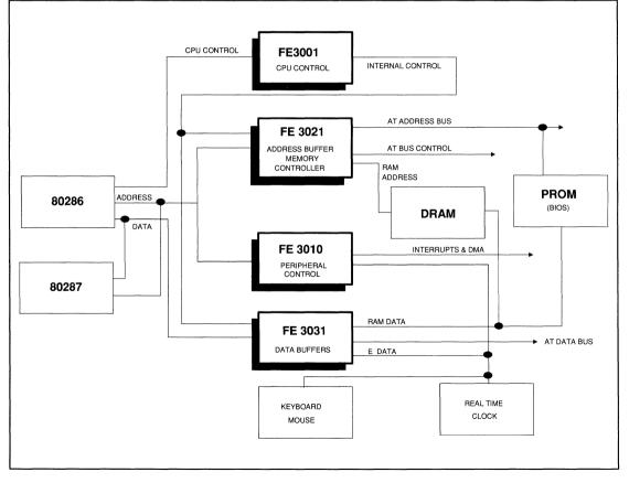
FIGURE 1-1. FE3600 CHIP SET FUNCTIONAL BLOCK DIAGRAM
