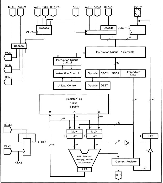
Figure 2. WTL 3167 simplified block diagram
