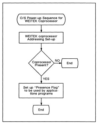
Figure 54. Operating systems power-up sequence for WTL 3167
