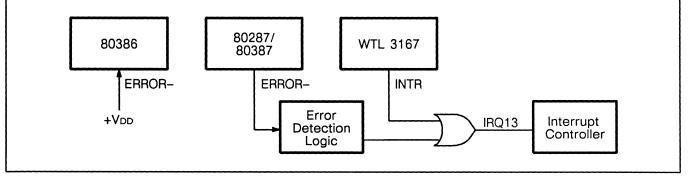
Figure 7. Interrupt output connection in an AT-compatible system
