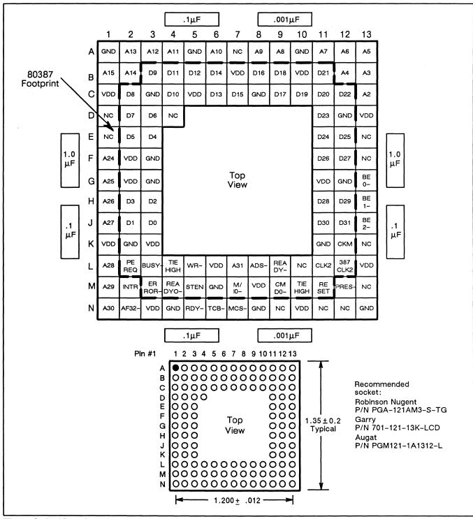
Figure 3. EMC socket pinout and dimensions
