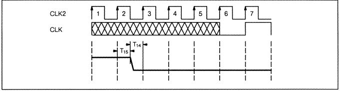
Figure 18. RESET timing
