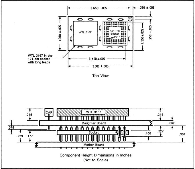
Figure 5. WTL 3167 coprocessor board physical dimensions
