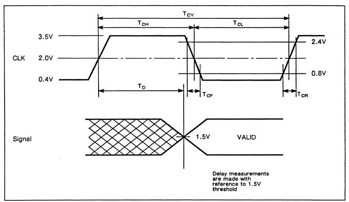
Figure 15. Reference levels in delay measurements
