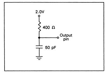
Figure 17. AC test load
