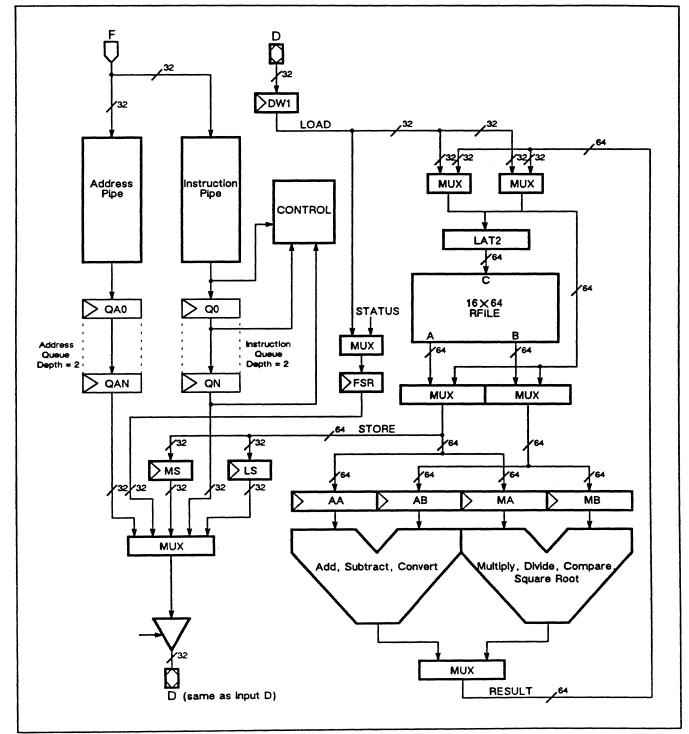
Figure 3. Conceptual block diagram
