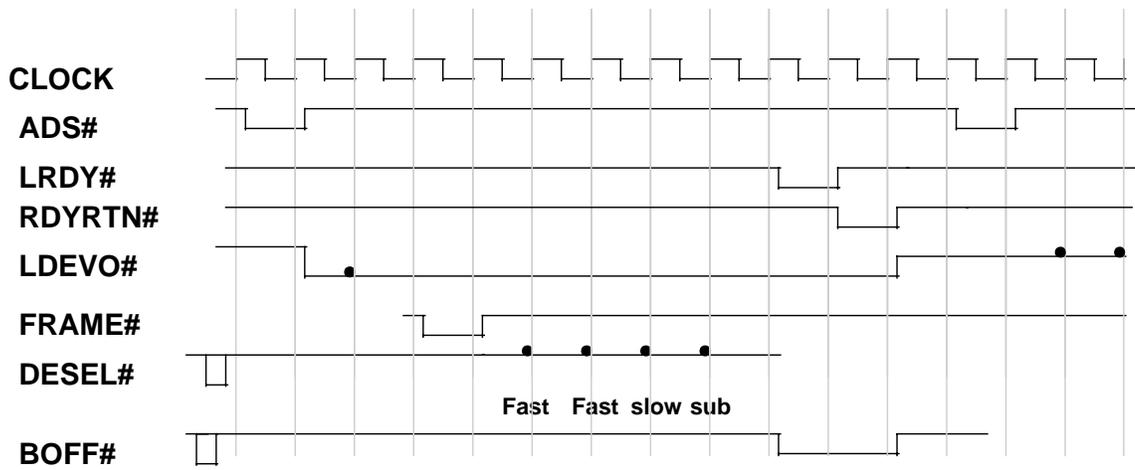
Without **LDEVO#** assert on the VL bus after the 2nd T2 in the regenerated CPU cycle, the core logic chipset will dispatch an ISA cycle according to the subtracting decoding rule mentioned in Sec. 2.0.
