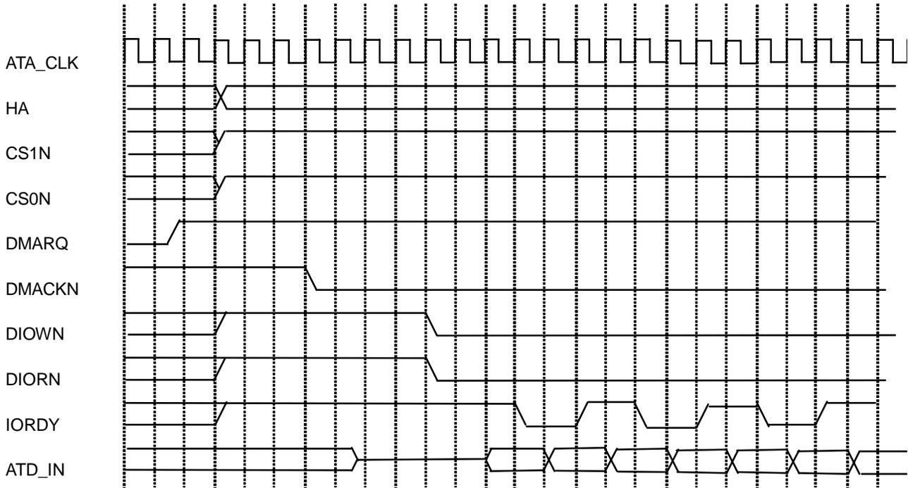
The above figure is a timing diagram that shows the transfer start position during read transfer in Ultra DMA Mode 5. Following are the steps for setting up the software used when transferring data.
