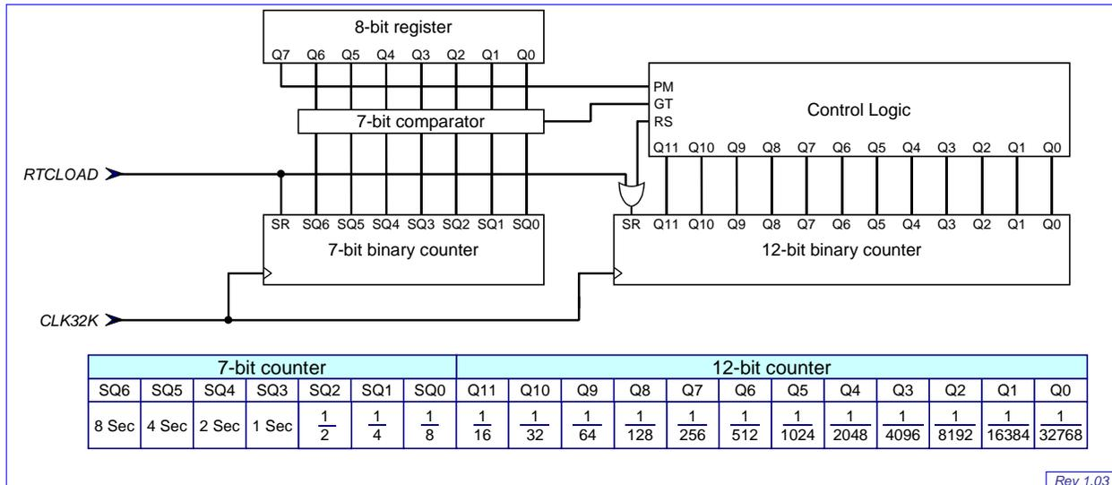
**Figure 11-3 Logic Diagram of Time Base Corrector**
