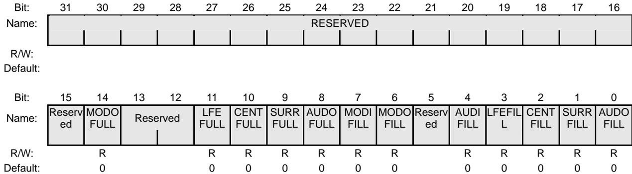
**Figure 24-18 ACFIFOSTS Register**
