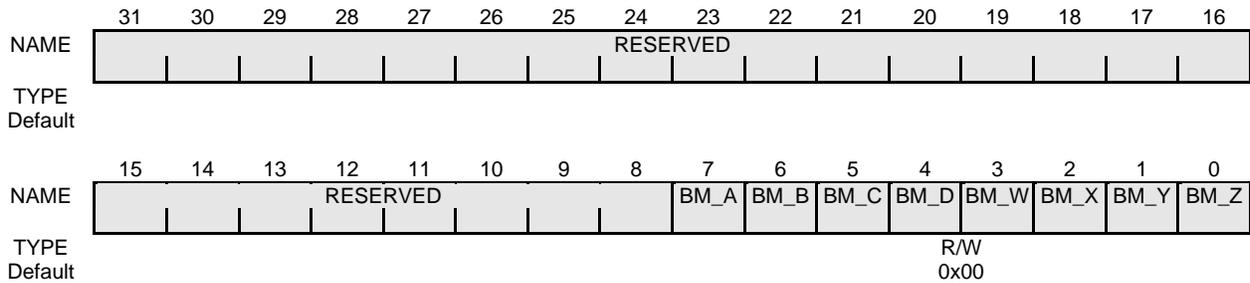
**Figure 16-37 PCI Bus Arbiter Broken Master Register**
