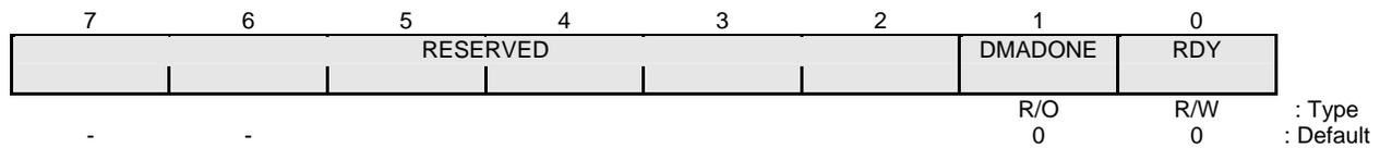
Figure 10-12 NAND Flash Memory Interrupt Status Register (NDFISR)
