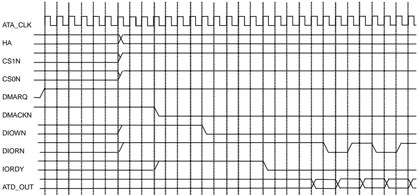
The above figure is timing diagram that shows the transfer start position during write transfer by Ultra DMA Mode 5. The steps for setting up the software used when transferring data are exactly the same as for when issuing a read command. The meaning of each signal on the ATA Bus changes: IORDY becomes the transfer Ready signal that the device provides to this controller; DIORN becomes the Strobe signal when transferring data to the device.
