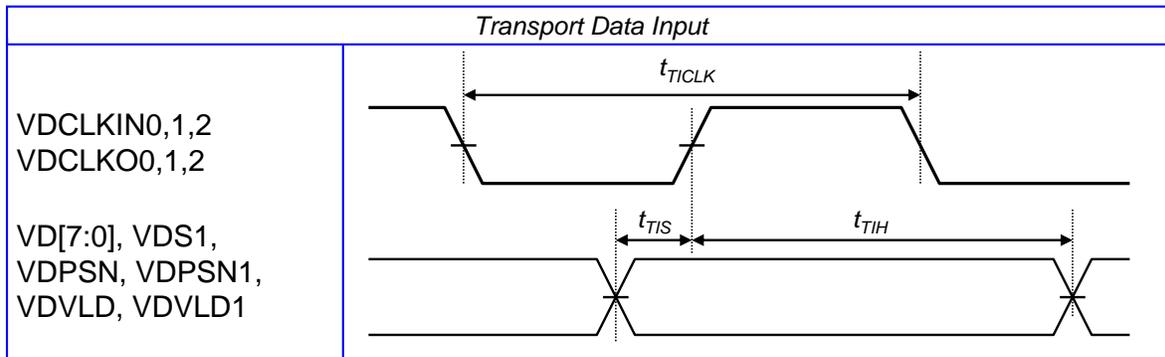
Figure 28-21 Video Port Transport data input
