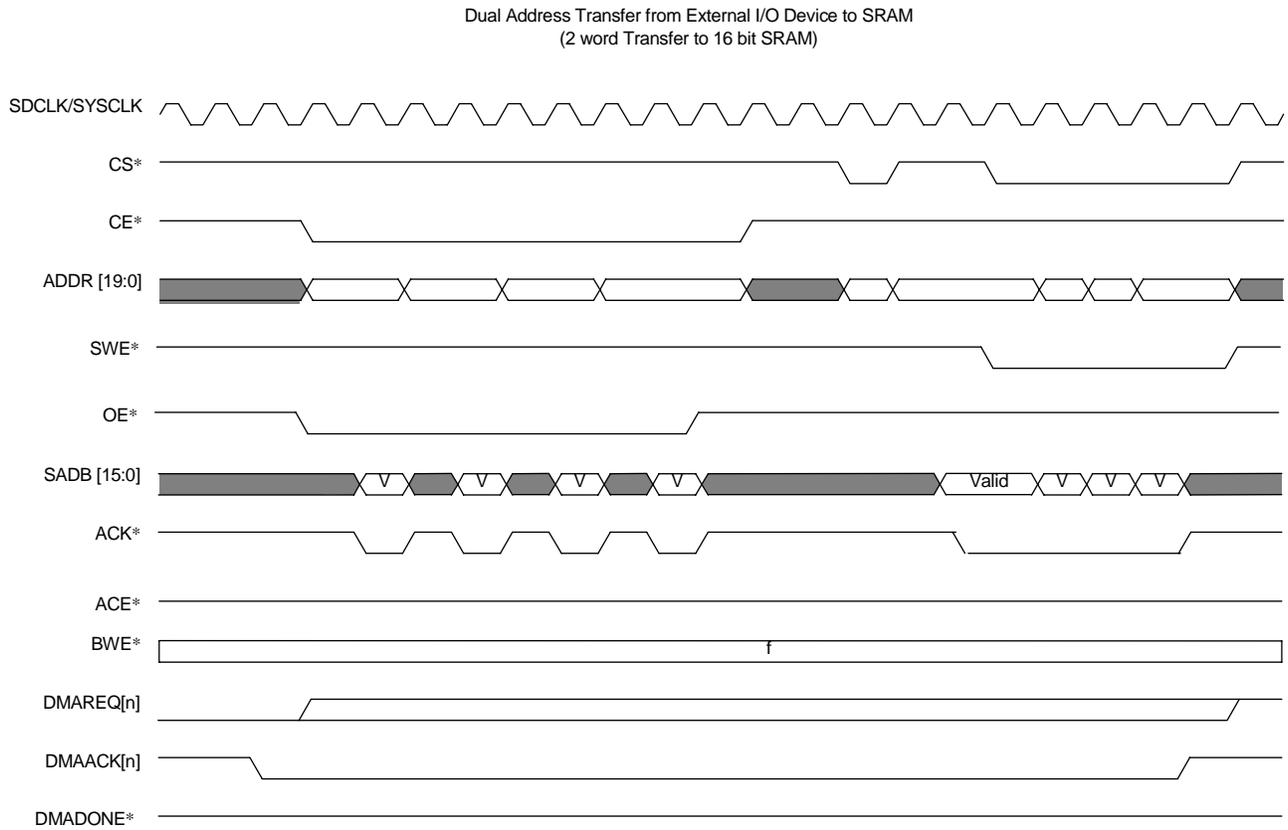
**Figure 14-21 Dual Address Transfer from External I/O Device to SRAM
