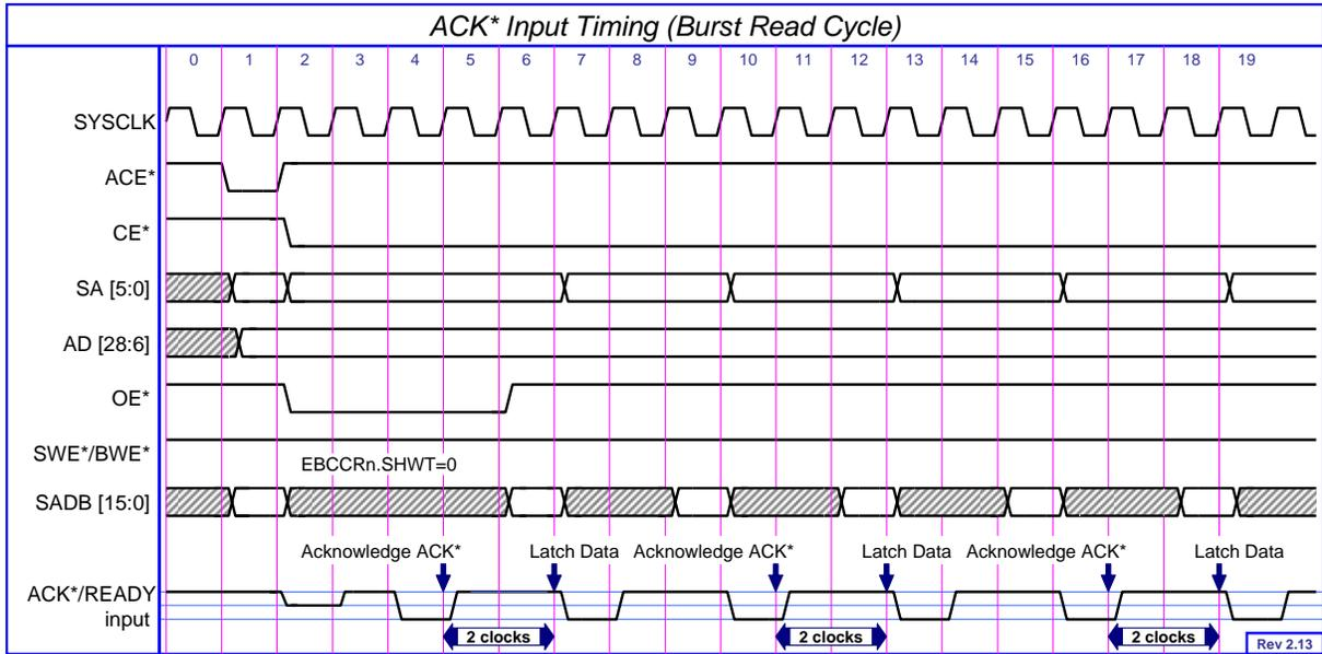
**Figure 9-10 ACK\* Input Timing (Burst Reade Cycle)**
