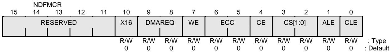
Figure 10-10 NAND Flash Memory Mode Control Register (NDFMCR)
