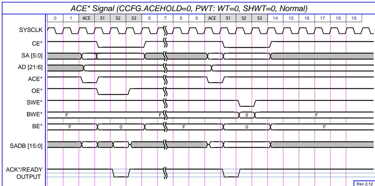
**Figure 9-16 ACE\* Signal (CCFG.ACEHOLD=0, PWT: WT=0, SHWT=0, Normal)**
