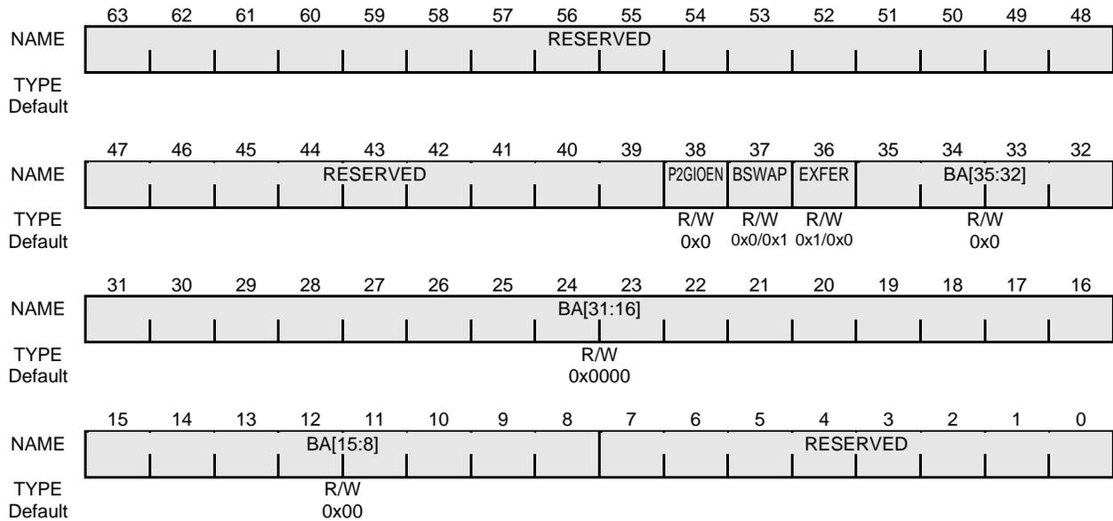
**Figure 16-59 P2G I/O Space G-Bus Base Address Register**
