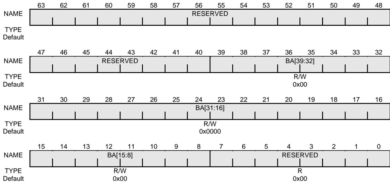
**Figure 16-51 G2P Memory Space 2 G-Bus Base Address Register**
