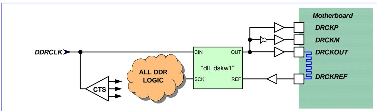
Figure 5-10 Structure of DDR Clock De-Skew Circuit
