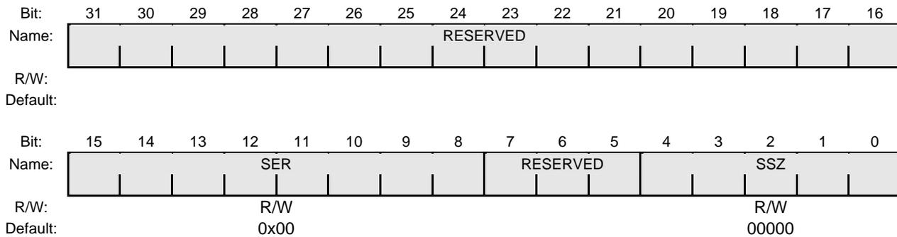
**Figure 20-6 SPI Control Register 1 (SPCR1)**
