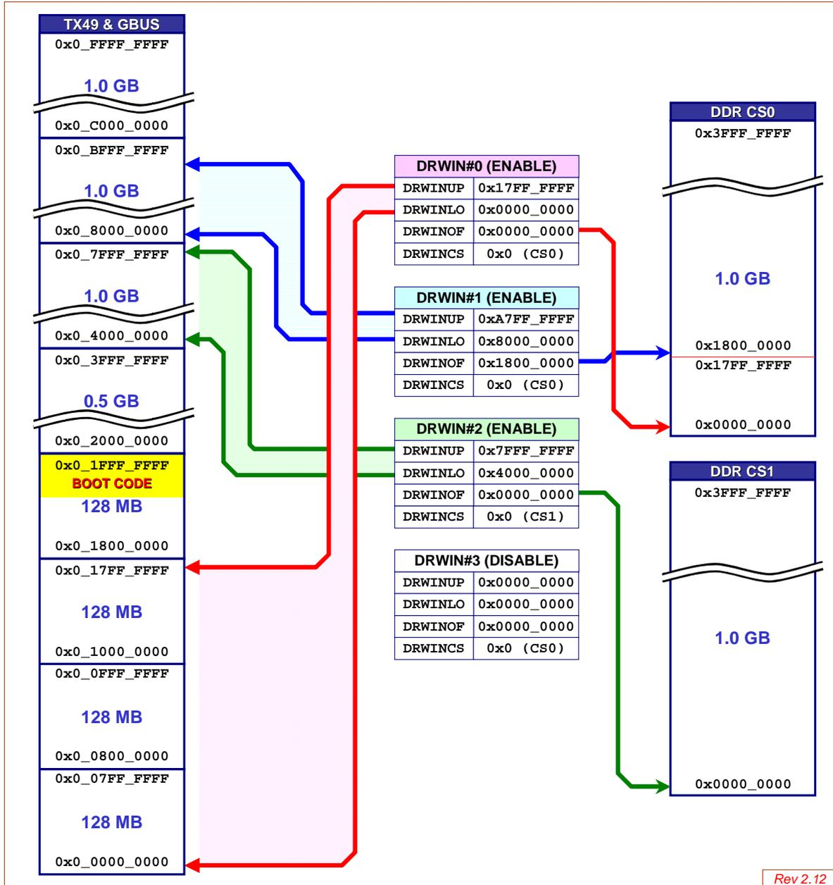
Figure 6-5 Example of DDR Memory Split-Mapping
