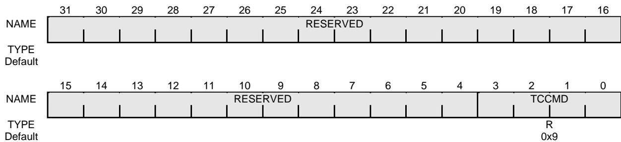
Figure 16-32 P2G Current Command Register
