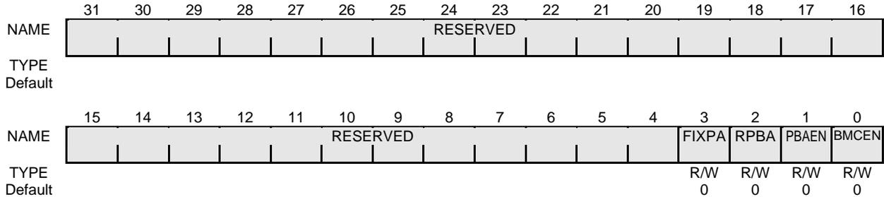
**Figure 16-34** PCI Bus Arbiter Configuration Register
