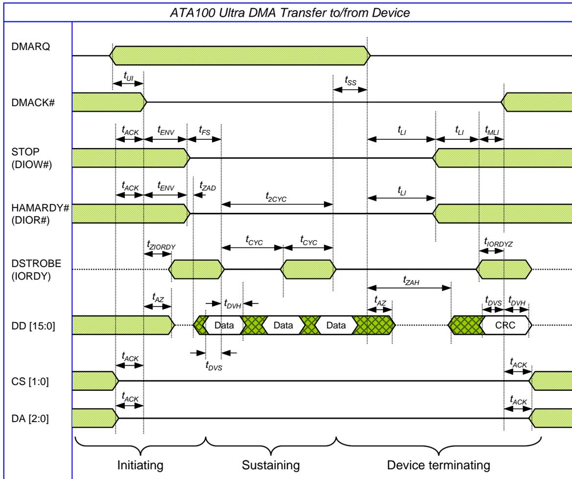
**Figure 28-17 Ultra DMA data Transfer to/from device**
