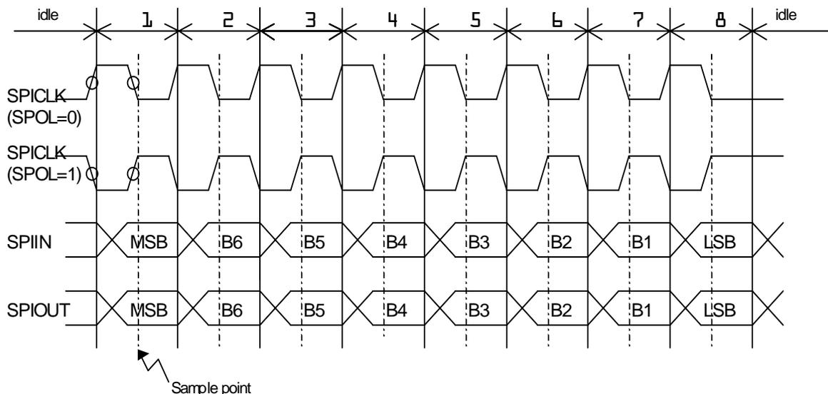
**Figure 20-3 Transfer Format when SPHA is “1”**
