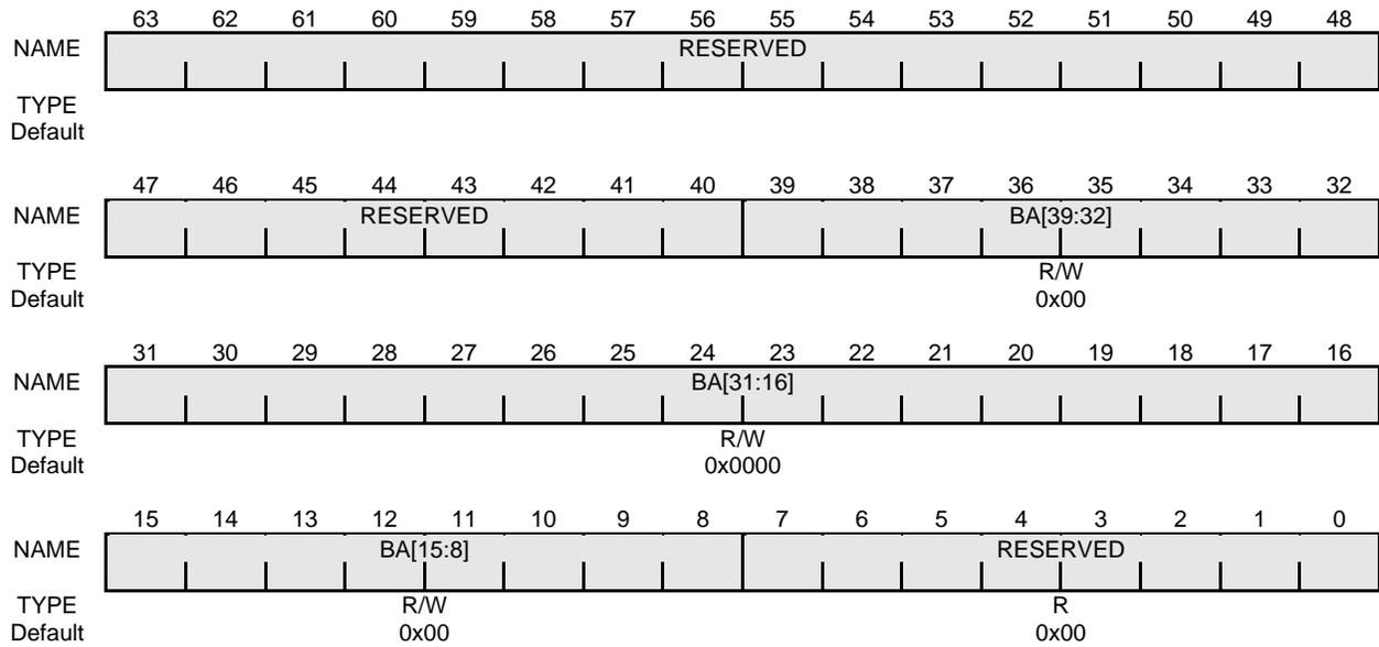
**Figure 16-52 G2P I/O Space G-Bus Address Register**
