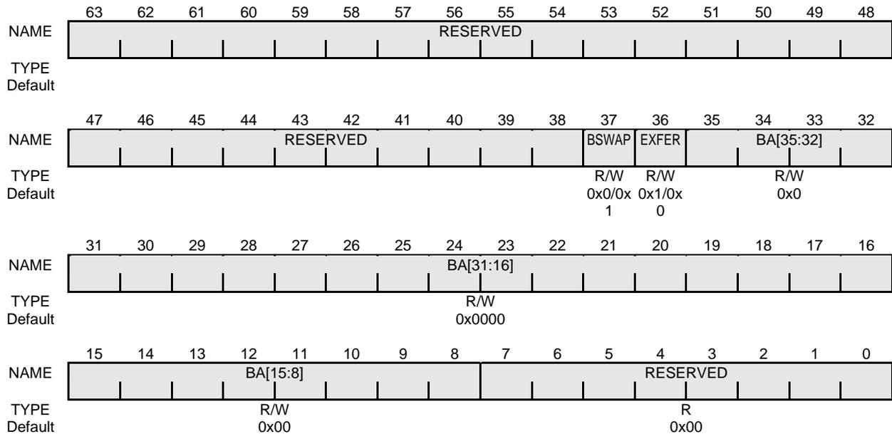
**Figure 16-43 G2P Memory Space 2 G-Bus Base Address Register**
