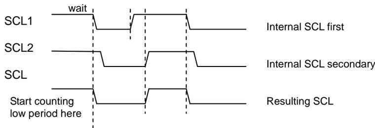
**Figure 22-3 Clock Synchronization**
