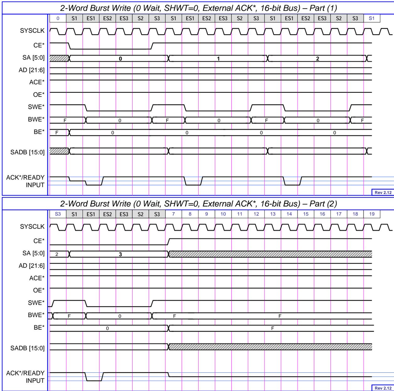
**Figure 9-32 2-word Burst Write (0 Wait, SHWT=0, External ACK\*, 16-bit Bus)**
