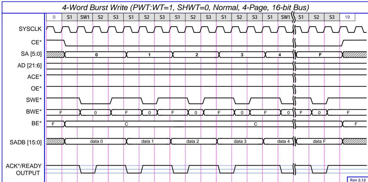
**Figure 9-28 4-word Burst Write (WT=1, PWT=0, SHWT=0, 4-page, 16-bit Bus)**
