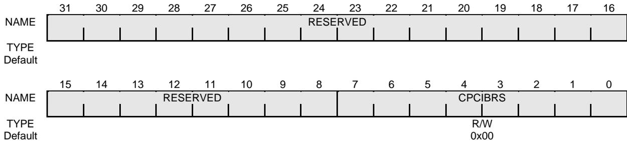
Figure 16-38 PCI Bus Arbiter Current Request Register
