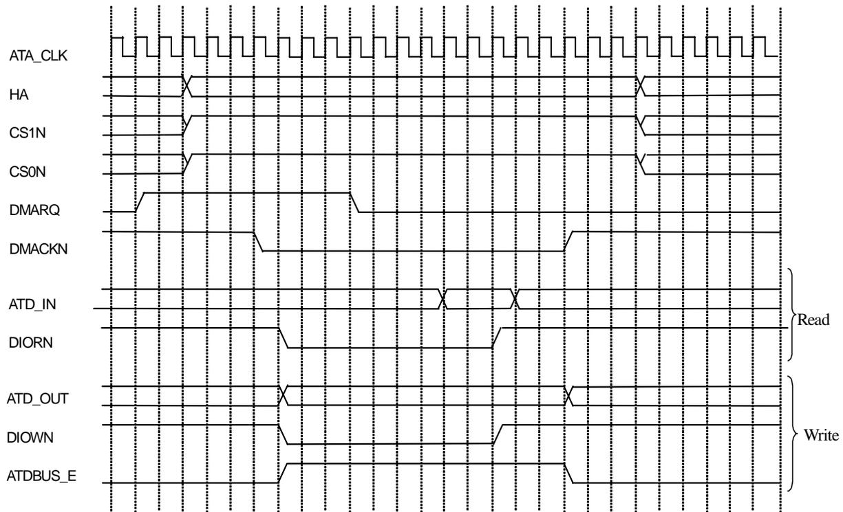
The above figure is a timing diagram that shows read/write transfer by Multiword DMA Mode 2. Following are the steps for setting up the software used when transferring data.
