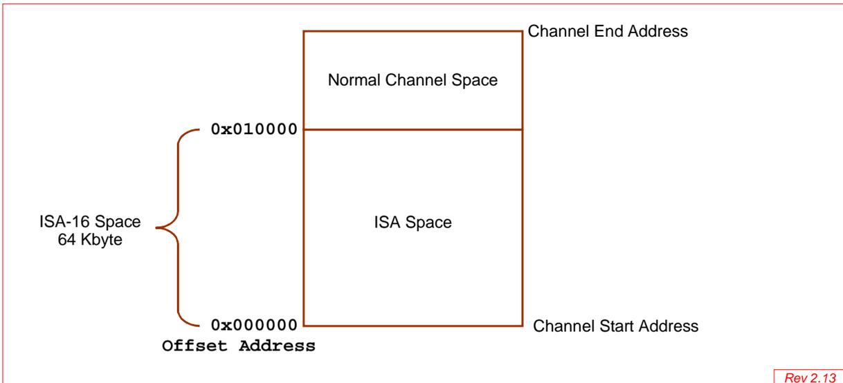
**Figure 9-14 Physical Address Mapping of the ISA Spaces**
