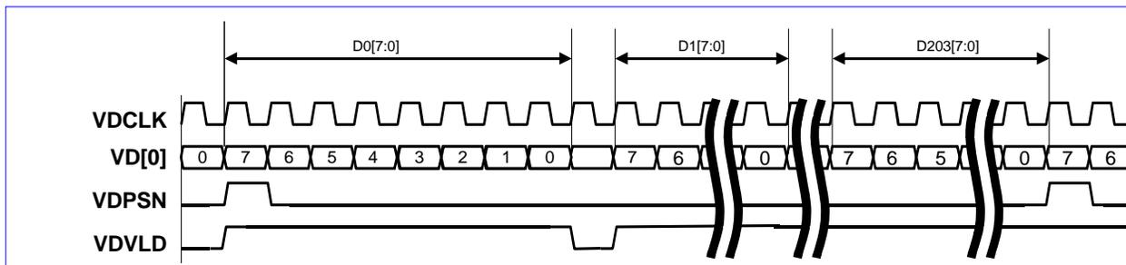
Figure 12-8 Serial transmission format with RS-coded packets (204 Bytes)
