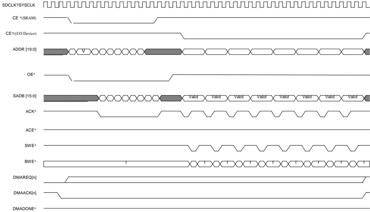
**Figure 14-20 Dual Address Transfer from Memory to External I/O Device
