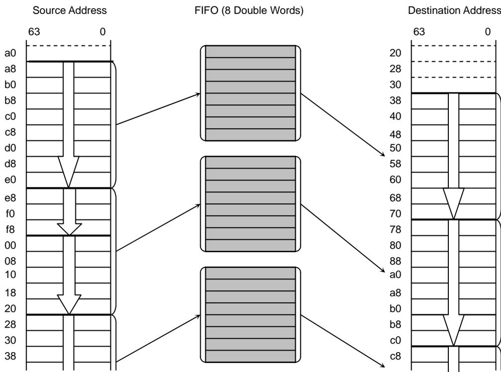
**Figure 14-4 Dual Address Burst Transfer (DMCCRn.USEXFSZ = 1)**
