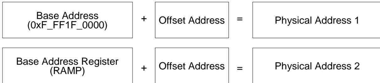
**Figure 6-7 Generating Physical Address for a Internal Register**
