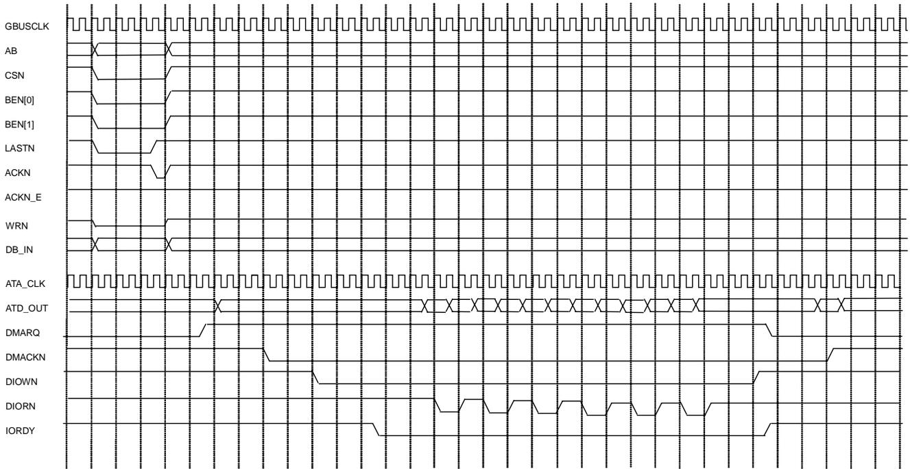
The above figure is a timing chart that shows the situation when using the ATAPI Packet Command Register described in Section 17.3.3.19 to issue a command packet to the device. Ultra DMA is used as the transfer protocol. Also, Ultra DMA uses the mode selected by bits [7:4] of the System Control Register described in Section 17.3.2.4.
