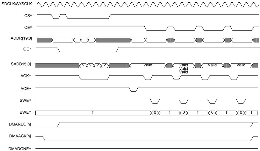
**Figure 14-23 Dual Address Transfer from Memory to External I/O Device**
