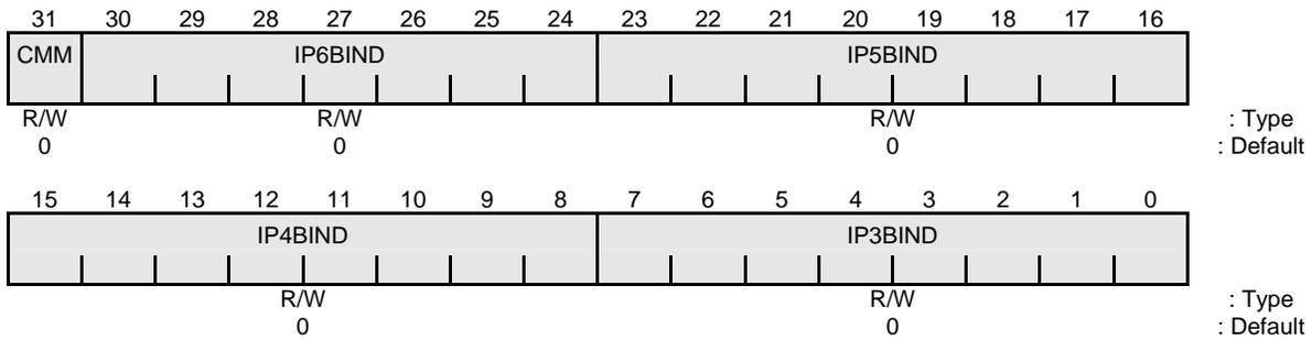
**Figure 8-5 Interrupt Source and Cause IP Binding Register**
