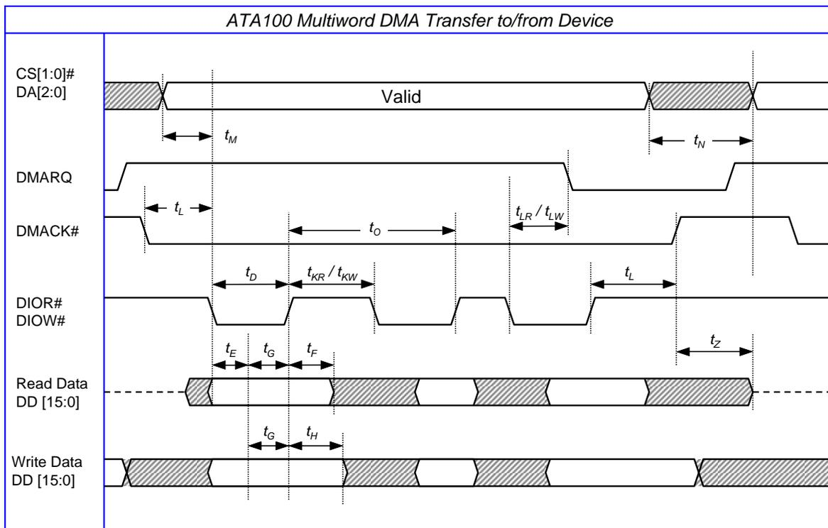
Figure 28-16 Multiword DMA data Transfer to/from device
