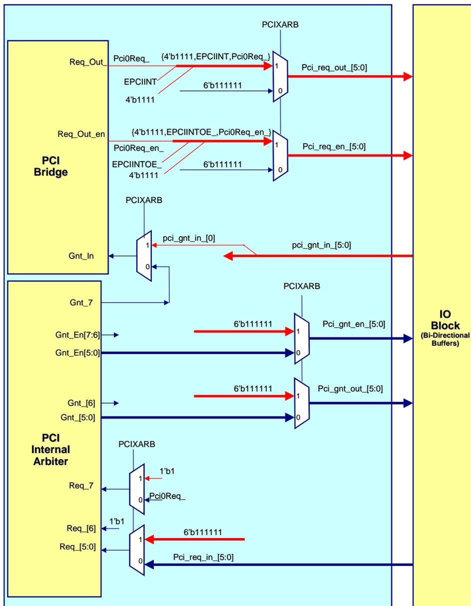
Figure 16-12 PCI Req/Gnt connections in Int/Ext Arbiter Mode
