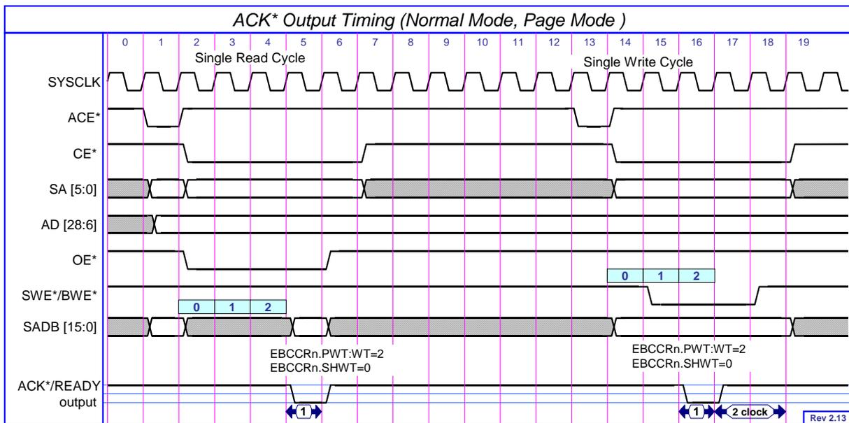
**Figure 9-8 ACK\* Output Timing (Single Read/Write Cycle)**
