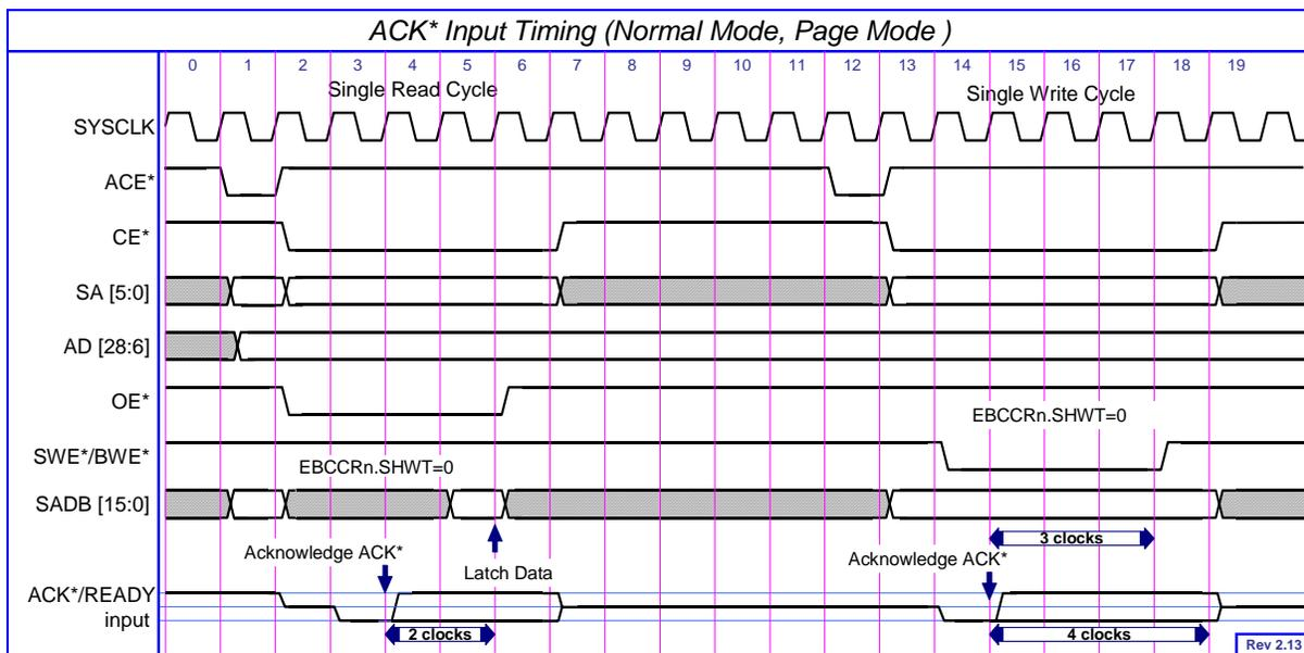
**Figure 9-9 ACK\* Input Timing (Single Read/Write Cycle)**
