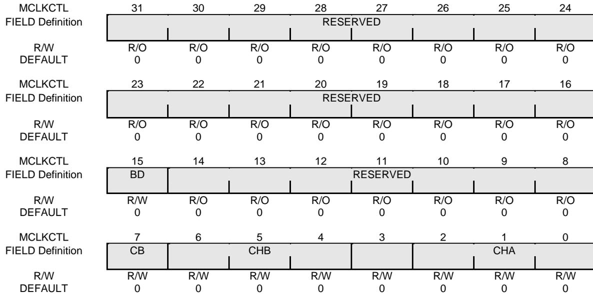
Figure 7-10 Definition of MCLKCTL Register
