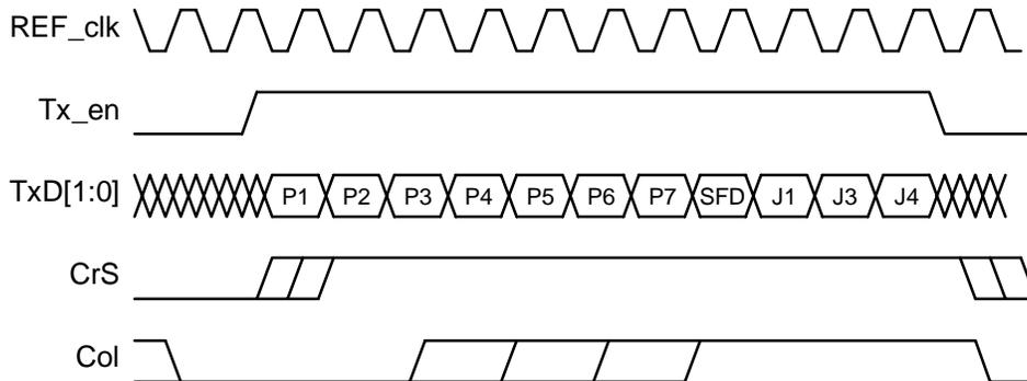
**Figure 18-13 Transmission when Collision Occurred in the Preamble**
