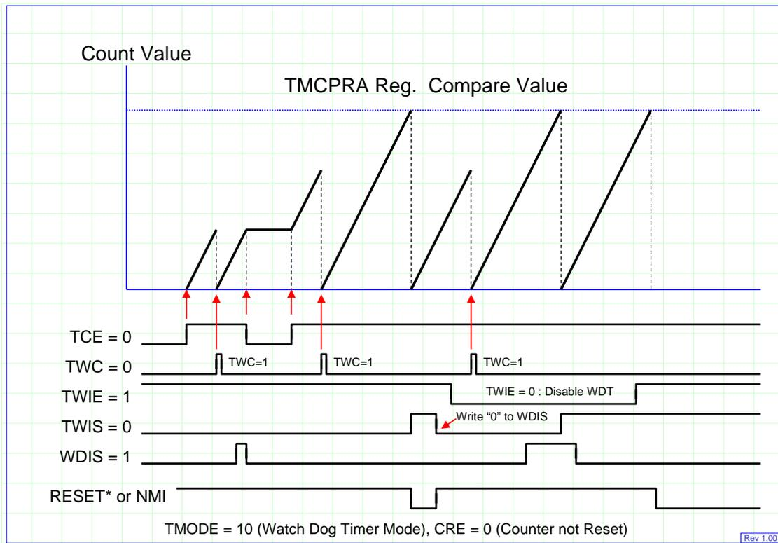
**Figure 13-6 Operation Example of the Watchdog Timer Mode**
