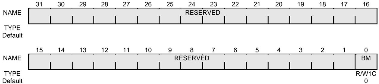
**Figure 16-35 PCI Bus Arbiter Status Register**
