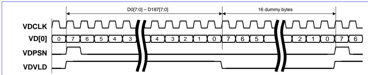
Figure 12-7 Serial transmission format with 204 Byte packets
