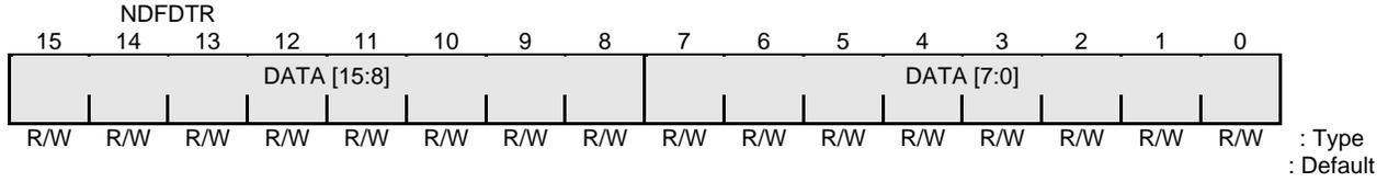
**Figure 10-9 NAND Flash Memory Data Transfer Register (NDFDTR)**
