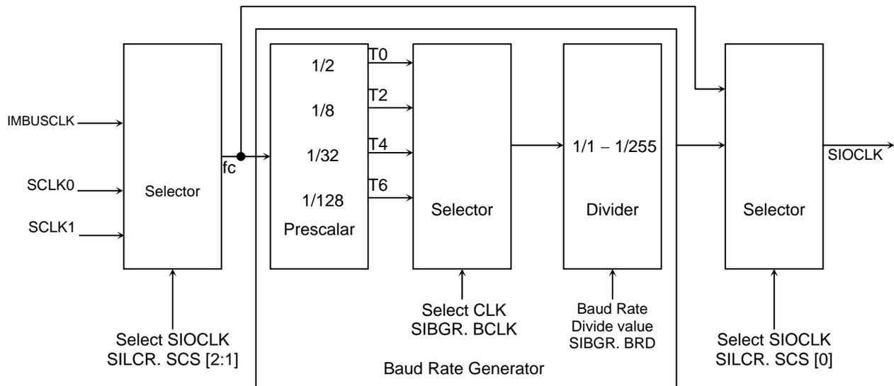
**Figure 19-3 Baud Rate Generator and SIOCLK Generator**
