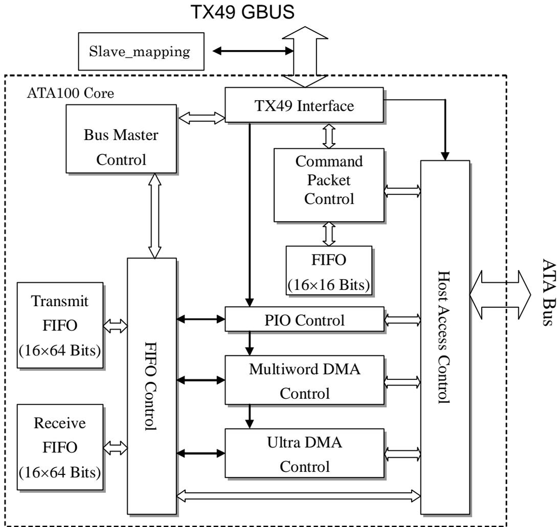
Figure 17-1 ATA100 Controller Block Diagram
