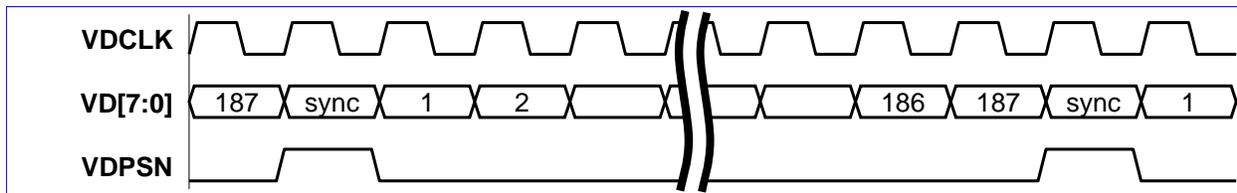
Figure 12-3 Transmission format with 188 Byte packets (VDVLD = 1)
