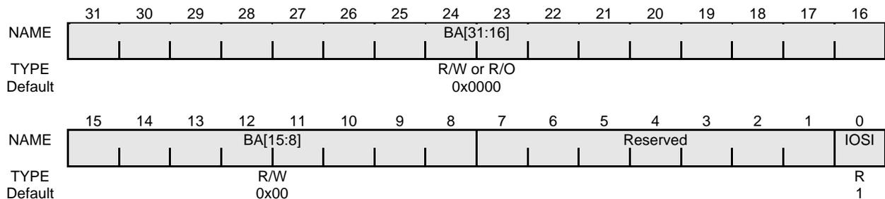
**Figure 16-20 P2G I/O Space PCI Base Address Register**
