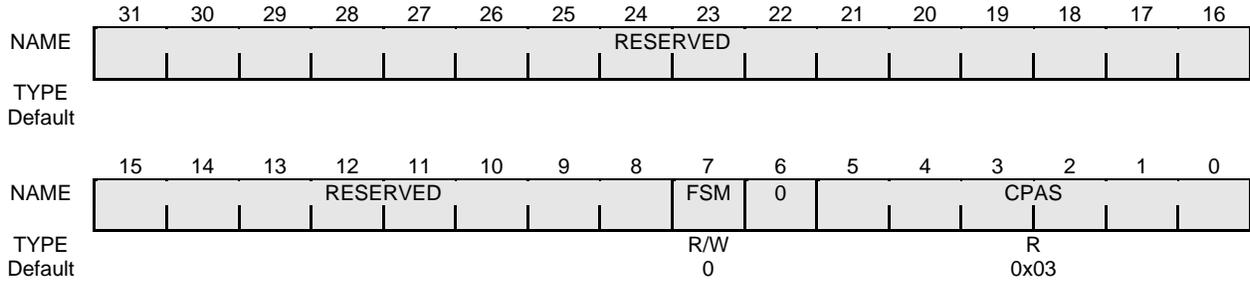
Figure 16-40 PCI Bus Arbiter Current State Register
