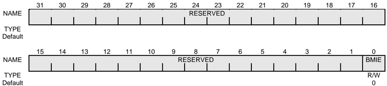
**Figure 16-36 PCI Bus Arbiter Interrupt Mask Register**
