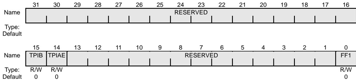
**Figure 13-13 Pulse Generator Mode Register**
