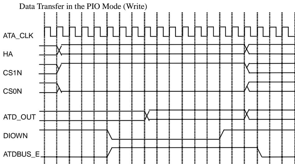
The above figures are timing diagrams of read/write transfer by PIO Mode 4. Following are the steps for setting up the software used when transferring data.
