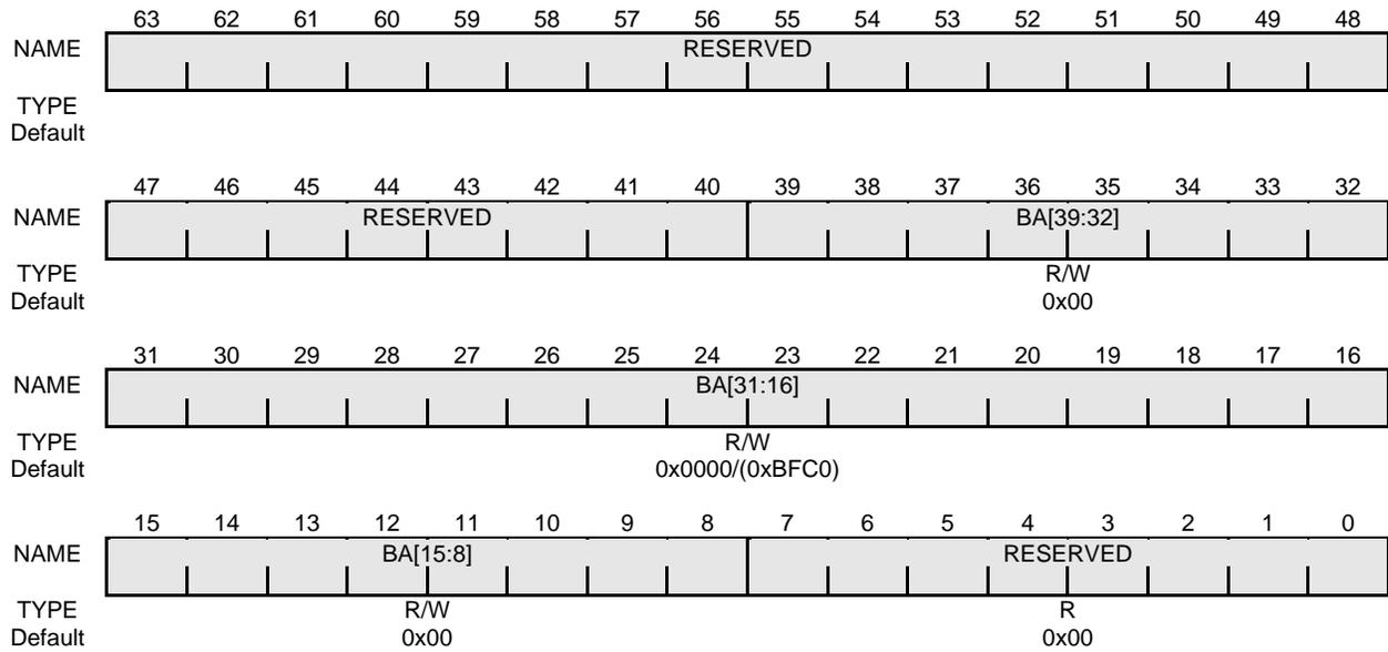
**Figure 16-50 G2P Memory Space 1 G-Bus Base Address Register**
