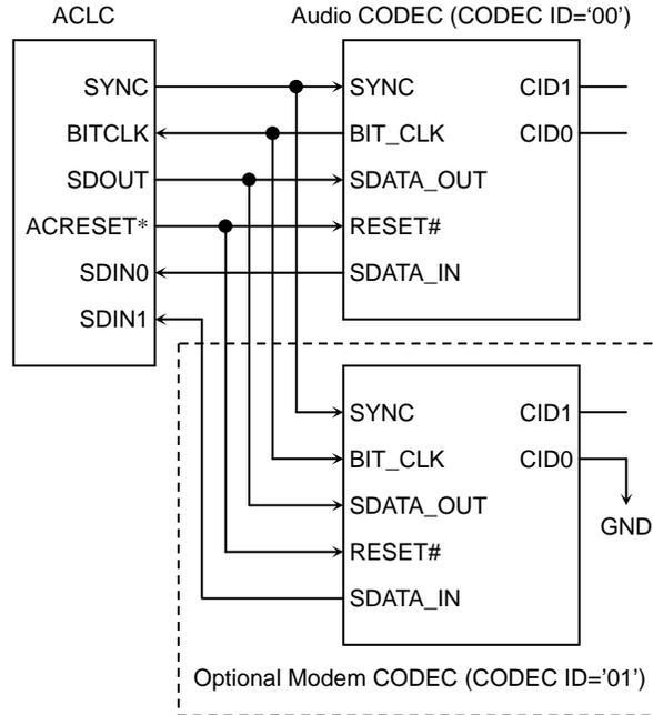
**Figure 24-2 Stereo Audio and Optional Modem Connection Diagram**
