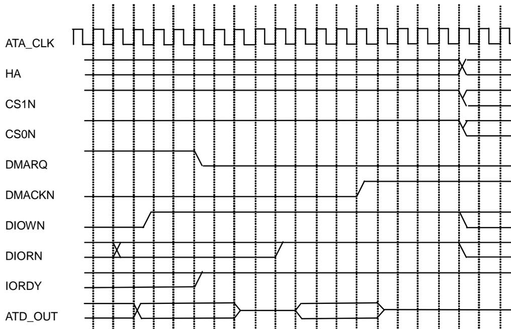
The above figure is a timing diagram that shows the transfer end position during write transfer by Ultra DMA Mode 5. Following is the flow of each control signal.
