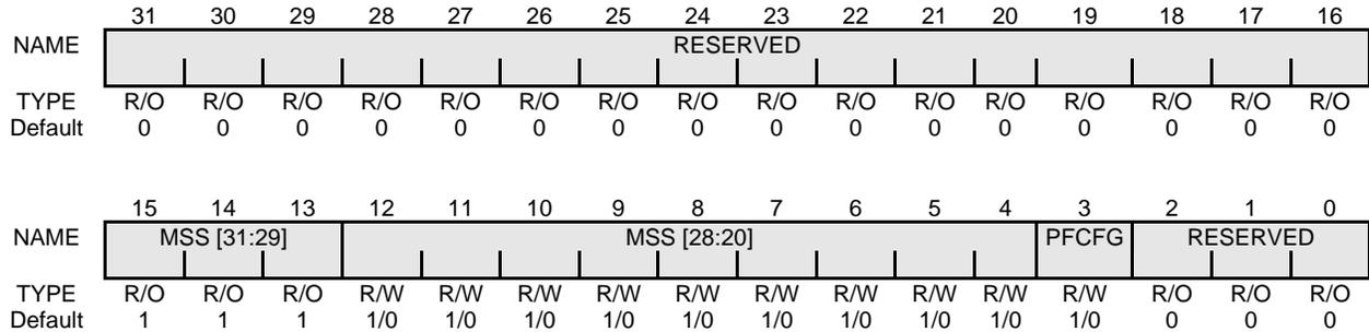
**Figure 16-19 P2G Memory Space (m) Configuration (m=0,1,2)**
