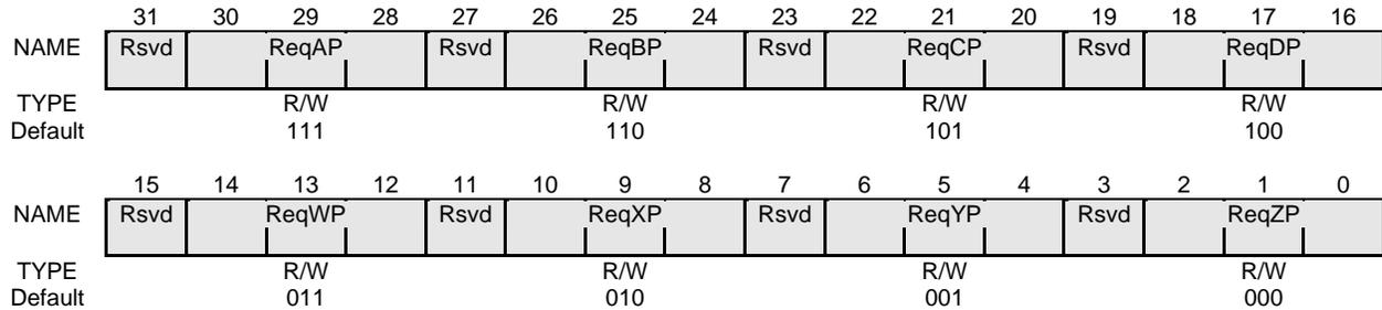
Figure 16-33 PCI Bus Arbiter Request Port Register
