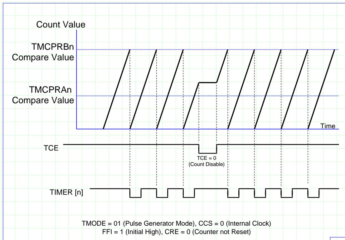
**Figure 13-5 Operation Example of the Pulse Generator Mode**
