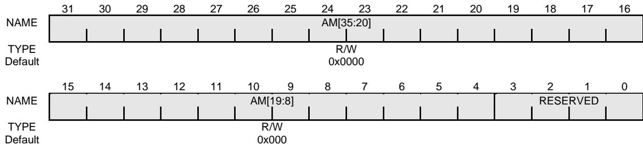
Figure 16-47 G2P Memory Space 2 Address Mask Register
