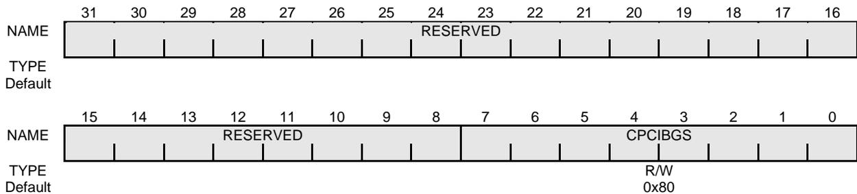
Figure 16-39 PCI Bus Arbiter Current Grant Register
