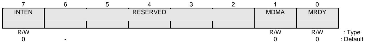
**Figure 10-13 NAND Flash Memory Interrupt Mask Register (NDFIMR)**
