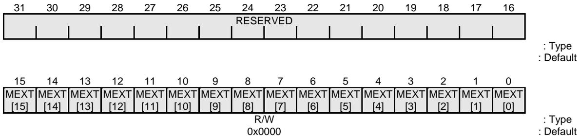
**Figure 8-21 Interrupt Request External Interrupt Mask Register**
