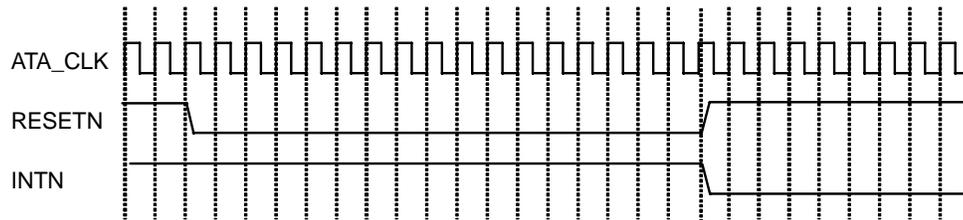
The above figure is a timing chart that shows the RESETN signal that is input to the device by setting bit [11] of the System Control Register to "1". As you can see from the above timing chart, the system is configured so you can send an interrupt signal to the microcontroller simultaneous to automatically clearing the above bit when the time set by the Host Reset Timer Register elapses.
