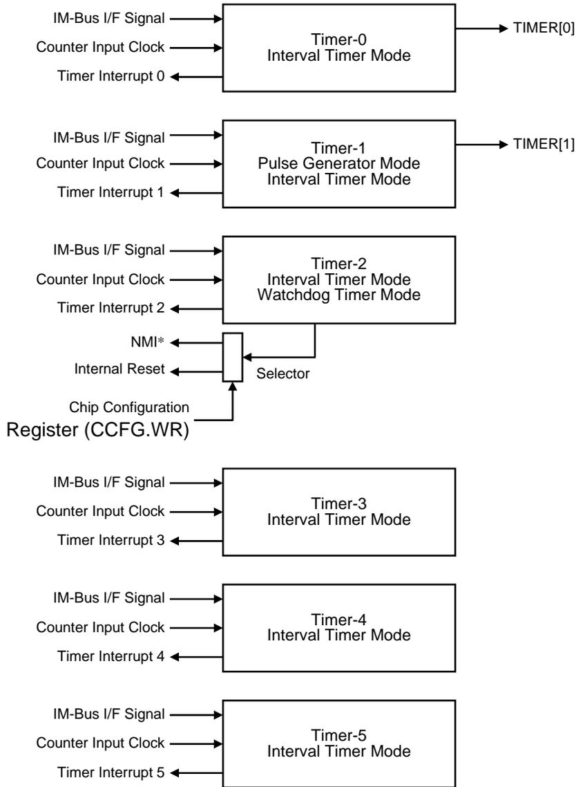
**Figure 13-1 Connecting Timer Module Inside the TX4939**
