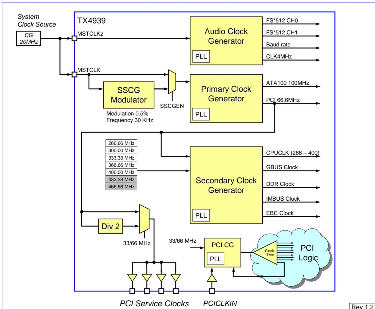
**Figure 5-1 Overview of Clocking System in TX4939**
