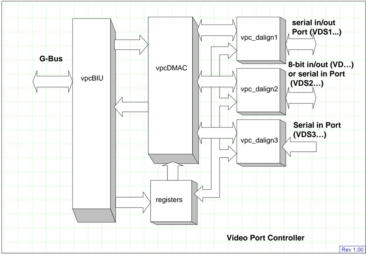
Figure 12-1 Block Diagram of Video Port Controller
