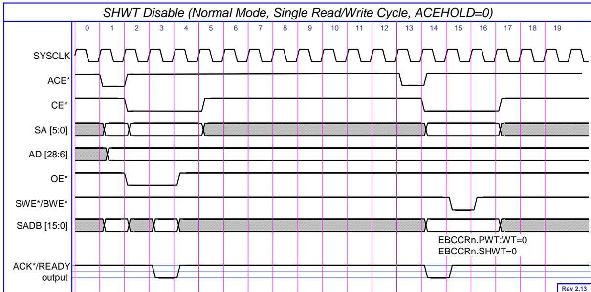
**Figure 9-6 SHWT Disable (Normal Mode, Single Read/Write Cycle)**
