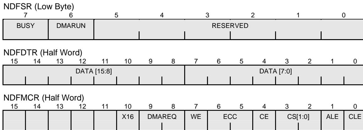
Figure 10-3 Field Definition of Registers NDFDTR and NDFMCR
