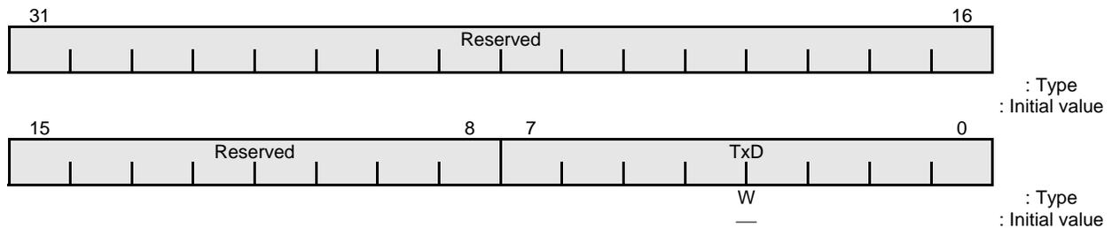
**Figure 19-13 Transmit FIFO Register**
