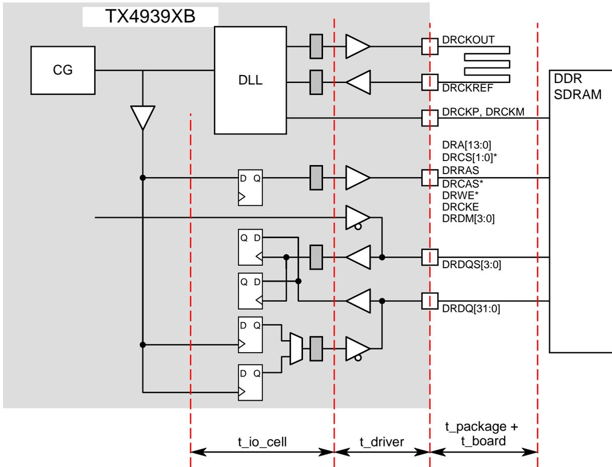
Figure 28-3 Block Diagram of DDR SDRAM Controller
