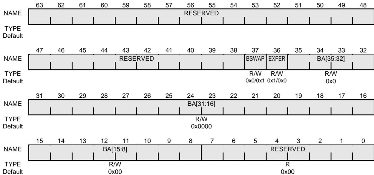
Figure 16-41 G2P Memory Space 0 G-Bus Base Address Register
