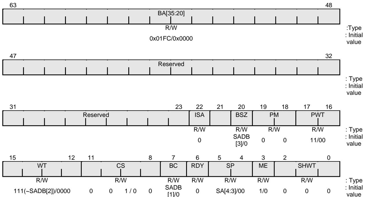
Only in the case of Channel 0 are fields with different defaults in the "Channel 0/Other channel" state. SADB[ ] represents the corresponding Data[ ] signal value when the RESET\* signal is de-asserted. SA[ ] represents the corresponding ADDR[ ] signal value when the RESET\* signal is de-asserted.
