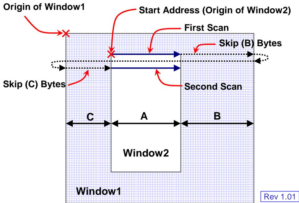
**Figure 12-9 Transmit Window 2 data to video port**
