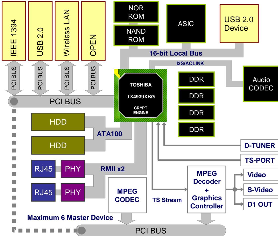
Figure 1-3 One ATA100 and Two Ethernet System
