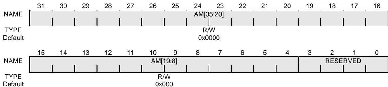
Figure 16-48 G2P I/O Space Address Mask Register
