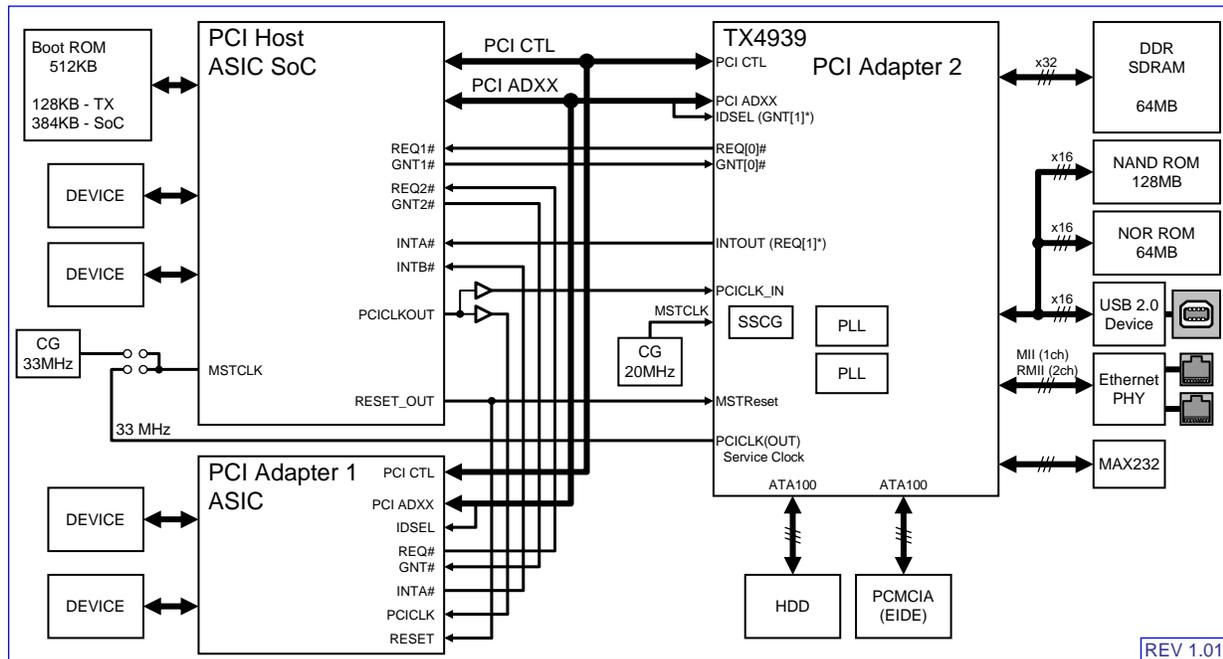
**Figure 16-3 Block Diagram of Sample PCI Adapter**
