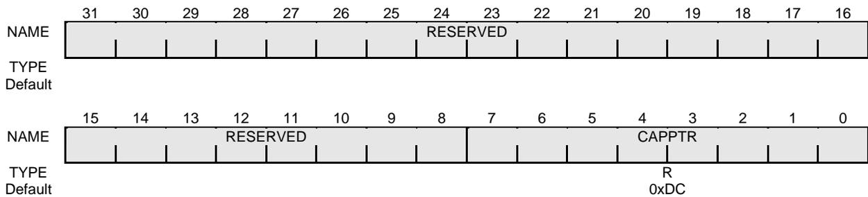
**Figure 16-22 Capabilities Pointer Register**
