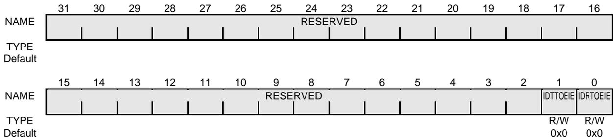
**Figure 16-26 G2P Interrupt Mask Register**
