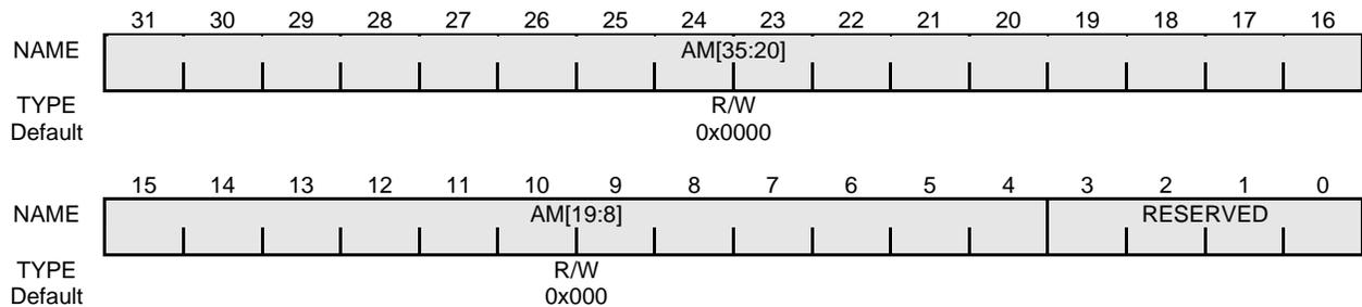
Figure 16-46 G2P Memory Space 1 Address Mask Register
