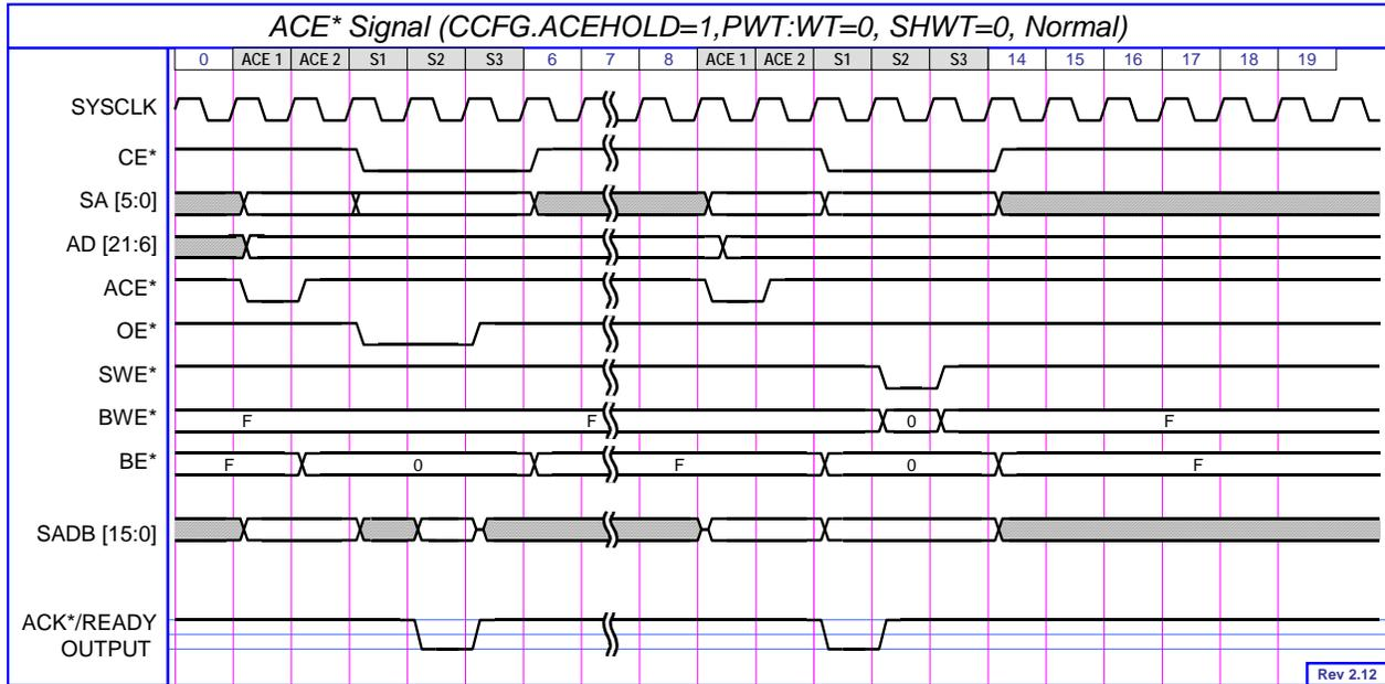
**Figure 9-15 ACE\* Signal (CCFG.ACEHOLD=1, PWT: WT=0, SHWT=0, Normal)**
