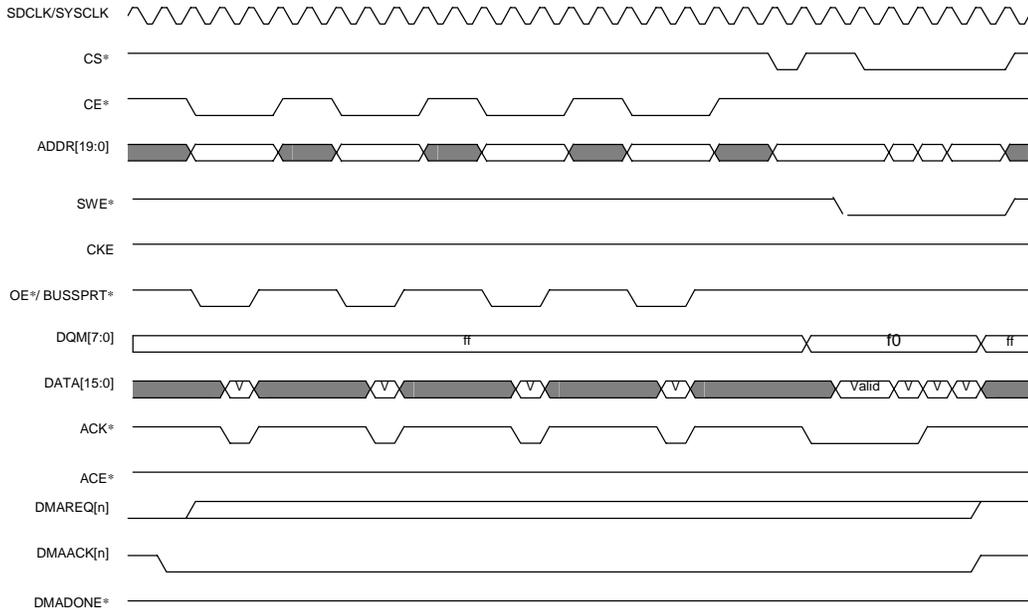
**Figure 14-22 Dual Address Transfer from External I/O Device (Non-Burst) to Memory (2-word Burst Transfer to 16-bit SRAM: Set DMCCRn.SBINH to "1")**
