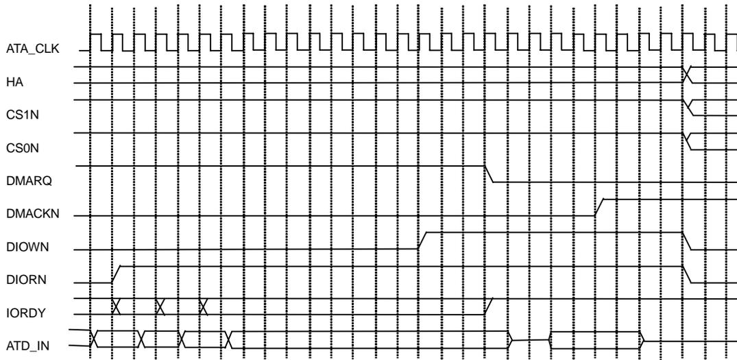
The above figure is a timing diagram that shows the transfer end position during read transfer by Ultra DMA Mode 5. Following is the flow of each control signal at the transfer end position.
