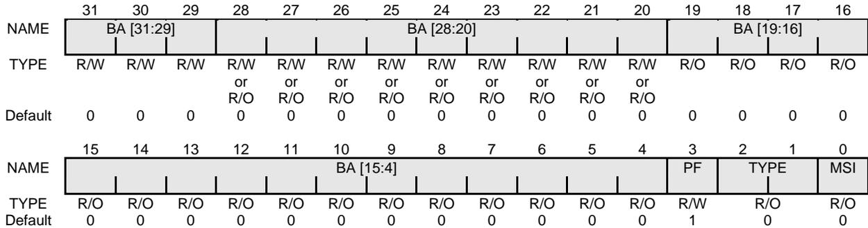
Figure 16-75 Memory Space (m) Lower Base Address Register
