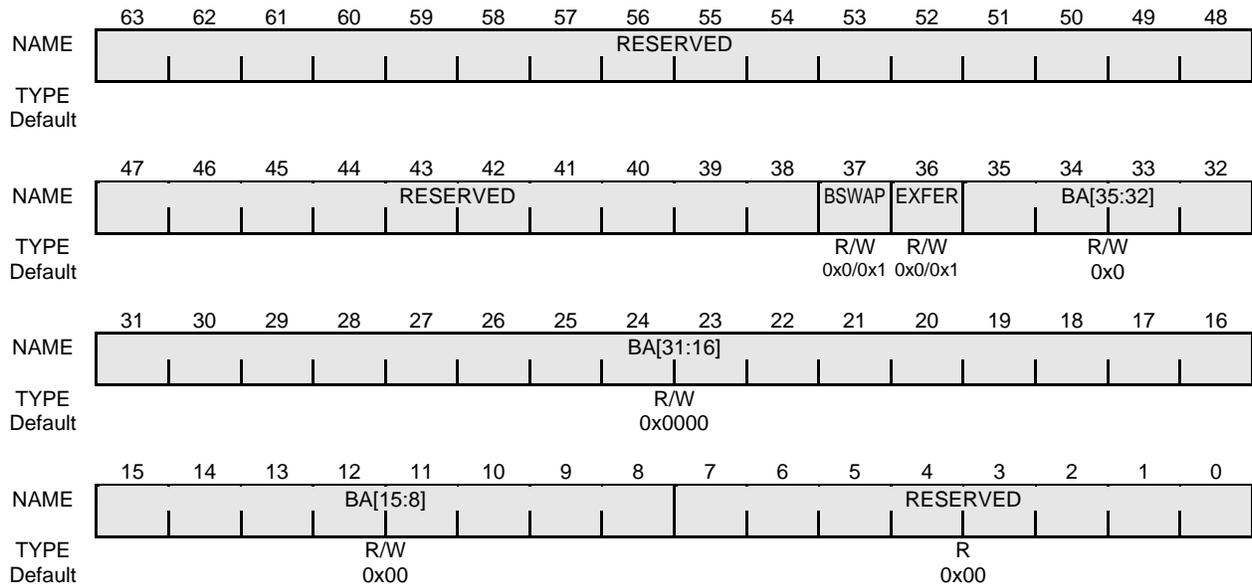
**Figure 16-42 G2P Memory Space 1 G-Bus Base Address Register**
