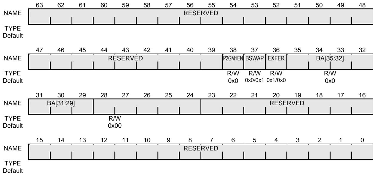
Figure 16-57 P2G Memory Space 1 G-Bus Base Address Register
