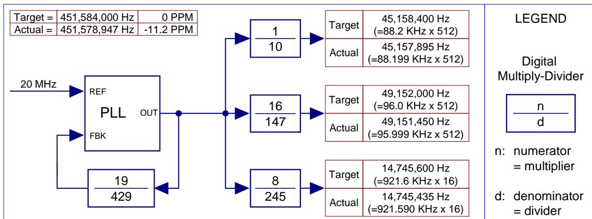
**Figure 5-4 Block Diagram of Fractional N PLL**
