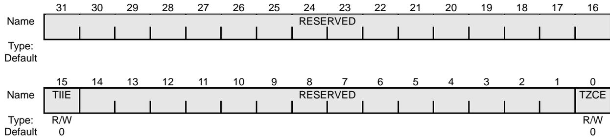
**Figure 13-11 Interval Timer Mode Register**
