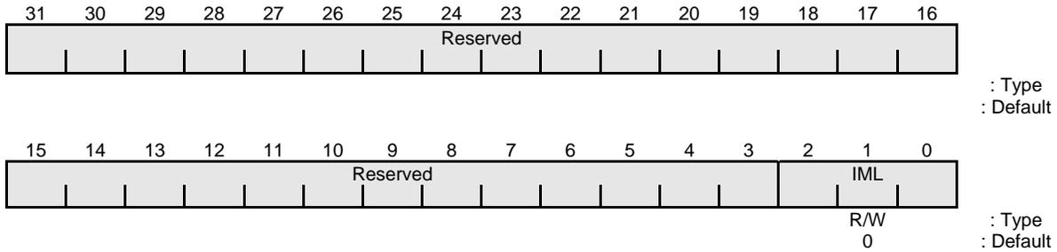
**Figure 8-10 Interrupt Mask Level Register**
