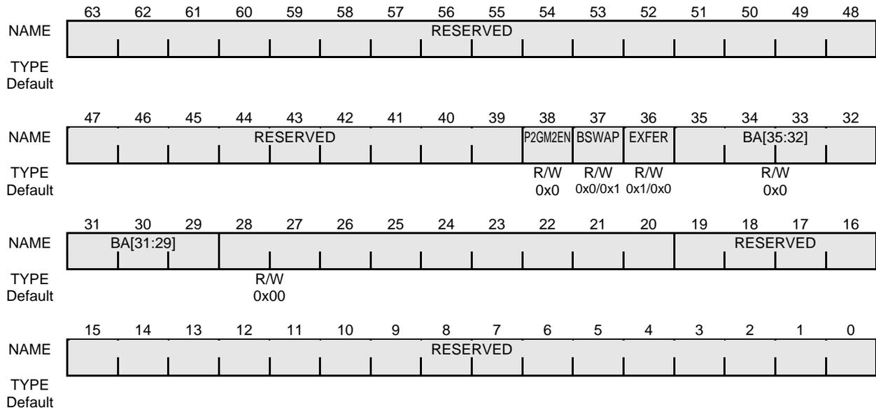
**Figure 16-58 P2G Memory Space 2 G-Bus Base Address Register**
