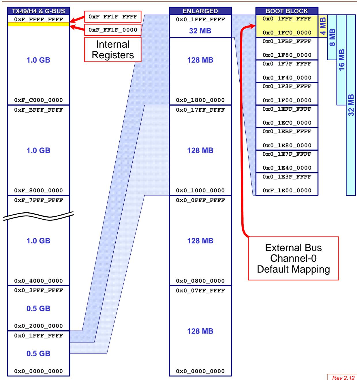
Figure 6-2 Physical Address Map at Initializing System
