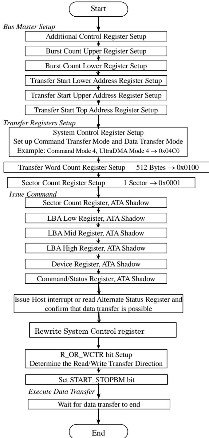
Note: R\_OR\_WCTR and START\_STOPBM of the DMA Command Start Register settings are unnecessary when a WRITE DMA, READ DMA, WRITE DMA EXT or READ DMA EXT command is issued to the device and bit [2] (Auto DMA Enable) of the System Control Register is set.
