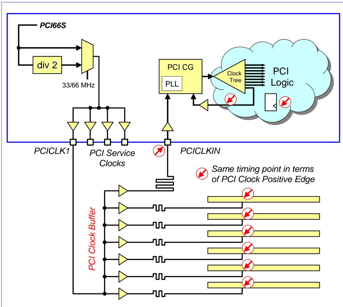
Figure 5-11 Structure of PCI Clock De-Skew Circuit
