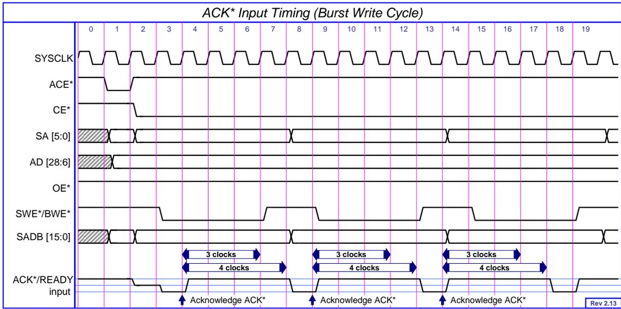
**Figure 9-11 ACK\* Input Timing (Burst Write Cycle)**
