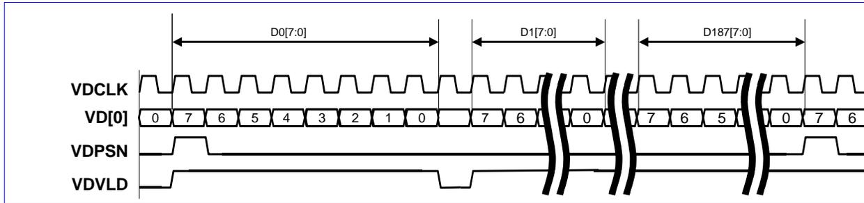
Figure 12-6 Serial transmission format with 188 Byte packets
