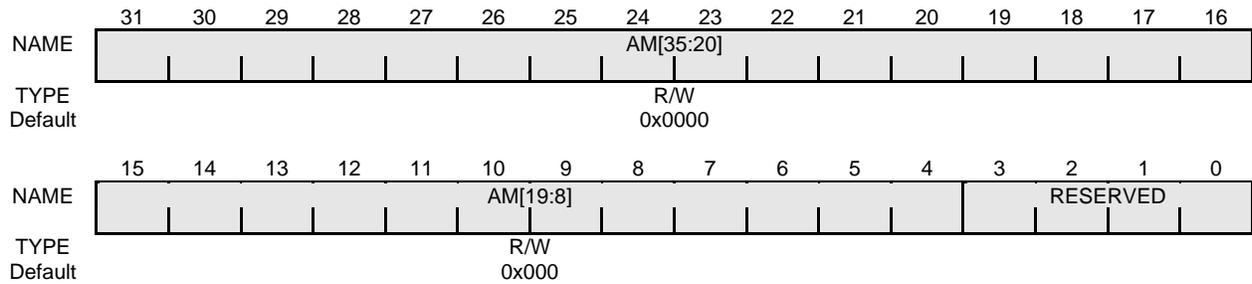
Figure 16-45 G2P Memory Space 0 Address Mask Register
