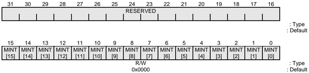
**Figure 8-20 Interrupt Request Internal Interrupt Mask Register**
