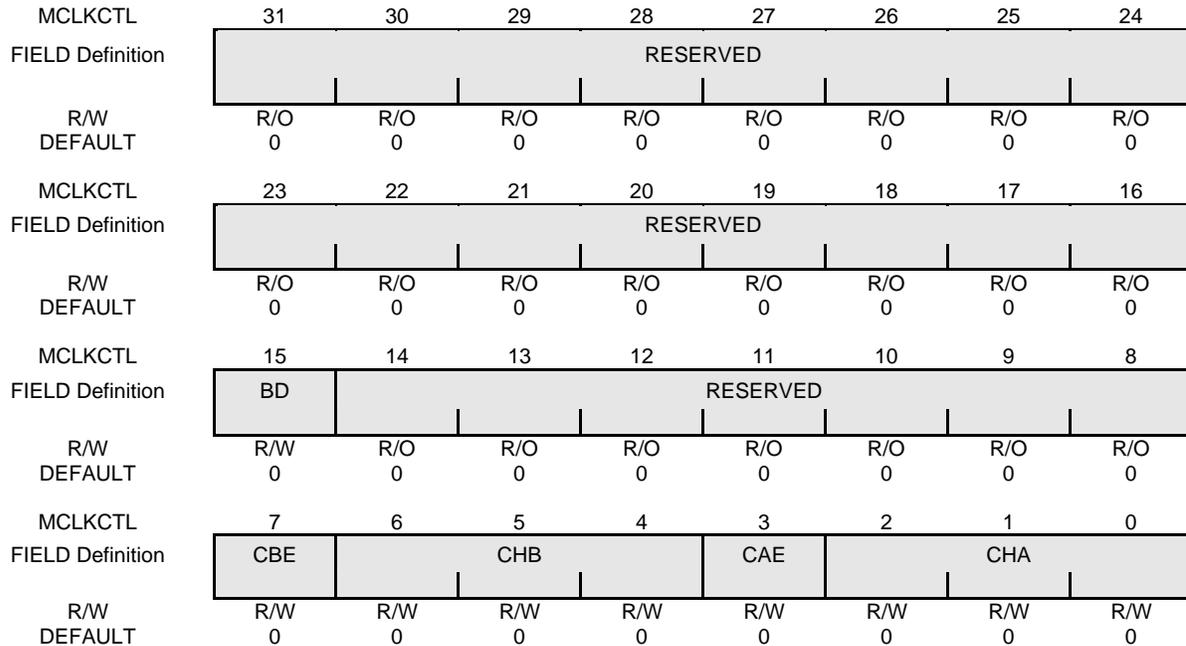
**Figure 5-7 Definition of MCLKCTL Register**
