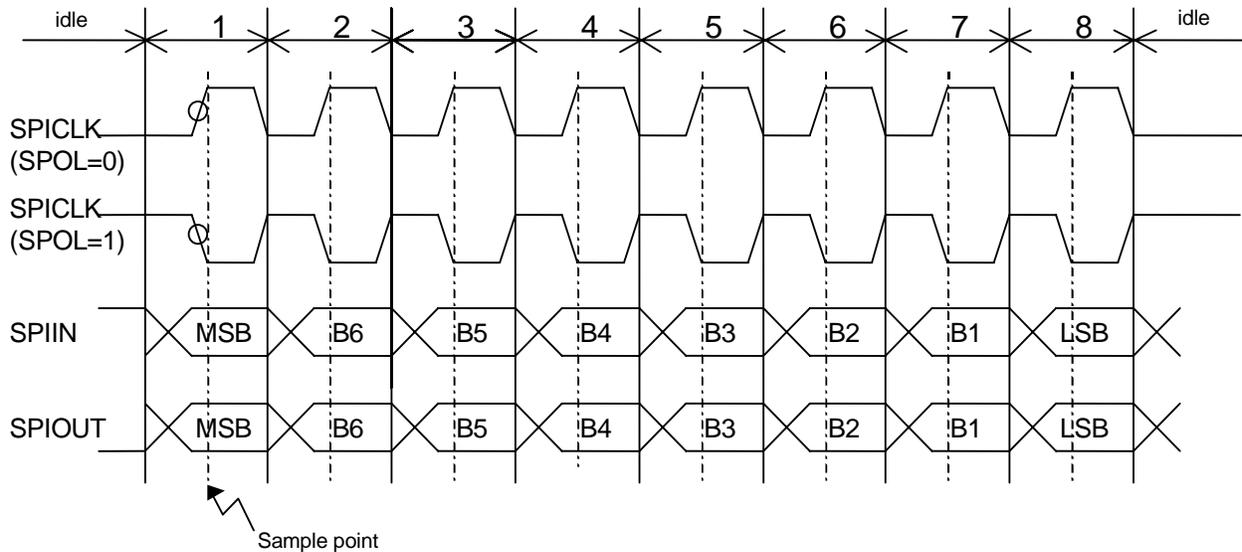
**Figure 20-2 Transfer Format when SPHA is "0"**
