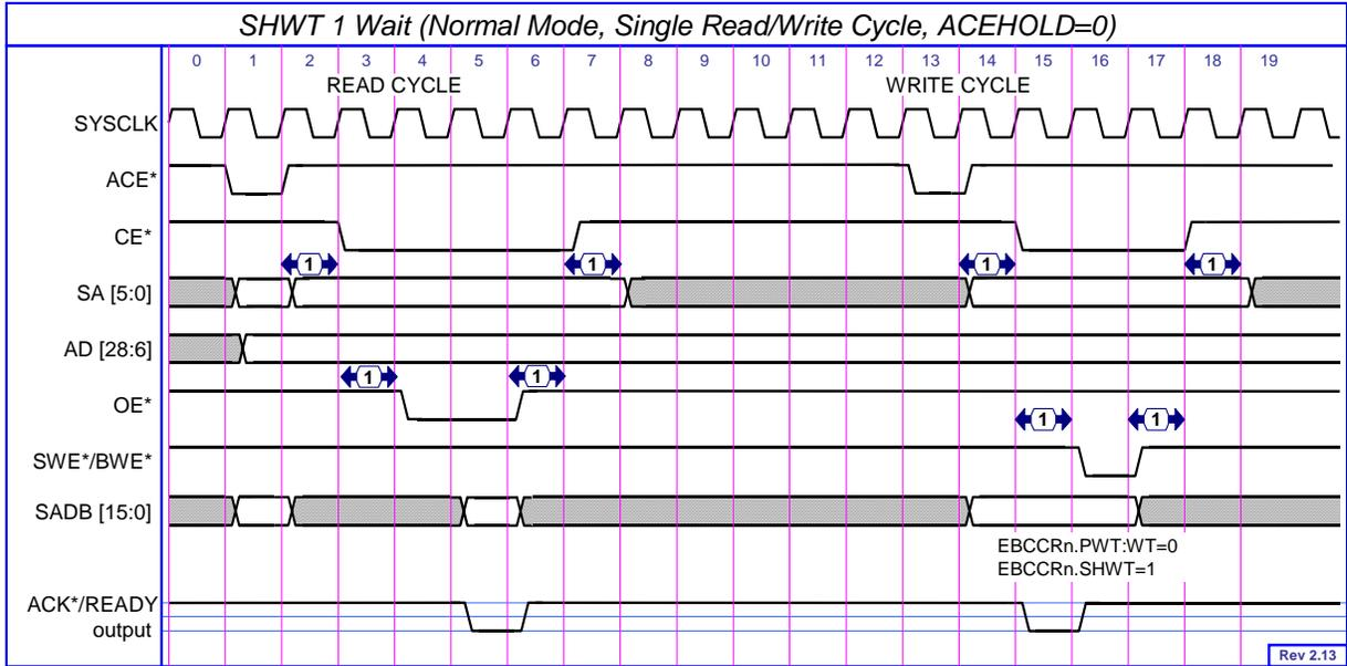
Figure 9-7 SHWT 1 Wait (Normal Mode, Single Read/Write Cycle)
