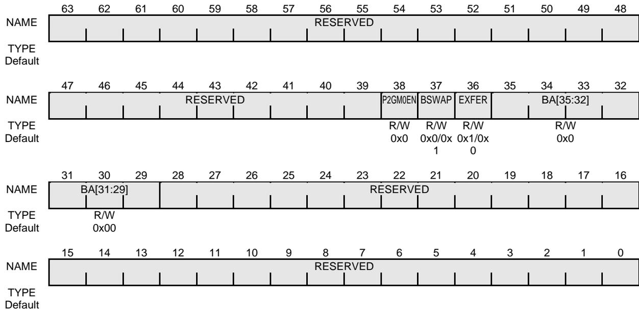
Figure 16-56 P2G Memory Space 0 G-Bus Base Address Register
