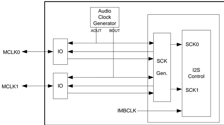
**Figure 23-2 the block diagram for I2S clock diagram.**
