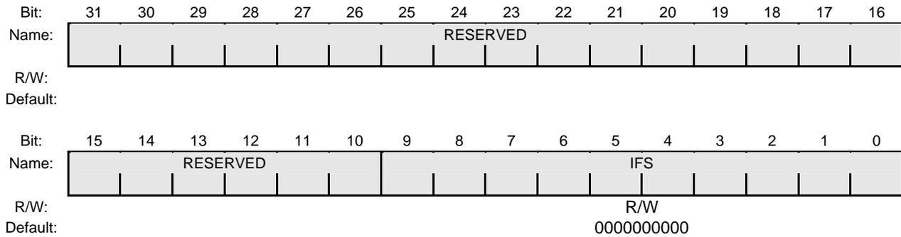
**Figure 20-7 SPI Interframe Delay Time Counter (SPFS)**
