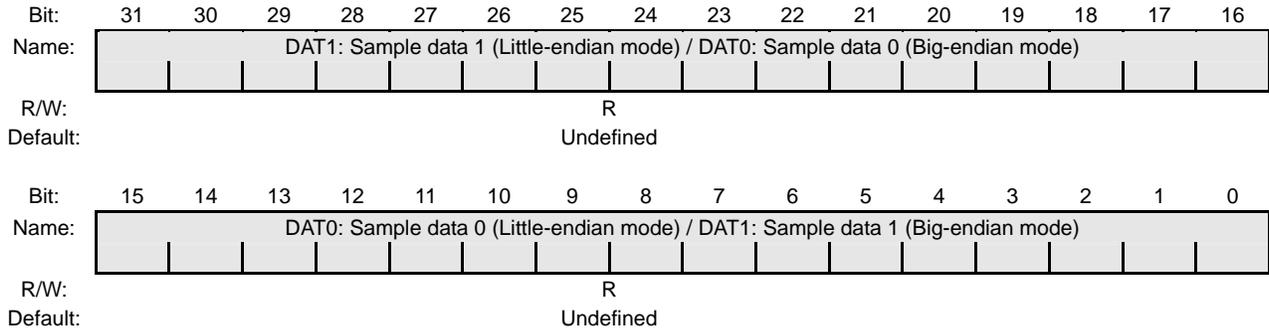
**Figure 24-24 ACMODIDAT Register**
