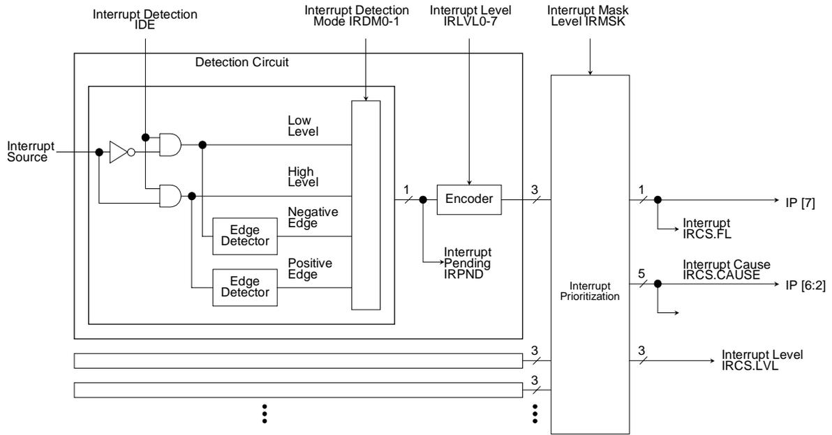
Figure 8-2 Internal Block Diagram of Interrupt Controller
