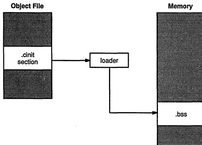
Figure 5-7. RAM Model of Autoinitialization
