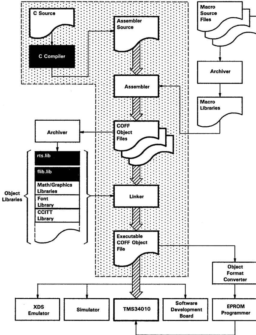
Figure 1-1. TMS34010 Software Development Flow
