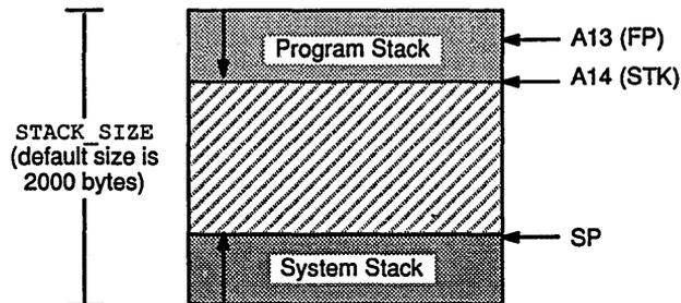
Figure 5-1. The Program and System Stacks
