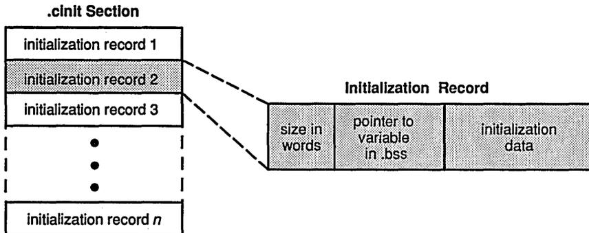
**Figure 5-5. Format of Initialization Records in the `.cinit` Section**
