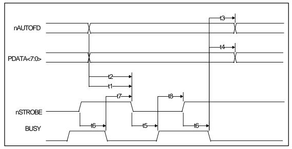
FIGURE 18 - ECP PARALLEL PORT FORWARD TIMING
