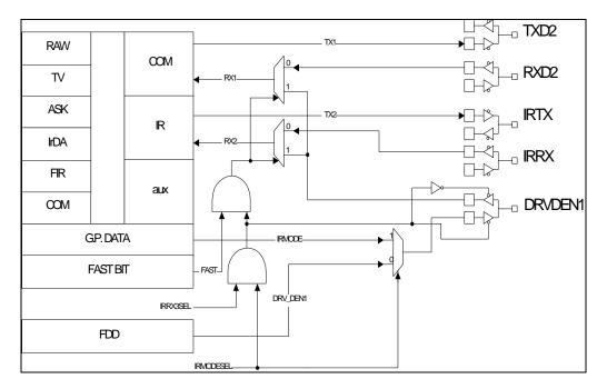
FIGURE 2 - IR INTERFACE BLOCK DIAGRAM
