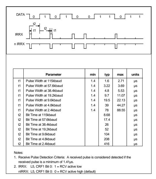
FIGURE 20 - IrDA RECEIVE TIMING
