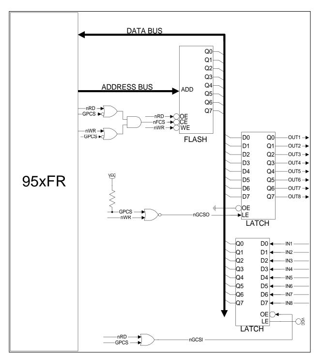
Figure 3 : Expanded GPIO Read/Write Using External Gates And Address Decoders
