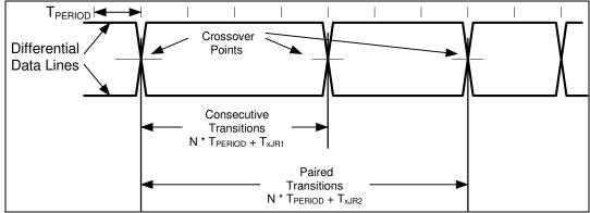
FIGURE 8 - DIFFERENTIAL DATA JITTER
