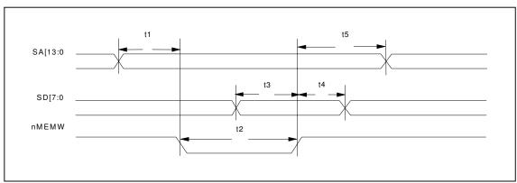
FIGURE 3 – SRAM MEMORY WRITE TIMING
