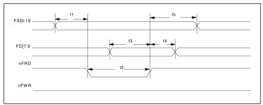
FIGURE 2 – FLASH READ TIMING
