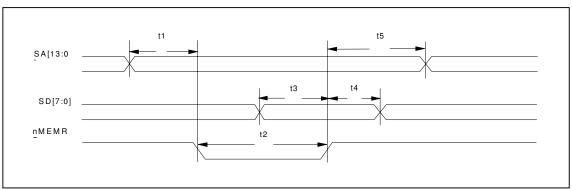
FIGURE 4 - SRAM MEMORY READ TIMING
