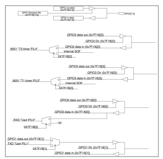
FIGURE 8 - GPIO MUXING BLOCK DIAGRAM
