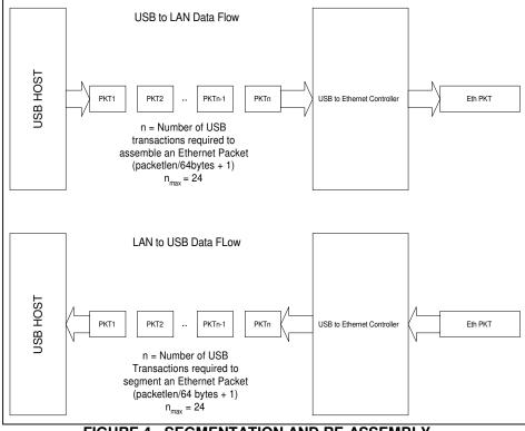
Assembly of Multiple USB Bulk Packets into an Ethernet Frame
