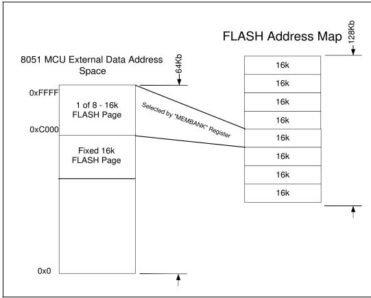
FIGURE 7 - MCU TO EXTERNAL DATA MEMORY MAP DIAGRAM
