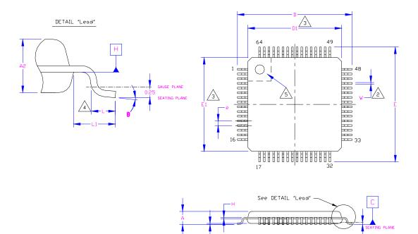
Figure 2 64 Pin STQFP Package Outline, 7x7x1.4 Body, 2 mm Footprint
