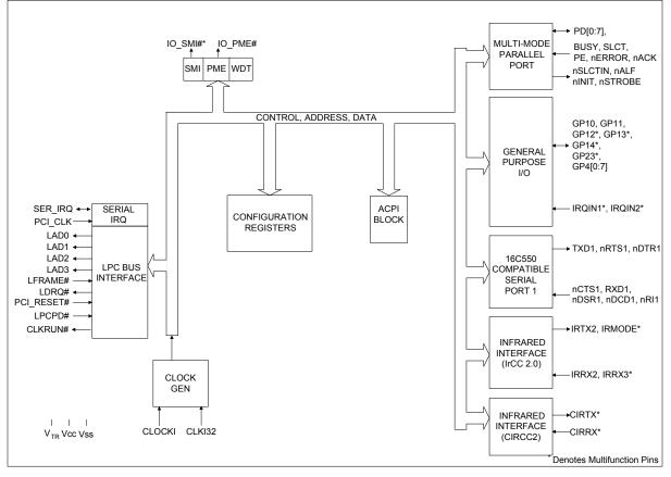
Figure 1 SIO1000 Block Diagram
