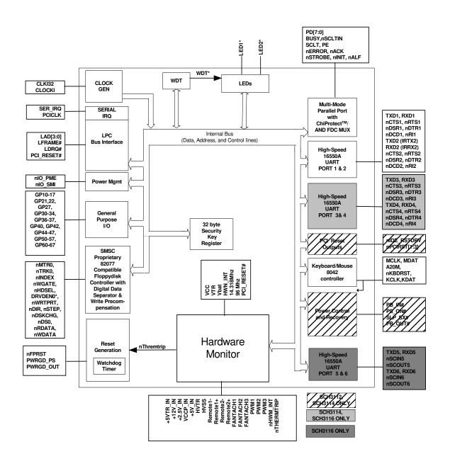
Figure 1 SCH311X Block Diagram
