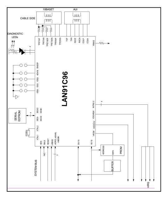
FIGURE 2 - SYSTEM DIAGRAM FOR ISA BUS WITH BOOT PROM
