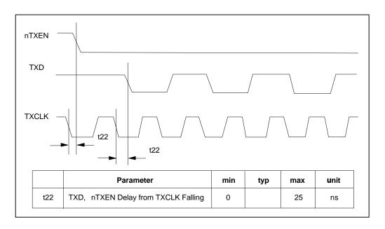
FIGURE 37 - EXTERNAL ENDEC INTERFACE - START OF TRANSMIT
