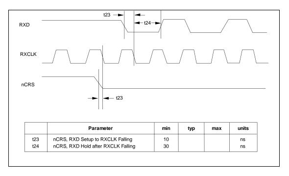
FIGURE 38 - EXTERNAL ENDEC INTERFACE - RECEIVE DATA (RXD SAMPLED BY FALLING RXCLK)
