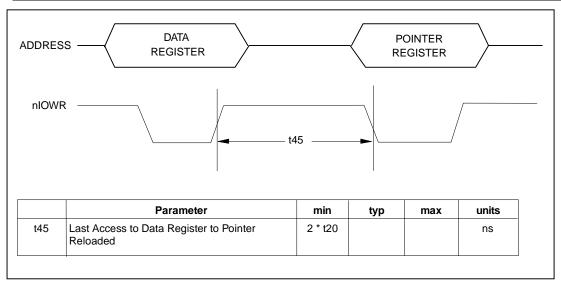
FIGURE 46 - MEMORY WRITE TIMING
