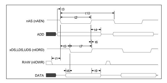
FIGURE 30 - 68000 WRITE TIMING
