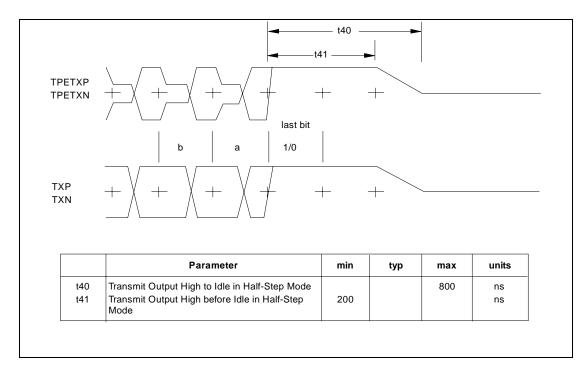
FIGURE 42 - TRANSMIT TIMING - END OF FRAME (AUI AND 10BASE-T)
