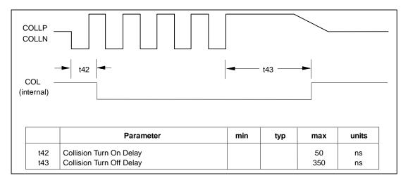
FIGURE 43 - COLLISION TIMING (AUI)
