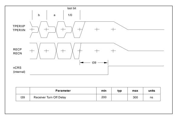
FIGURE 41 - RECEIVE TIMING - END OF FRAME (AUI AND 10BASE-T)
