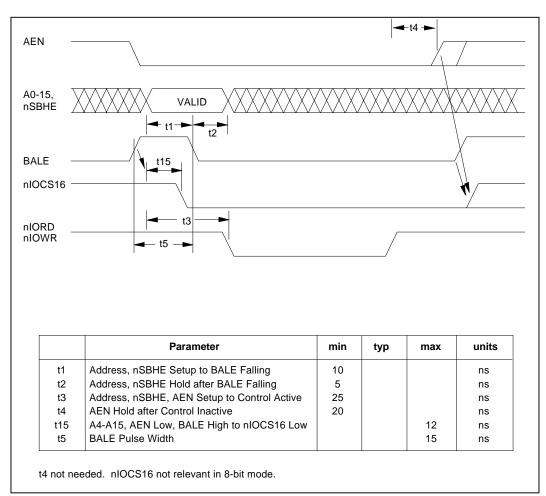
FIGURE 32 - ISA REGISTER ACCESS WHEN USING BALE
