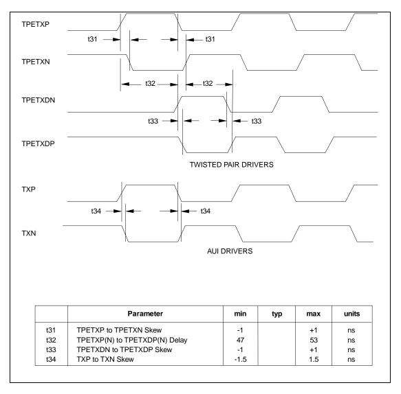
FIGURE 39 - DIFFERENTIAL OUTPUT SIGNAL TIMING (10BASE-T AND AUI)
