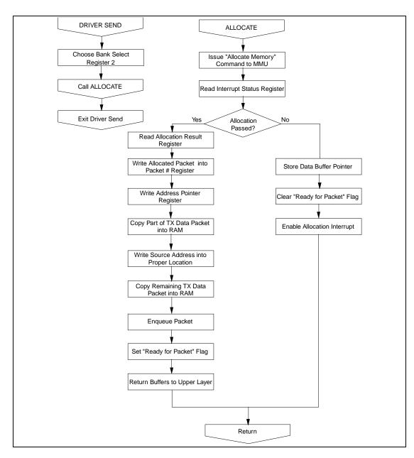
FIGURE 16 - DRIVER SEND AND ALLOCATE ROUTINES
