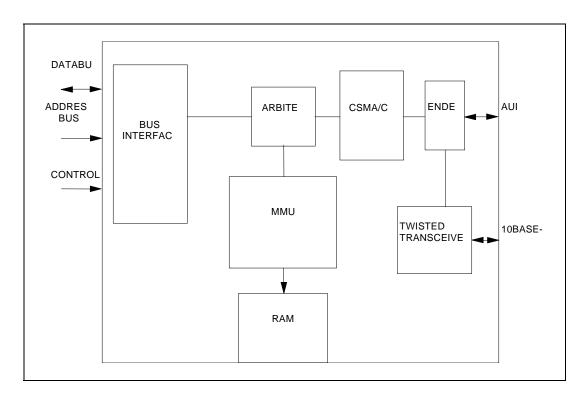
FIGURE 3 - LAN91C96 INTERNAL BLOCK DIAGRAM
