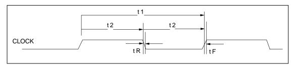
FIGURE 45 – INPUT CLOCK TIMING
