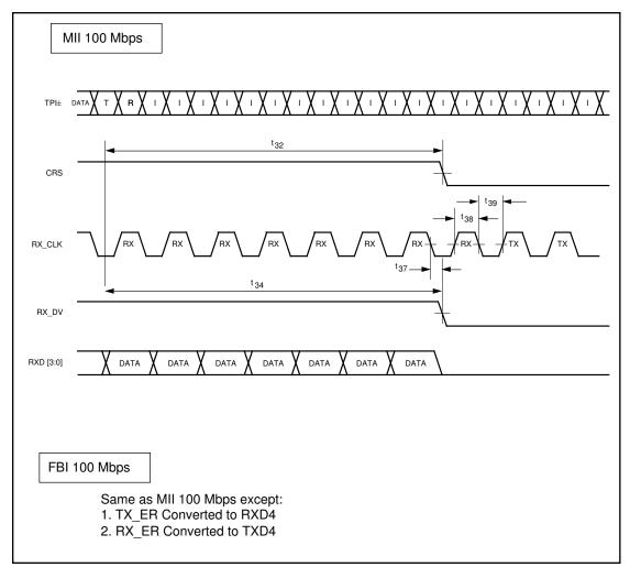
FIGURE 22 - RECEIVE TIMING, END OF PACKET - 100 Mbps
