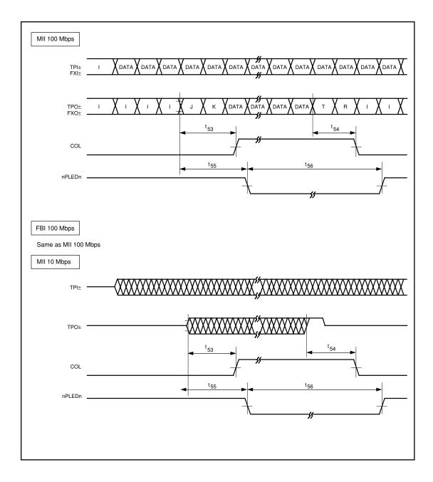
FIGURE 27 - COLLISION TIMING, TRANSMIT
