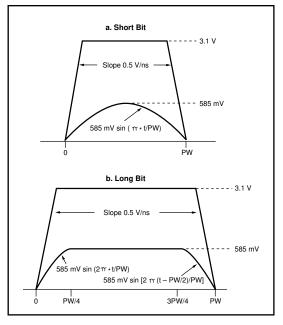
FIGURE 5 -TP INPUT VOLTAGE TEMPLATE-10MBPS
