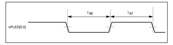
FIGURE 33 - LED DRIVER TIMING
