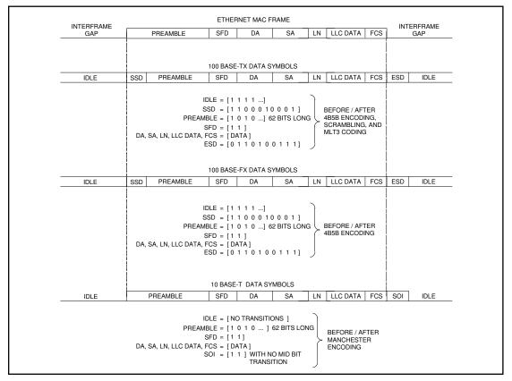
FIGURE 2 - TX/FX/10BT FRAME FORMAT
