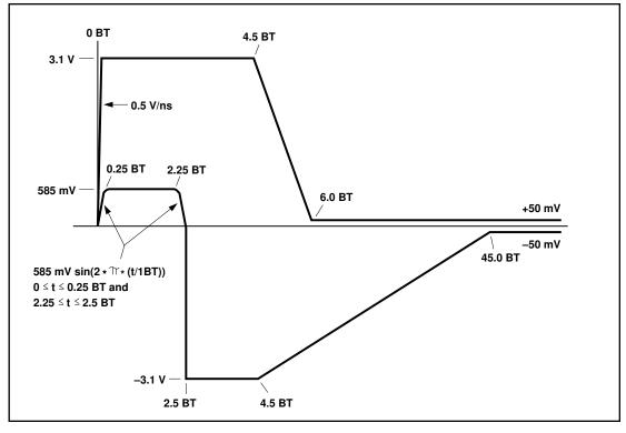
FIGURE 6 - SOI OUTPUT VOLTAGE TEMPLATE - 10 MBPS
