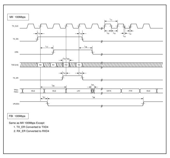
FIGURE 19 - TRANSMIT TIMING - 100 Mbps
