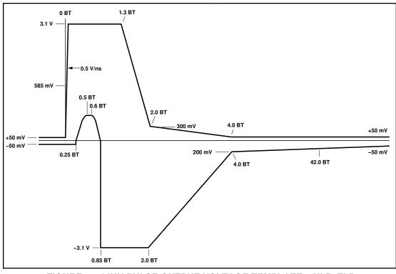
FIGURE 7 - LINK PULSE OUTPUT VOLTAGE TEMPLATE \_ NLP, FLP
