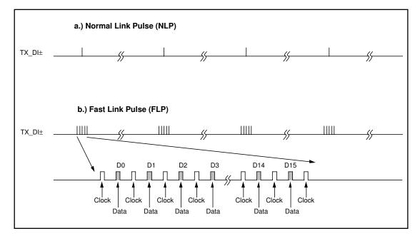
FIGURE 8 - NLP VS. FLP LINK PULSE
