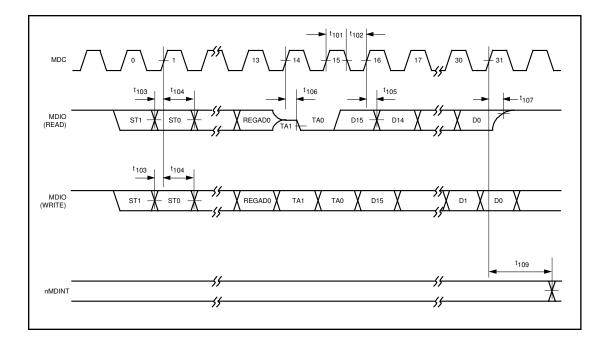
FIGURE 34 - MI SERIAL PORT TIMING
