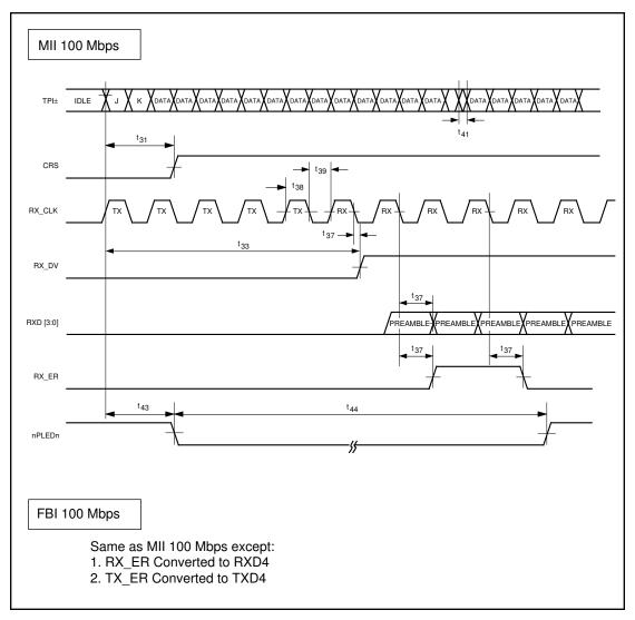
FIGURE 21 - RECEIVE TIMING, START OF PACKET - 100 Mbps
