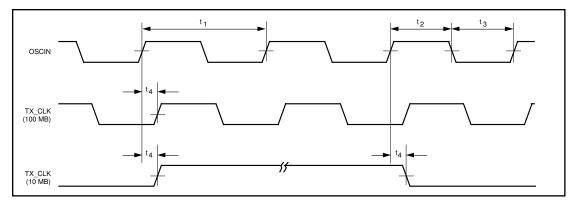
FIGURE 18 - 25 MHZ OUTPUT TIMING
