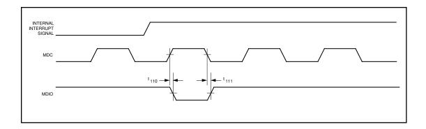
Figure 35 - MDIO Interrupt Pulse Timing
