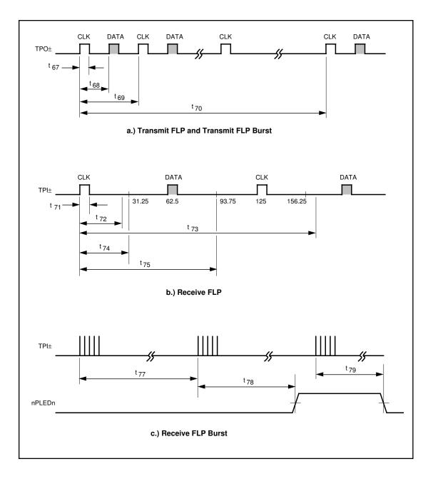
FIGURE 31 - FLP LINK PULSE TIMING
