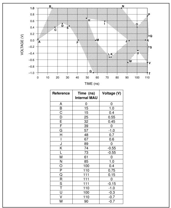
FIGURE 4 - TP OUTPUT VOLTAGE TEMPLATE-10 MBPS
