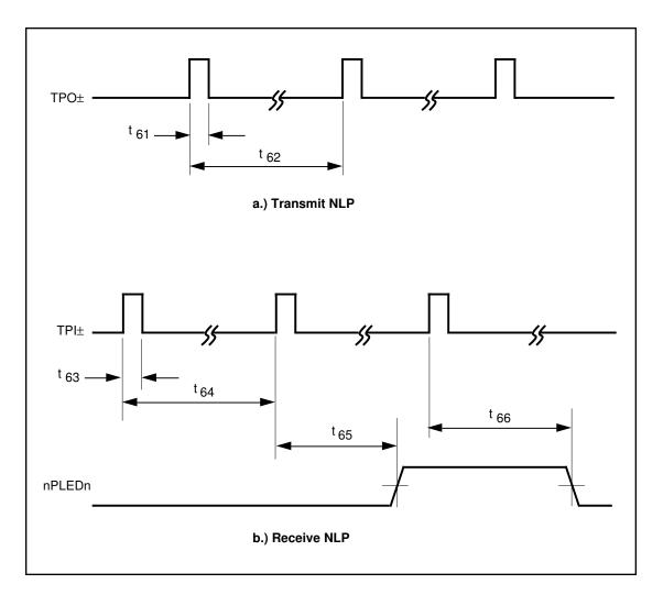
FIGURE 30 - NLP LINK PULSE TIMING
