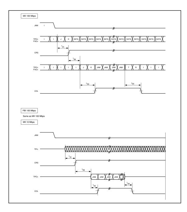
**FIGURE 29 - JAM TIMING**
