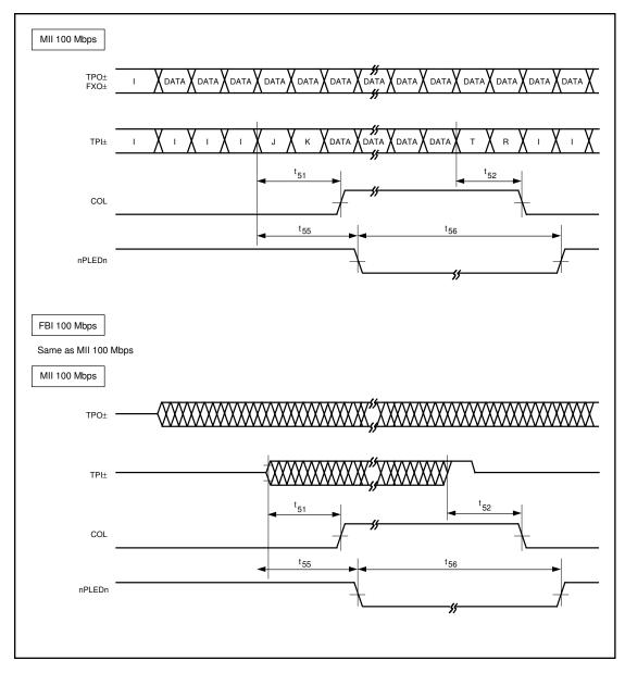
FIGURE 26 - COLLISION TIMING, RECEIVE
