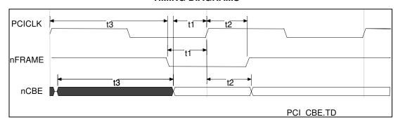
FIGURE 6 - PCI COMMAND TIMING
