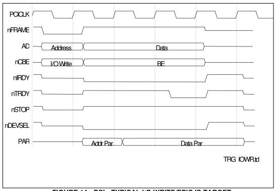
FIGURE 14 - PCI - TYPICAL I/O WRITE/EPIC IS TARGET
