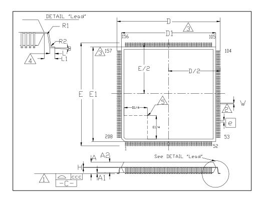
FIGURE 23 - 208 PIN PQFP PACKAGE OUTLINE, 2.6 MM FOOTPRINT
