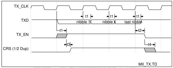
FIGURE 17 - MII - TRANSMIT TIMING FOR 10/100Mb/s
