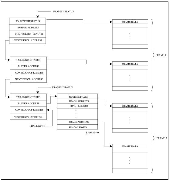
FIGURE 3 - TRANSMIT BUFFER STRUCTURE
