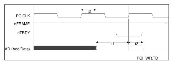
FIGURE 10 - PCI/DATA WRITE TIMING
