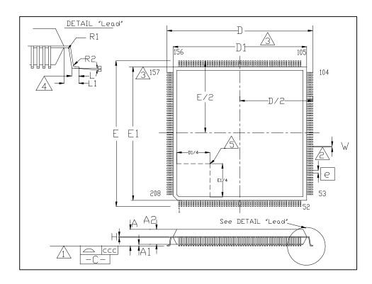
FIGURE 24 - 208 PIN PQFP PACKAGE OUTLINE, 2.6 MM FOOTPRINT
