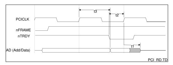
FIGURE 9 - PCI/DATA READ TIMING
