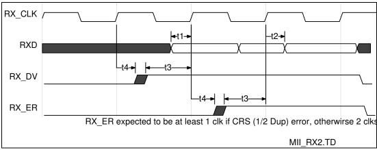
FIGURE 19 - MII - RECEIVE ERROR (RX\_ER) TIMING FOR 100Mb/s
