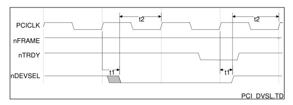
FIGURE 7 - PCI/nDEVSEL TIMING
