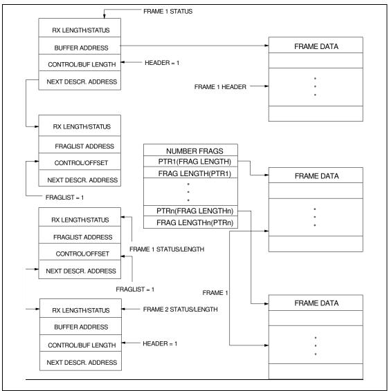
FIGURE 4 - RECEIVE BUFFER STRUCTURE
