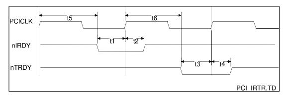
FIGURE 8 - PCI/nIRDY AND nTRDY TIMING
