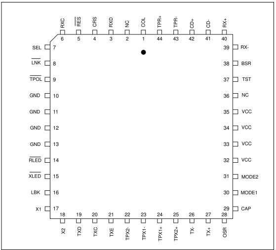
FIGURE 3-1. 83C694C 44-PIN PLCC PACKAGE DRAWING
