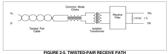
The 83C694D supports the IEEE 802.3 loopback design (section 14.2.1.3) which provides for continuous loopback from transmit to receive in normal operation. This means that transmitted data is always looped back during TP operation, simulating the physical broadcast characteristics of 802.3 coaxial cable networks.
