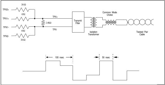
FIGURE 2-6. TWISTED-PAIR TRANSMIT PATH AND TIMING
