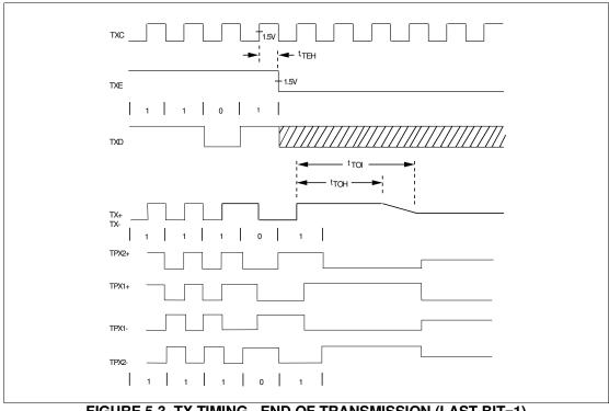
FIGURE 5-3. TX TIMING - END OF TRANSMISSION (LAST BIT=1)
