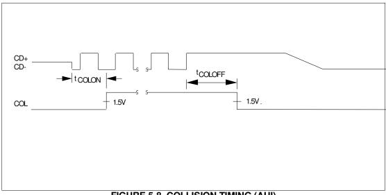
FIGURE 5-8. COLLISION TIMING (AUI)
