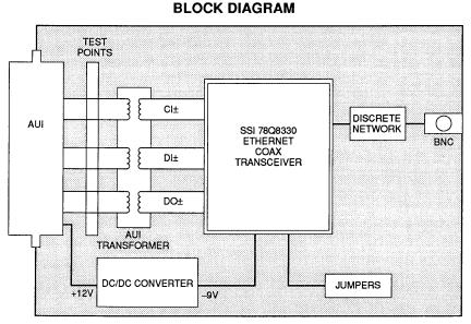
FIGURE 1: SSI 78Q8330 Demo Board Block Diagram
