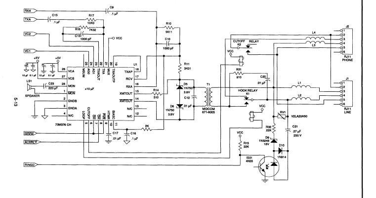
FIGURE 2: SSI 73M376 Based DAA Circuit
