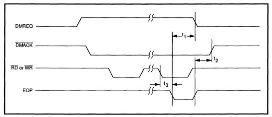
FIGURE 8: Burst DMA Terminated by EOP
