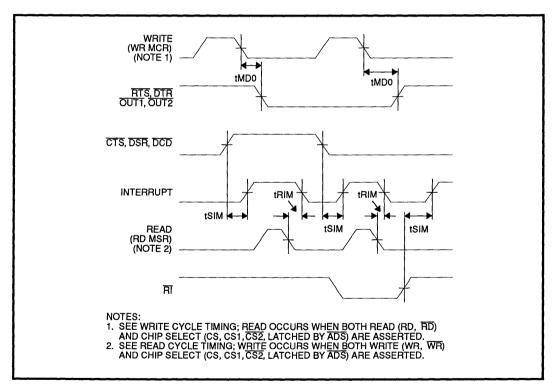
FIGURE 9: Modem Controls Timing
