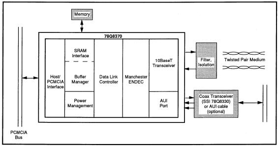
Figure 1-1: Block Diagram (78Q8370)
