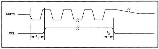
FIGURE 21: Collision Timing
