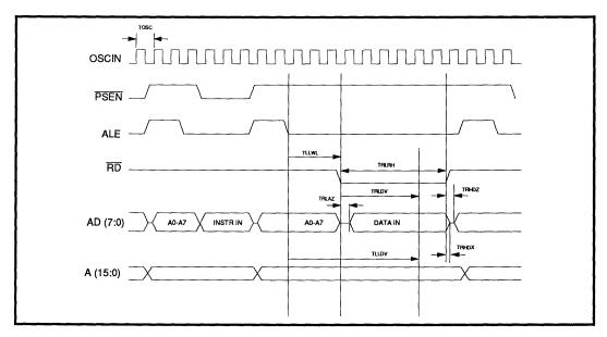
FIGURE 6: External Data Memory Read Cycle
