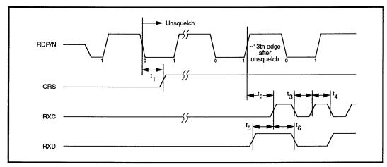
FIGURE 23: Receive Start Timing
