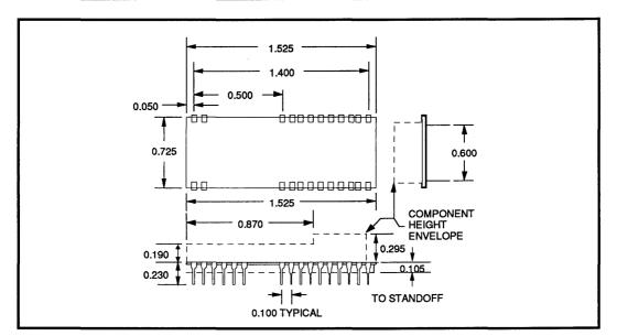
**FIGURE 2: Mechanical Specifications**
