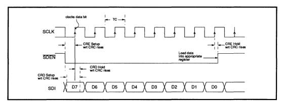
FIGURE 1: Serial Port Timing Relationship
