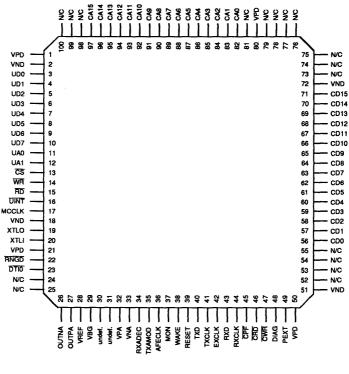
SSI 73D2920 100-Lead TQFP
