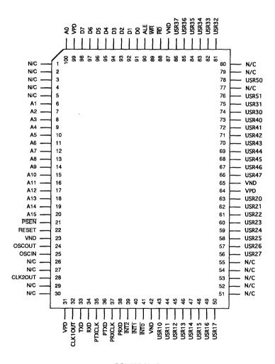
SSI 73D2910 100-Lead QFP
