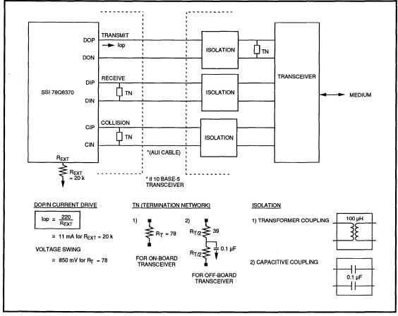
Figure 7.2. Attachment Unit Interface (AUI) Connections
