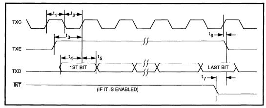
FIGURE 14: Transmit Timing
