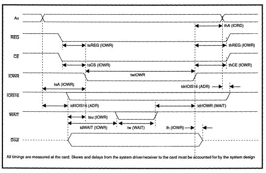
FIGURE 16: I/O Output Timing Specification (WRITE)
