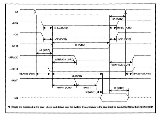
FIGURE 17: I/O Output Timing Specification (READ)
