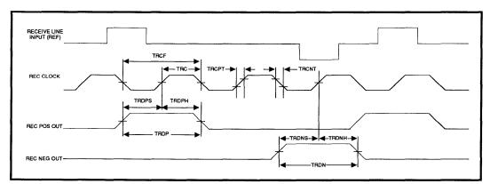
**FIGURE 2: Receive Waveforms**
