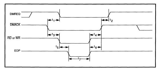
FIGURE 5: Single-Cycle DMA Timing
