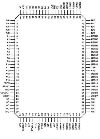
SSI 73D246 Controller 100-Lead QFP
