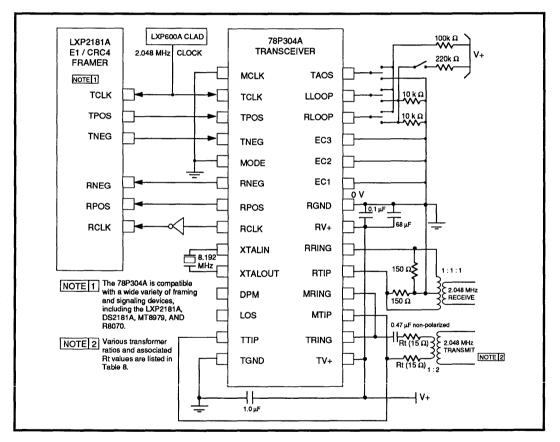
FIGURE 9: SSI 78P304A 2.048 MHz E1 Application (Hardware Mode)
