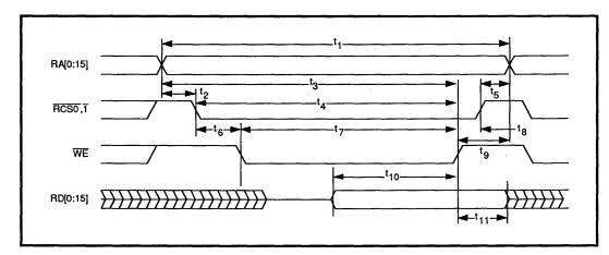
FIGURE 13: SRAM Write Timing
