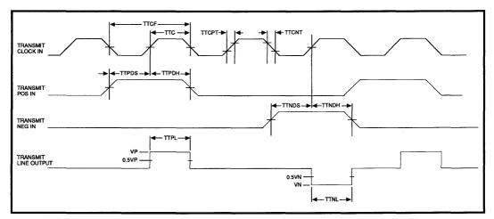
FIGURE 3: Transmit Waveforms
