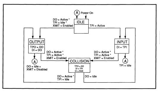
**FIGURE 2: Collision Detection Function**
