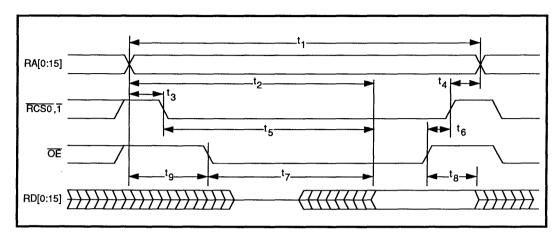
FIGURE 12: SRAM Read Timing
