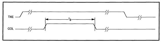
FIGURE 15: Transmit Timing
