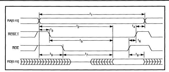
FIGURE 14: SRAM Read Timing
