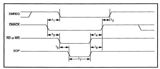
FIGURE 8: Single-Cycle DMA Timing
