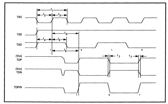
FIGURE 18: Transmit Start Timing
