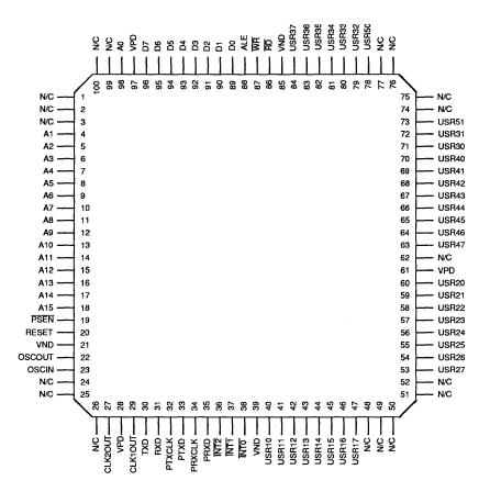
SSI 73D2910 100-Lead TQFP
