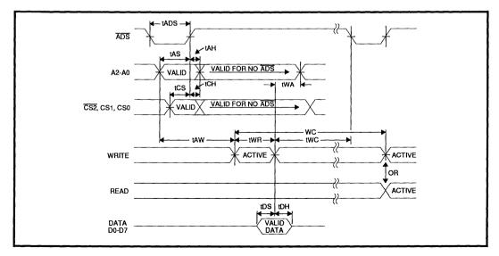
FIGURE 5: Write Cycle Timing
