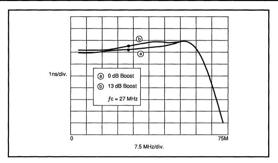
FIGURE 3: 32F8001 Group Delay Response with fc = 27 MHz
