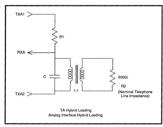
FIGURE 3: TXA Hybrid Loading Analog Interface Hybrid Loading
