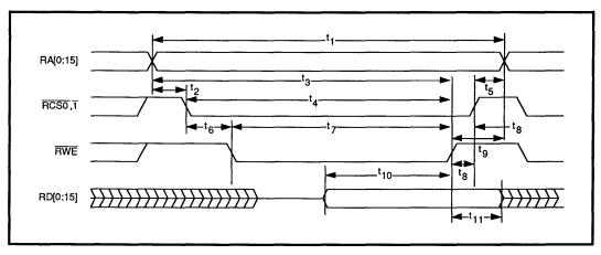
FIGURE 15: SRAM Write Timing
