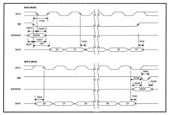
FIGURE 4: Modem Serial Bus Timing
