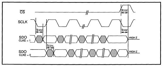
FIGURE 6: SSI 78P300 Serial Data Output Timing Diagram
