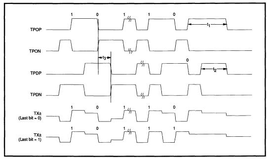
FIGURE 20: Transmit Timing (TP)
