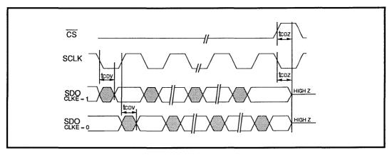
Figure 7: SSI 78P304A Serial Data Output Timing Diagram
