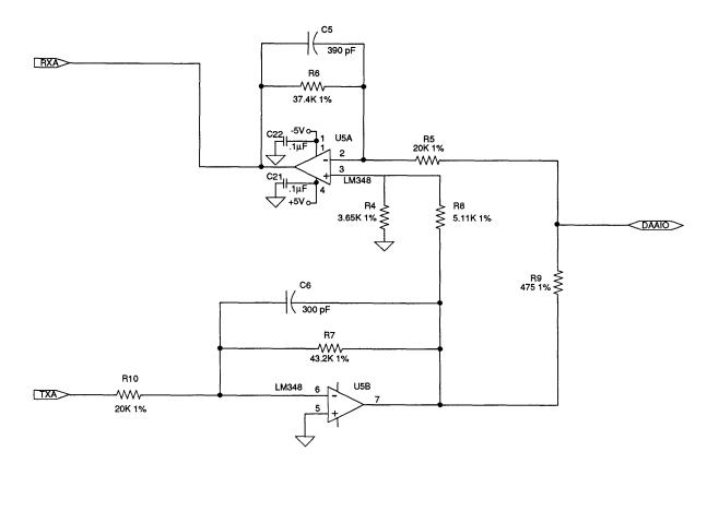
FIGURE 3: SSI 73D2240 Hybrid
