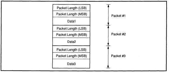
Figure 2-3: Packet Format in Transmit Buffer
