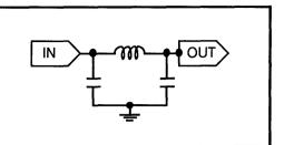
FIGURE 9: Receive Filter Diagram
