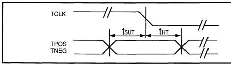
FIGURE 1: 78P300 Transmit Clock Timing Diagram
