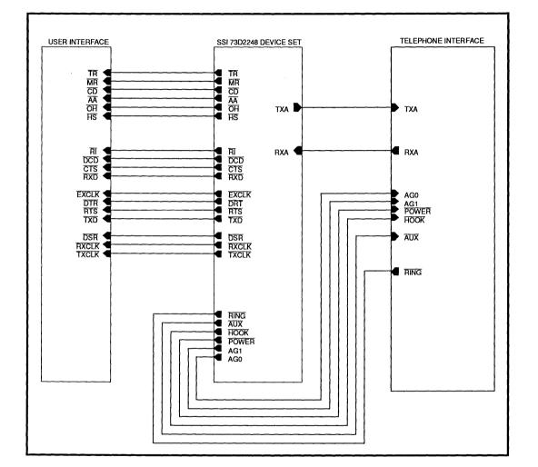
FIGURE 13: Modem Block Diagram
