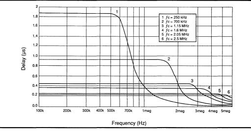
FIGURE 3: Typical Normal/Differentiated Output Group Delay Response
