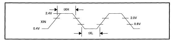
FIGURE 2: External Clock Input\* (8 MHz Maximum)
