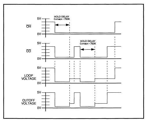
FIGURE 1: Relay Hold and Power Down Timing Diagrams
