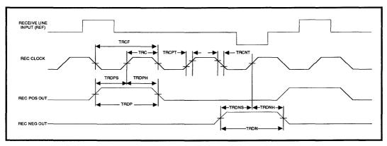
FIGURE 2: Receive Waveforms
