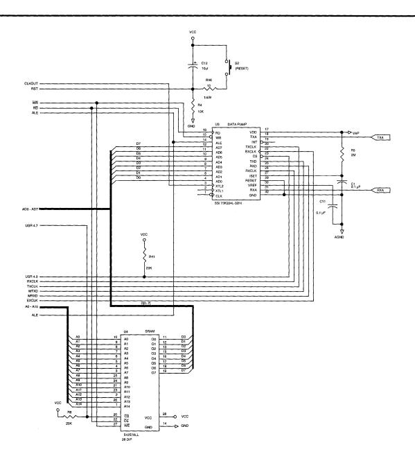
FIGURE 16B: 2248 Modem System Interconnect - Back End
