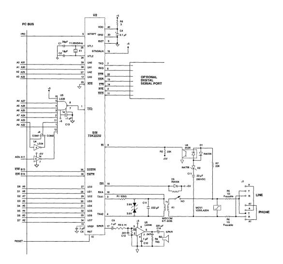
FIGURE 9: 73K22U Typical Integral Application Single-Port Mode
