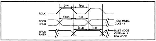
FIGURE 3: 78P300 Receive Clock Timing Diagram
