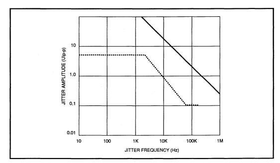
FIGURE 3: Jitter Tolerance for 78P236
