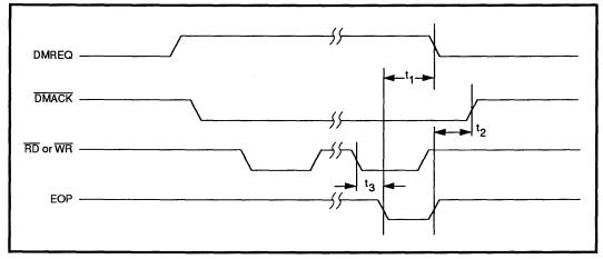
FIGURE 11: Burst DMA Terminated by EOP
