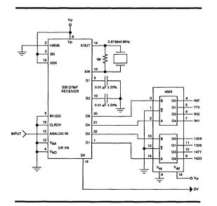
FIGURE 14: Touch-Tone™ to 2-of-8 Output Converter
