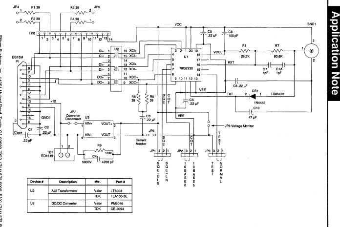
FIGURE 3: Schematics of 78Q8330 Demo Board
