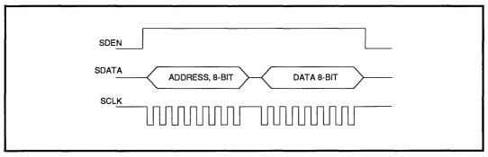
FIGURE 2: Serial Port Data Transfer Format
