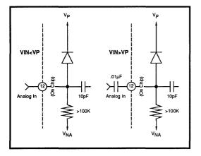
**FIGURE 1: Input Coupling**
