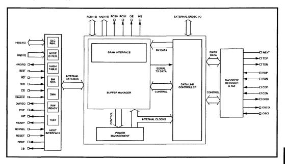
FIGURE 2: 78Q8360 Block Diagram
