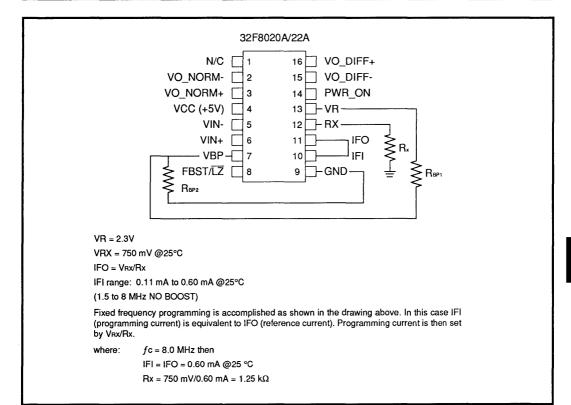
FIGURE 1: 32F8020A/8022A Applications Setup
