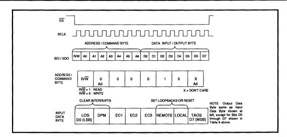
FIGURE 5: SSI 78P304A Serial Interface Data Structure
