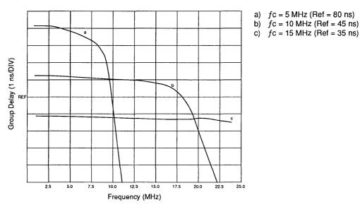
FIGURE 8: 32F8011/8012 Typical Group Delay Variation (Normal Low Pass Output) Maximum Boost
