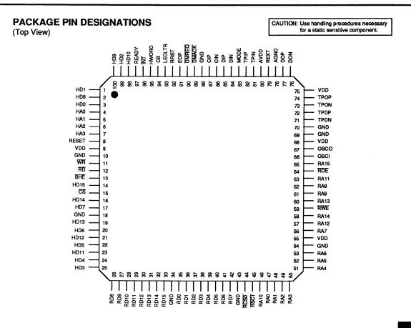
100-Lead TQFP Generic Bus Mode
