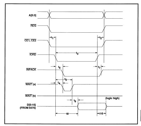
FIGURE 4. I/O Read Cycle (PCMCIA mode)
