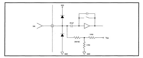
FIGURE 1: VIN Equivalent Input Circuit
