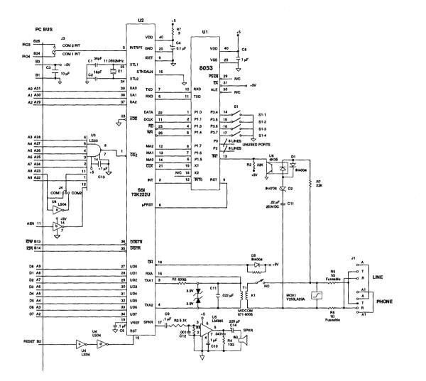
FIGURE 10: 73K22U Typical Integral Application Dual-Port Mode
