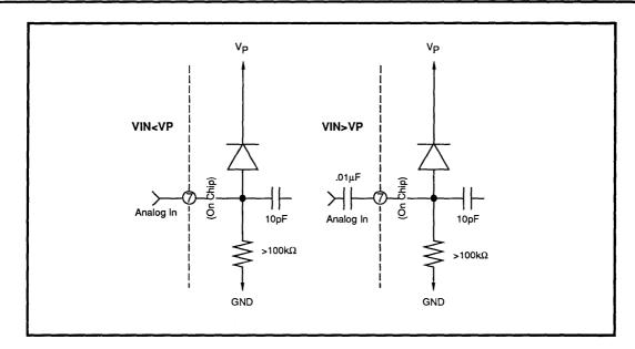
FIGURE 1: Input Coupling
