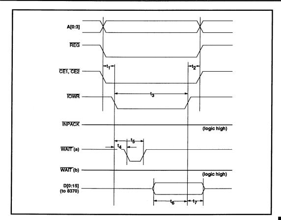
FIGURE 5: I/O Write Cycle (PCMCIA mode)
