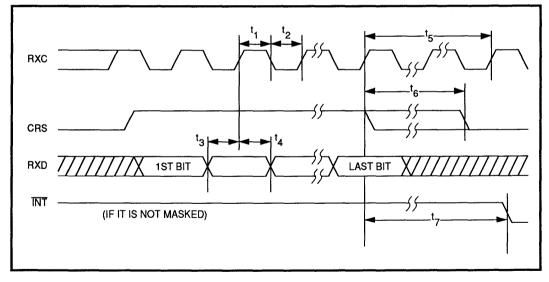
FIGURE 22: Receive Timing
