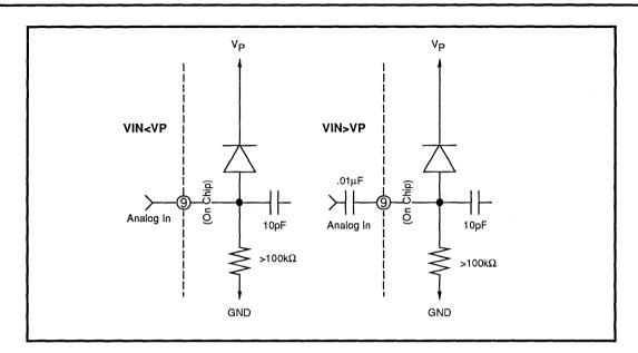
FIGURE 1: Input Coupling
