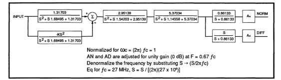
FIGURE 1: 32F8101/8102/8103/8104 Normalized Block Diagram
