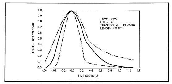
FIGURE 5: Transmitter Pulse Shape for 78P236
