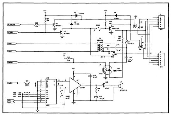
FIGURE 2: Telephone Interface Circuit
