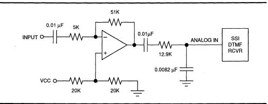
FIGURE 5: Filter for Use in Environments where a Third Tone Exists
