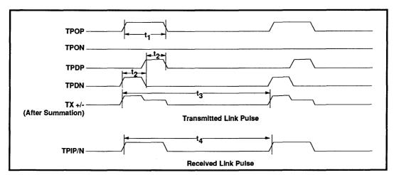
FIGURE 21: Link Test Timing
