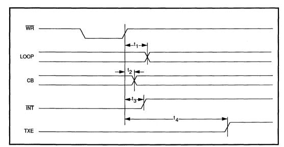
FIGURE 11: LOOP, CB and INT Timing
