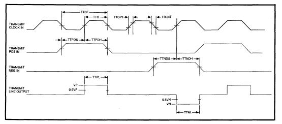
**FIGURE 3: Transmit Waveforms**
