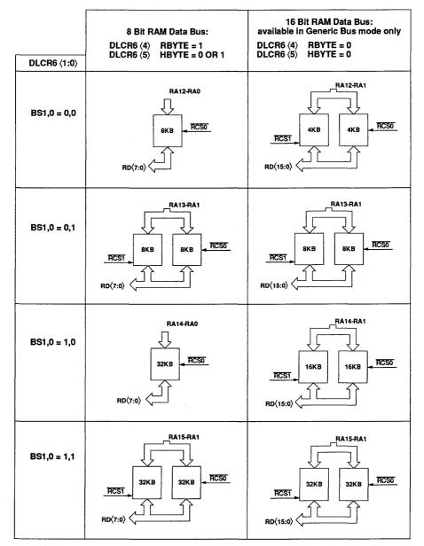
Figure 2-2: SRAM Configurations
