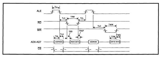
FIGURE 1: Bus Timing Diagram (Parallel Version)
