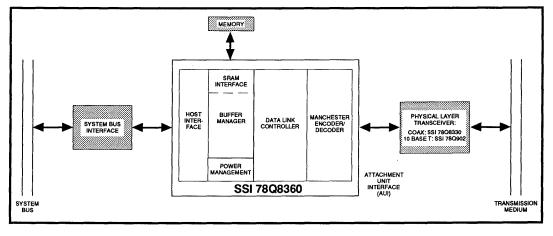
FIGURE 1: System Diagram
