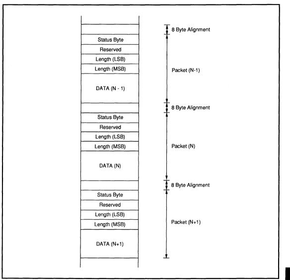
Figure 2-5: Packet Format in Receive Buffer
