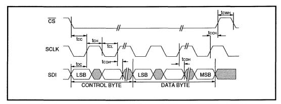
FIGURE 6: SSI 78P304A Serial Data Input Timing Diagram
