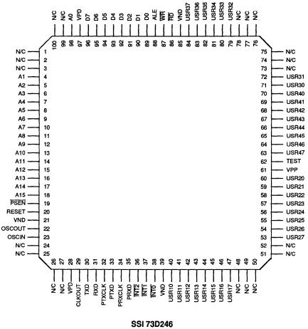
SSI 73D246 Controller 100-Lead TQFP
