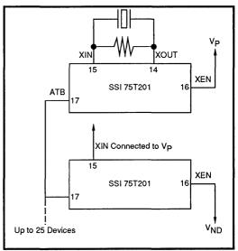
**FIGURE 2: Crystal Connections**
