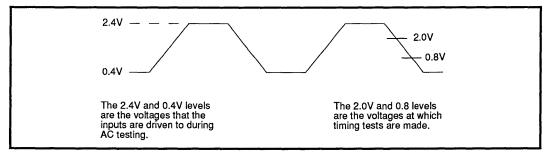
FIGURE 3: AC Test Points\*
