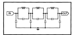
FIGURE 8: Transmit Filter Diagram
