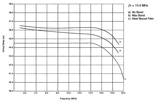
FIGURE 3: 32F8011/8012 Typical Group Delay Variation (Differentiated Output)
