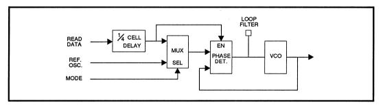
FIGURE 17A: Standard Configuration of a Data Synchronizer Phase-Locked Loop
