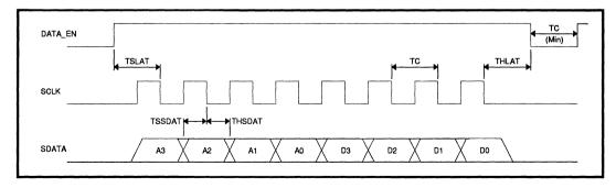
FIGURE 3: Serial Data Interface Timing
