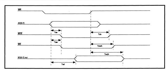
FIGURE 11: Register 70H Write Timing
