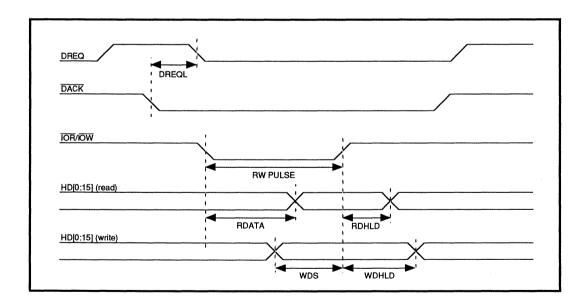
FIGURE 1: Host DMA 8/16-Bit Interface Timing
