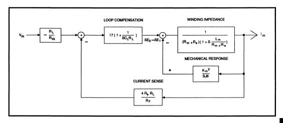
FIGURE 4(A): Transfer Function of SSI 32H6230 in Typical Application with Fixed Field DC Motor
