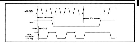
FIGURE 1: Write Mode Timing Diagram
