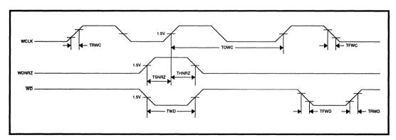
FIGURE 5: Write Timing
