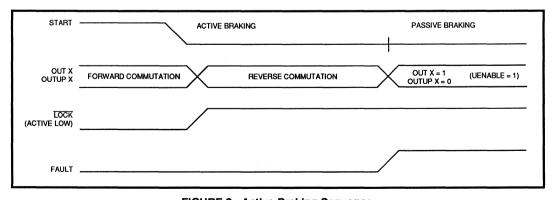
FIGURE 3: Active Braking Sequence
