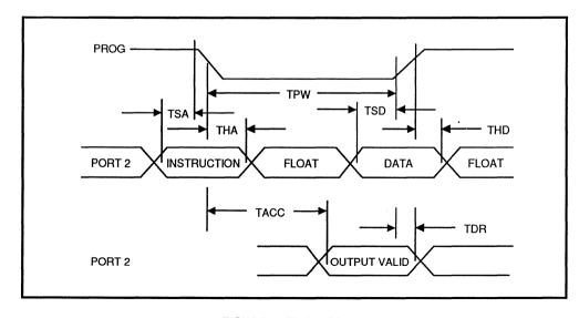
FIGURE 1: Timing Diagram
