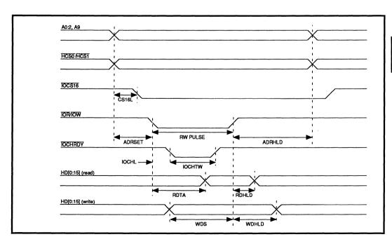
FIGURE 4: Host Programmed 8/16-Bit Timing
