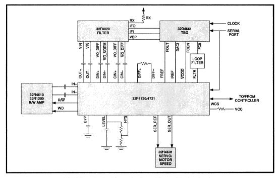
FIGURE 17: Typical Setup for Zoned Recording Application
