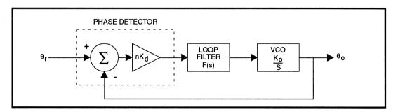
FIGURE 17B: Phase-Lock Loop System Representation
