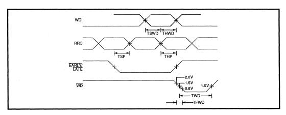
FIGURE 9: Write Mode Timing
