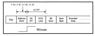
FIGURE 1: Disk Operation Lock Sequence in Read Mode Soft Sector Operation
