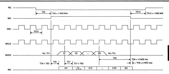
FIGURE 12: Write Mode NRZ Data Timing
