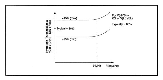
FIGURE 9: Percentage Threshold vs. Frequency
