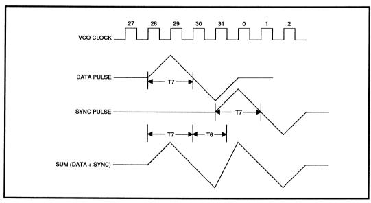
FIGURE 7 : Servo Writer Data-Sync Pulse Generation
