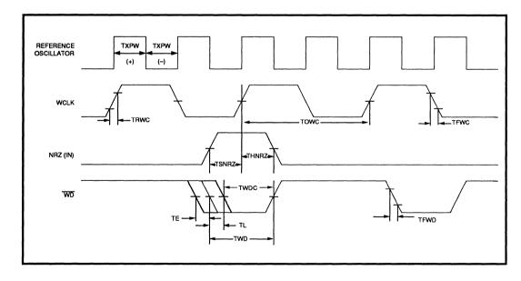
FIGURE 10: Write Timing
