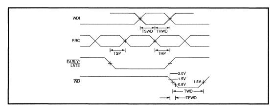
FIGURE 9: Write Mode Timing
