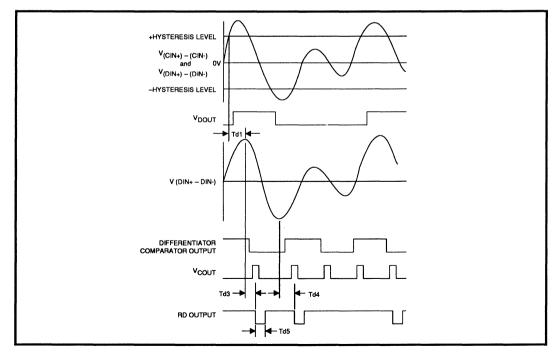
FIGURE 7: Read Mode Digital Section Timing Diagram
