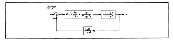
FIGURE 8(b): Simplified Track Mode Transfer Function
