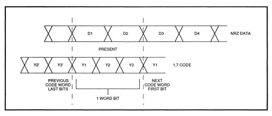
FIGURE 4: NRZ Data Word Comparision to 1, 7 Code Word Bit (See Table 1, for Decode Scheme)
