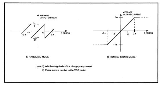
FIGURE 1: Phase Detector Transfer Function
