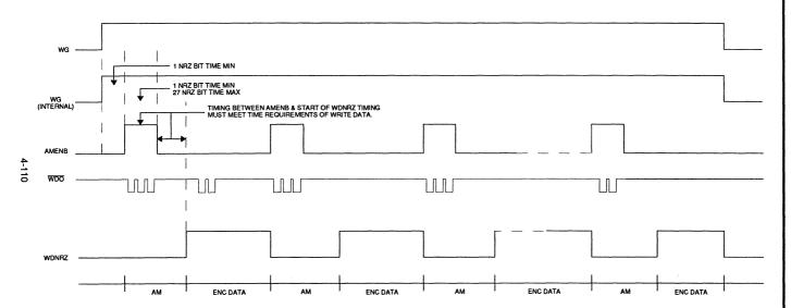
FIGURE 8: Multiple Address Mark Write
