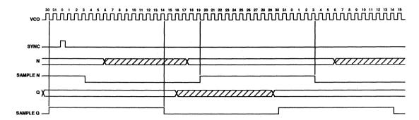
FIGURE 2: Dedicated Servo Timing Diagram
