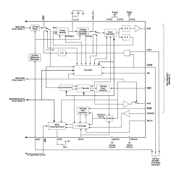
FIGURE 17b: SSI 32P4622 System Configuration (Sheet 2)
