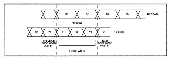
FIGURE 3: NRZ Data Word Comparision to 1, 7 Code Word (See Tables 1, and 2 for Decode Scheme)
