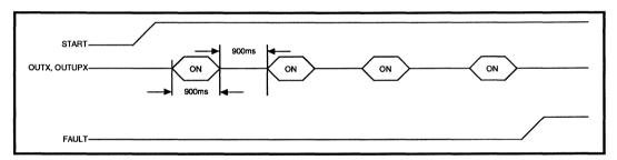
FIGURE 2: Jammed Platter Sequence
