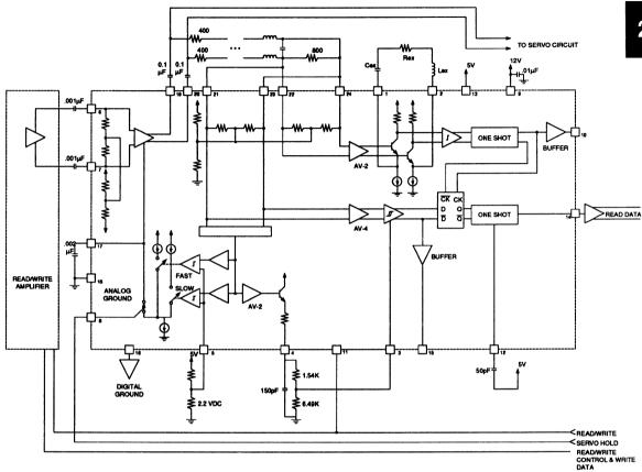
NOTES: Circuit traces for the 12V bypass capacitor and the AGC Hold Capacitor should be as short as possible with both capacitors returned to the Analog Ground Pin.
