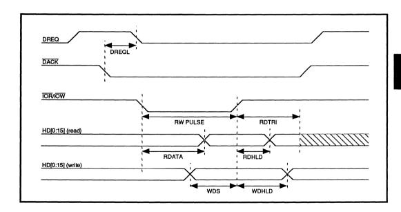
FIGURE 2: Host DMA 8/16-Bit Interface Timing (Non-Demand Mode)
