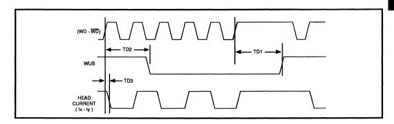
FIGURE 1: Write Mode Timing Diagram
