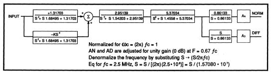
FIGURE 3: 32F8030 Normalized Block Diagram
