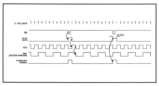
FIGURE 2: Data Synchronization Waveform Diagram
