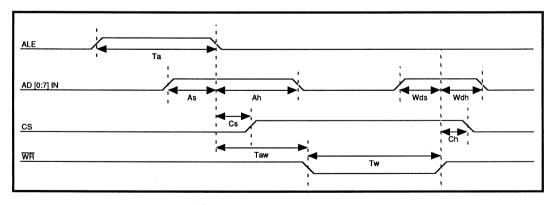
FIGURE 3: Register Write Timing
