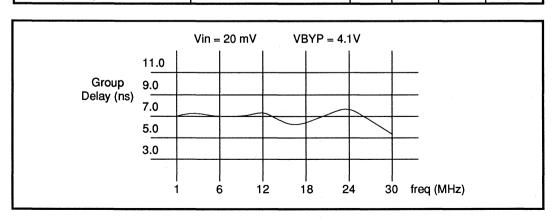
FIGURE 1: AGC Amplifier - Typical Group Delay Variation
