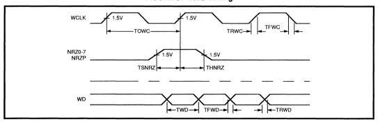
FIGURE 6: Write Timing
