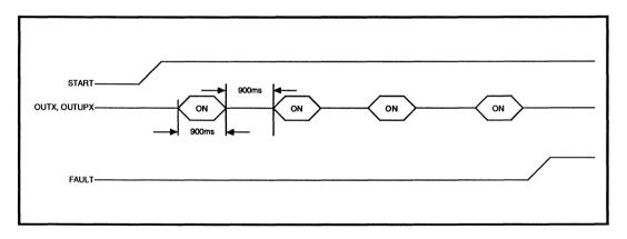
FIGURE 2: Jammed Platter Sequence
