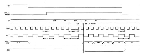
FIGURE 10: Read Mode NRZ Data Timing
