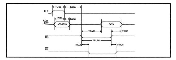
FIGURE 4(a): Read Cycle Timing
