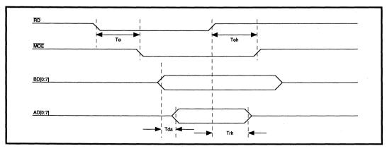
FIGURE 7: Register 70H Read Timing
