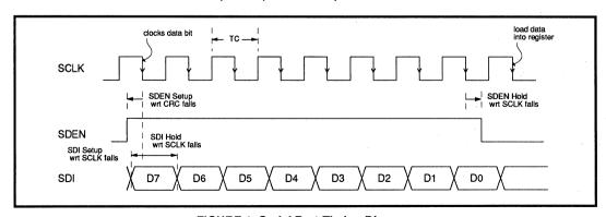
FIGURE 1: Serial Port Timing Diagram
