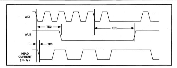
FIGURE 1: Write Mode Timing Diagram
