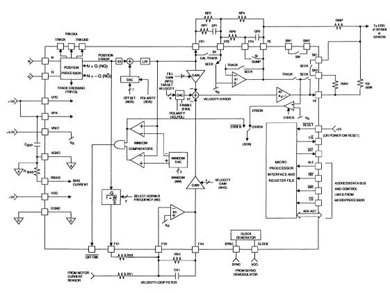
FIGURE 2: SSI 32H6220 Typical Application
