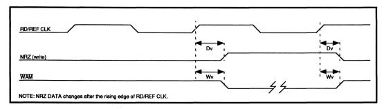
FIGURE 9: Disk Write Timing
