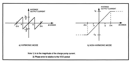
**FIGURE 4: Phase Detector Transfer Function**
