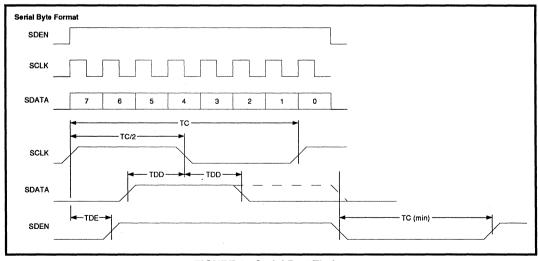
FIGURE 1: Serial Port Timing
