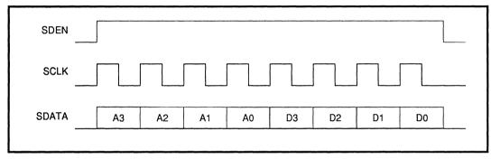
FIGURE 2: Serial Port Timing
