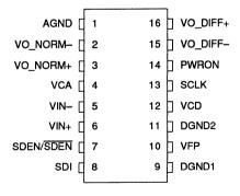
SSI 32F8130: Pin 7 = SDEN SSI 32F8131: Pin  $7 = \overline{SDEN}$
