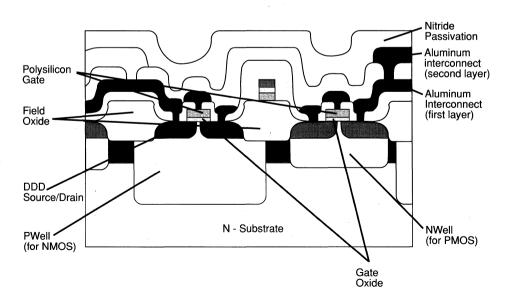
FIGURE 1: CG CMOS Process Transistor
