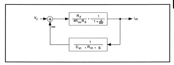
FIGURE 10(b): Simplified Transfer Function of SSI 32H6220 in Seek Mode
