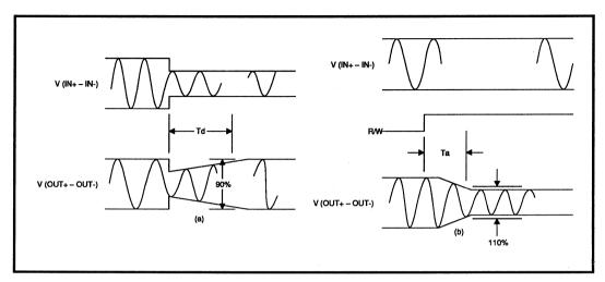
FIGURE 1(a), (b): AGC Timing Diagrams
