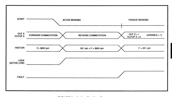
FIGURE 3: Active Braking Sequence
