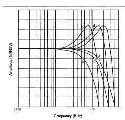
FIGURE 4: 32F8011/8012 Normal Low Pass Output Response (VO\_NORM)
