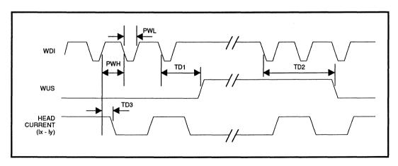
FIGURE 1: Write Mode Timing Diagram
