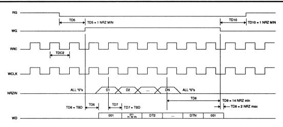
FIGURE 16: Write Mode NRZ Data Timing
