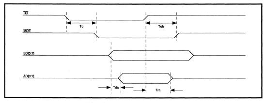
FIGURE 7: Register 70H Read Timing
