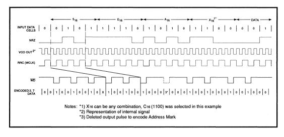
FIGURE 8: Write Address Mark Generation
