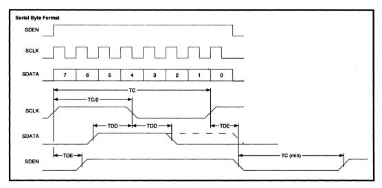
FIGURE 1: Serial Port Timing
