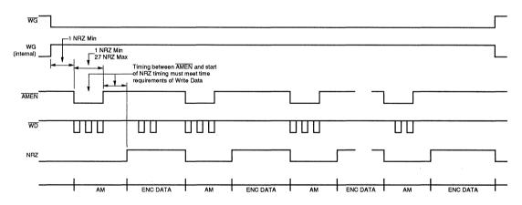
FIGURE 11: Multiple Address Mark Write
