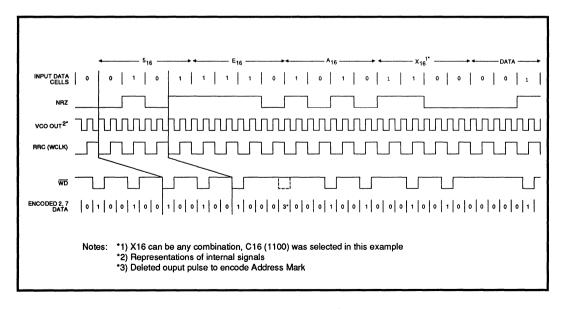
FIGURE 8: Write Address Mark Generation
