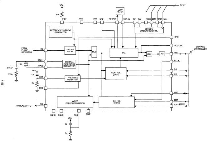
FIGURE 13: Typical SSI 32D535 Application
