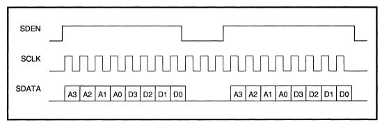
FIGURE 3: Serial Port Timing, Multiple Transfers
