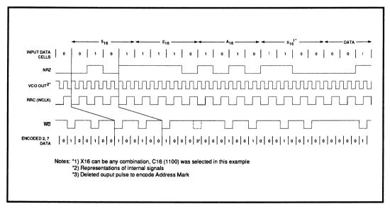
FIGURE 8: Write Address Mark Generation
