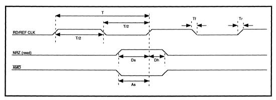
FIGURE 5: Disk Read Timing
