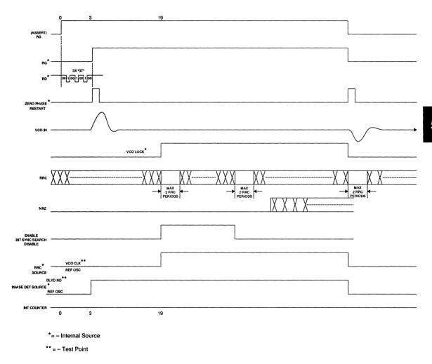
FIGURE 13: Read Mode Locking Sequence (Soft and Hard Sector)
