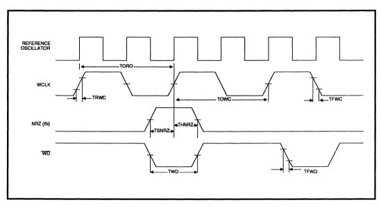
FIGURE 10: Write Timing
