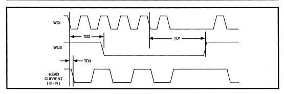
FIGURE 1: Write Mode Timing Diagram
