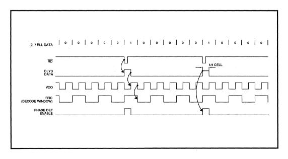
FIGURE 2: Data Synchronization Waveform Diagram
