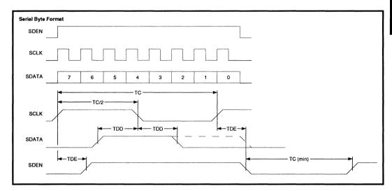
FIGURE 1: Serial Port Timing
