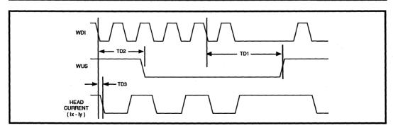
FIGURE 1: Write Mode Timing Diagram
