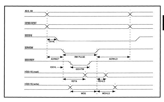
FIGURE 2: Host Programmed 8/16-Bit Timing
