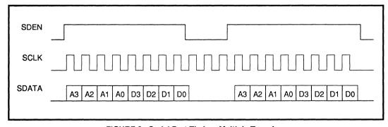
FIGURE 3: Serial Port Timing, Multiple Transfers
