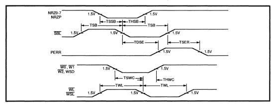
FIGURE 7: Control Timing
