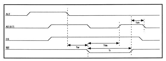
FIGURE 5: Register Read Timing
