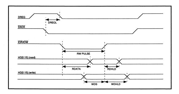
FIGURE 1: Host DMA 8/16-Bit Interface Timing
