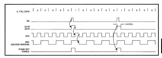
FIGURE 5: Data Synchronization Waveform Diagram
