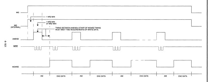
FIGURE 10: Multiple Address Mark Write
