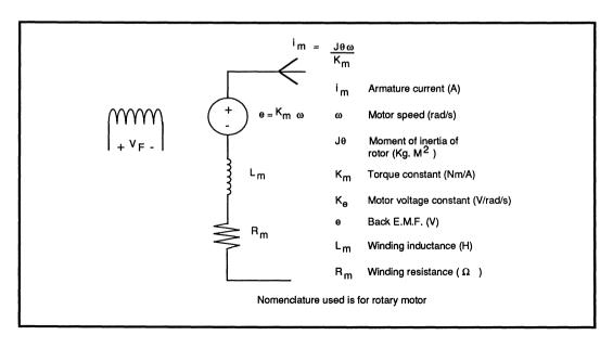
FIGURE 3: Equivalent Circuit for Fixed Field DC Motor
