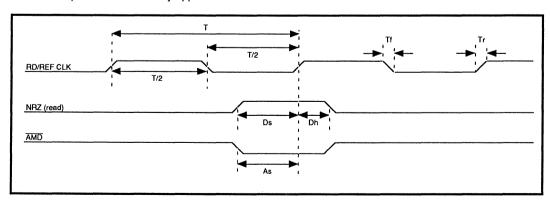
FIGURE 5: Disk Read Timing
