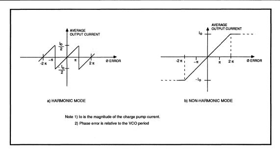
FIGURE 1: Phase Detector Transfer Function
