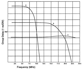
FIGURE 6: 32F8011/8012 Typical Group Delay Variation (Differentiated Output) Maximum Boost
