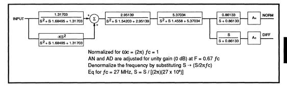
FIGURE 5: 32F8000 Normalized Block Diagram
