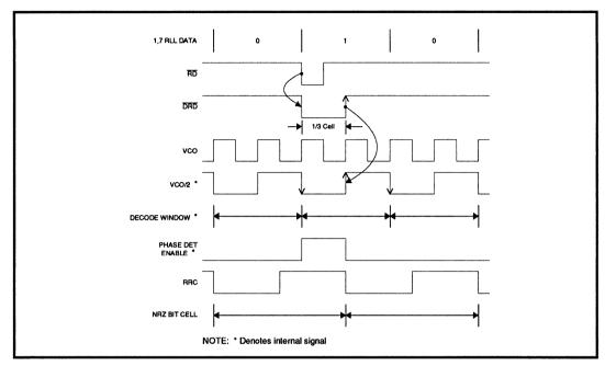
FIGURE 2: Data Synchronization Waveform
