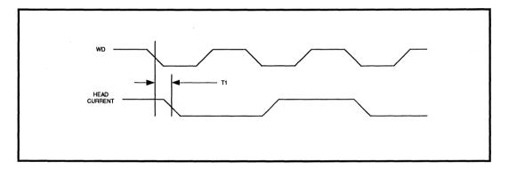
FIGURE 1: Head Current Switching Delay
