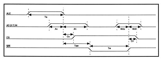
FIGURE 3: Register Write Timing
