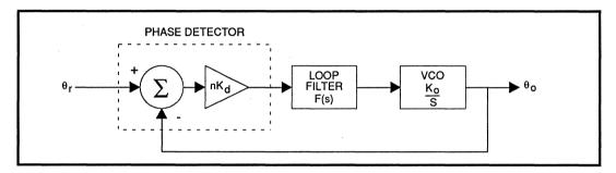
FIGURE 17B: Phase-Lock Loop System Representation
