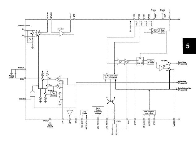
FIGURE 5a: SSI 32P4622 Circuit Block Diagram (Sheet 1)
