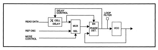
FIGURE 16A: Modified Data Synchronizer Phase-Locked-Loop with Quarter Cell Delay Control
