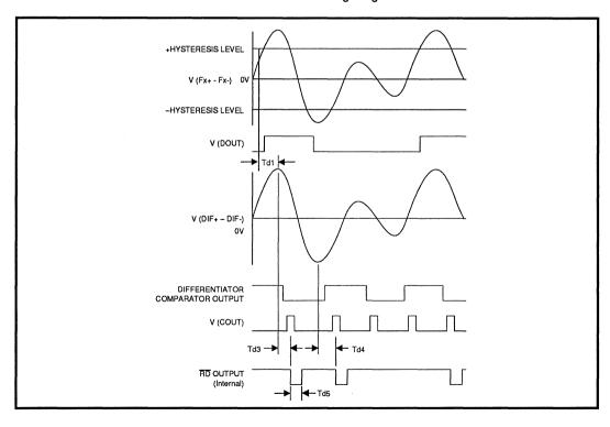
FIGURE 7: Read Mode Digital Section Timing Diagram
