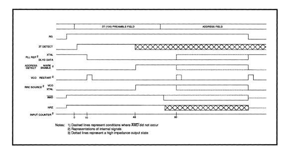
FIGURE 4: Soft Sector Mode Timing Diagram
