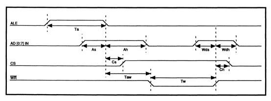
**FIGURE 5: Register Write Timing**
