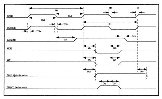
FIGURE 9: Buffer Memory Read/Write Timing
