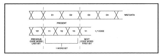
FIGURE 2: NRZ Data Word Comparision to 1, 7 Code Word Bit (See Table 1, for Decode Scheme)
