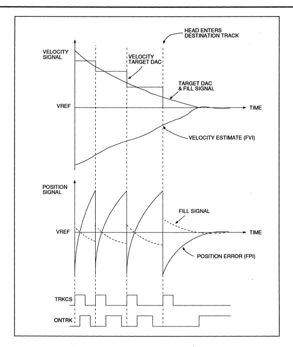
FIGURE 9: Typical Waveforms During Final Deceleration Mode
