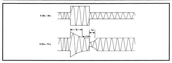
FIGURE 1: AGC Timing Diagram
