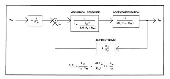
FIGURE 4(B): Simplified Transfer Function of SSI 32H6230 in DC Motor Application
