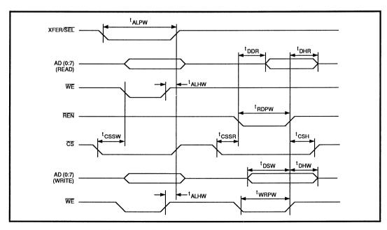
FIGURE 4: TMS320XX Bus Interface Timing Diagram
