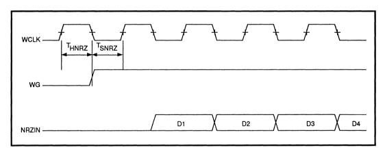
FIGURE 3: WG Timing Requirement for Predictable Write Encoding
