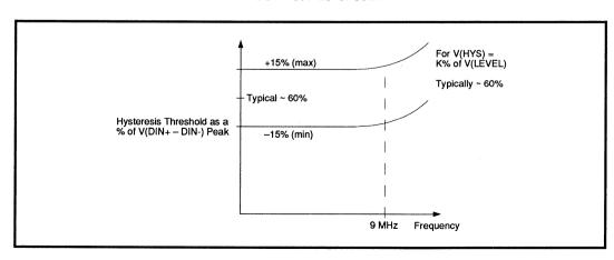
FIGURE 6: Percentage Threshold Versus Frequency
