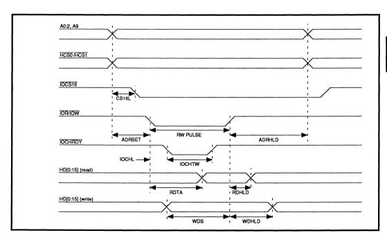
FIGURE 3: Host Programmed 8/16-Bit Timing
