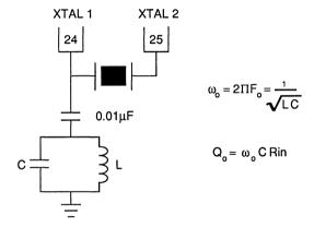
The typical input impedance looking into XTAL1 is approximately Rin =  $250\Omega$ . It is recommended to design the value of Qo at approximately 10 to 15. Therefore, a resonant frequency of Fo = 20 MHz would result in L  $\cong$  0.16  $\mu$ H and C  $\cong$  380 pF.
