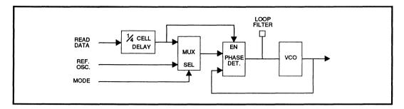
FIGURE 14A: Standard Configuration of a Data Synchronizer Phase-Locked Loop
