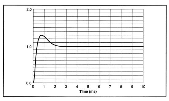
FIGURE 4: Position Closed Loop Step Response
