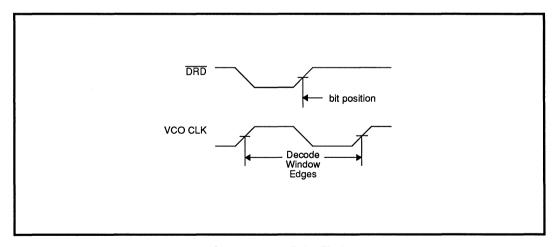
**FIGURE 12: Test Point Timing**
