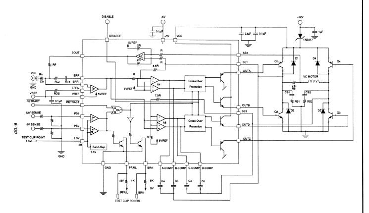
FIGURE 2: SSI 32H6240 Typical Application
