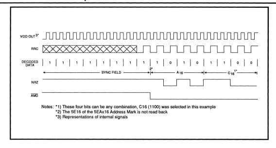
FIGURE 5: Address Mark Detection and NRZ Output Waveform
