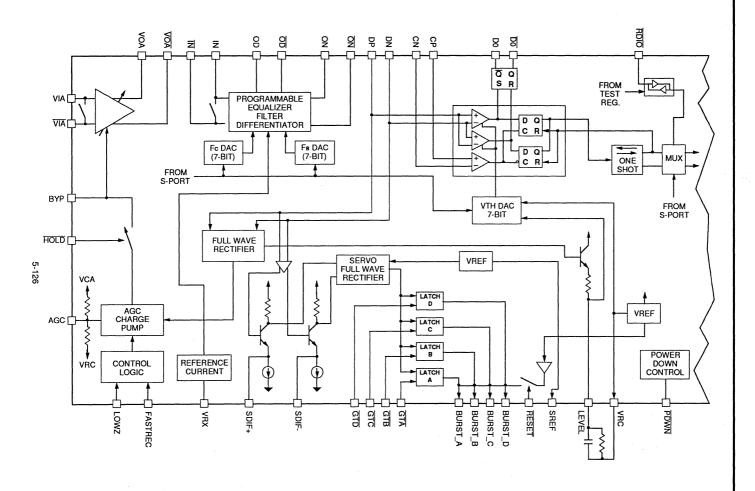
FIGURE 1(A): SSI 32P4740 Combo Device Part 1
