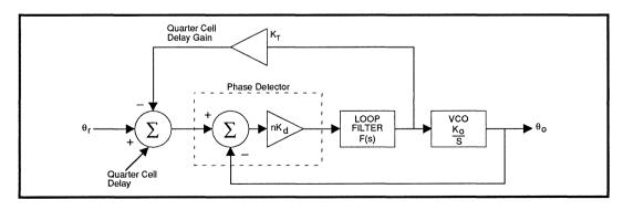
FIGURE 19B: Modified Data Synchronizer System Representation
