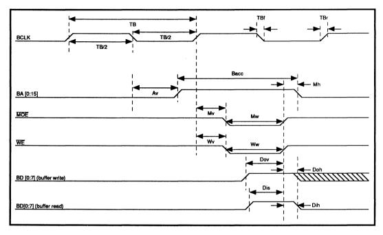
FIGURE 12: Buffer Memory Read/Write Timing
