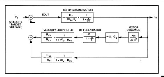
FIGURE 10(a): Transfer Function of SSI 32H6220 in Seek Mode
