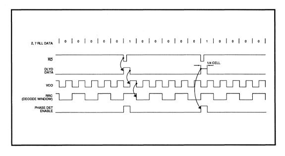
FIGURE 2: Data Synchronization Waveform Diagram
