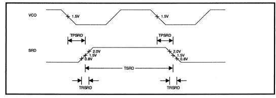
FIGURE 10: Read Mode Timing
