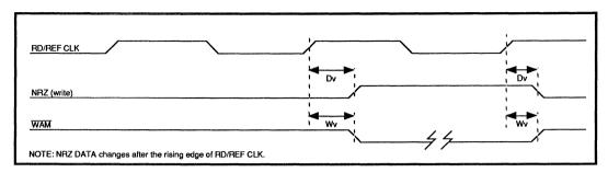
FIGURE 6: Disk Write Timing
