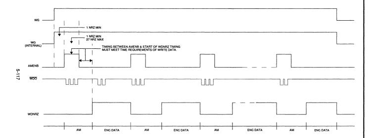
FIGURE 14: Multiple Address Mark Write
