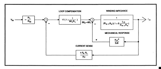
FIGURE 4(A): Transfer Function Of SSI 32H569 In Typical Application With Fixed Field DC Motor
