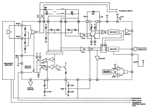
NOTE: Circuit traces for the 12V bypass capacitor and the AGC Hold Capacitor should be as short as possible with both capacitors returned to the Analog Ground Pin.
