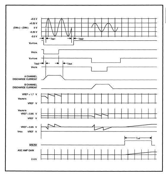
FIGURE 3: Servo Read Mode I Timing Diagram
