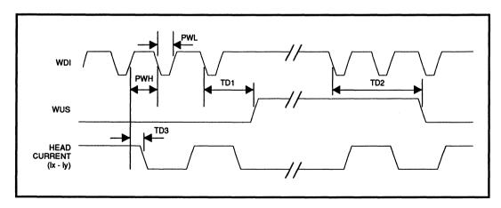
FIGURE 1: Write Mode Timing Diagram
