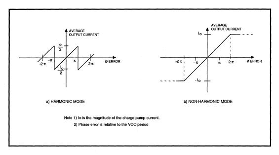
**FIGURE 1: Phase Detector Transfer Funtion**
