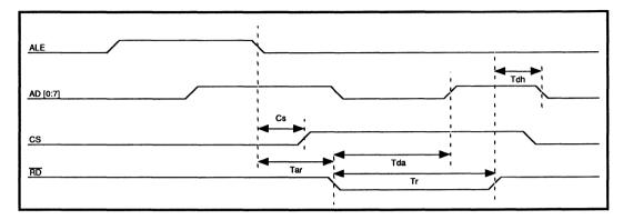
FIGURE 6: Register Read Timing
