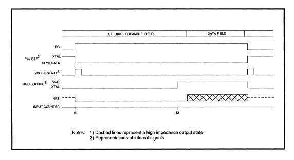
FIGURE 6: Hard Sector Mode Timing Diagram
