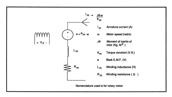
FIGURE 3: Equivelant Circuit For Fixed Field DC Motor
