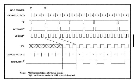
FIGURE 7: Hard Sector Mode Decode Timing
