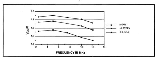
FIGURE 4d: Level Gain
