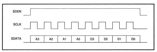
FIGURE 2: Serial Port Timing
