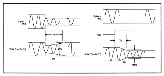
FIGURE 1(a), (b): AGC Timing Diagrams
