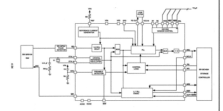
FIGURE 12: SSI 32D5322 Typical Application
