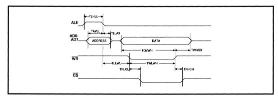
FIGURE 4(b): Write Cycle Timing
