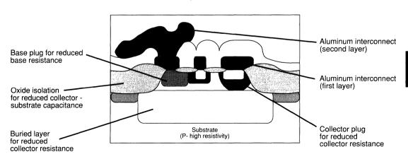
FIGURE 2: BN Bipolar Process NPN Transistor
