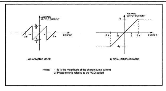
**FIGURE 1: Phase Detector Transfer Function**
