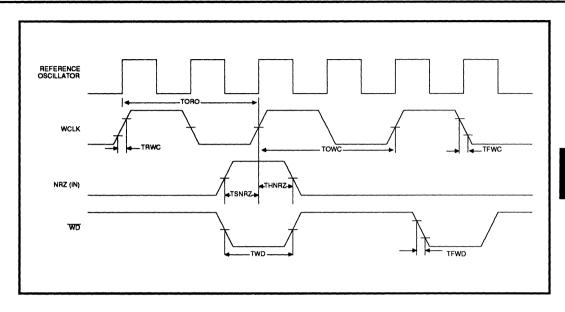
FIGURE 10: Write Timing
