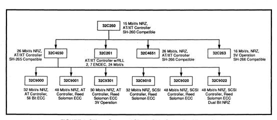
FIGURE 1: Silicon Systems' Single Chip Controller Hierarchy
