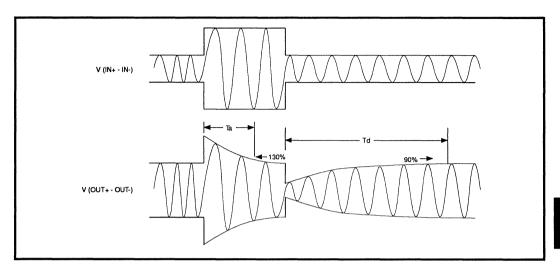
FIGURE 6: AGC Timing Diagram
