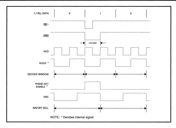
FIGURE 8: Data Synchronization Waveform
