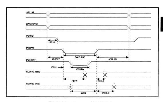
FIGURE 2: Host Programmed 8/16-Bit Timing
