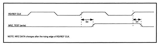
FIGURE 7: NRZ Test Output Timing
