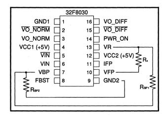
FIGURE 1: 32F8030 Applications Setup, 16-Pin SO or DIP
