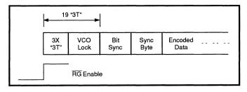
FIGURE 2: Disk Operation Lock Sequence in Read Mode Hard Sector Operation
