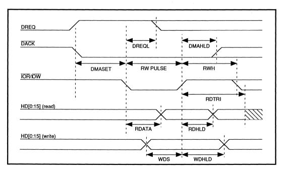
FIGURE 3: Host DMA 8/16-Bit Interface Timing (Demand Mode)
