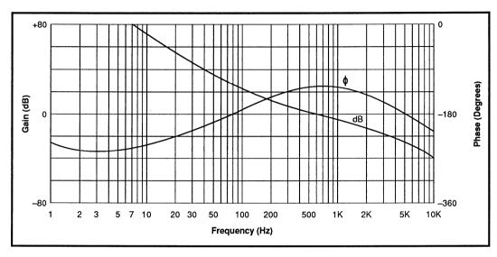
FIGURE 3: Overall Position Open Loop Bode Plot
