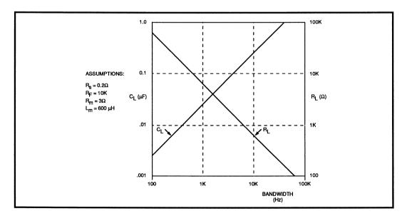
**FIGURE 6: Typical Motor Driver Compensation**
