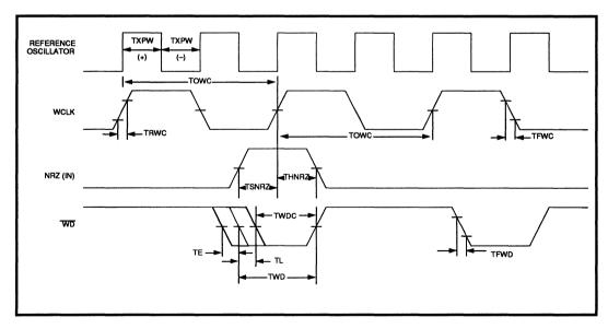
FIGURE 10: Write Timing
