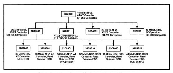
FIGURE 1: Silicon Systems' Disk Controller Chip Hierarchy
