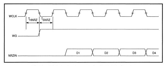
FIGURE 5: WG Timing Requirement for Predictable Write Encoding
