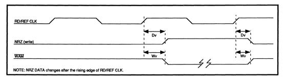
FIGURE 6: Disk Write Timing
