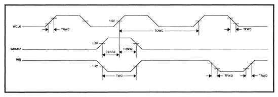
FIGURE 10: Write Timing
