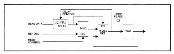
FIGURE 19A: Modified Data Synchronizer Phase-Locked-Loop with Quarter Cell Delay Control
