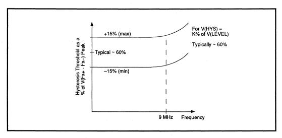
FIGURE 4: Percentage Threshold vs. Frequency
