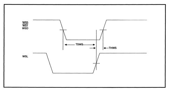
**FIGURE 11: Control Timing**
