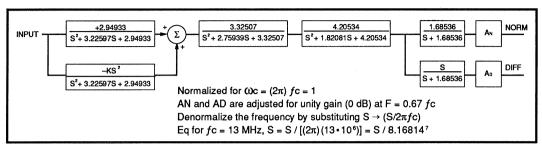
FIGURE 12: 32F8011/8012 Normalized Block Diagram
