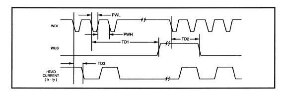
FIGURE 1: Write Mode Timing Diagram
