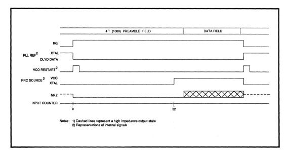
FIGURE 6: Hard Sector Mode Timing Diagram
