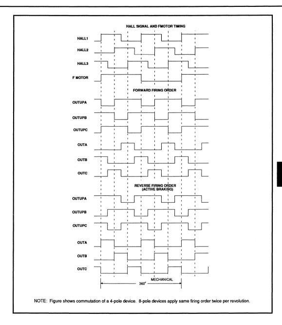
FIGURE 1: Commutation Timing Diagram
