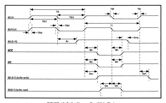
FIGURE 10: Buffer Memory Read/Write Timing
