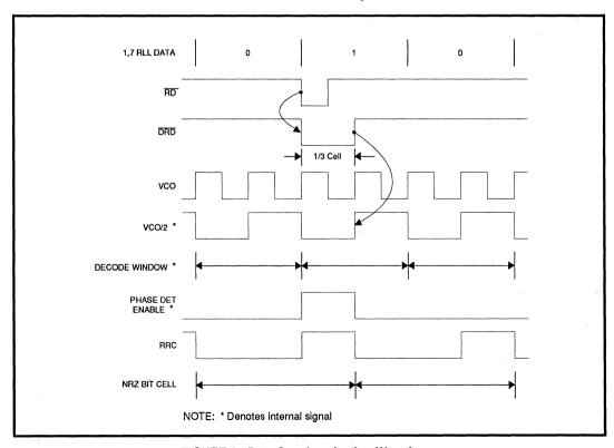
FIGURE 3: Data Synchronization Waveform
