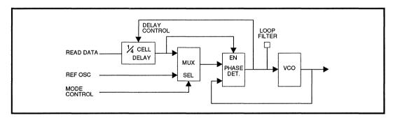
FIGURE 19A: Modified Data Synchronizer Phase-Locked-Loop with Quarter Cell Delay Control
