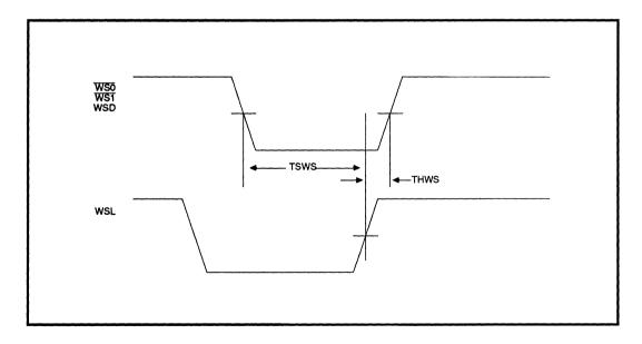
FIGURE 11: Control Timing
