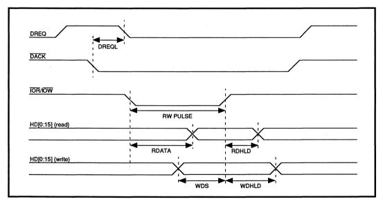
FIGURE 2: Host DMA 8/16-Bit Interface Timing
