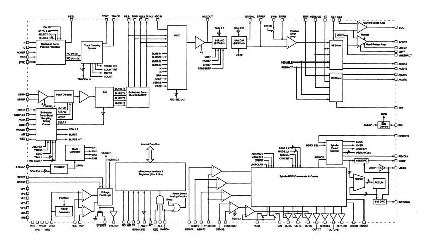
FIGURE 1: SSI 32H4631 Block Diagram
