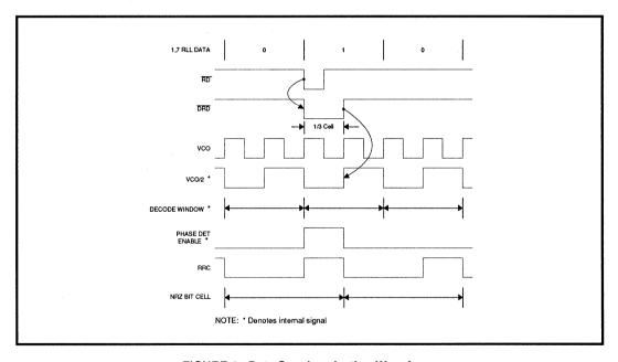
FIGURE 1: Data Synchronization Waveform
