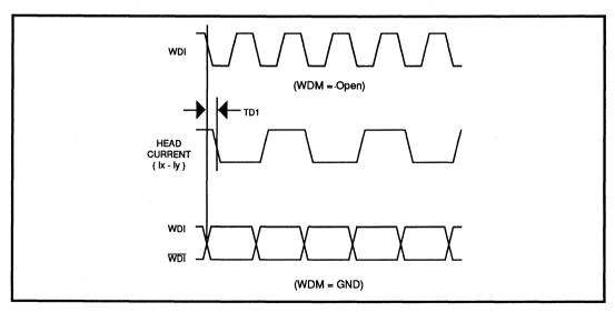
FIGURE 1: Write Mode Timing Diagram
