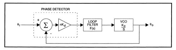
FIGURE 14B: Phase-Lock Loop System Representation
