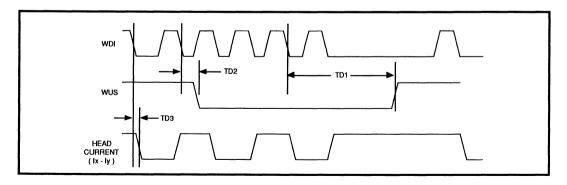
FIGURE 1: Write Mode Timing Diagram
