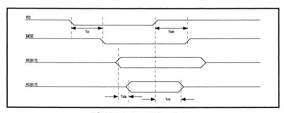
FIGURE 8: Register 70H Read Timing
