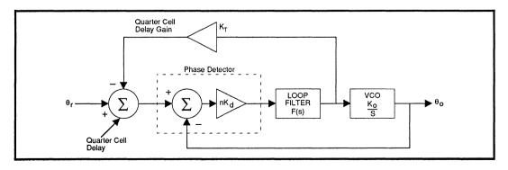
FIGURE 19B: Modified Data Synchronizer System Representation
