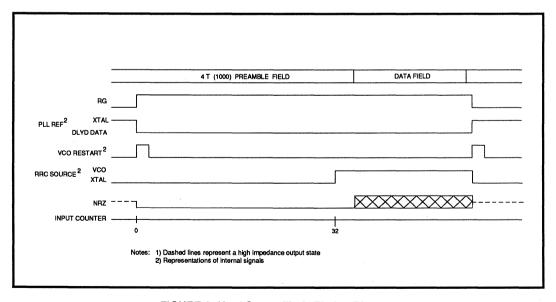
FIGURE 6: Hard Sector Mode Timing Diagram
