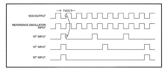
FIGURE 1: Relationship of VCO Output to Phase Detector Input
