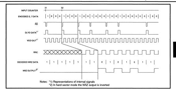
FIGURE 7: Hard Sector Mode Decode Timing
