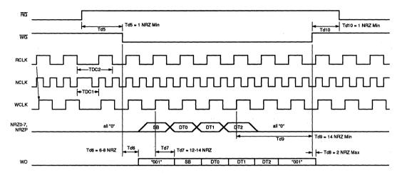
FIGURE 13: Write Mode NRZ Timing
