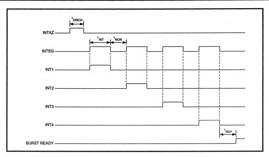
FIGURE 1: Embedded Servo Burst Processor Timing Diagram
