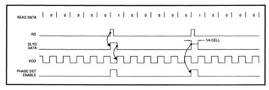
FIGURE 5: Data Synchronization Waveform Diagram
