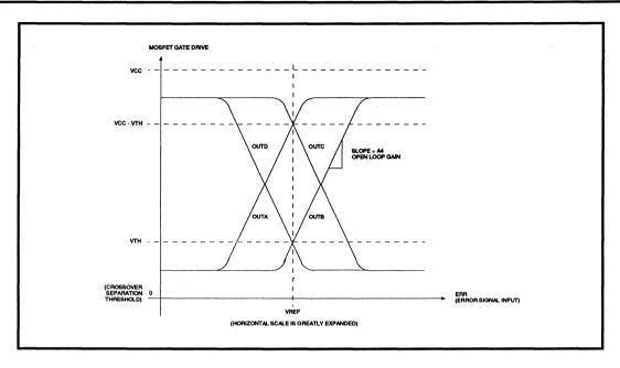
FIGURE 4(B): Simplified Transfer Function Of SSI 32H569 In DC Motor Application
