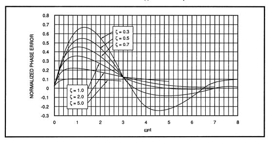
FIGURE 3: Transient Phase Error  $\theta e(t)$  Due to a Step In Frequency  $\Delta \omega$ 4-211
