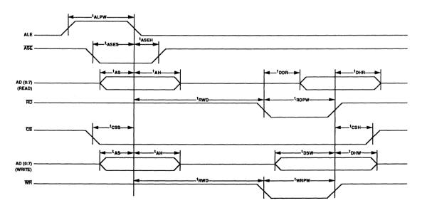
FIGURE 5: Intel Microprocessor Bus Interface Timing Diagram
