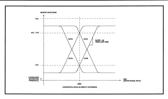
FIGURE 5: Simplified Transfer Function of SSI 32H6230 in DC Motor Application
