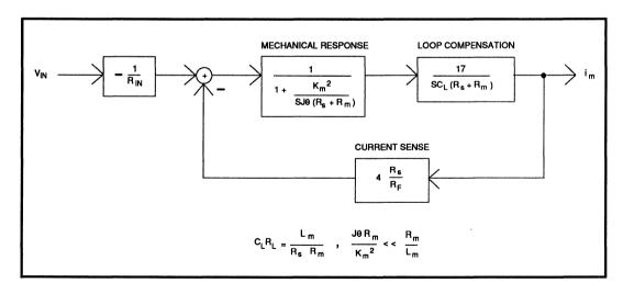
FIGURE 4(B): Simplified Transfer Function Of SSI 32H569 In DC Motor Application
