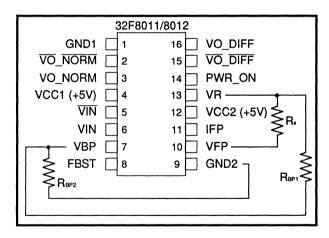
FIGURE 1: 32F8011/8012 Applications Setup, 16-Pin SO or DIP
