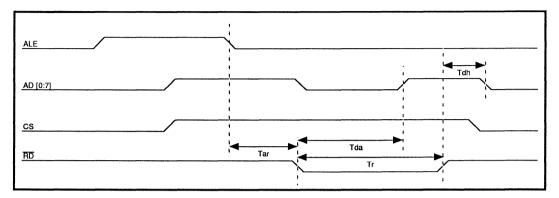
FIGURE 4: Register Read Timing
