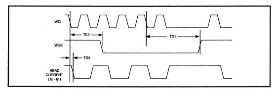
FIGURE 1: Write Mode Timing Diagram
