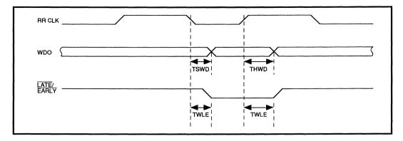
FIGURE 11: Write Data Timing - RLL ENDEC Mode
