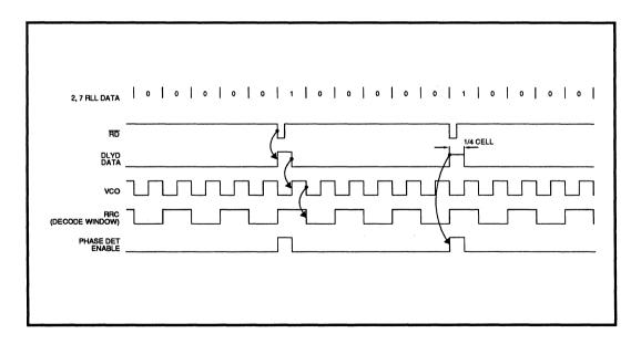
FIGURE 2: Data Synchronization Waveform Diagram
