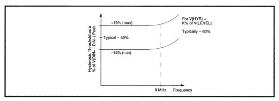
FIGURE 18: Percentage Threshold vs. Frequency
