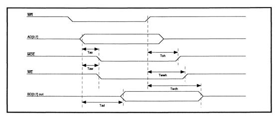
FIGURE 8: Register 70H Write Timing
