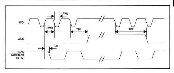
FIGURE 1: Write Mode Timing Diagram
