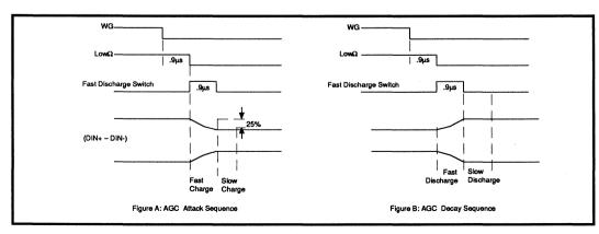
FIGURE 7: AGC Timing Diagram
