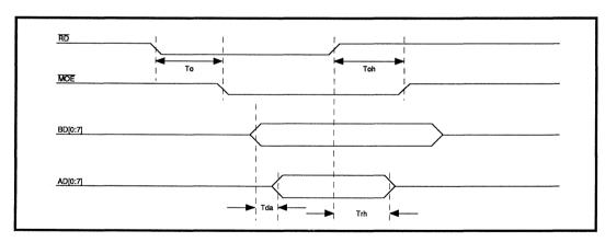
FIGURE 10: Register 70H Read Timing
