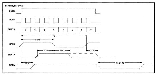
FIGURE 1: Serial Port Timing
