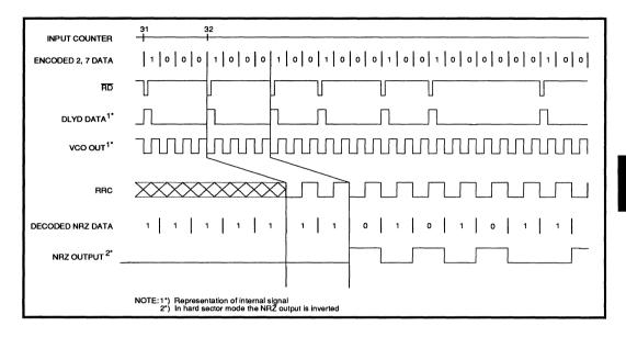
FIGURE 7: Hard Sector Mode Decode Timing
