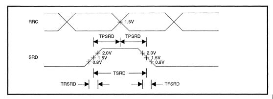
FIGURE 10: Read Mode Timing
