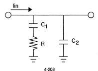
The role of C1 is as an integrating element. The larger this capacitance, the longer the acquisition time; the smaller the capacitance, the greater the ability to track high frequency jitter. The resistor R reduces the phase shift induced by C1. The capacitor C2 will suppress high frequency transients and will have minimal effect on the loop response if it is small relative to C1 (typically C2 = C1/10)
