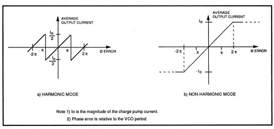
**FIGURE 4: Phase Detector Transfer Function**
