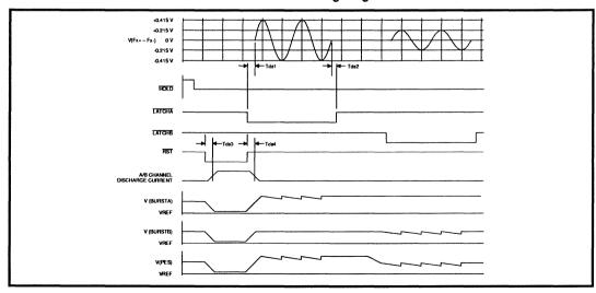
FIGURE 2: Servo Timing Diagram
