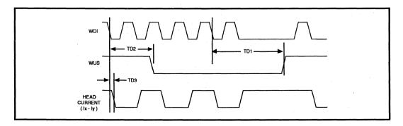
FIGURE 1: Write Mode Timing Diagram
