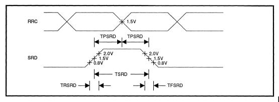
FIGURE 10: Read Mode Timing
