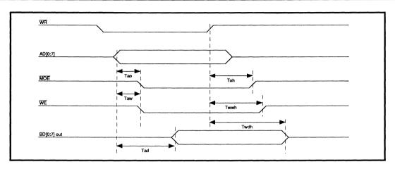
FIGURE 9: Register 70H Write Timing
