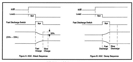
FIGURE 7: AGC Timing Diagram
