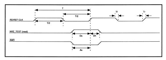
FIGURE 6: NRZ Test Input Timing
