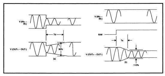
FIGURE 1(a), (b): AGC Timing Diagrams
