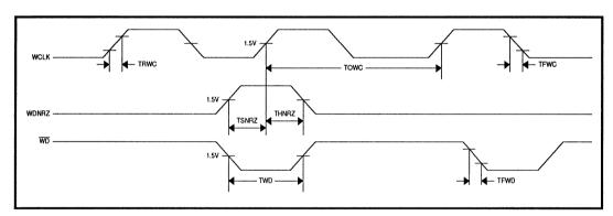
FIGURE 4: Write Timing
