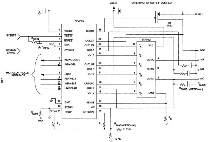
Typical Bipolar Start/Unipolar Run 32M595 Application
