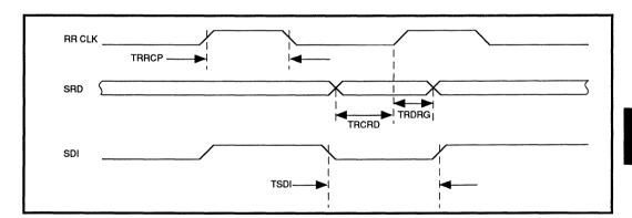
FIGURE 12: Read Data Timing - RLL ENDEC Mode
