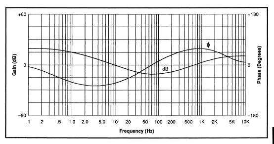
FIGURE 2: Position Loop Filter Bode Plot
