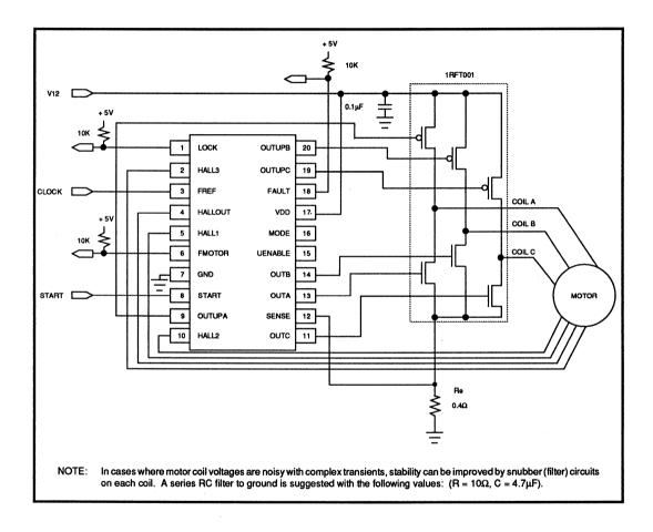
FIGURE 4:Typical Three-Phase, 4-Pole, Bipolar, Non-Center Tapped Motor Using A Power FET Module
