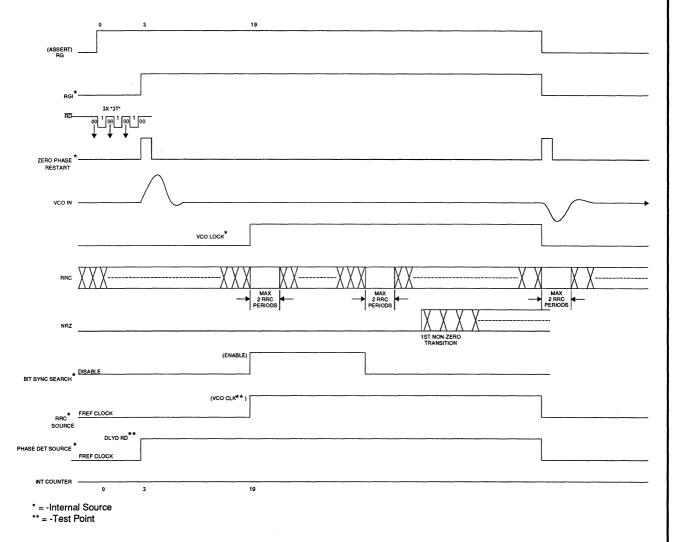
FIGURE 13: Read Mode Locking Sequence (Soft and Hard Sector)
