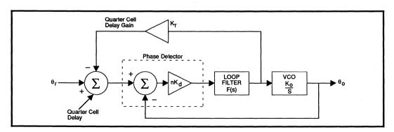
FIGURE 16B: Modified Data Synchronizer System Representation
