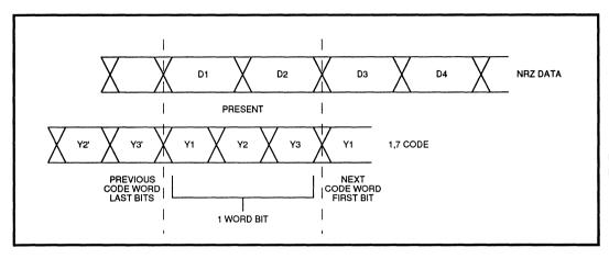
FIGURE 2: NRZ Data Word Comparision to 1, 7 Code Word Bit (See Table 1, for Decode Scheme)
