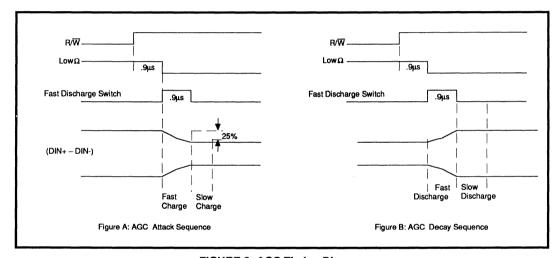
**FIGURE 6: AGC Timing Diagram**
