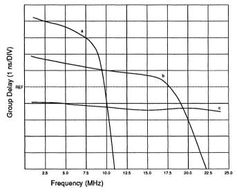
FIGURE 7: 32F8011/8012 Typical Group Delay Variation (Differentiated Output) No Boost
