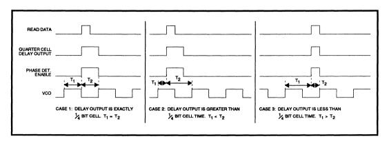
FIGURE 15B: Timing of Phase Detector Enable Logic. The read data input pulse can shift to the left by T1 and to the right by T2 before an error occurs in the phase detector output polarity, If the quarter cell delay output is not exactly 1/4 bit cell wide, then T1  $\neq$  T2, as shown in cases 2 and 3.
