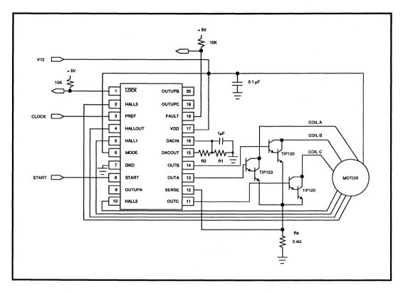
Typical Three-Phase, 8-Pole, Unipolar,
