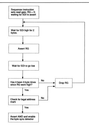
FIGURE 1: Encoder Sequence for Soft Sector Mode
