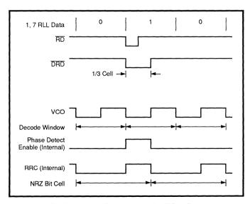
FIGURE 3: Data Synchronization Waveforms
