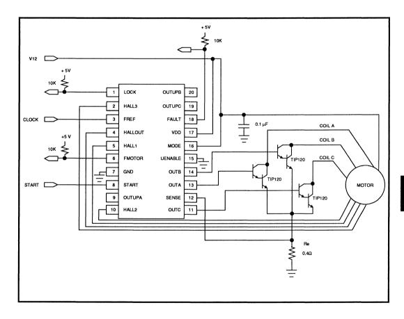
FIGURE 5:Typical Three-Phase, 8-Pole, Unipolar,
