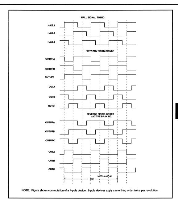
FIGURE 1: Commutation Timing Diagram
