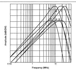
FIGURE 5: 32F8011/8012 Differented Low Pass Output Response (VO\_DIFF)
