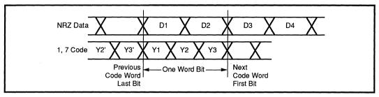
FIGURE 4: NRZ Data Word Comparison to 1, 7 Code Word Bit
