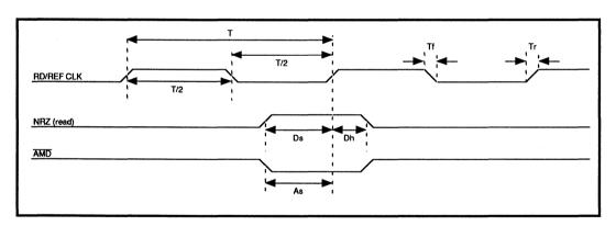
FIGURE 8: Disk Read Timing
