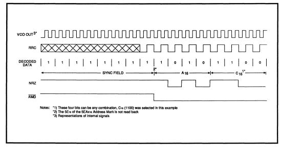
FIGURE 5: Address Mark Detection and NRZ Output Waveform
