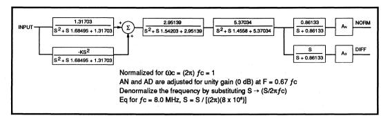
FIGURE 3: 32F8020/8022 Normalized Block Diagram
