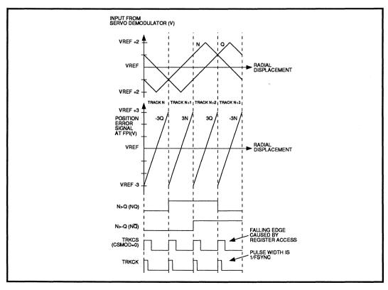
FIGURE 6: Position Signal Waveforms
