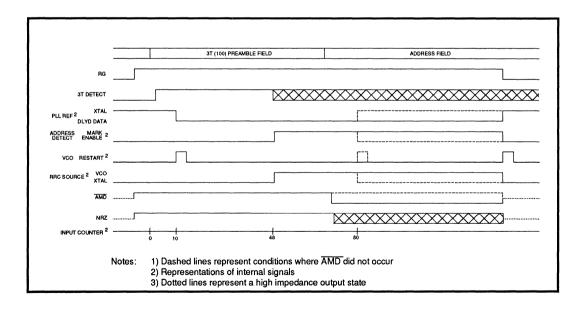
FIGURE 4: Soft Sector Mode Timing Diagram
