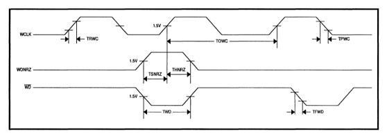
FIGURE 4: Write Timing
