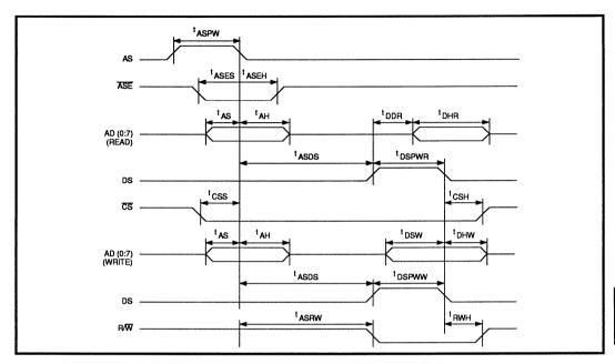
FIGURE 3: Motorola Microprocessor Bus Interface Timing Diagram
