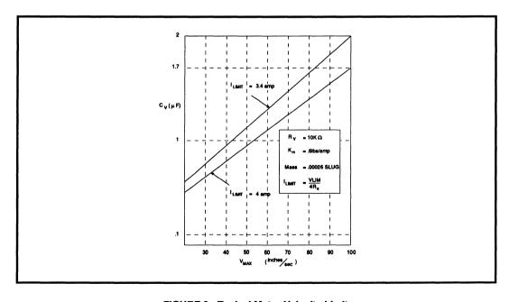
FIGURE 9: Typical Motor Velocity Limit
