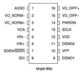
SSI 32F8130: Pin 7 = SDEN SSI 32F8131: Pin 7 = SDEN
