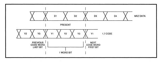
FIGURE 9: NRZ Data Word Comparison to 1, 7 Code Word Bit (See Table 1 for decode scheme)
