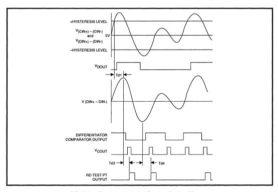
FIGURE 8: Read Mode Digital Section Timing Diagram
