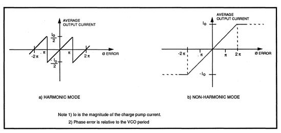
**FIGURE 4: Phase Detector Transfer Function**
