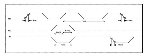
FIGURE 11: Write Timing
