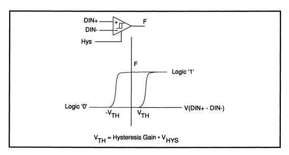
FIGURE 4b: Hysteresis Comparator Transfer Function
