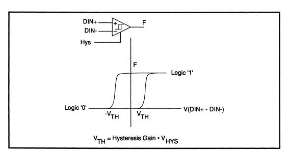
FIGURE 5b: Hysteresis Comparator Transfer Function
