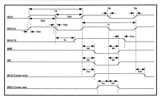
FIGURE 9: Buffer Memory Read/Write Timing
