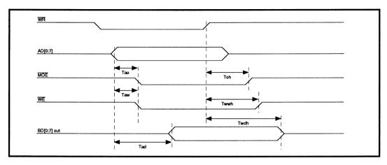
FIGURE 8: Register 70H Write Timing
