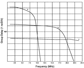
FIGURE 8: 32F8011/8012 Typical Group Delay Variation (Normal Low Pass Output) Maximum Boost
