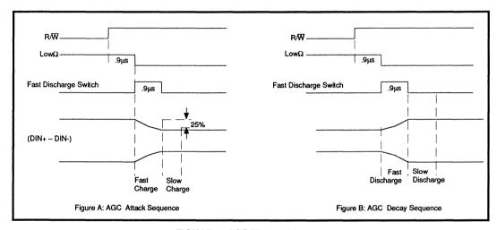
FIGURE 7: AGC Timing Diagram
