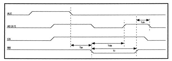
FIGURE 4: Register Read Timing
