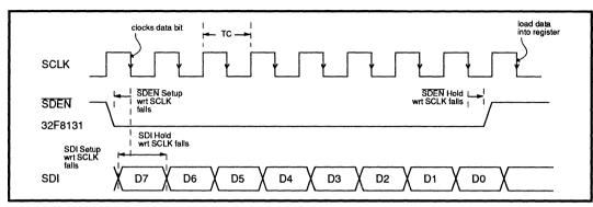
FIGURE 2: Serial Port Timing Relationship
