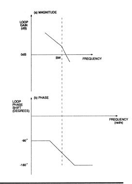
FIGURE 11: Bode Plot of Simplified Track Mode Transfer Function
