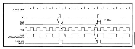
FIGURE 5: Data Synchronization Waveform Diagram
