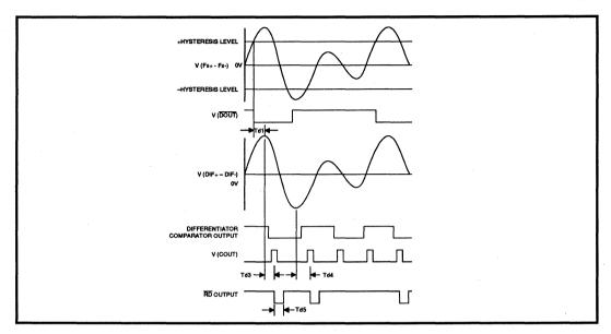
FIGURE 6: Read Mode Digital Section Timing Diagram
