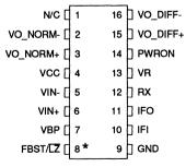
\* Pin 8 = FBST - SSI 32F8020 \(\overline{LZ}\) - SSI 32F8022
