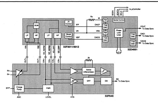
FIGURE 2: Applications Setup, Constant Density Recording 32F8011/8012, 32P54X, 32D4661
