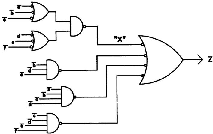
$$Z = \bar{a} * \bar{b} * \bar{c} * \bar{d} + \bar{b} * \bar{d} * \bar{e} + [ (\bar{a} + \bar{b} + \bar{c}) * (\bar{d} + \bar{e} + \bar{f}) ] + \bar{c} * \bar{d} * \bar{e} * \bar{f} ;$$
