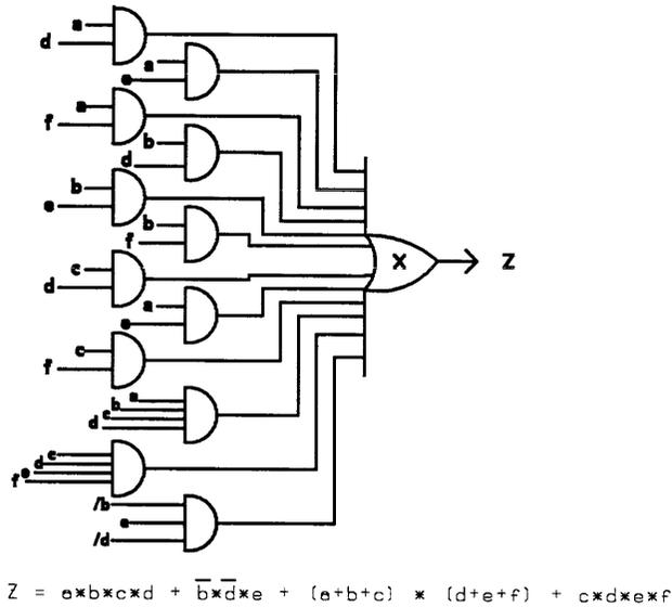
Figure 3-26 Two Level SOP Configuration
