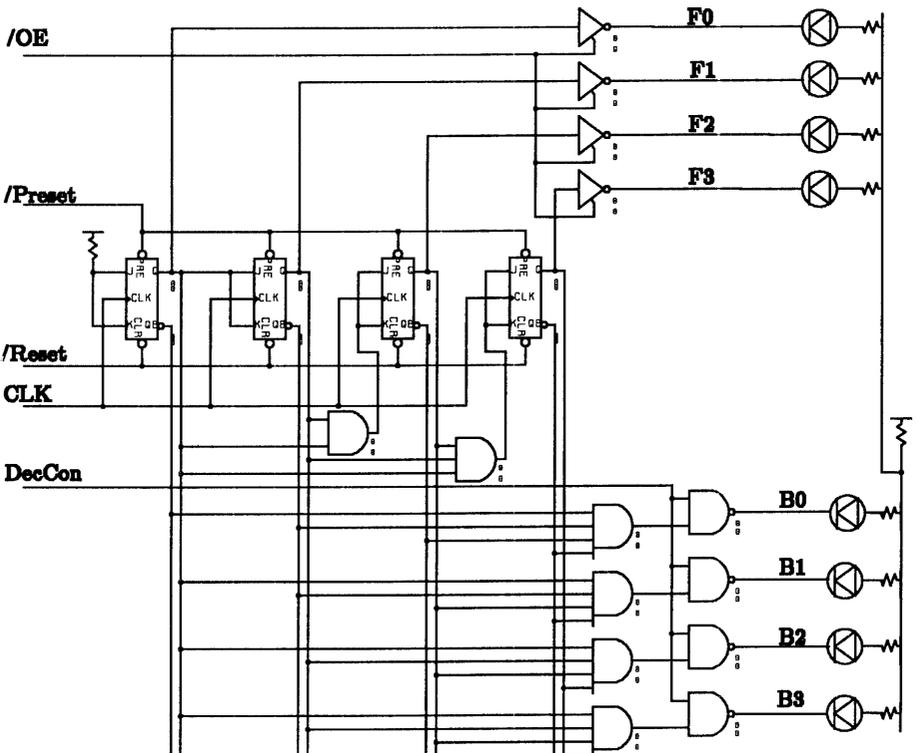
Figure 9-3 4 Bit Timer/Decoder
