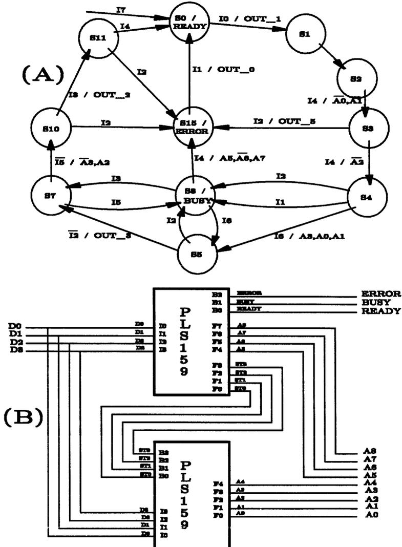
Figure 9-6 State Machine Design Example
