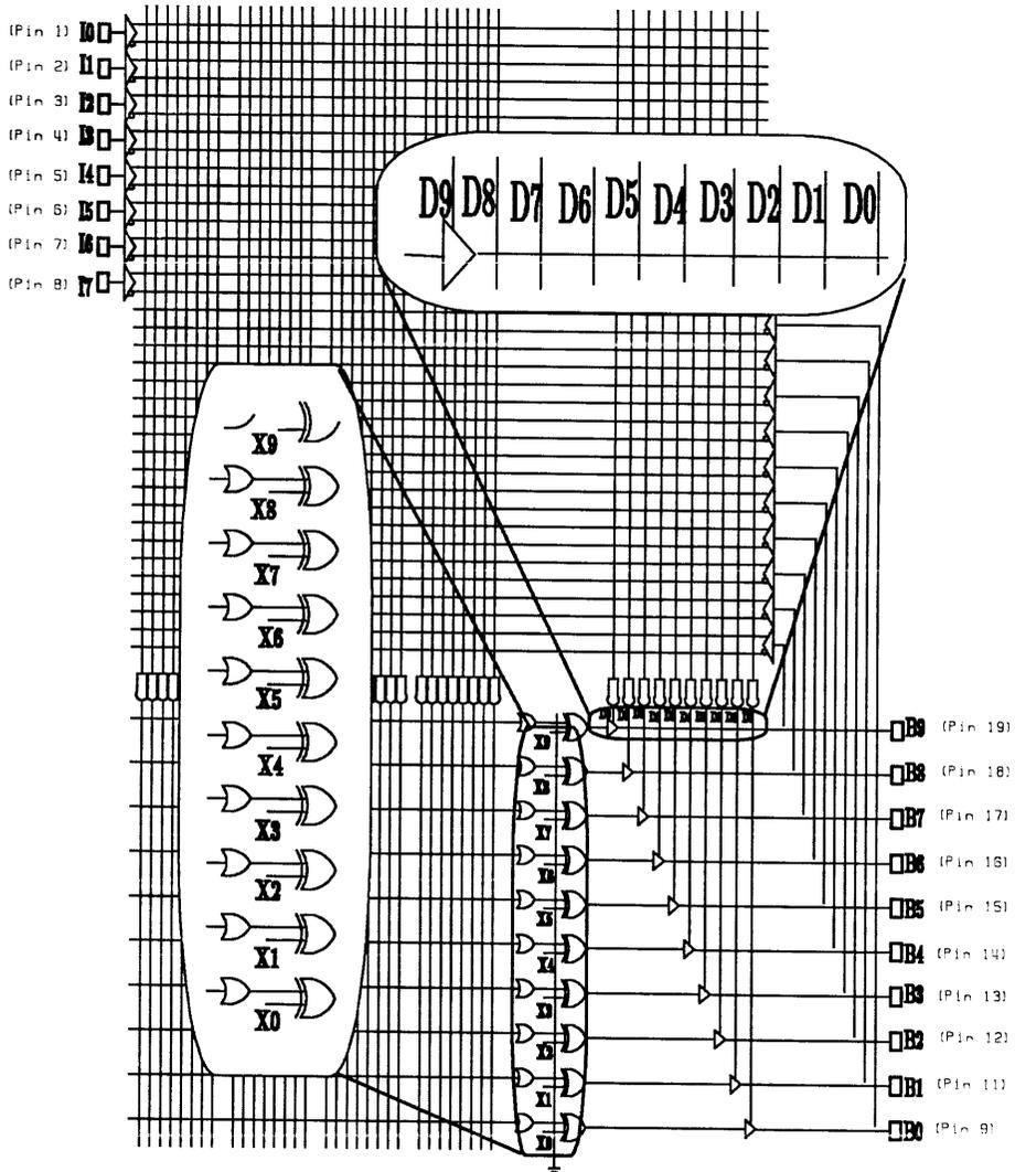
Figure 3-8 PLS153 Logic Diagram (20 Pin PLD)
