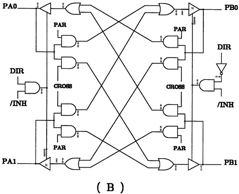
Figure 9-1 Two 2-bit Port Controller
