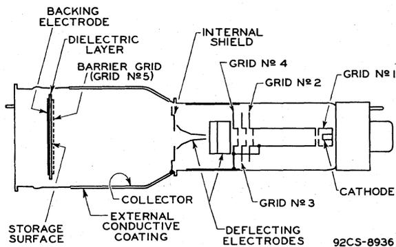
Fig. 1 - Schematic Arrangement of Type 6499.
