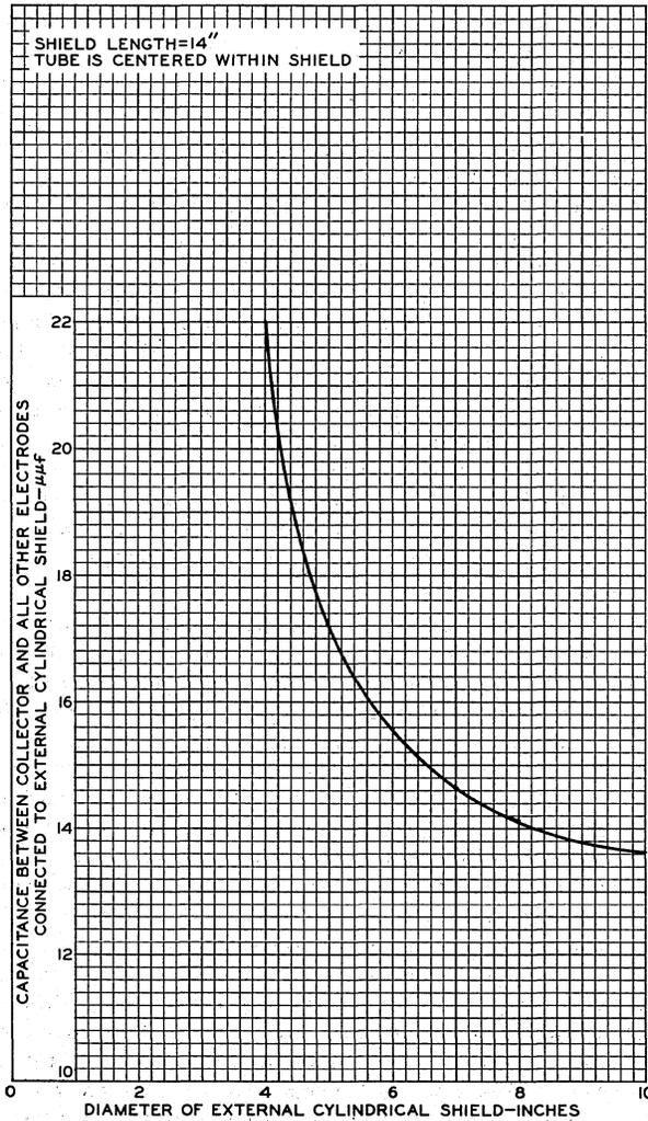
Fig. 5 - Curve Showing Indicated Capacitance vs. Shield Diameter.
