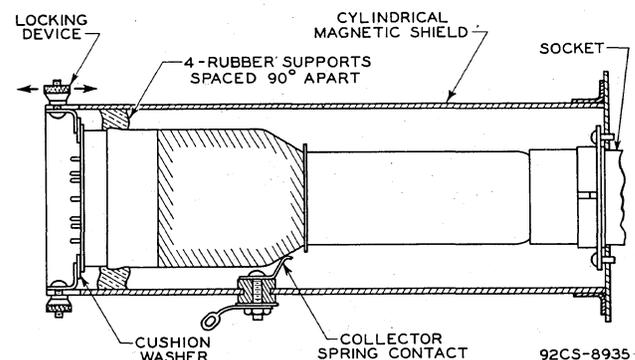
Fig. 7 - Suggested Arrangement for Supporting Type 6499 Within External Magnetic Shield.
