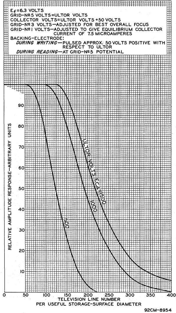
Fig. 8 - Resolution Characteristics of Type 6499.
