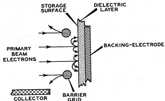
Fig. 2 - Storage Surface Instantaneously Positive With Respect to Barrier Grid.
