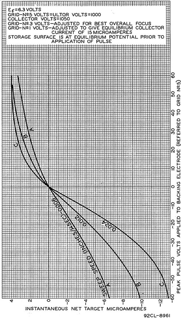
Fig. 10 - Typical Target Characteristics of Type 6499.
