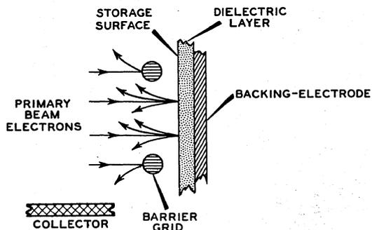
Fig. 3 - Storage Surface Instantaneously Negative With Respect to Barrier Grid.
