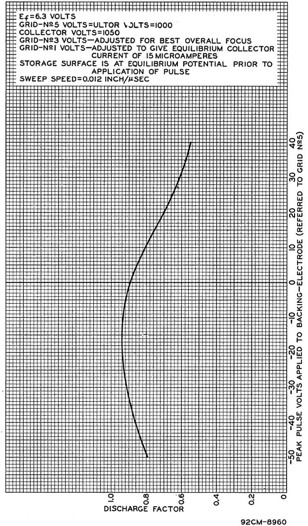
Fig. 11 - Approximate Discharge-Factor Curve of Type 6499.
