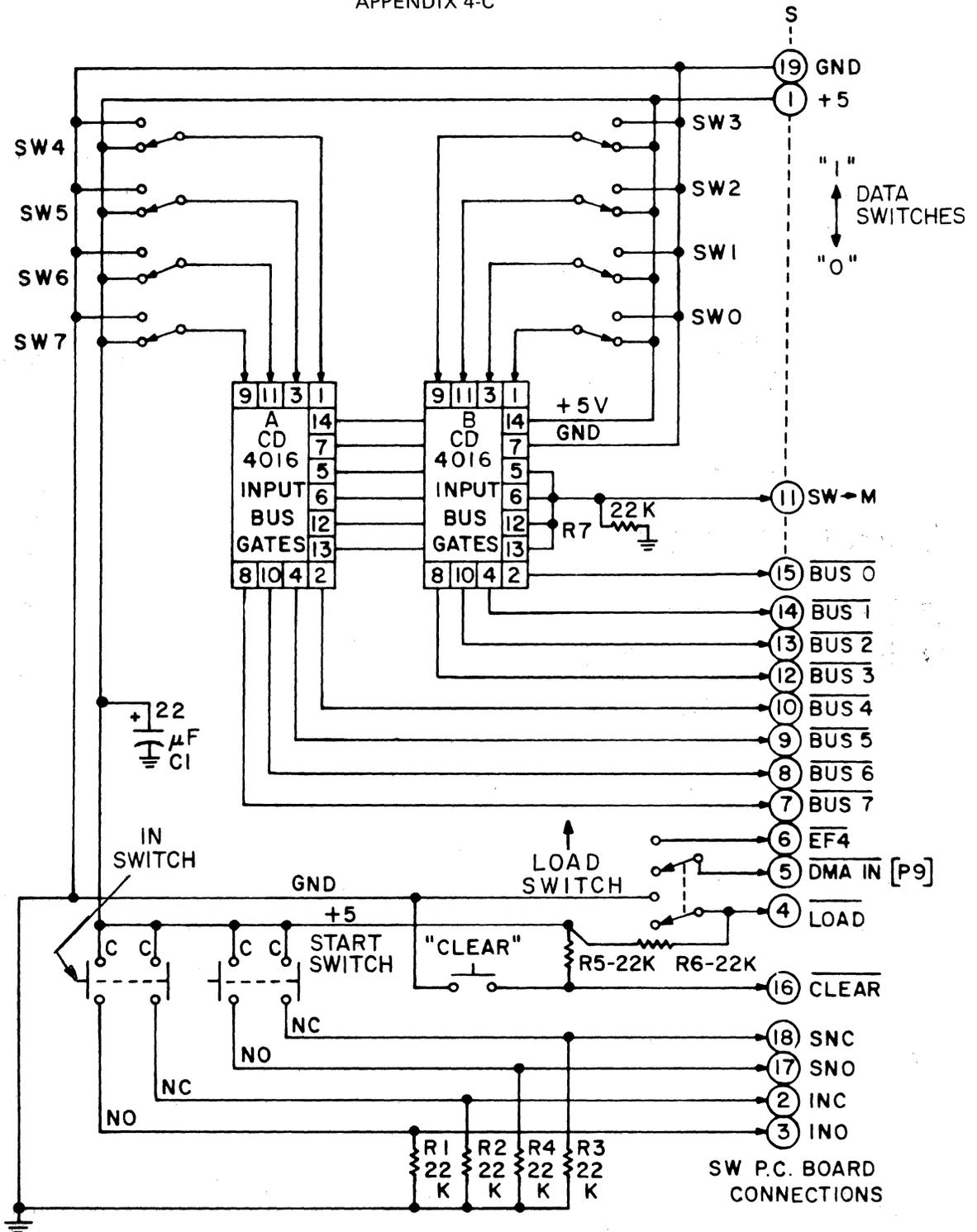
MICROTUTOR Input Byte Switch Logic
