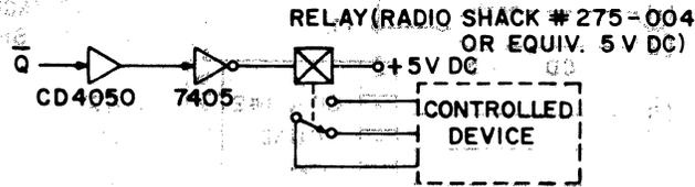
Fig. 6—Output Relay Circuit.
