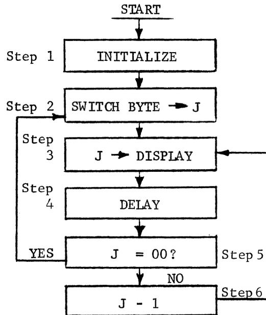
We will let the byte at M(00) represent the variable J. Translating the above flow chart steps into sequences of instruction bytes yields the following program. Don't forget that programs are loaded into memory starting at address 00 but that the program begins execution with the instruction byte at M(01):
