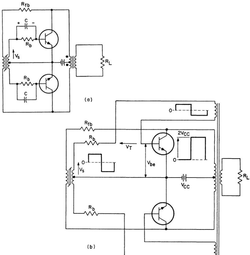
Figure 210. Two-transistor, two-transformer push-pull switching converters in which transistor-storage times are reduced: (a) Capacitor in parallel with each base resistor assures sharp turn-off of associated transistor; (b) Feedback winding from output transformer in series with base of each transistor assures sharp cutoff characteristics.
