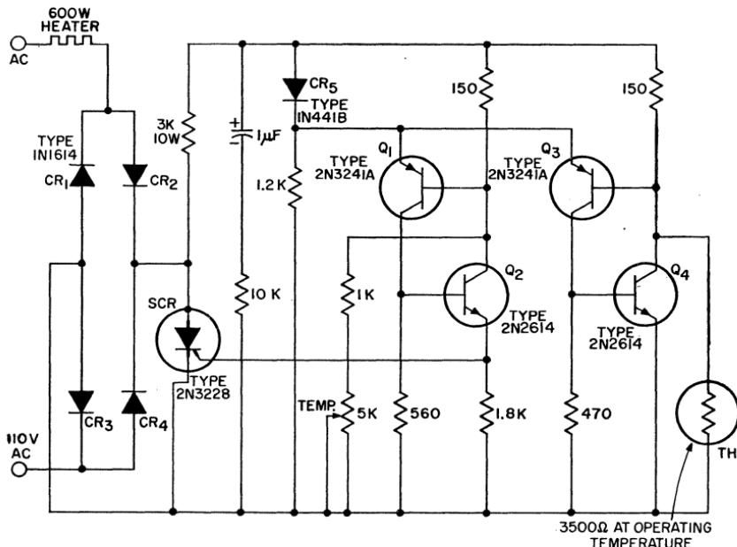
Figure 286. Half-wave SCR heater control circuit.
