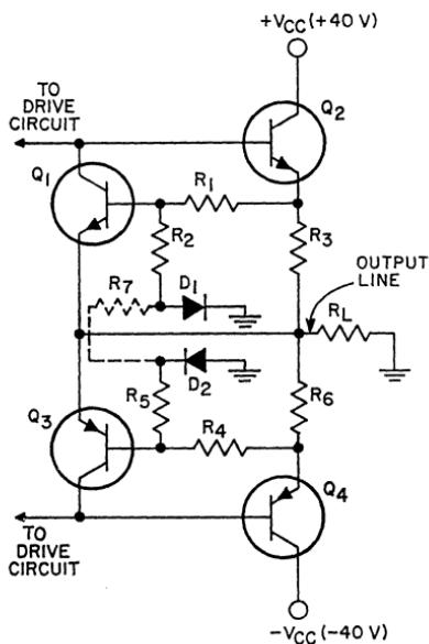
Figure 447. Quasi-complementary audio output in which diode-resistor biasing network is used to prevent complementary transistors  $Q_1$  and  $Q_2$  from being forward-biased by the output voltage swing.
