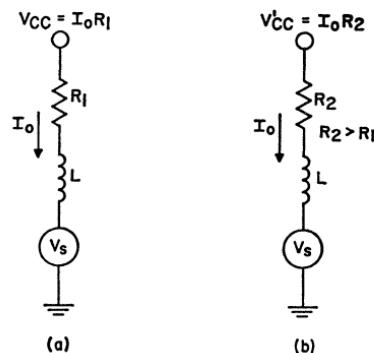
Figure 175. Circuits used in Example 1 to demonstrate the use of case-4 equations.
