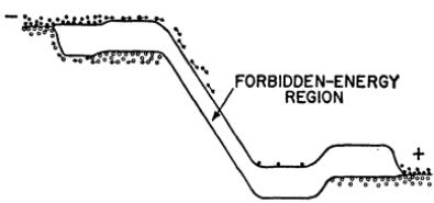
(c) CHANGE IN POTENTIAL CONFIGURATION WHEN POSITIVE BIAS IS APPLIED TO GATE
