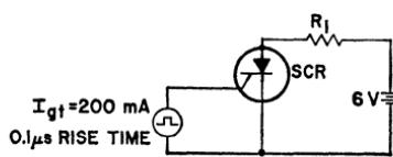
Figure 50. Test circuit used to determine turn-on time of thyristors.
