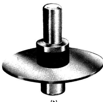
Figure 376. RCA-2N5470 coaxial transistor
