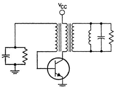
Figure 467. Class C oscillator that operates into a tuned load circuit.
