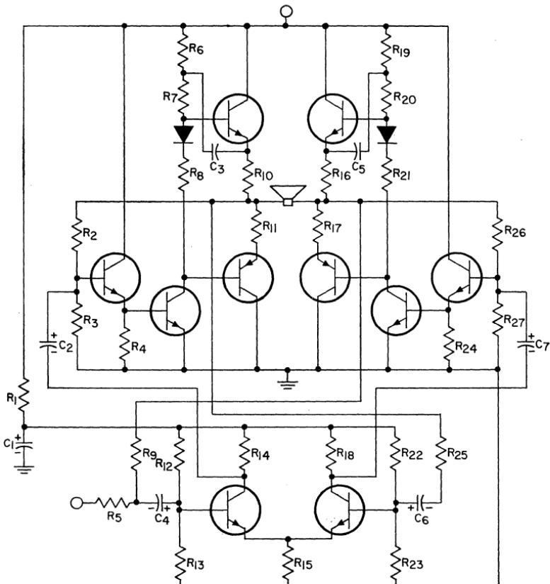
Figure 454. Basic circuit configuration for a bridge type of audio amplifier.
