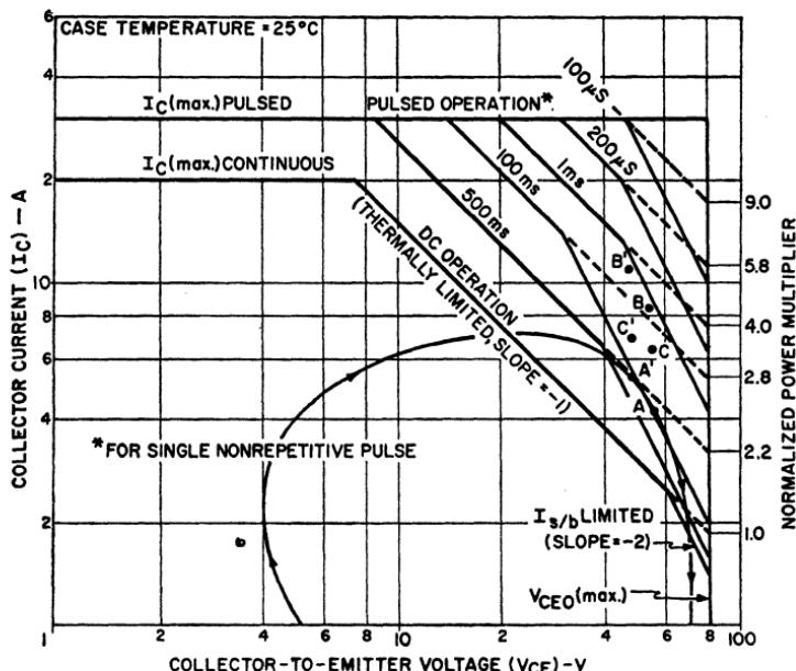
Figure 118. Safe-area rating chart for an RCA 40411 transistor.
