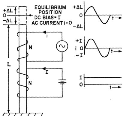
Figure 460. Reaction of bar of material that has a positive strain coefficient to an alternating magnetic field when static biasing is employed. Waveforms show change in length of bar (top), alternating current used to produce alternating field (center), and direct current (bottom) used to produce the bias field.
