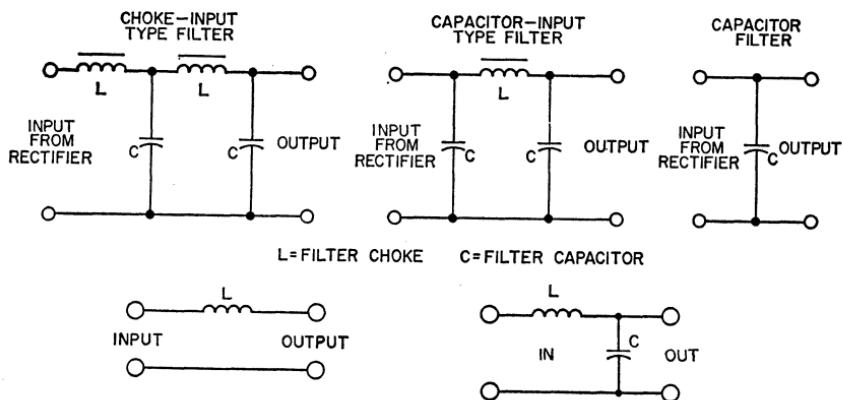
Figure 186. Typical filter circuits.
