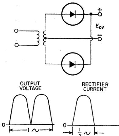
Figure 180. Single-phase full-wave circuit with center-tapped power transformer.
