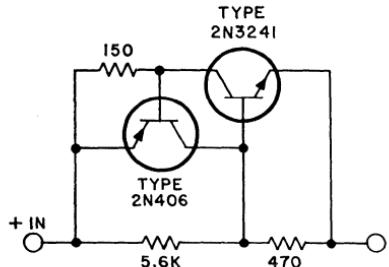
Figure 270. Two-transistor switch. Characteristics of this circuit are similar to those of a trigger diode.
