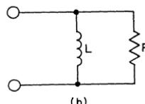
Figure 462. (a) Actual equivalent circuit and (b) simplified approximation of a magnetostrictive transducer.
