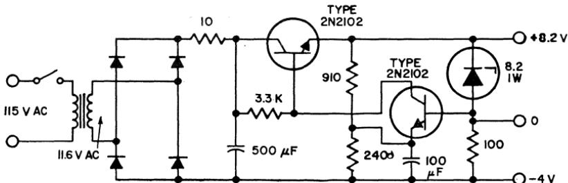
Figure 235. Schematic diagram of reference voltage supply for regulated power supply shown in Fig. 234.
