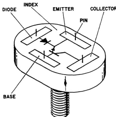
Figure 335. Package outline for the RCA SSB developmental transistor showing internal-package diode used for transistor bias-point control.
