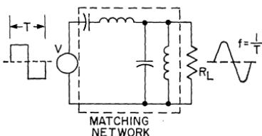
Figure 465. Use of a transducer and resonant matching network to convert a square-wave input to a sinusoidal output. Reactive component of transducer is used as the shunt inductor or capacitor of the matching network depending upon whether a magnetostrictive or electrostrictive type of transducer is used.
