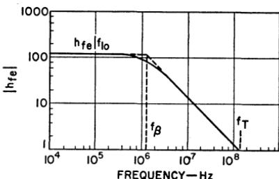
Figure 143. Magnitude of  $h_{fe}$  as a function of frequency for the 2N2102 silicon power transistor.
