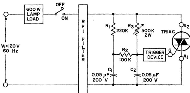
Figure 290. Double-time-constant phase-control circuit for brightness control of incandescent lamps in which a small amount of triac current flows when potentiometer is set for maximum resistance.
