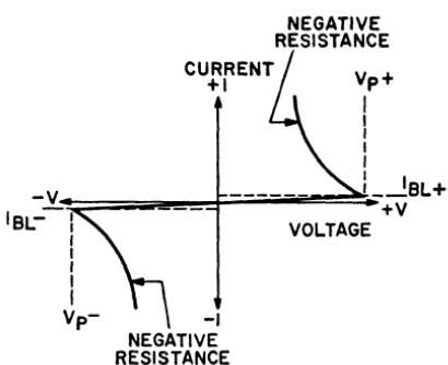
Figure 259. Voltage-current characteristic for triggering-device shown in Fig. 258.
