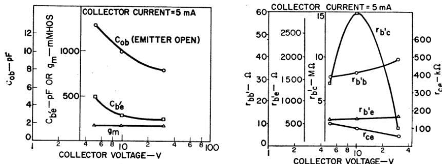
Figure 149. Hybrid-pi parameters as a function of collector voltage for the 2N2102 silicon power transistor.
