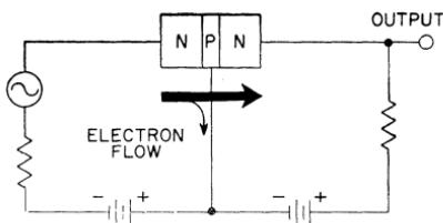
Figure 9. N-P-N structure biased for power gain.
