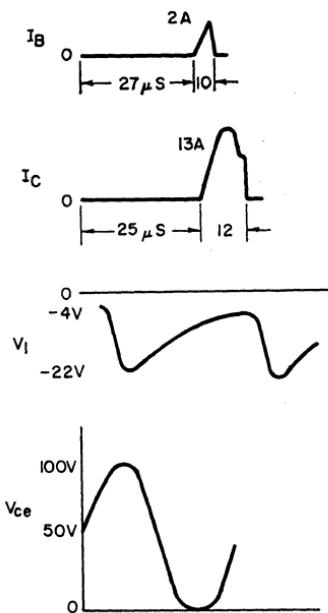
Figure 473. Current and voltage waveforms for the class C oscillator shown in Fig. 472.
