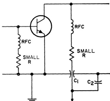
Figure 398. Circuit showing biasing techniques and bypassing capacitances used to eliminate instabilities in common-emitter frequency multipliers.
