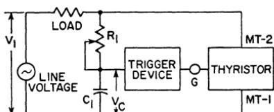
Figure 258. Thyristor power control in which switching is controlled by basic triggering-device circuit.
