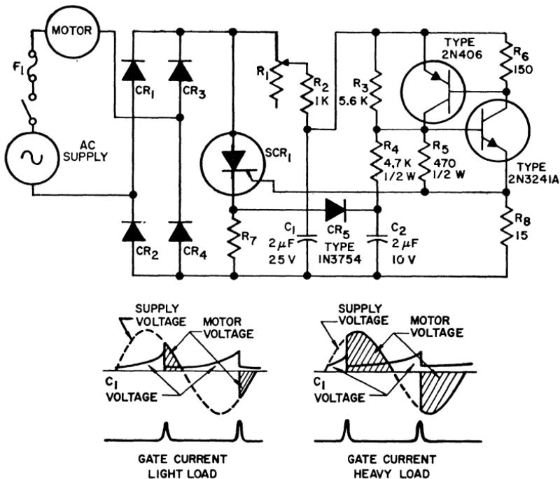
Figure 281. Full-wave SCR motor control circuit, with regulation.
