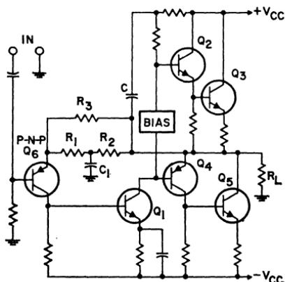
Figure 430. Quasi-complementary audio power amplifier that operates from symmetrical dual dc power supplies. The p-n-p transistor input stage is required to prevent ripple component from driving amplifier.
