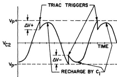
Figure 291. Voltage waveform across triggering capacitor  $C_2$  in double-time-constant circuits shown in Figs. 289 and 290.
