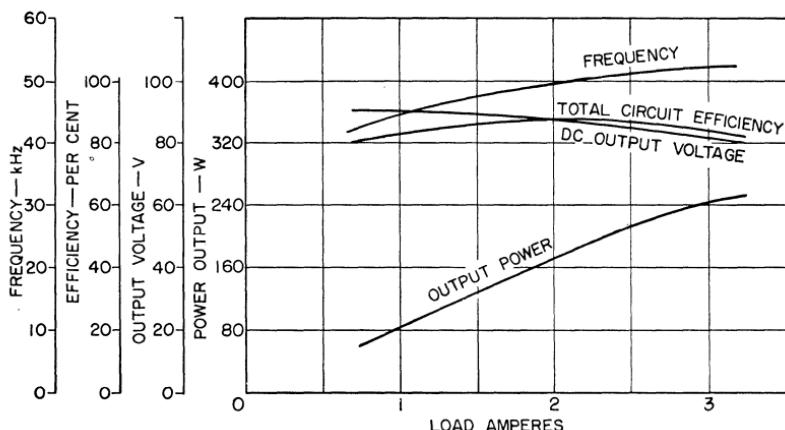
Figure 214. Output characteristics (i.e., frequency, efficiency, voltage, and power) of the 250-watt converter as a function of the load.
