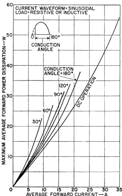
Figure 39. Power-dissipation rating chart for the RCA-2N3873 SCR.
