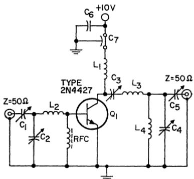
$C_1, C_2, C_4, C_5 = 7\text{-to}-100 \text{ pF Arco 423 or equiv.}$
