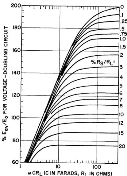
Figure 195. Relationship of applied ac peak voltage to dc output voltage in capacitor-input voltage-doubling circuit.
