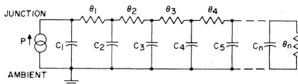
Figure 83. Simplified equivalent circuit for transistor structure shown in Fig. 81.
