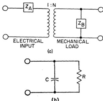
Figure 464. (a) Actual equivalent circuit and (b) simplified approximation of a piezoelectric crystal.
