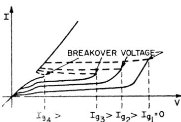
Figure 28. Curves showing breakdown characteristics of a thyristor for different values of gate current.
