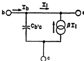
Figure 141. Simplified form of hybrid-pi equivalent circuit shown in Fig. 140.
