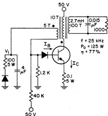
Figure 472. 125-watt, 25-kHz, class C oscillator.
