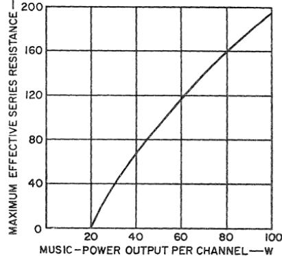
Figure 440. Maximum effective series resistance as a function of music power output.
