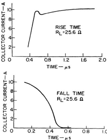
Figure 217. Collector-current rise and fall times.
