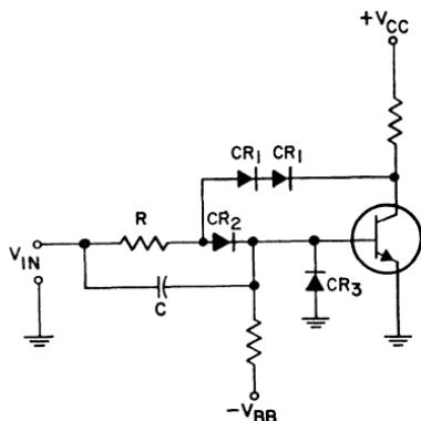
Figure 164. Practical "collector-catcher" circuit.
