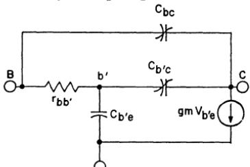
Figure 297. Simplified high-frequency equivalent circuit for an "overlay" transistor.
