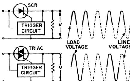
Figure 246. Integral-cycle thyristor power control circuits.
