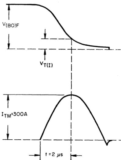
Figure 51. Initial ON-state voltage and current waveforms for the 2N3873 SCR.
