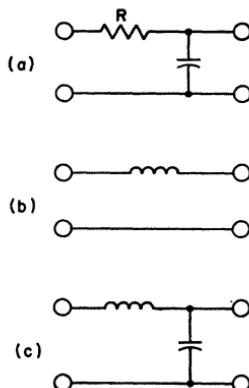
Figure 240. Typical filter circuits for use between pass element and load in a switching regulator: (a) capacitive filter; (b) inductive filter; (c) inductive-capacitive filter.
