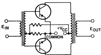
Figure 413. Basic class AB, push-pull, transformer-coupled amplifier.
