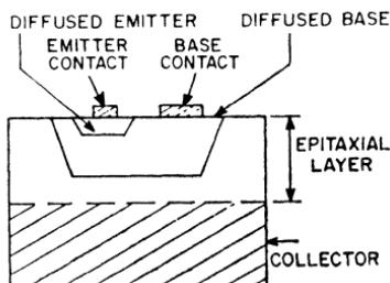
Figure 81. Structure of double-diffused epitaxial planar transistor.
