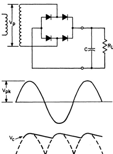
Figure 187. Bridge-rectifier circuit with capacitor input filter.
