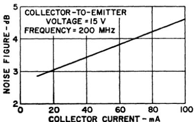
Figure 358. Noise figure as a function of collector current for a typical RCA-2N5109 transistor.
