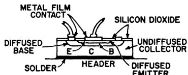
Figure 71. Cross-section of double-diffused silicon planar power transistor.
