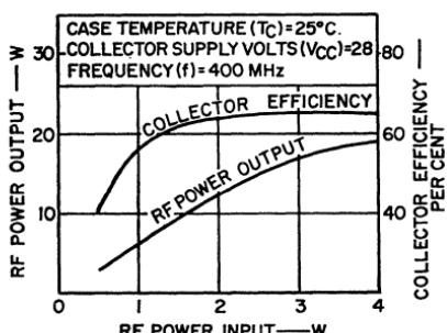
Figure 373. Typical power output or collector efficiency as a function of power input at 400 MHz.
