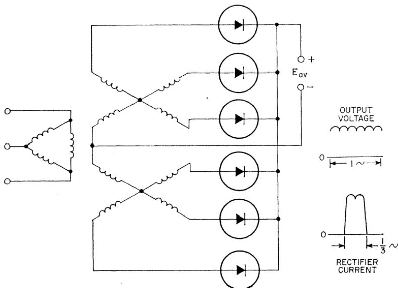
Figure 185. Three-phase "double-Y" and interphase-transformer circuit.
