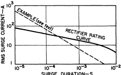
Figure 191. Surge rating chart for stack rectifier CR210.
