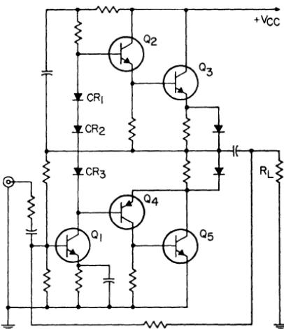
Figure 441. Quasi-complementary amplifier that incorporates two stabilization networks.
