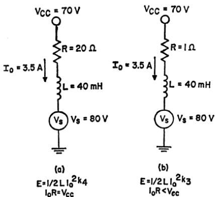
Figure 176. Circuits used in Example 2 to show the difference between cases 3 and 4.
