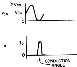
Figure 469. Collector voltage and current waveforms for the Class C oscillator shown in Fig. 467.
