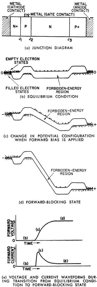
Figure 29. Potential-hill diagrams for various stages of thyristor transition from equilibrium condition to forward-blocking condition (electron energy increases upward, hole energy increases downward).
