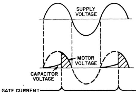
Figure 272. Half-wave SCR motor control circuit, without regulation.
