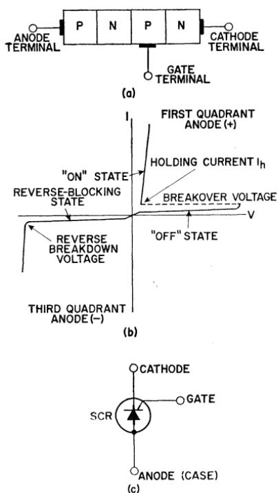
Figure 25. (a) Junction diagram, (b) principal voltage-current characteristic, and (c) schematic symbol for an SCR thyristor.
