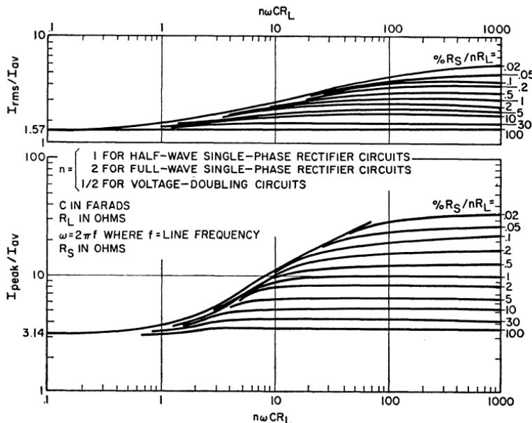
Figure 192. Relationship of peak, average, and rms rectifier currents in capacitor-input circuits.
