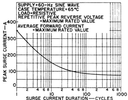
Figure 42. Surge-current rating curve for the RCA-2N3873 SCR.
