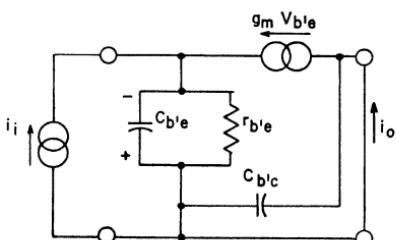
Figure 145. High-frequency common-base hybrid-pi transistor model used for calculation of  $h_{fb}$  (transverse voltage drops in the base are neglected).
