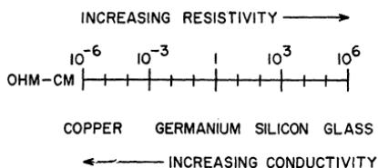
Figure 1. Resistivity of typical conductor, semiconductor, and insulator.
