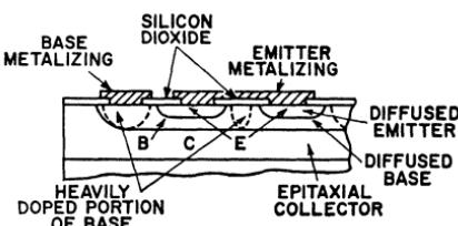
Figure 76. Cross-section of overlay transistor.
