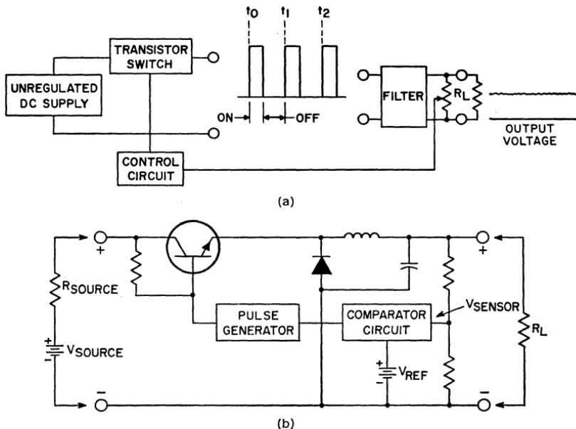
Figure 239. Basic configuration of switching type of transistor voltage regulator:
