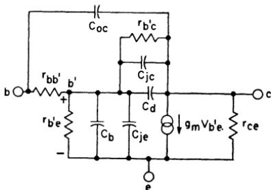
Figure 125. Complete hybrid-pi equivalent circuit for a transistor used in a common-emitter configuration.
