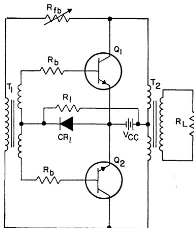
Figure 212. Two-transistor, two-transformer push-pull inverter that uses a diode starting circuit.
