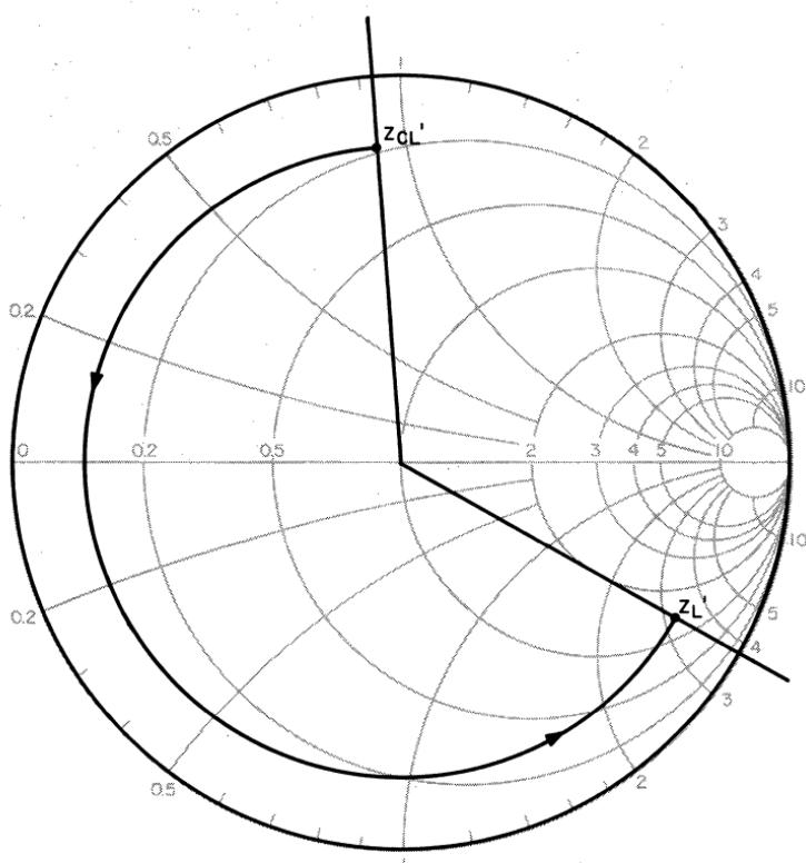
Figure 317. Smith-chart admittance plot for design of output transmission-line matching section.
