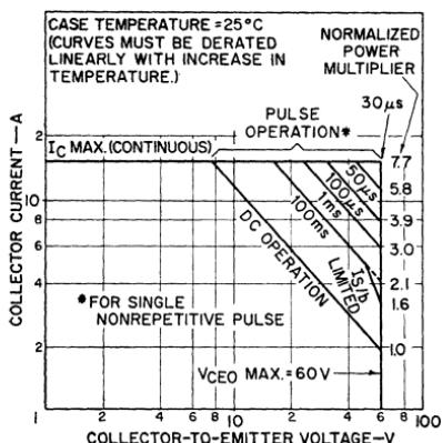
Figure 444. Safe-area-of-operation rating chart for the RCA-2N3055 homotaxial-base transistor.
