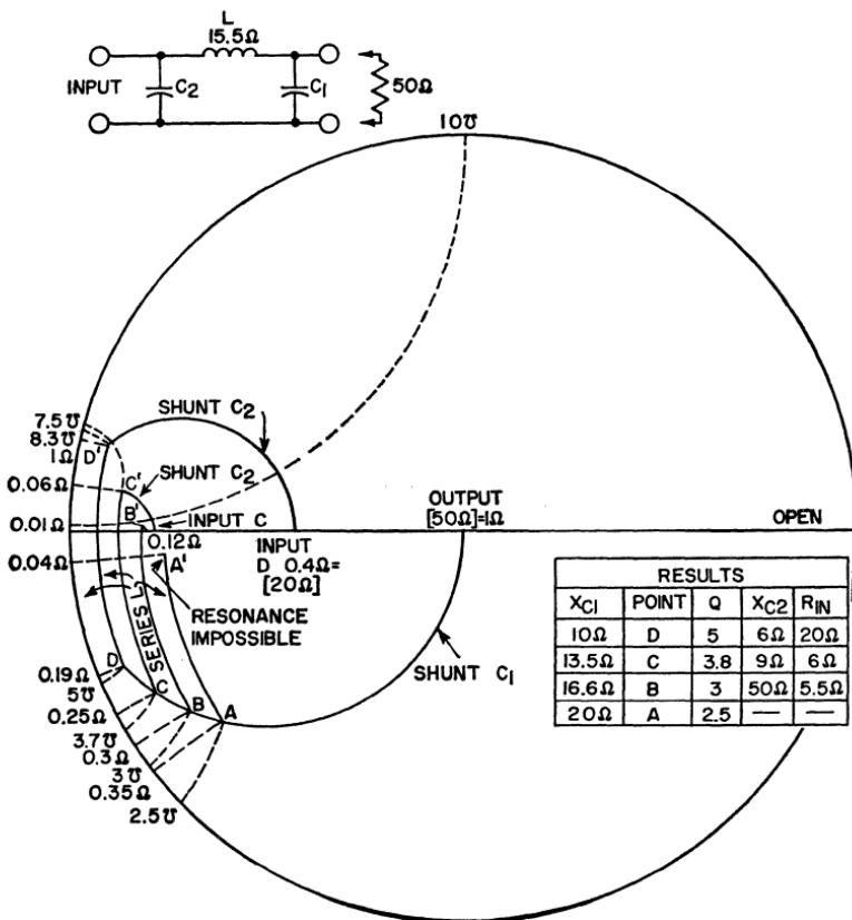
Figure 315. Circuit configuration for pi matching network and network map showing tuning range for variable components used in this type of matching network.
