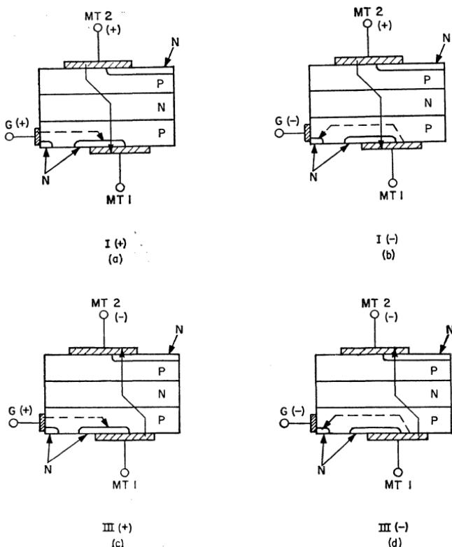
Figure 27. Current flow in the four triggering modes of a triac: (a) Mode I(+);
