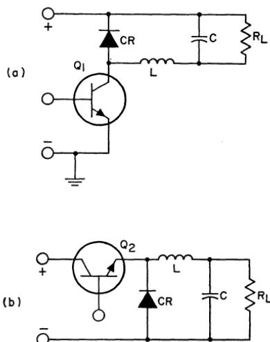
Figure 243. Basic transistor switching arrangements: (a) filter elements and load impedance in collector circuit of switching transistor; (b) filter elements and load impedance in emitter circuit of switching transistor.
