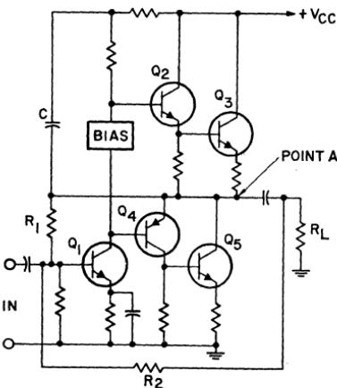
Figure 429. Quasi-complementary audio power amplifier that operates from a single dc supply.
