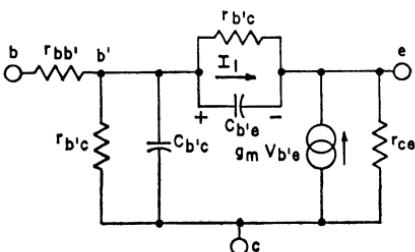
Figure 140. Hybrid-pi equivalent circuit for a transistor used in a common-collector configuration.
