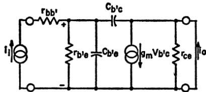
Figure 142. Medium- and high-frequency common-emitter hybrid-pi transistor model used for calculation of  $h_{fe}$ .
