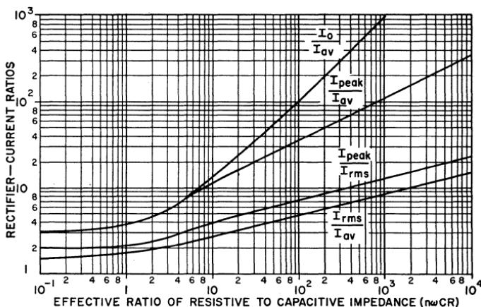
Figure 193. Forward-current ratios for rectifiers in capacitor-input circuits in which  $R_s$  is much less than  $1/C$ .
