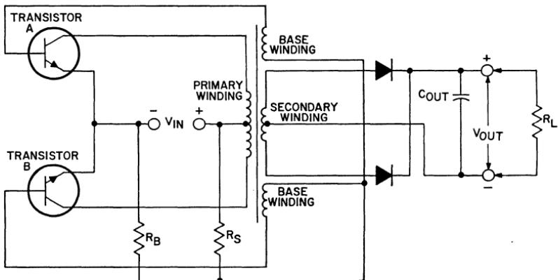
Figure 205. Two-transistor, one-transformer push-pull switching converter.
