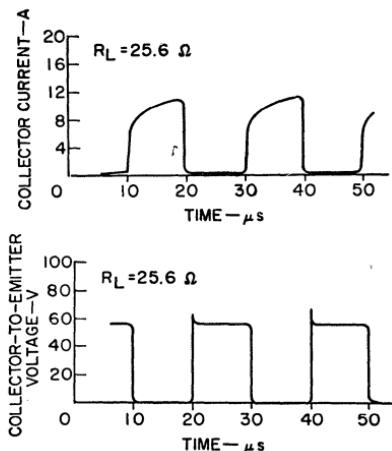
Figure 216. Collector-current and voltage waveforms for the 2N3265 transistors used in the 250-watt converter.
