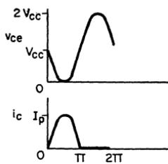
Figure 470. Collector voltage and current waveforms for an oscillator circuit that has a conduction angle of 180 degrees.
