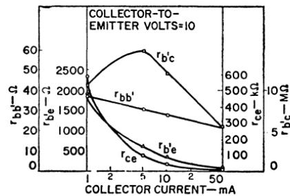
Figure 148. Hybrid-pi parameters as a function of collector current for the 2N2102 silicon power transistor.
