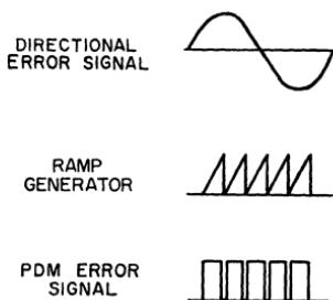
Figure 478. Input and output waveforms for the pulse-duration-modulated servo control system.
