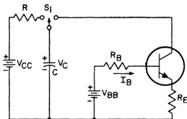
Figure 104. Capacitive-discharge test circuit used to determine forward-bias second-breakdown energy levels in transistors.
