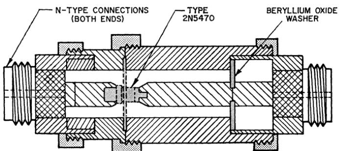
Figure 377. Heat sink for use with coaxial transistor package.
