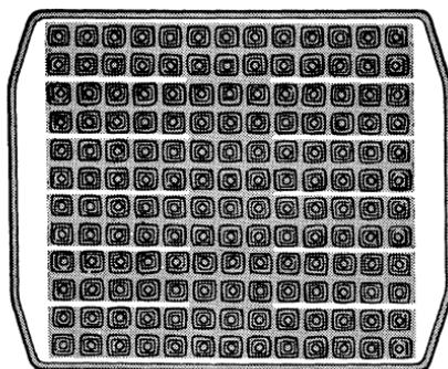
Figure 75. Emitter structure of an overlay transistor.
