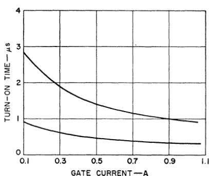
Figure 49. Turn-on time characteristics for the RCA-2N3873 SCR.
