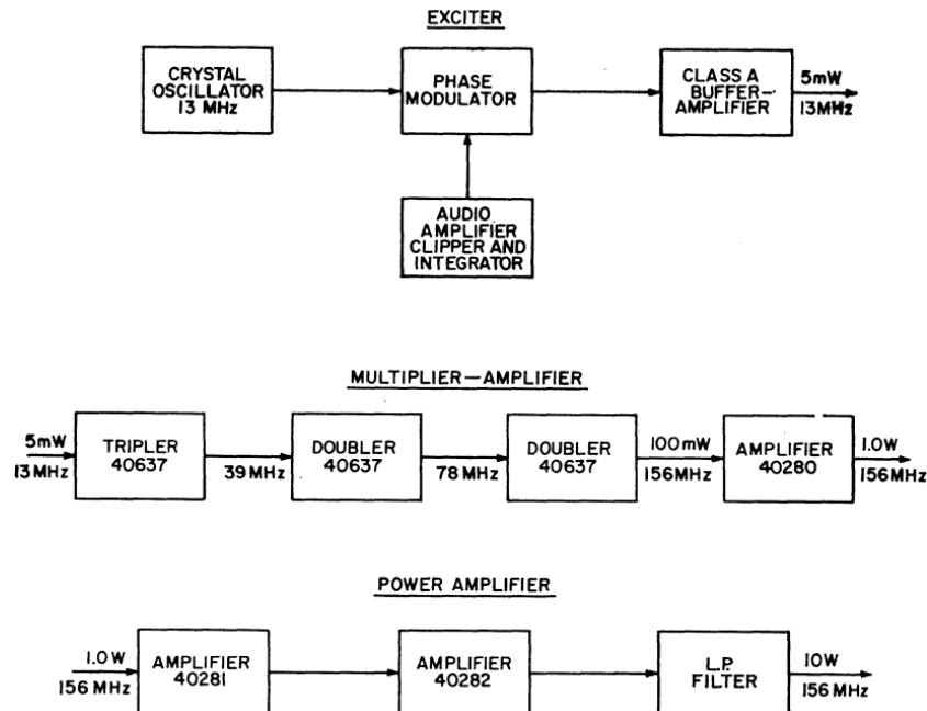
Figure 320. Block diagram of a typical vhf FM marine-band transmitter.
