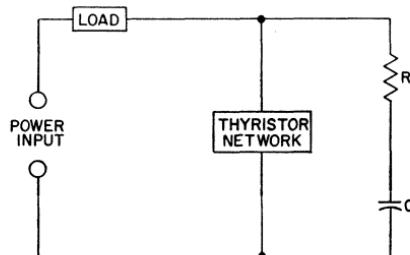
Figure 63. Diagram showing use of RC network for transient suppression in thyristor circuits.
