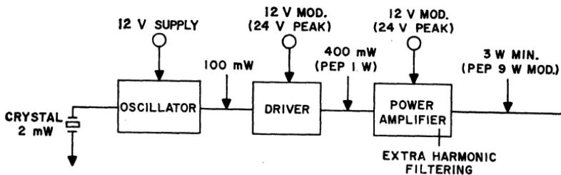
Figure 323. Block diagram of a 5-watt (dc input power to final amplifier) citizens-band transmitter.
