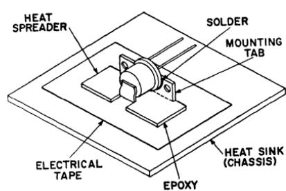
Figure 34. Typical heat-sink isolation technique for a chassis-mounted two-lead TO-5 thyristor.
