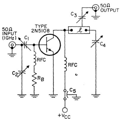
$C_1, C_2, C_3, C_4 = \text{Variable capacitor, } 0.3 \text{ to } 3.5 \mu\text{F}$ , Johanson piston type or equiv.
