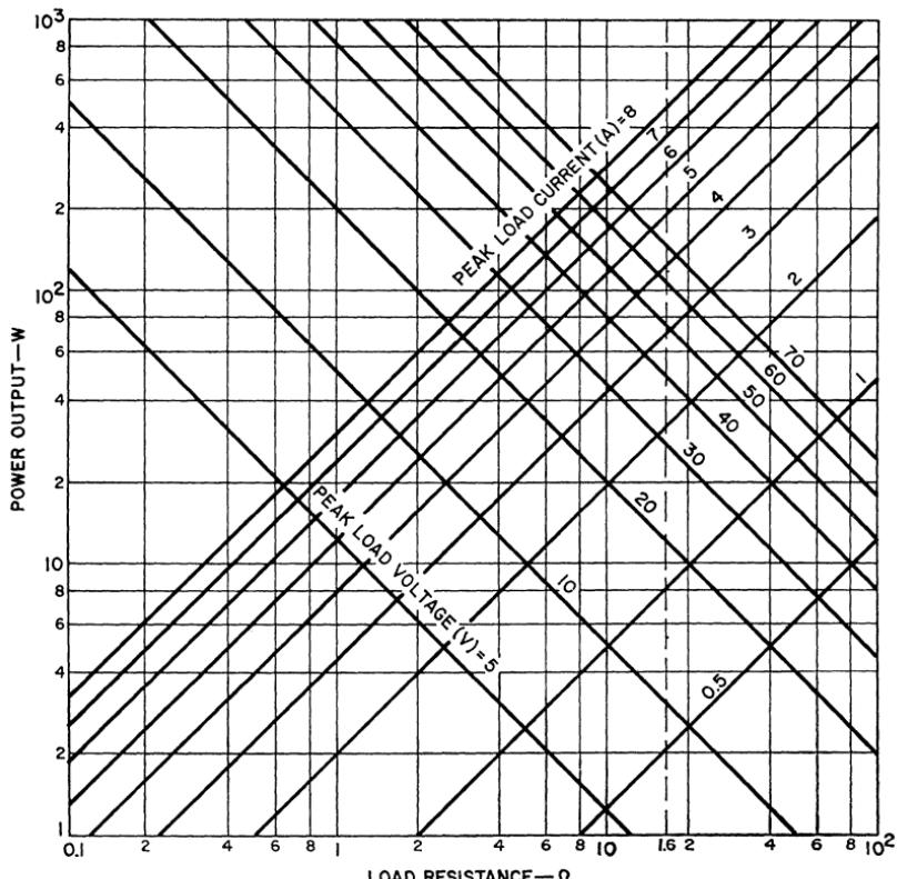
Figure 431. Peak transistor currents and load voltages for various output powers and load resistances.
