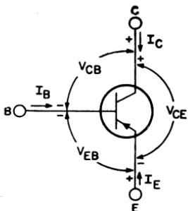
Figure 150. Terminal parameters for a p-n-p transistor.
