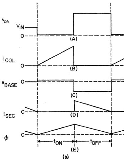
Figure 204. Ringing-choke converter circuit: (a) Schematic diagram; (b) Typical operating waveforms in a ringing-choke converter—(A) primary voltage; (B) primary current; (C) base-to-emitter voltage; (D) secondary current; (E) magnetic flux in transformer core.
