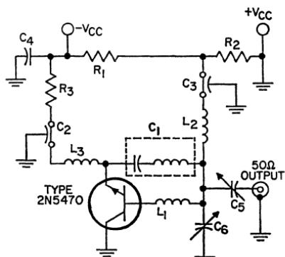
$C_1 = 0.82$  pF, "gimmick" capacitor (manufactured by Quality Components, Inc. St. Mary's, Pa.)
