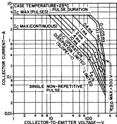
Figure 110. Safe-area rating chart for the 2N3585 silicon power transistor.
