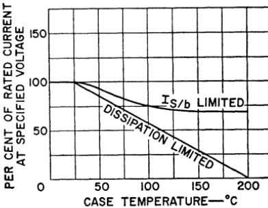
Figure 112. Safe-area temperature-derating curves for the 2N3585 silicon power transistor.
