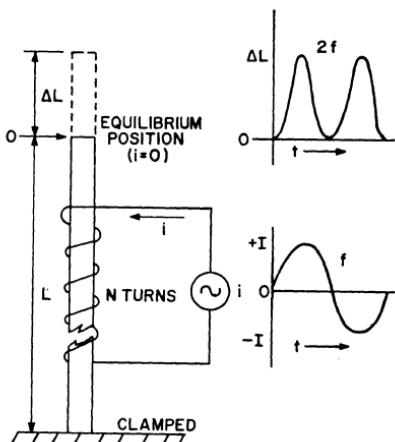
Figure 459. Reaction of a bar of material that has a positive strain coefficient to an alternating magnetic field when no static biasing field is used. Waveforms show change in length of bar (top) and alternating current (bottom) used to produce the magnetic field.
