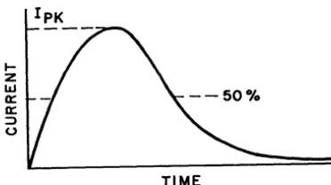
Figure 262. Typical gate-current waveform for circuit shown in Fig. 258.
