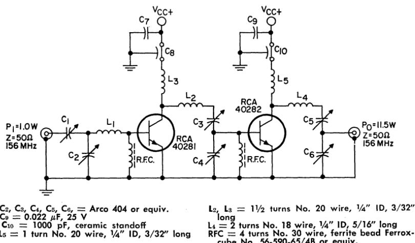
Figure 322. 156-MHz marine-band power amplifier.
