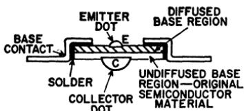
Figure 68. Cross-section of drift-field transistor.
