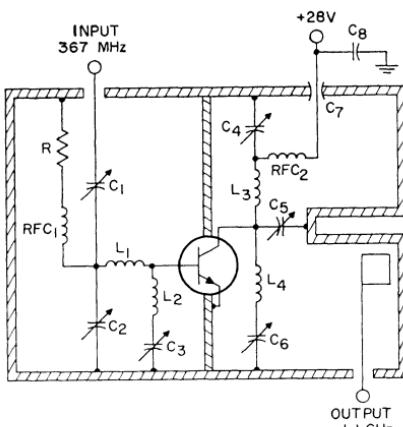
Figure 403. 367-MHz-to-1.1-GHz common-emitter transistor frequency tripler.
