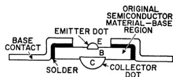
Figure 67. Cross-section of alloy-junction transistor.
