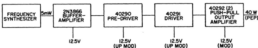
Figure 343. Block diagram of broadband 118-to-136-MHz Aircraft Transmitter.
