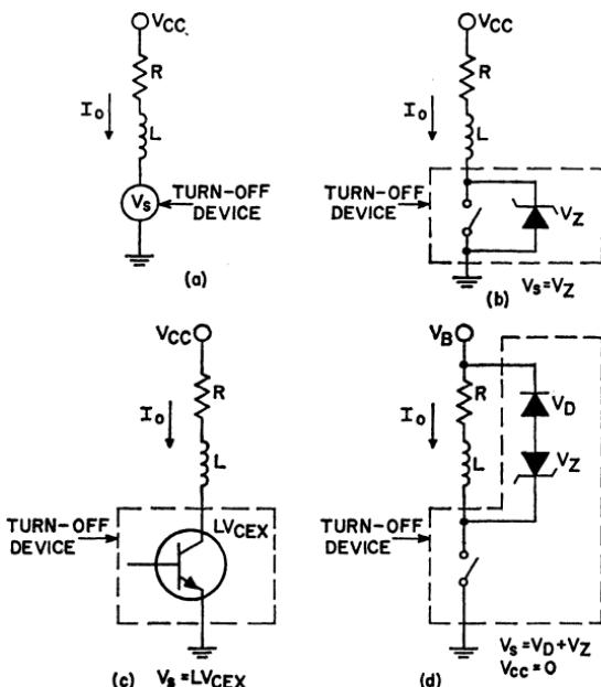
Figure 171. Basic switching circuits with inductive loads.
