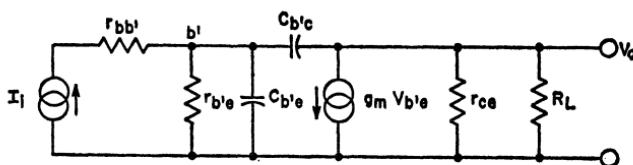
Figure 135. Equivalent circuit for common-emitter amplifier.
