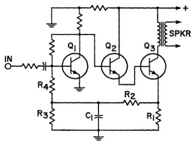
Figure 418. Three-stage, transformer-coupled, class A amplifier.
