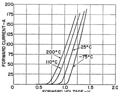
Figure 18. Typical forward characteristics of a silicon rectifier.
