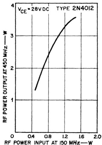
Figure 407. Power output as a function of power input for the 150-to-450-MHz frequency tripler.
