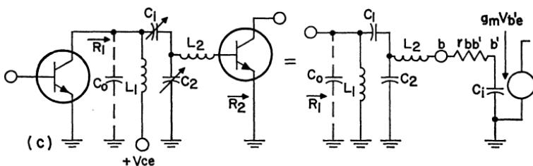
FOR  $R_1 > R_2$ ;  $R_2 = r_{bb'}$ ;  $X_{L_2} \gg X_{C_1}$
