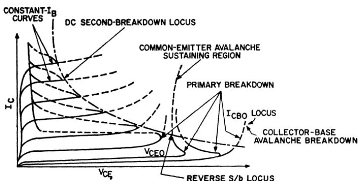
Figure 96. Transistor collector characteristics.
