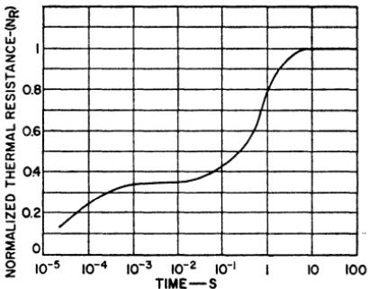
Figure 109. Normalized thermal resistance as a function of the duration of applied power for the 2N3442 silicon power transistor.
