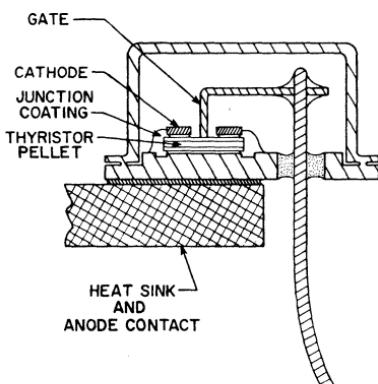
Figure 33. Cross-section of RCA two-lead TO-5 thyristor package.
