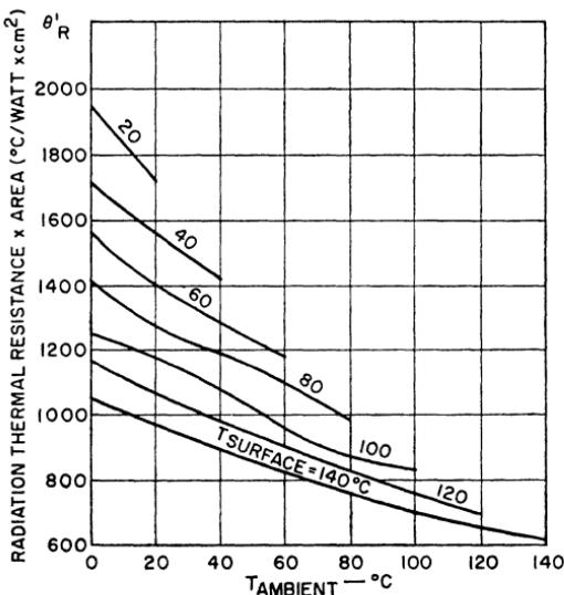
Figure 91. Radiation thermal resistance as a function of ambient temperature for various heat-sink surface temperatures. (Reprinted from *Control Engineering*, October 1956.)
