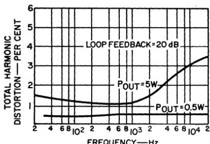
Figure 456. Total harmonic distortion of the bridge audio amplifier as a function of frequency.
