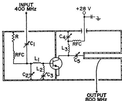
Figure 400. 400-to-800-MHz common-emitter transistor frequency multiplier.
