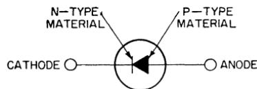
Figure 10. Schematic symbol for a semiconductor diode.
