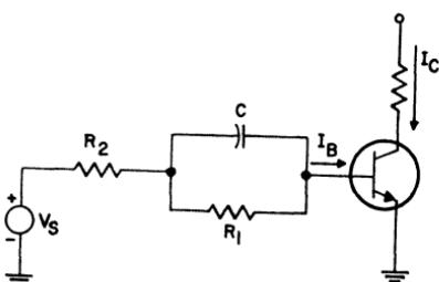
Figure 165. Circuit that uses speed-up capacitor to reduce transistor switching times.
