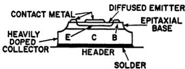
Figure 73. Cross-section of epitaxial-base silicon power transistor.
