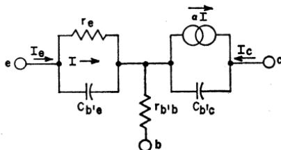
Figure 139. "T" equivalent circuit for a transistor used in a common-base configuration when the effects of base-width modulation are neglected.
