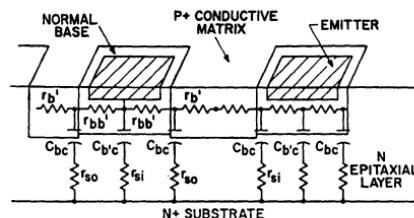
Figure 391. Cross-sectional view of an overlay transistor indicating the capacitance and loss distributions.
