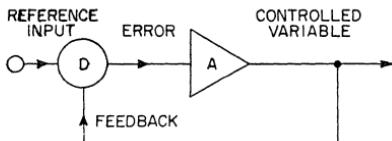
Figure 474. Block diagram of a simple control system that uses direct feedback.
