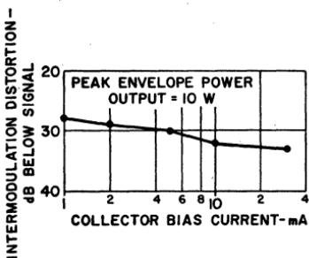
Figure 333. Intermodulation distortion as a function of collector bias current for the RCA SSB developmental transistor.
