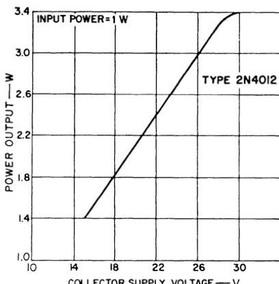
Figure 402. Power output as a function of supply voltage for the 400-to-800-MHz frequency doubler.
