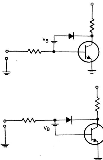
Figure 163. "Collector-catcher" circuits in which feedback is used.
