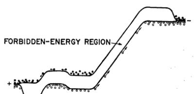
(e) THYRISTOR APPROACHES REVERSE-BLOCKING STATE, BUT DEPLETION LAYER BUILT UP IN N-TYPE BASE STILL CONTAINS SOME EXCESS CHARGE CARRIERS.
