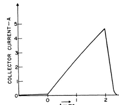
Figure 106. Test waveforms for a 2N3442 transistor subjected to  $E_{S/b}$  inductive energy test.
