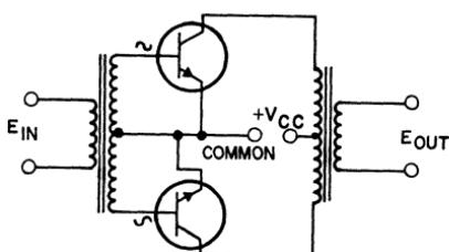
Figure 412. Basic class B, push-pull transformer-coupled amplifier.
