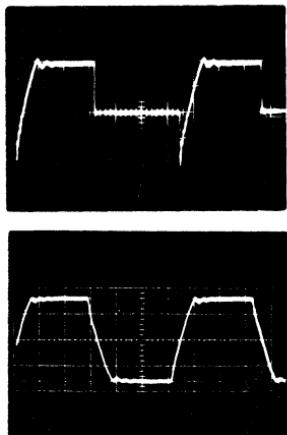
Figure 219. Typical operating waveforms for SCR inverter shown in Fig. 218.
