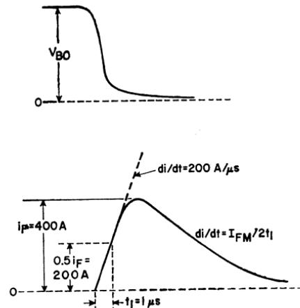
Figure 44. Voltage and current waveforms used to determine  $di/dt$  rating of the RCA-2N3873 SCR.
