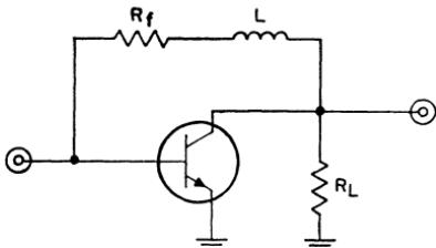
Figure 349. Common-emitter amplifier that uses shunt RL feedback to increase circuit bandwidth.
