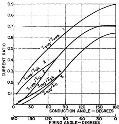
Figure 250. Ratio of thyristor current as a function of conduction and firing angles for single-phase full-wave conduction into a resistive load.
