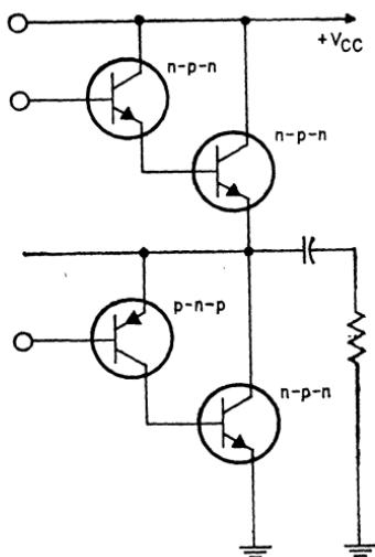
Figure 425. Basic quasi-complementary type of series-output circuit.
