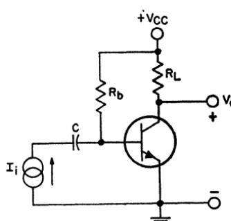
Figure 134. Common-emitter transistor amplifier.
