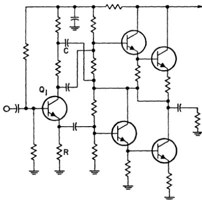
Figure 423. Push-pull series-output amplifiers are connected as Darlington pairs and drive-signal phase inversion is provided by phase-splitter stage  $Q_1$ .
