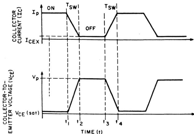
Figure 167. Idealized collector current and voltage waveforms for a transistor that has equal turn-on and turn-off currents.
