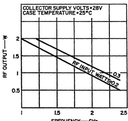
Figure 383. Power output as a function of frequency for the RCA-2N5470 transistor.
