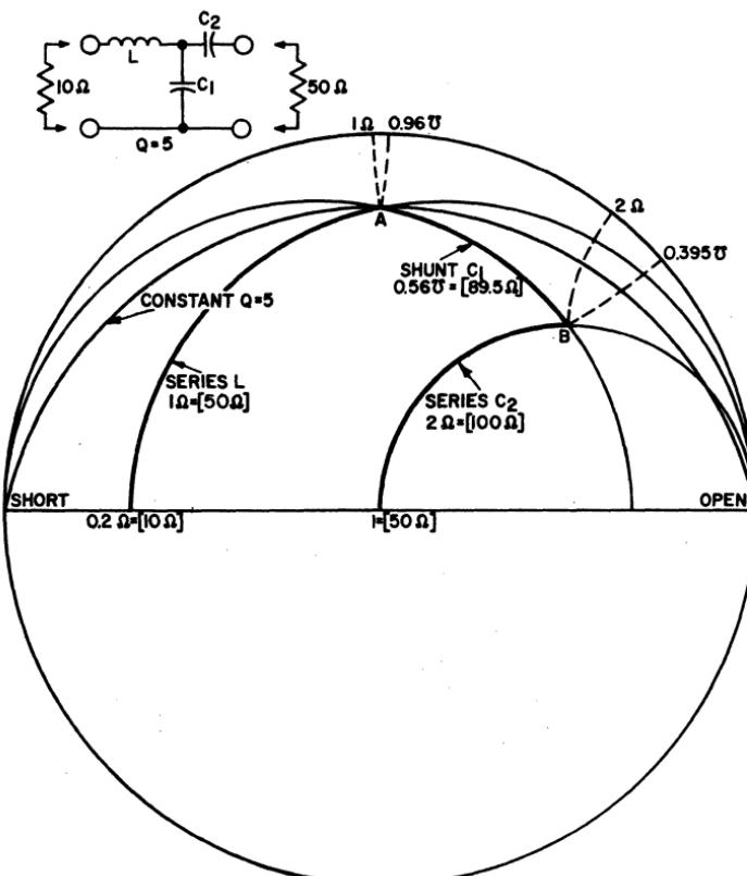
Figure 313. Circuit configuration and the network map used to determine the component values for a "lossy"-L matching network.
