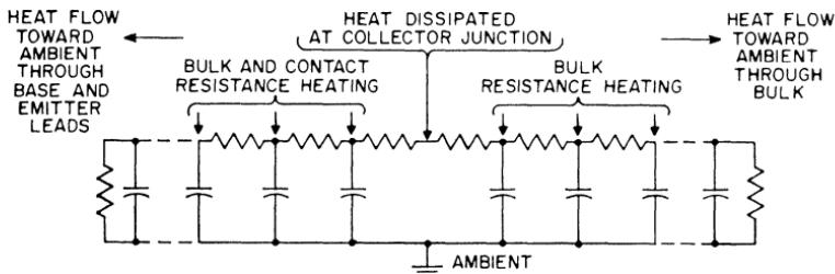
Figure 82. Thermal equivalent circuit for transistor structure shown in Fig. 81.
