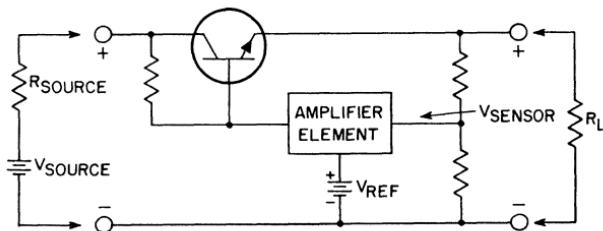
Figure 222. Basic series voltage regulator.
