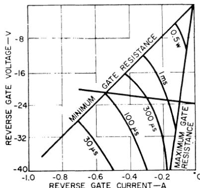
Figure 62. Reverse gate characteristics for typical RCA SCR's showing load line for a reverse gate-source voltage of 24 volts and an external circuit resistance of 5 ohms.
