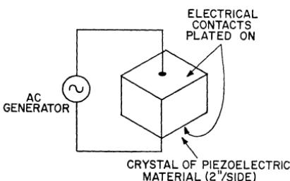
Figure 461. Application of an alternating voltage to a piezoelectric crystal to produce high-frequency sound waves.
