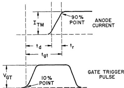
Figure 48. Gate current and voltage turn-on waveforms for a thyristor.
