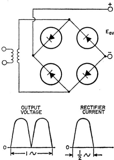
Figure 181. Single-phase full-wave circuit without center-tapped power transformer (i.e., bridge-rectifier circuit).
