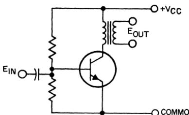
Figure 411. Basic class A, transformer-coupled amplifier.
