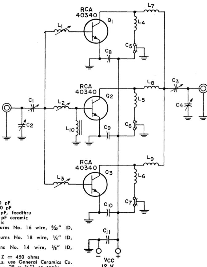
Figure 325. 50-MHz parallel-transistor power amplifier that delivers 50 watts of output power from a 12-volt dc supply.
