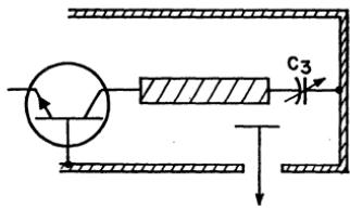
Figure 316. Capacitive-probe-coupled output cavity.
