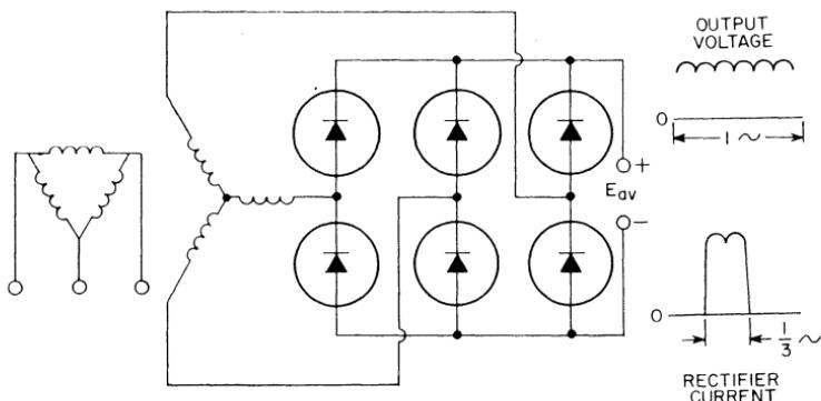
Figure 183. Three-phase "Y" full-wave circuit.
