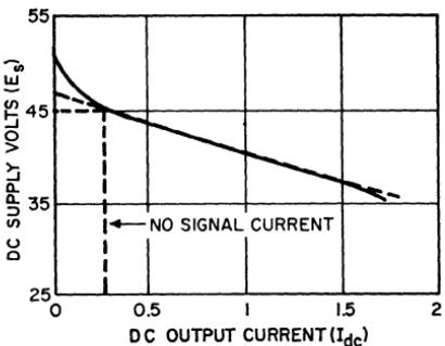
Figure 435. Typical power-supply regulation curve.
