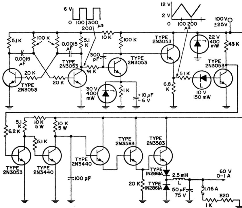
Figure 244. Typical step-down transistor switching regulator.
