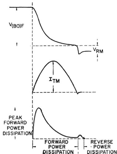
Figure 52. Instantaneous power dissipation in a thyristor during turn-on.
