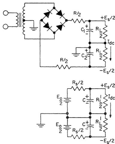
Figure 434. Equivalent circuit for split capacitive-input rectifier supply.
