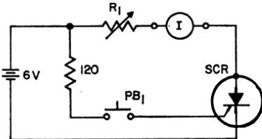
Figure 45. Test circuit used to determine holding and latching currents of thyristors.
