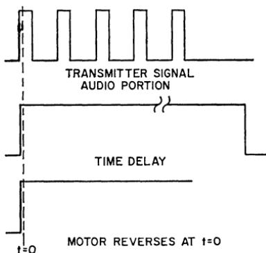
Figure 285. Timing diagram for reversing system.
