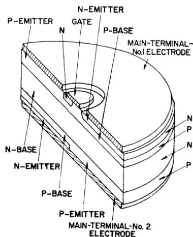
Figure 37. Cross-section of a typical triac pellet.
