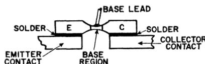
Figure 66. Cross-section of grown-junction transistor.
