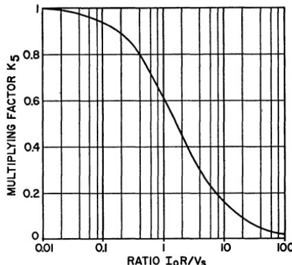
Figure 174. Multiplying factor  $k_5$  as a function of the ratio  $I_o R / V_s$ .
