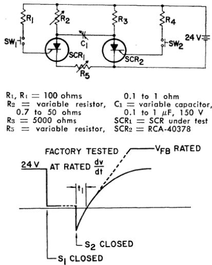
Figure 54. Test circuit and voltage waveforms used to determine turn-off times of thyristors.
