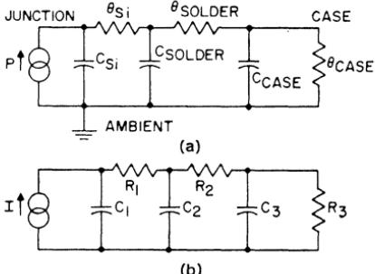
Figure 84. Simplified equivalent circuits for a small-signal medium-power transistor: (a) thermal circuit; (b) electrical analog of thermal circuit.
