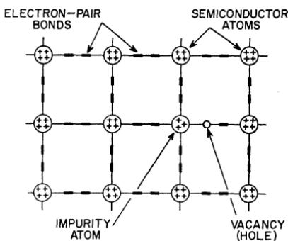
Figure 4. Lattice structure of p-type material.
