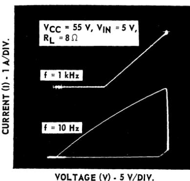
Figure 442. Effect of large signal phase shift on the load-line characteristics of a transistor at low frequencies.
