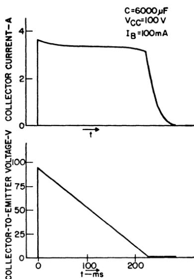
Figure 105. Test waveforms for a 2N3442 transistor subjected to capacitive-discharge second-breakdown energy test.
