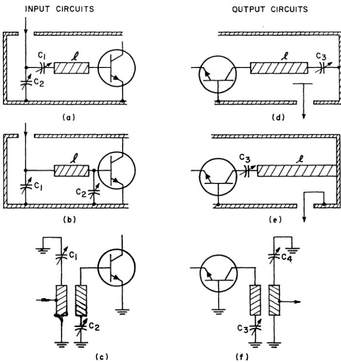
Figure 380. Transistor input and output coupling circuits suitable for use at microwave frequencies: (a) direct-coupled input network using series tuning capacitor; (b) direct-coupled input network using shunt tuning capacitor; (c) resonant-line input circuit; (d) capacitive-probe-coupled output cavity; (e) inductive-probe-coupled coaxial output cavity; (f) resonant-line output circuit.
