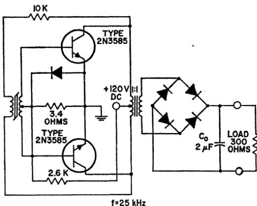
Figure 113. High-speed inverter using RCA 2N3585 transistors.
