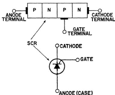
Figure 12. Junction diagrams and schematic symbols for SCR's and triacs.
