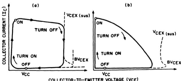
Figure 169. Inductive load line for the test circuit shown in Fig. 168; (a) typical load line; (b) load line when  $L(di/dt) < V_{CEX(\text{sus})}$ .
