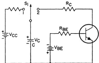
Figure 108. Capacitive-discharge test circuit used to determine reverse-bias second-breakdown energy levels in transistors.
