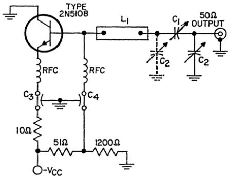
**C<sub>1</sub>, C<sub>2</sub>** = Variable capacitor, 0.35 to 3.5 pF,
