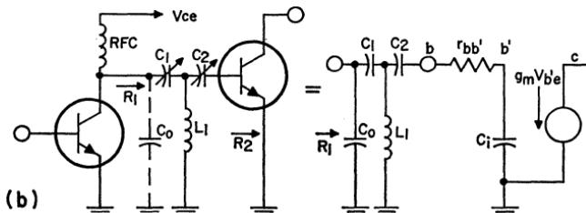
FOR  $X_{C_2} \gg X_{C_1}$ ;  $R_1 > R_2 = r_{bb'}$
