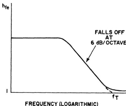
Figure 79. Transistor current-gain parameter  $h_{FE}$  as a function of frequency.
