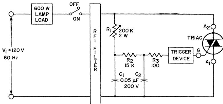
Figure 292. Double-time-constant circuit that uses a series gate resistor.
