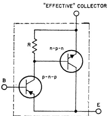
Figure 426. Connection of p-n-p driver transistor to n-p-n output transistor.
