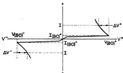
Figure 265. Typical voltage-current characteristic of a bidirectional trigger diac.
