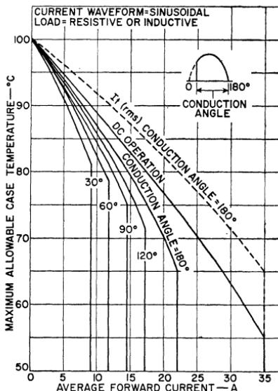
Figure 40. Current rating chart for the RCA-2N3873 SCR.
