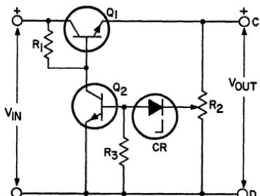
Figure 226. Series voltage regulator without current limiting.
