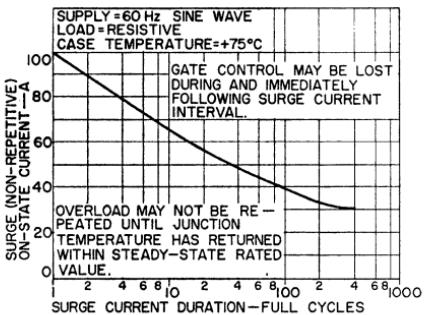
Figure 43. Surge-current rating chart for a typical triac.
