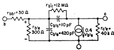
Figure 129. Hybrid-pi equivalent circuit for the 2N2102 triple-diffused silicon planar transistor.
