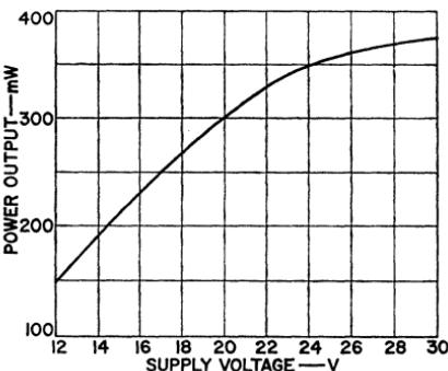
Figure 387. Power output as a function of supply voltage for the 1.68-GHz oscillator shown in Fig. 386.
