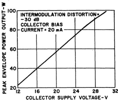
Figure 334. Peak envelope power as a function of collector supply voltage for the RCA SSB developmental transistor.
