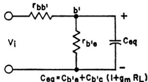
Figure 136. Equivalent input circuit for common-emitter amplifier.
