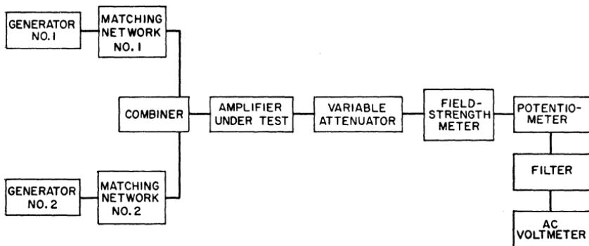
Figure 355. Block diagram of cross-modulation test setup in which a field-strength meter is used.
