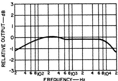
Figure 457. Relative response of the bridge audio amplifier.
