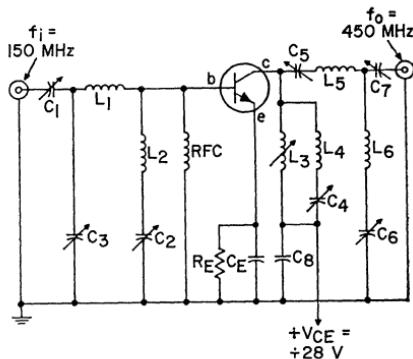
Figure 406. 150-to-450-MHz common-emitter transistor frequency tripler.
