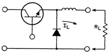
Figure 241. Use of inductance and commutating diode as filter network between pass transistor and load in switching voltage regulator.
