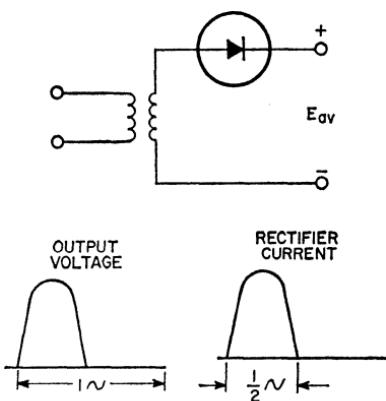
Figure 179. Single-phase half-wave circuit.
