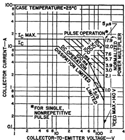
Figure 111. Safe-area rating chart for the 2N3442 silicon power transistor.
