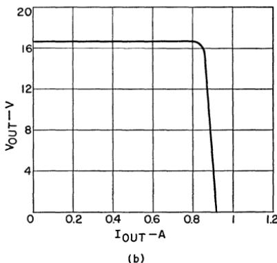
Figure 230. Current-limiting series voltage regulator in which series pass transistor must be capable of withstanding input voltage and short-circuit current simultaneously: (a) schematic diagram; (b) response characteristics.
