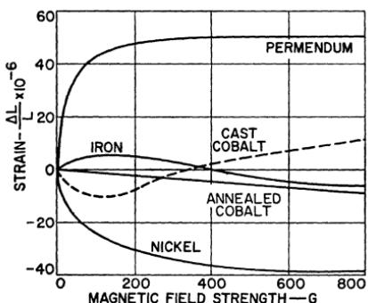
Figure 458. Strain as a function of magnetic field strength for several magnetostrictive materials.
