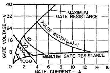
Figure 61. Forward gate characteristics of typical RCA SCR's showing load line for a source of 20 volts and a required gate current of 1 ampere.
