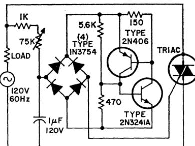
Figure 271. Circuit showing application of two-transistor switch as thyristor triggering device.
