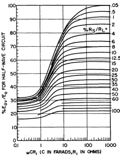
Figure 194. Relationship of applied ac peak voltage to dc output voltage in half-wave capacitor-input circuit.
