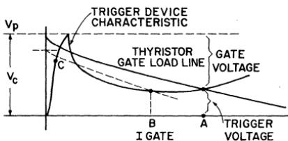
Figure 261. Load line for the circuit shown in Fig. 258.
