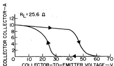
Figure 215. Experimental load line for the 2N3265 transistor using a load impedance of 25.6 ohms and a supply voltage of 28 volts.
