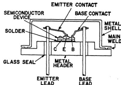
Figure 77. Assembly details for high-power silicon transistor.
