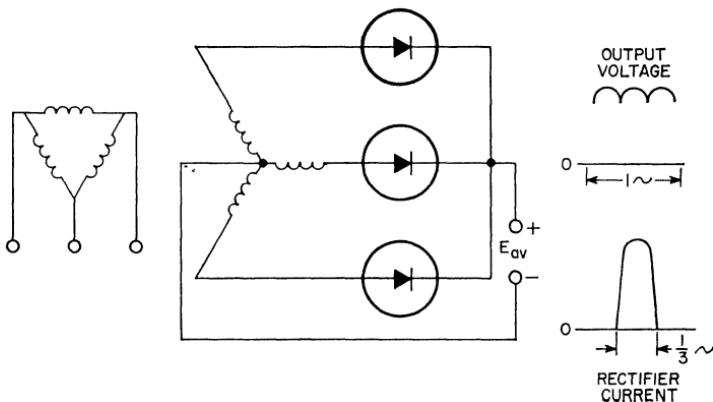
Figure 182. Three-phase "Y" half-wave circuit.
