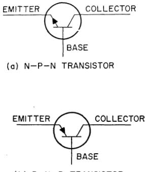
Figure 14. Schematic symbols for transistors.
