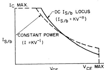
Figure 99. Variation in forward-bias second-breakdown energy level as a function of collector voltage.
