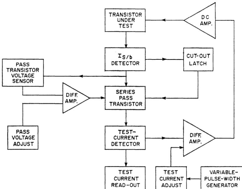
Figure 103. Block diagram of typical  $I_{s/b}$  test set.
