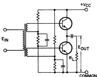
Figure 414. Class AB, push-pull amplifier with series output connection.
