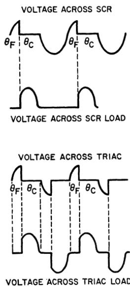
Figure 247. Voltage waveforms showing conduction angle for half-wave operation (SCR) and full-wave operation (triac) of thyristor phase-control circuits.
