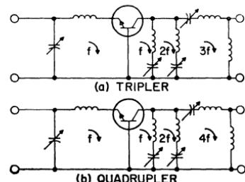
Figure 397. Basic configurations for use of an overlay transistor in a common-base frequency tripler (a) and frequency quadrupler (b).
