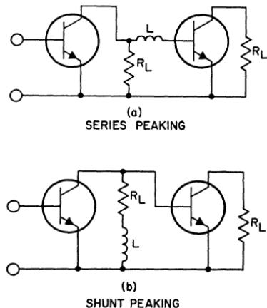
Figure 352. Circuits showing use of peak coils to increase bandwidth: (a) series peaking; (b) shunt peaking.
