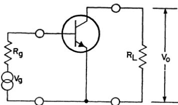
Figure 347. Common-emitter transistor amplifier.
