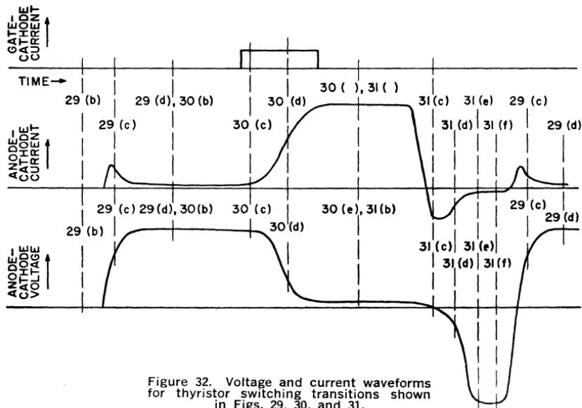
Figure 32. Voltage and current waveforms for thyristor switching transitions shown in Figs. 29, 30, and 31.
