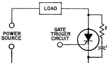
Figure 47. Diagram showing use of RC network to improve the dv/dt capability of an SCR.
