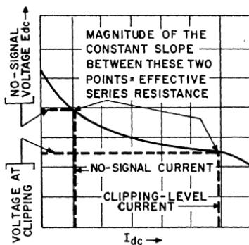
Figure 432. Regulation curve for capacitive power supply.
