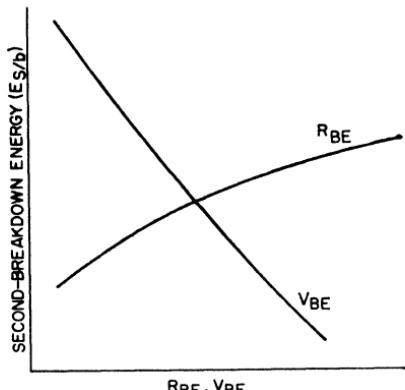
Figure 102. Variation in reverse-bias second-breakdown energy level as a function of  $V_{BE}$  and  $R_{BE}$ .
