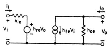
Figure 122. h-parameter equivalent circuit for a transistor used in a common-emitter configuration.
