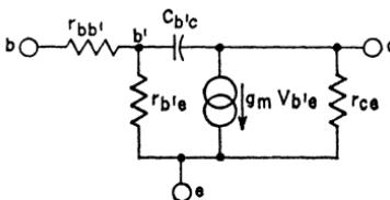
Figure 130. Simplified low-frequency hybrid-pi transistor equivalent circuit.
