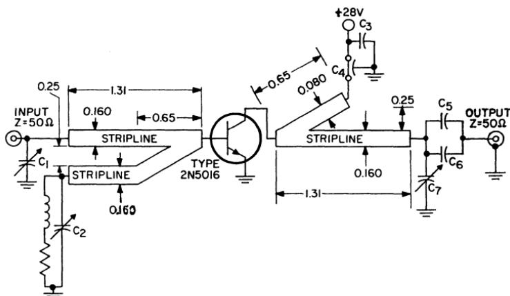
$C_1, C_2, C_7$  = trimmer capacitor, 2 to 18 pF, Amperex HTIOA/218 or equiv.
