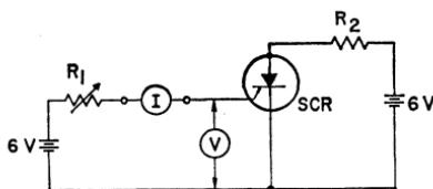
Figure 56. Test circuit used to determine gate-trigger-pulse requirements of thyristors.
