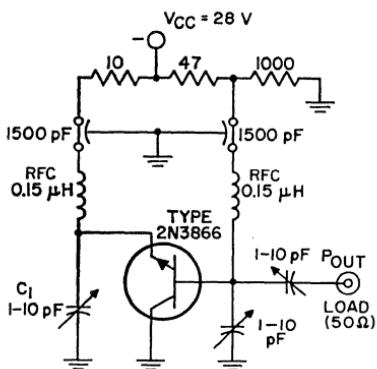
Figure 365. 0.5-watt, 1000-MHz lumped-constant oscillator using the RCA 2N3866 transistor.
