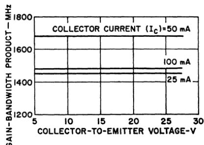
Figure 357. Gain-bandwidth product as a function of collector voltage for a typical RCA-2N5109 Transistor.
