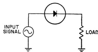
Figure 11. Simple diode rectifying circuit.
