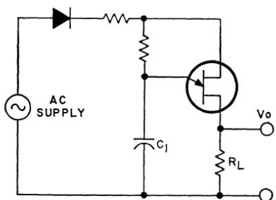
Figure 268. Pulse-triggering circuit that uses a unijunction transistor.
