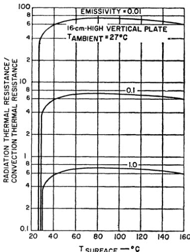
Figure 92. Ratio of radiation thermal resistance to convection thermal resistance as a function of heat-sink surface temperature for various surface emissivities. (Reprinted from *Control Engineering*, October 1967.)
