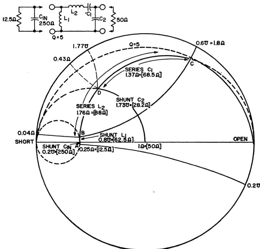
Figure 314. Circuit configuration and network map used to determine component values for matching network that includes four unspecified components.
