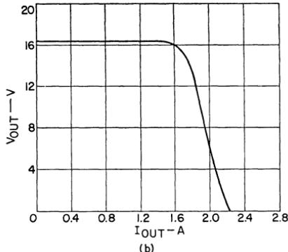
Figure 228. Series voltage regulator using pass transistor as part of current-limiting circuit: (a) schematic diagram; (b) response characteristics (for  $R_4 = 0$ ).
