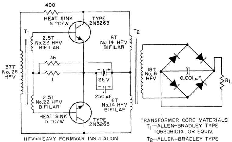
Figure 213. Schematic diagram of 250-watt, 50-kHz push-pull dc-to-dc converter.
