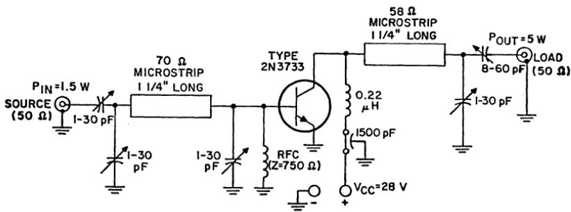
Figure 366. 5-watt, 375-MHz stripline amplifier.
