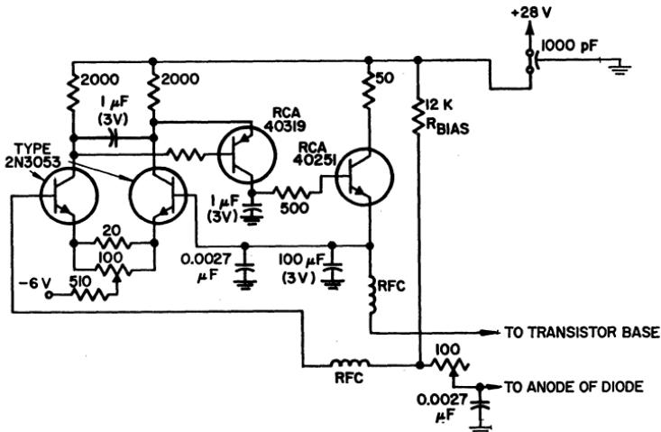
Figure 337. Linear 30-MHz amplifier with temperature-compensating circuit.
