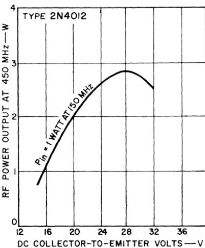
Figure 408. Power output as a function of collector supply voltage for the 150-to-450-MHz frequency tripler.
