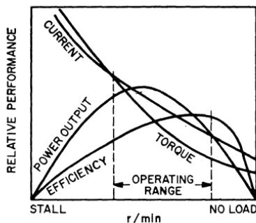
Figure 274. Typical performance curves for a universal motor.
