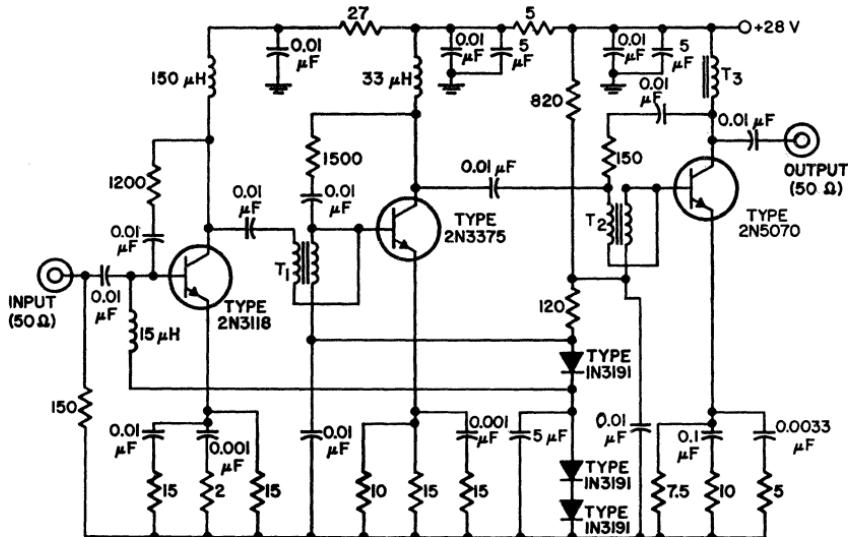
$T_1, T_2 = 18$  turns twisted pair. No. 28 enamel wire on Q<sub>1</sub> CF 102 form       $T_3 = 50$  turns No. 30 enamel wire on CF 102 Q<sub>1</sub> form
