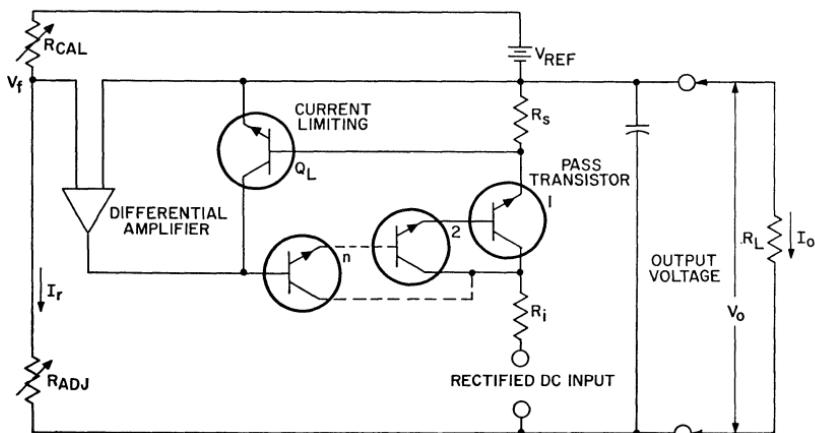
Figure 231. Voltage-regulated current-limited power supply.
