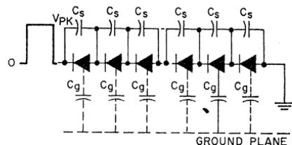
Figure 24. High-voltage rectifier assembly using shunt capacitors ( $C_s$ ) to compensate for stray capacitances ( $C_g$ ) and to equalize the reverse-recovery times of the rectifier units.
