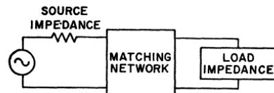
Figure 298. Basic components considered in the design of a matching network.
