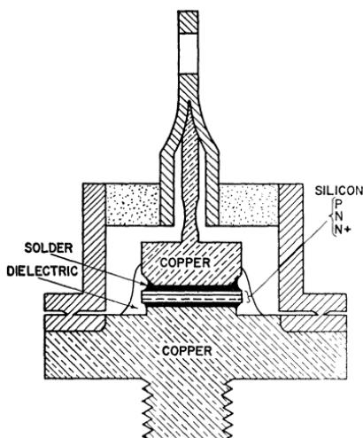
Figure 17. Cross-sectional diagram of a typical silicon rectifier.
