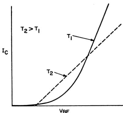
Figure 158. Typical transconductance characteristics for a silicon power transistor at high currents.
