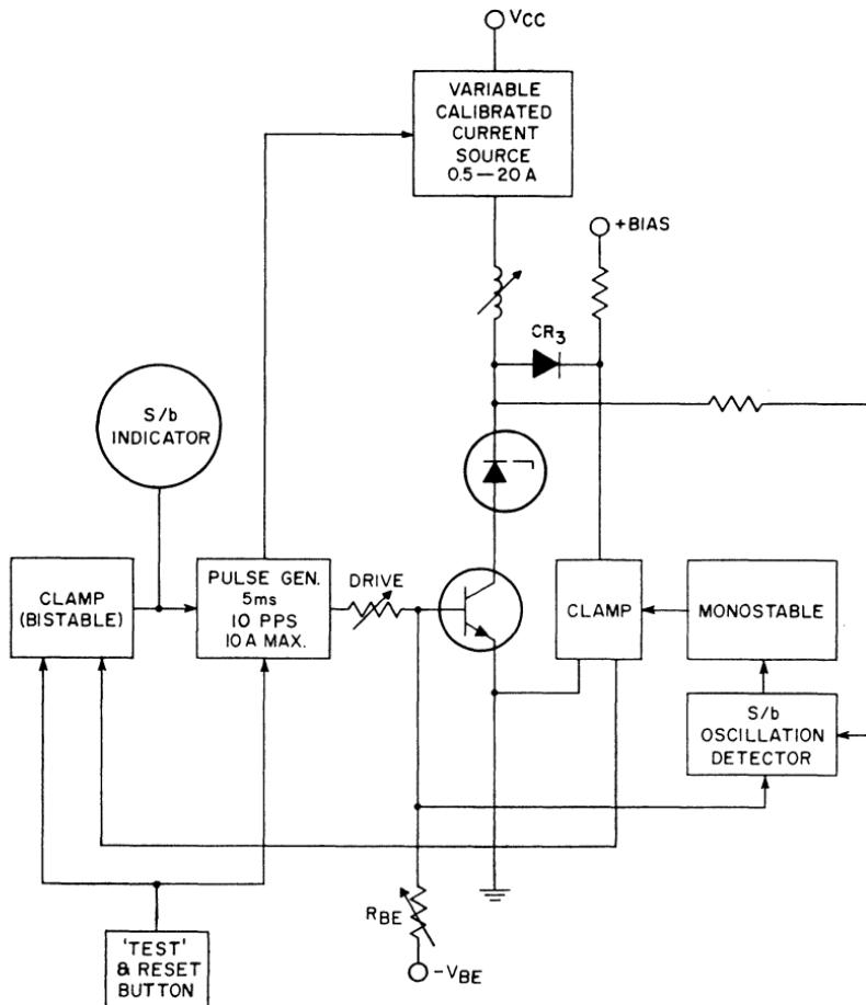
Figure 107. Block diagram of  $E_{S/b}$  test set.
