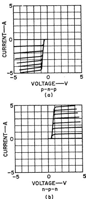
Figure 428. Output characteristics for (a) p-n-p/n-p-n driver-output transistor pair shown in Fig. 426 and for (b) Darlington pair of n-p-n transistors shown in Fig. 427.
