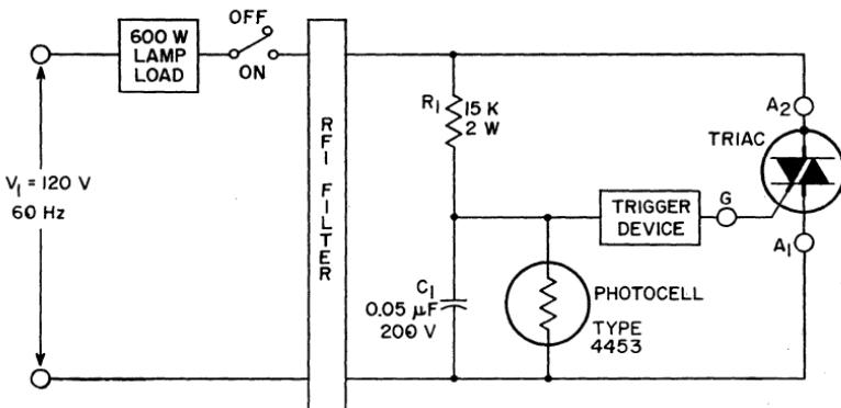
Figure 294. Photocell-operated lamp control circuit that energizes lamp load when photocell is not illuminated.
