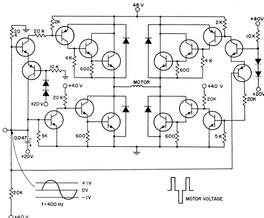
Figure 476. Pulse-width-modulated servo-motor-driver output stage.
