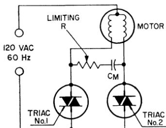
Figure 282. Motor-reversing circuit using two triacs.
