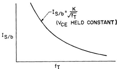
Figure 98. Variation in forward-bias second-breakdown energy level as a function of transistor frequency capability.
