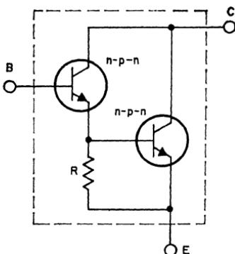
Figure 427. Darlington connection of n-p-n driver transistor to n-p-n output transistor.
