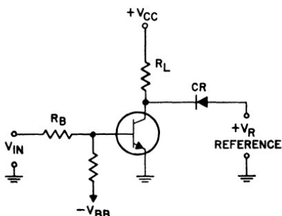
Figure 162. "Collector-catcher" circuit.
