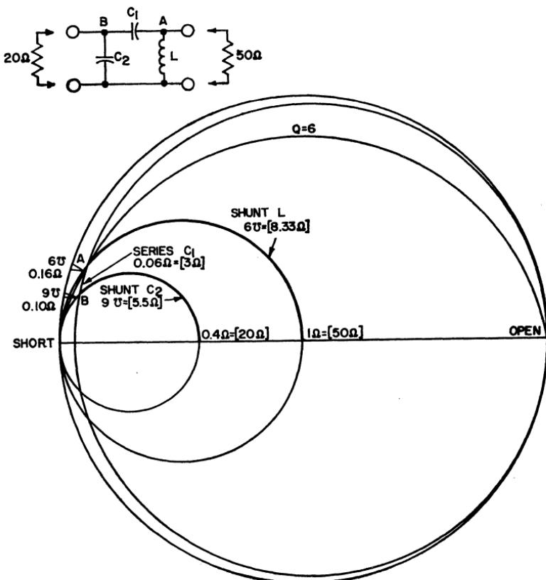
Figure 311. Circuit configuration and network map used to determine the component values for a tapped-C matching network.
