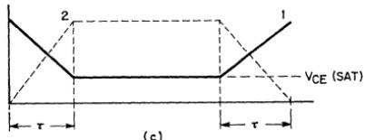
Figure 481. Approximate switching waveforms of the output transistors in the control amplifier shown in Fig. 479.
