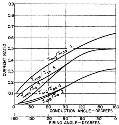
Figure 249. Ratio of SCR current as a function of conduction and firing angles for single-phase half-wave conduction into a resistive load.
