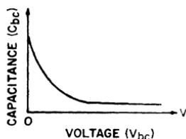
Figure 393. Collector-to-base capacitance  $C_{bc}$  as a function of collector bias in overlay transistors.
