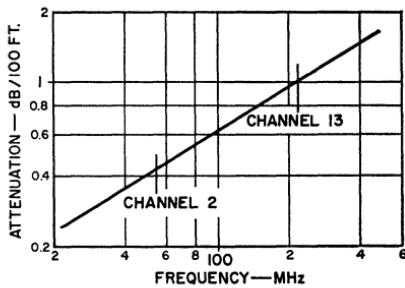
Figure 346. Attenuation characteristics of a coaxial cable as a function of frequency.
