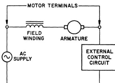
Figure 273. Schematic diagram for a series-wound universal motor.
