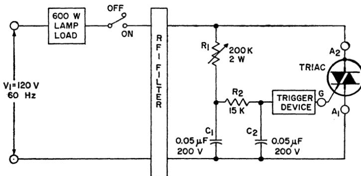
Figure 289. Double-time-constant circuit for brightness control of incandescent lamps in which triac is cut off when potentiometer is set for maximum resistance.
