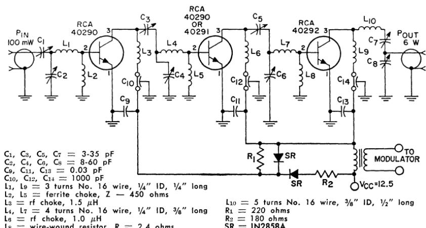
Figure 342. 35-MHz, 6-watt, narrow-band amplitude-modulated transmitter.
