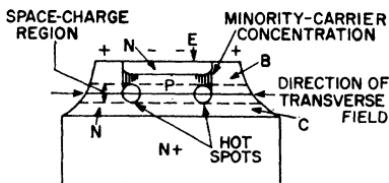
Figure 97. Cross-section of power transistor under forward-bias conditions.
