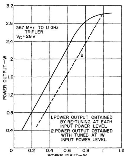
Figure 404. Power output as a function of power input for the 367-MHz-to-1.1-GHz frequency tripler.
