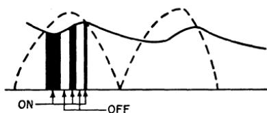
Figure 242. Effect of high-frequency switching of the switching regulator on power-supply ripple component.
