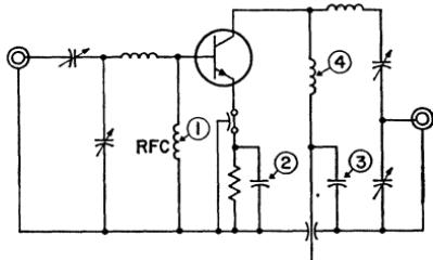
Figure 326. Circuit indicating areas where simple precautions prevent low-frequency oscillations.
