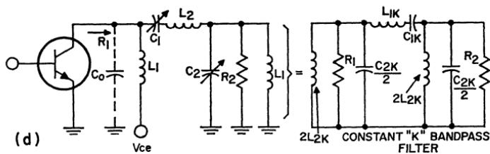
$$(1) (f_2 - f_1) = \frac{1}{2\pi C_0 R_L} \quad (2) L_2 = L_{IK} \frac{R_1}{\pi(f_2 - f_1)} \quad (3) L_1 = 2L_{IK} \frac{(f_2 - f_1)R_1}{2\pi f_1 f_2}$$
