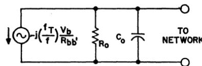
Figure 299. Equivalent circuit for the output of a transistor.
