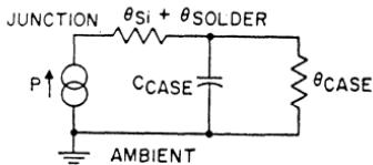
Figure 86. Simplified thermal equivalent circuit for a transistor for  $\theta_{\text{Si}} C_E \ll t < \theta_{\text{case}} C_{\text{case}}$ .
