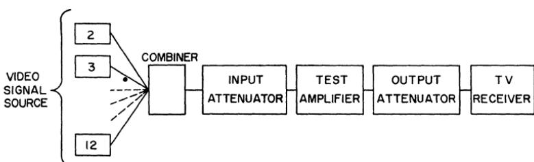
Figure 354. Block diagram of basic test setup used for cross-modulation measurements.
