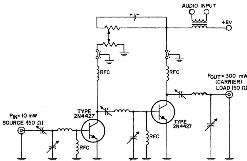
Figure 363. Driver and output stage for a 243-MHz beacon transmitter.
