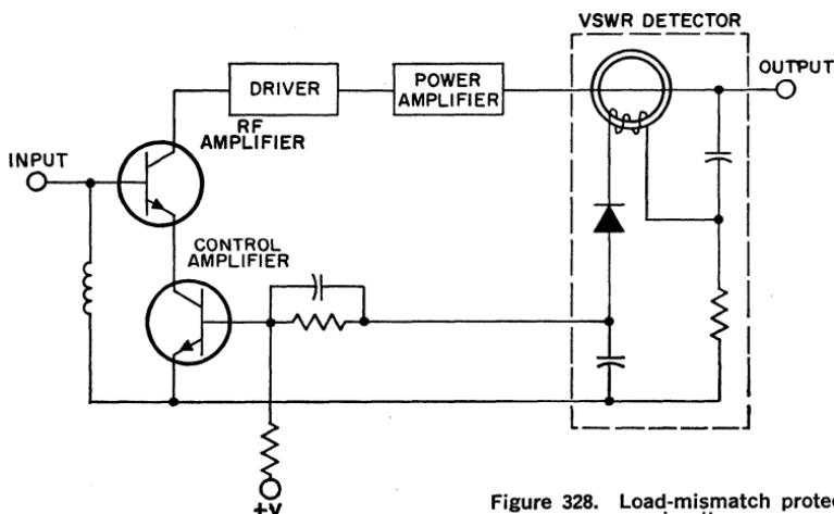
Figure 328. Load-mismatch protection circuit.
