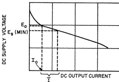
Figure 439. Power-supply regulation curve.
