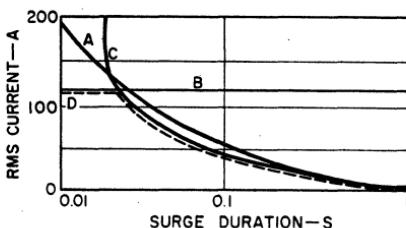
Figure 190. Typical coordination chart for determination of fusing requirements: Curve A—surge rating for 20-ampere rectifier; Curve B—expected surge current in half-wave circuit; Curve C—opening characteristics of protective device; Curve D—resulting surge current in modified circuit.
