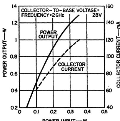
Figure 384. Power output as a function of input for the 2-GHz amplifier shown in Figure 382.
