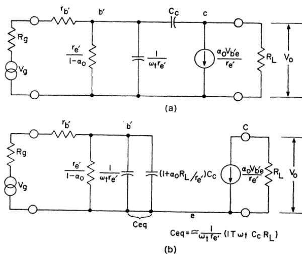
Figure 348. Equivalent circuits for common-emitter amplifier shown in Fig. 347: (a) without parasitic elements; (b) simplified equivalent circuit.
