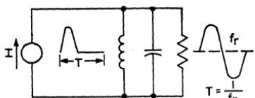
Figure 468. Simplified equivalent circuit for the class C oscillator shown in Fig. 467.
