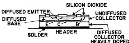
Figure 72. Cross-section of triple-diffused silicon planar power transistor.
