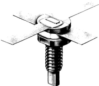
Figure 372. Hermetic Strip-Line Type Ceramic-to-Metal transistor Package (Isolated Electrodes)
