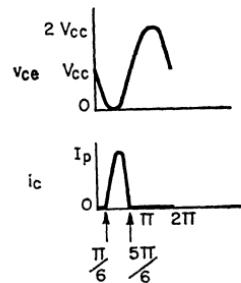
Figure 471. Collector voltage and current waveforms for an oscillator circuit that has a conduction angle of 120 degrees.
