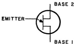
Figure 267. Schematic symbol for a unijunction transistor.
