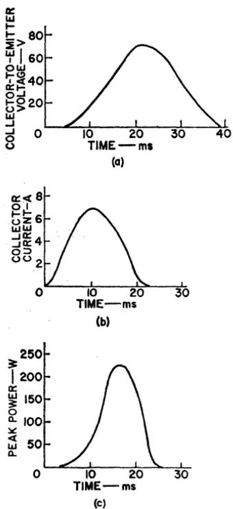
Figure 117. Audio power-amplifier waveforms.
