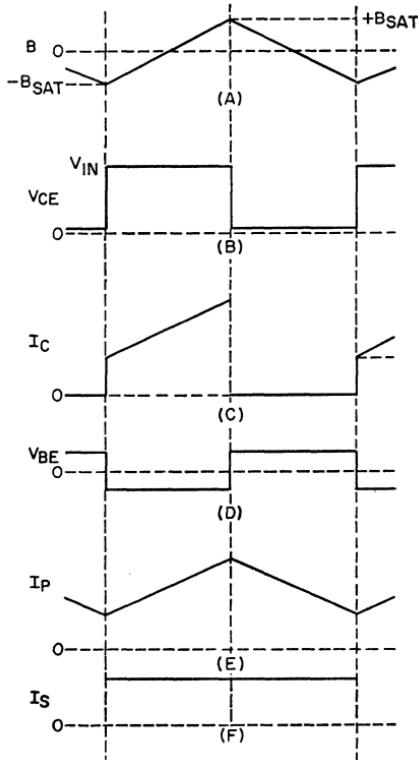
Figure 206. Typical operating waveforms for a two-transistor, one-transformer switching converter: (A) flux density in transformer core; (B) collector voltage of one transistor; (C) collector current of one transistor; (D) base voltage of one transistor; (E) primary current; (F) secondary current.
