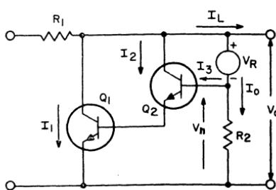
Figure 237. Shunt regulator circuit using two transistors as the shunt pass element.
