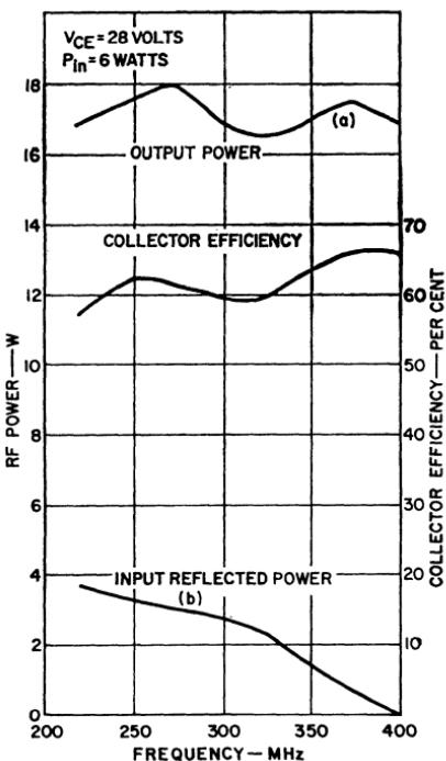
Figure 371. RF power output, input reflected power, and collector efficiency of the RCA 2N5016 transistor as functions of frequency.
