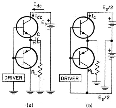
Figure 436. Typical complementary-symmetry circuits.
