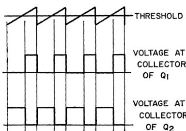
Figure 480. Waveforms showing the threshold switching control for the control amplifier shown in Fig. 479.
