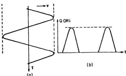
Figure 395. (a) Sinusoidal voltage developed by the amplifier section of an overlay transistor to drive the nonlinear collector-to-base capacitance; (b) distorted charge, or current, waveform produced by the nonlinear collector-to-base capacitance of an overlay transistor in the generation of harmonic power.
