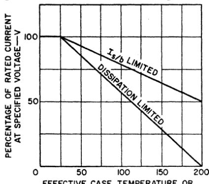
Figure 119. Temperature derating for the RCA 40411 transistor.
