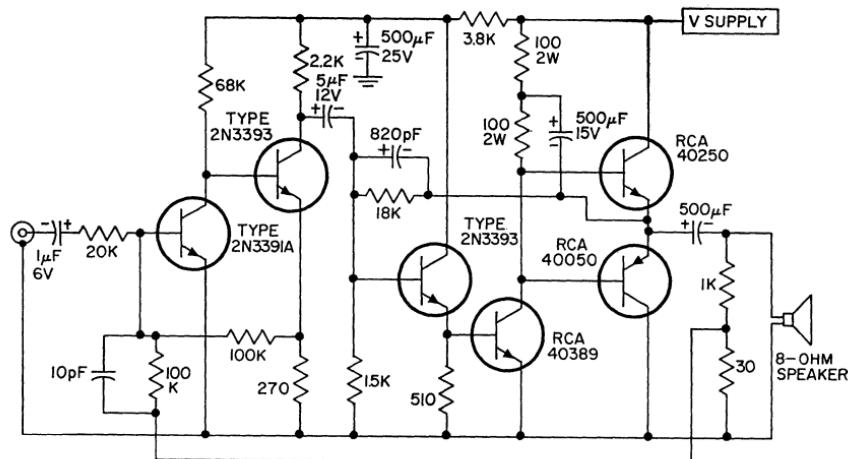
Figure 438. Class B complementary-symmetry power amplifier.
