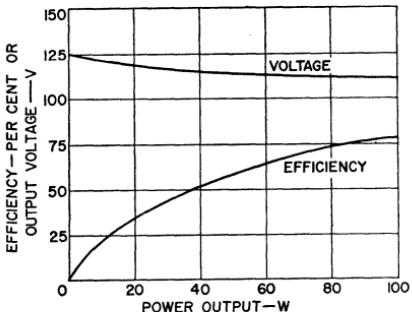
Figure 208. Output voltage and efficiency as a function of power output for the converter circuit shown in Fig. 207.
