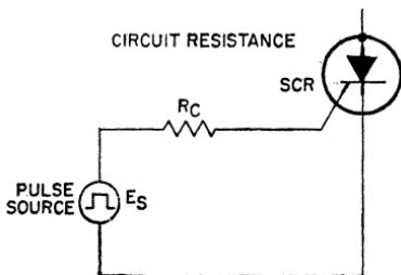
Figure 59. Equivalent diagram of the basic gate-trigger circuit for a thyristor.
