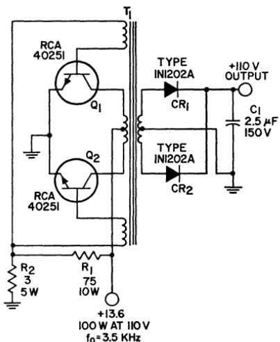
Figure 207. Schematic diagram of 13.6-to-110-volt transformer-coupled push-pull converter.
