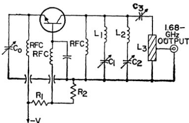
Figure 410. Oscillator-quadrupler circuit.
