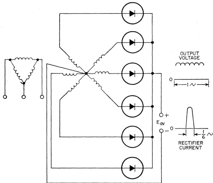
Figure 184. Six-phase "star" circuit.
