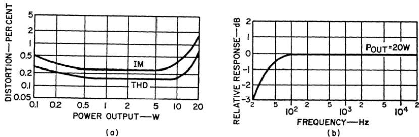
Figure 450. Performance characteristics for the 20-watt complementary-symmetry amplifier: (a) distortion as a function of power output; (b) relative response as a function of frequency. (Universal complementary-symmetry design.)
