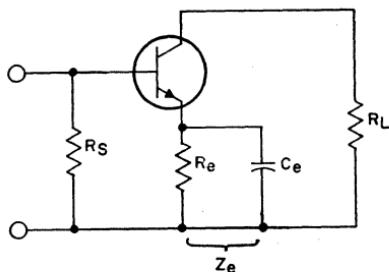
Figure 350. Transistor amplifier that uses emitter degeneration to increase circuit bandwidth.
