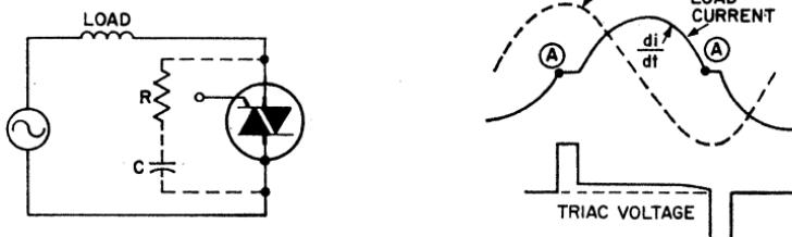
Figure 65. Simplified diagram and voltage and current waveforms for operation of a triac in a circuit that has an inductive load and a lagging-current power factor.
