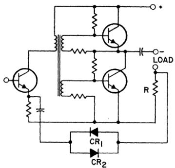
Figure 445. Push-pull power amplifier with short-circuit protection.
