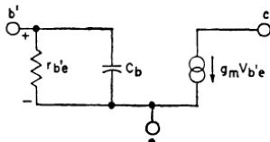
Figure 126. Elementary small-signal transistor equivalent circuit.
