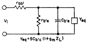
Figure 137. General equivalent input circuit for a common-emitter amplifier.
