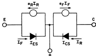
Figure 151. Ebers-Moll model of a p-n-p transistor controlled by diode currents.
