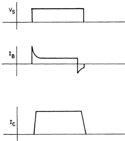
Figure 166. Waveforms for circuit shown in Fig. 165: (a) source voltage  $V_s$ ; (b) base current  $I_B$ ; (c) collector current  $I_C$ .
