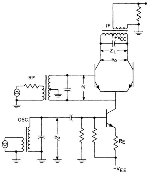
Fig. 186 — Circuit diagram of a CA3005 or CA3006 balanced mixer (operating mode D). The equations for product detection or multiplication are based on this circuit.
