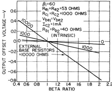
Fig. 31 — Output offset voltage as a function of the beta ratio of the differential pair of transistors for several values of external base resistors.
