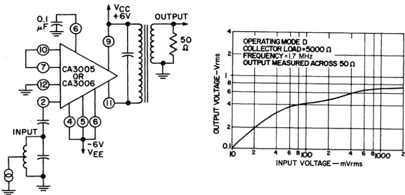
Fig. 171 — Limiting characteristics and circuit diagram of a CA3005 or CA3006 cascode limiter having a 5000-ohm collector load impedance.
