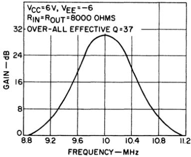
Fig. 87 — Schematic diagram and response curves for 10-MHz tuned-input, tuned-output narrow-band amplifier using CA3000.
