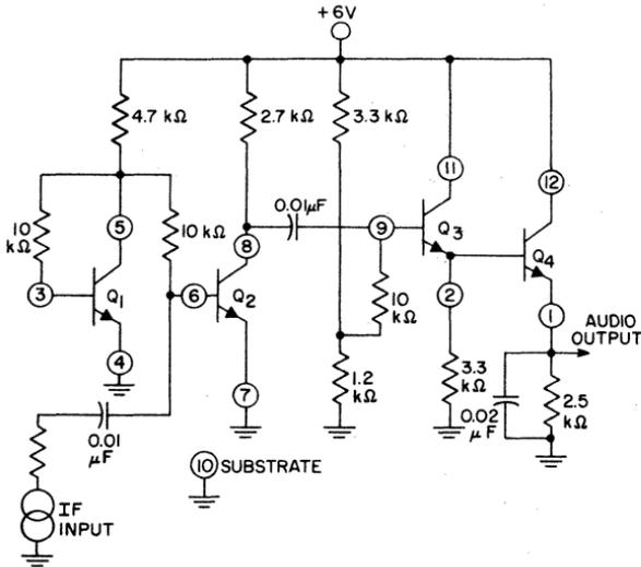
Fig. 303 — Schematic diagram for a CA3018 final if amplifier and second detector.
