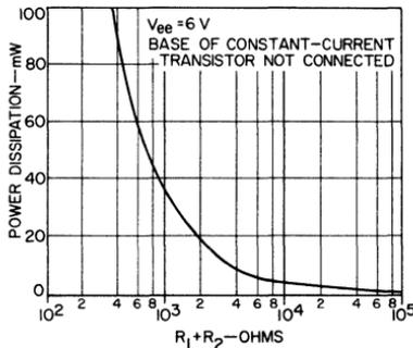
Fig. 56 — Power dissipation in the bias network of the current-sink transistors as a function of the sum of base-bias resistors  $R_1$  and  $R_2$ .
