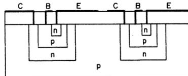
Fig. 4 — Addition of metallized contacts to transistor elements.
