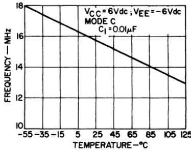
Fig. 97 — High-frequency 3-dB bandwidth of the CA3001 as a function of temperature.
