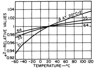
Fig. 47 — Relative values of the square of the alpha for the current-sink transistor as a function of temperature for several beta values.
