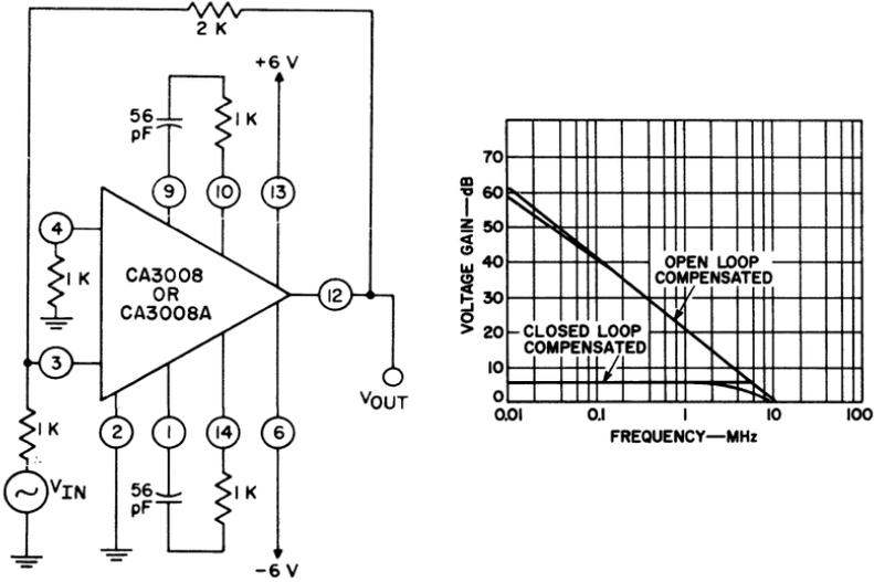
Fig. 217 — Circuit diagram and closed-loop response of an inverting type of operational amplifier used as a 6-dB video amplifier.
