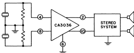
Fig. 308—Block Diagram of Stereo System using CA3036 as Phono Preamplifier.
