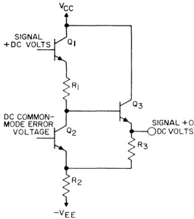
Fig. 9 — Output circuit used in linear integrated circuits to compensate for a shift in dc voltage level between output and input.
