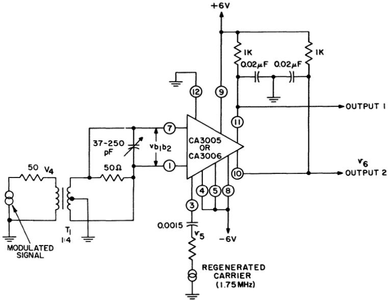
Fig. 194 — Product detector using the CA3005 or CA3006.
