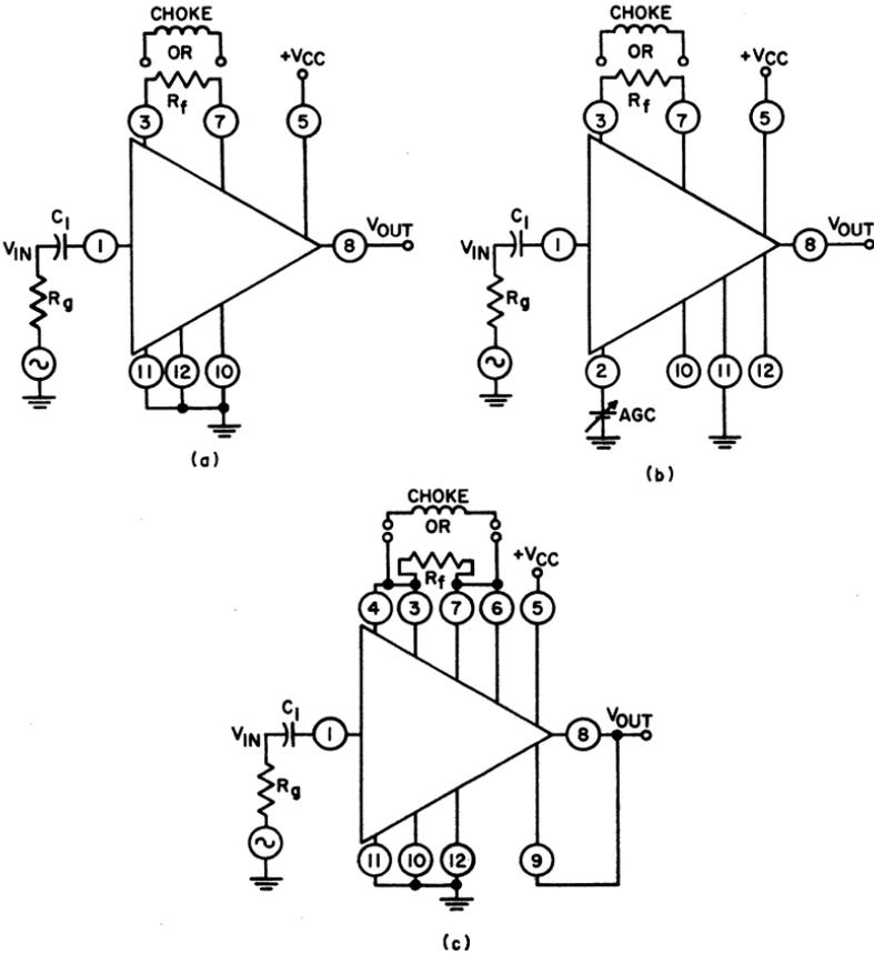
Fig. 120 — Typical connections for the CA3021, CA3022, and CA3023 for (a) wide-band and band-pass applications, (b) wide-band and band-pass applications that require agc, and (c) limiter applications.
