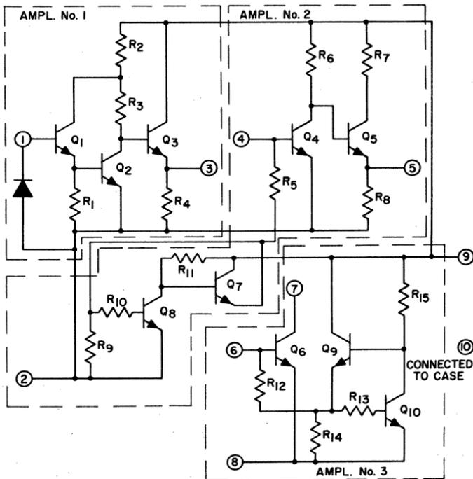
Fig. 280 — Schematic diagram of the CA3035 or CA3035V1 integrated-circuit wide-band amplifier array.
