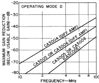
Fig 161 — Maximum gain control provided by variations in the current through transistor  $Q_3$  as a function of frequency.
