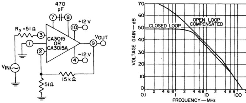
Fig. 231 — Circuit diagram and response for a 50-dB noninverting operational amplifier with phase-lead compensation.
