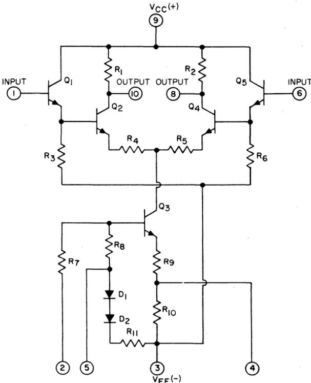
Fig. 71 — Schematic diagram of the CA3000 integrated-circuit dc amplifier.
