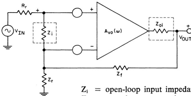
$Z_i$  = open-loop input impedance
