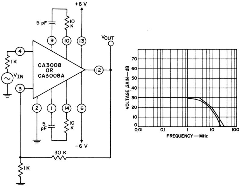
Fig. 214—Circuit diagram and closed-loop response of a noninverting type of operational amplifier used as a 30-dB video amplifier.
