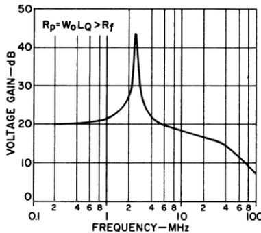
Fig. 128 — Voltage gain as a function of frequency in a band-pass amplifier when the tuned-circuit resonant impedance  $R_p$  is higher than the cancellation resistance  $R_{fc}$ .
