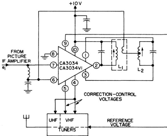
Fig. 279 — Block diagram of a typical afc application of the CA3034 or CA3034V1 in a color television receiver.
