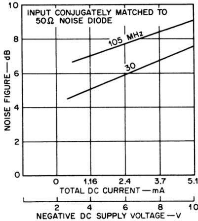
Fig. 154 — Representative noise performance of the CA3004, CA3005, or CA3006 operated in a differential-amplifier configuration (operating mode D).
