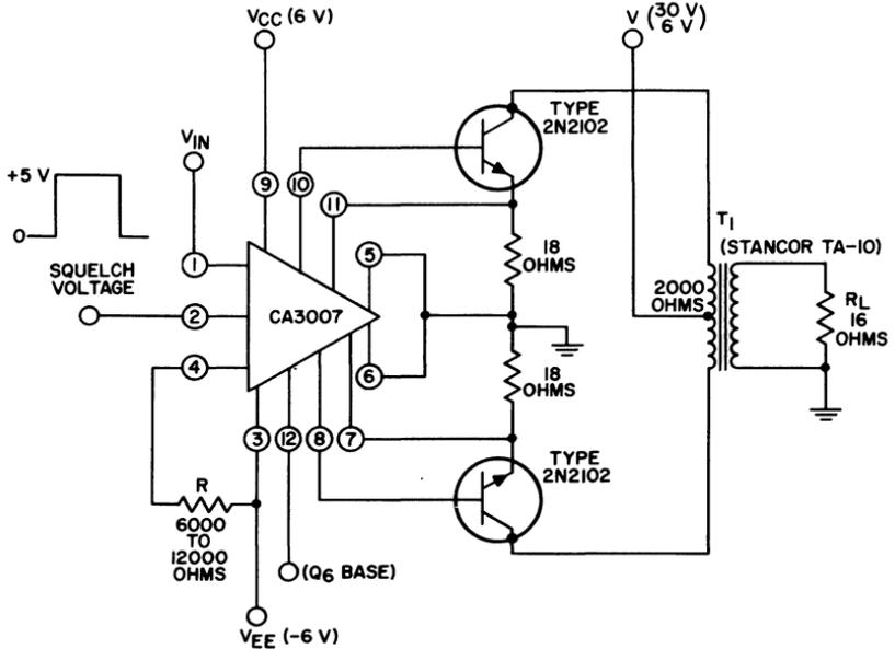
Fig. 90 — CA3007 used as an audio driver for a direct-coupled 300-milliwatt audio amplifier.
