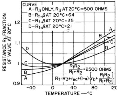
Fig. 38 — Resistance ratio  $R_t$  as a function of temperature for several values of the beta of the current-sink transistor.
