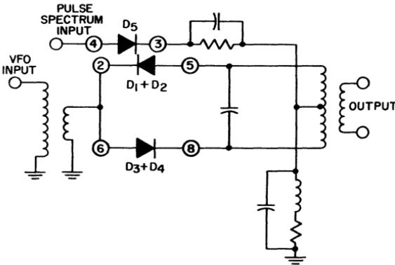
Fig. 285 — Typical synthesizer mixer circuit using the CA3019.
