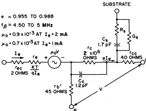
Fig. 50 — Equivalent-circuit model of an integrated-circuit transistor.
