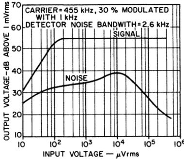
Fig. 135 — Schematic diagram and performance curves for 455-kHz amplifier using two CA3021 circuits.
