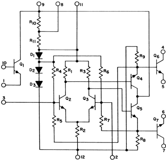
Fig. 237 — Schematic diagram of the CA3020 integrated-circuit multipurpose wide-band amplifier.
