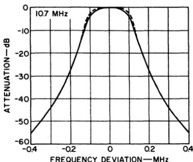
Fig. 272 — Selectivity curve for if-amplifier strip of Fig. 269.
