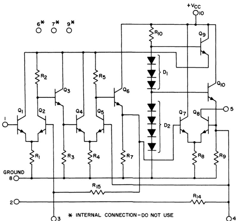
Fig. 253 — Schematic diagram of the CA3011 or CA3012 integrated-circuit wide-band amplifier.
