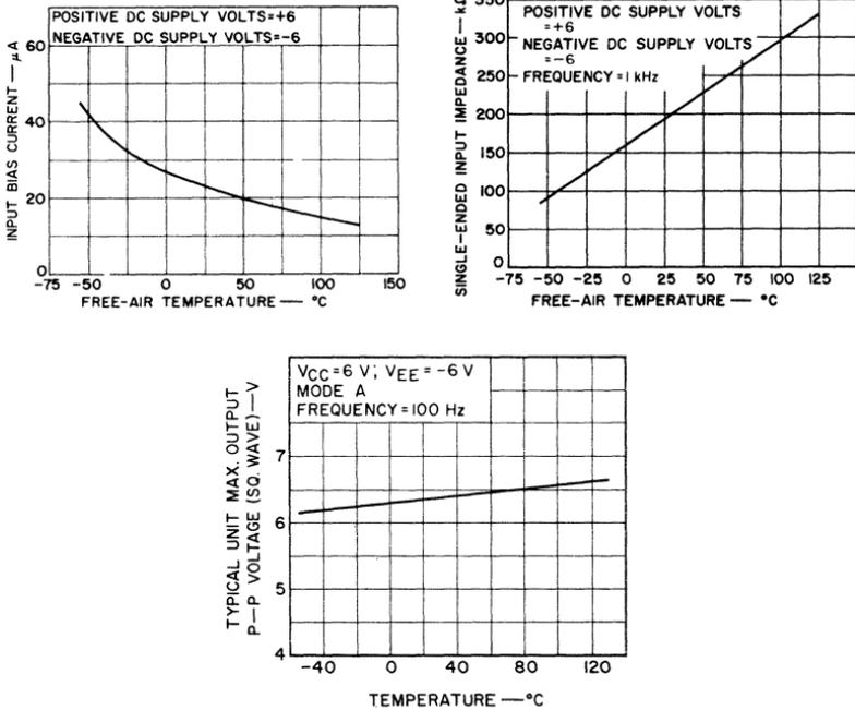
Fig. 82 — Input bias current, input impedance, and dynamic output voltage of CA3000 as functions of temperature.
