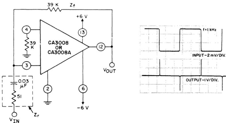
Fig. 223 — Circuit diagram and the input and output waveforms for an operational amplifier used as a differentiator.
