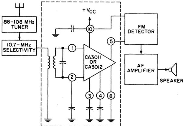
Fig. 263 — Block diagram of typical FM receiver using CA3011 or CA3012 integrated-circuit wide-band amplifier.
