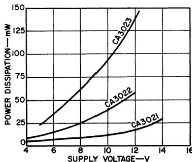
Fig. 121 — Power dissipation as a function of supply voltage for the CA3021, CA3022, and CA3023.
