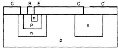
Fig. 6 — Use of oxide as a dielectric to form integrated capacitor.
