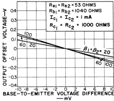
Fig. 36 — Output offset voltage as a function of the difference in the base-to-emitter voltages of the differential pair of transistors for several beta values.
