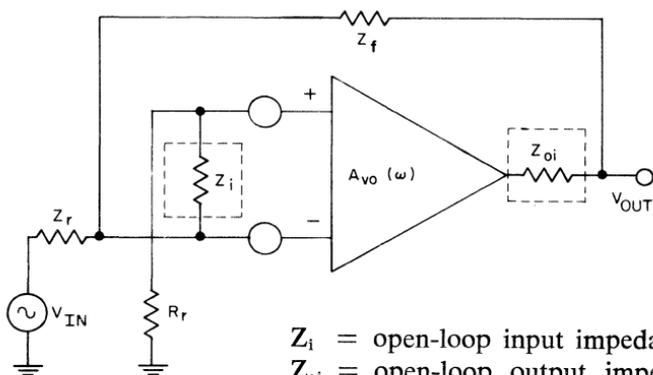
$Z_i$  = open-loop input impedance
