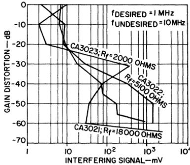
Fig. 130 — Cross-modulation distortion characteristics of the CA3021, CA3022, and CA3023.
