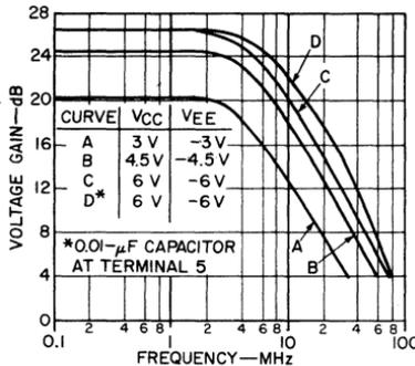
Fig. 110 — Effective single-state response characteristics for CA3002 if amplifier using 0.01-microfarad coupling capacitors. Curve D represents operation with 0.01-microfarad bypass capacitor connected at terminal 5 (not shown).
