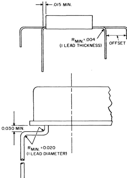
Fig. 19 — Lead-forming requirements for RCA integrated-circuit packages.
