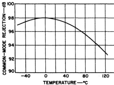
Fig. 80 — Common-mode rejection of CA3000 as a function of frequency and of temperature in test circuit shown.
