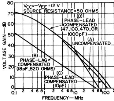
Fig. 229 — Open-loop gain as a function of frequency for compensated and uncompensated operational amplifiers.
