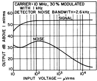
Fig. 134 — Schematic diagram and performance curves for 10-MHz if amplifier using two CA3023 circuits.
