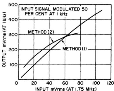
Fig. 116 — Input-output characteristics of the envelope detectors shown in Fig. 115.
