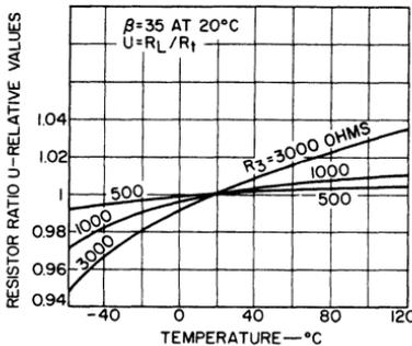
Fig. 48 — Resistor ratio  $U$  as a function of temperature for several values of the emitter resistor ( $R_3$ ) of the current-sink transistor.
