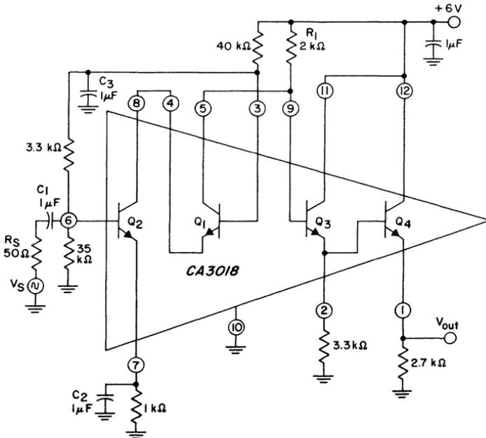
Fig. 299 — Schematic diagram for a CA3018 cascode video amplifier.
