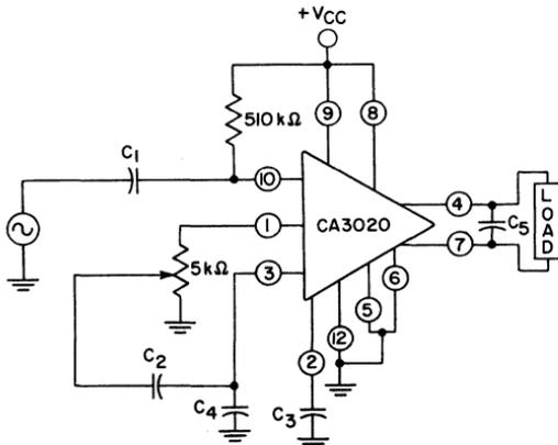
Fig. 245 — Methods of restricting the bandwidth of the CA3020.
