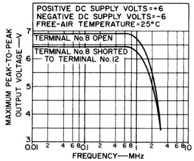
Fig. 206 — Output-swing capabilities as a function of frequency.
