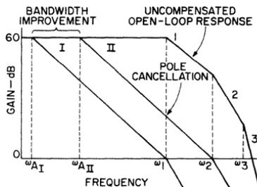
I—Compensated open-loop response using simple depression of higher corner frequencies.
