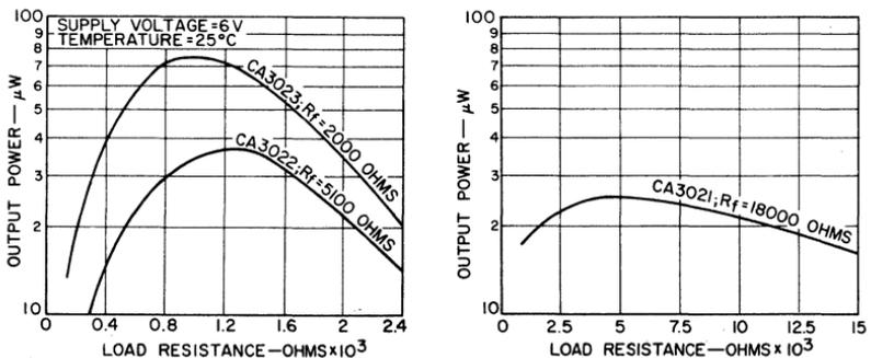
Fig. 126 — Maximum linear signal output of the CA3021, CA3022, and CA3023 as a function of load resistance.
