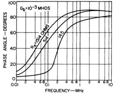
Fig. 54 — Output-impedance phase angle of the current-sink transistor as a function of frequency for several values of base-termination conductance.
