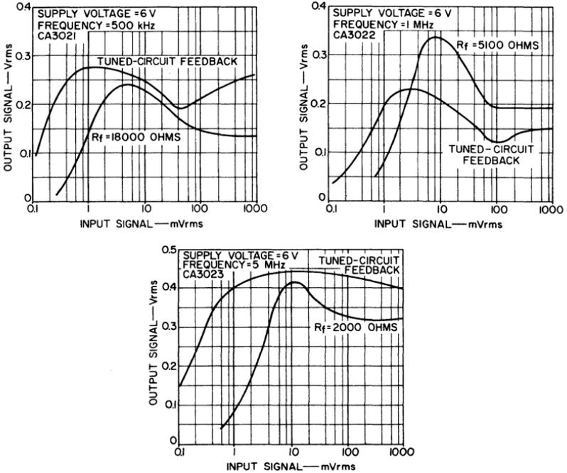
Fig. 133 — Limiting characteristics of the CA3021, CA3022, and CA3023.
