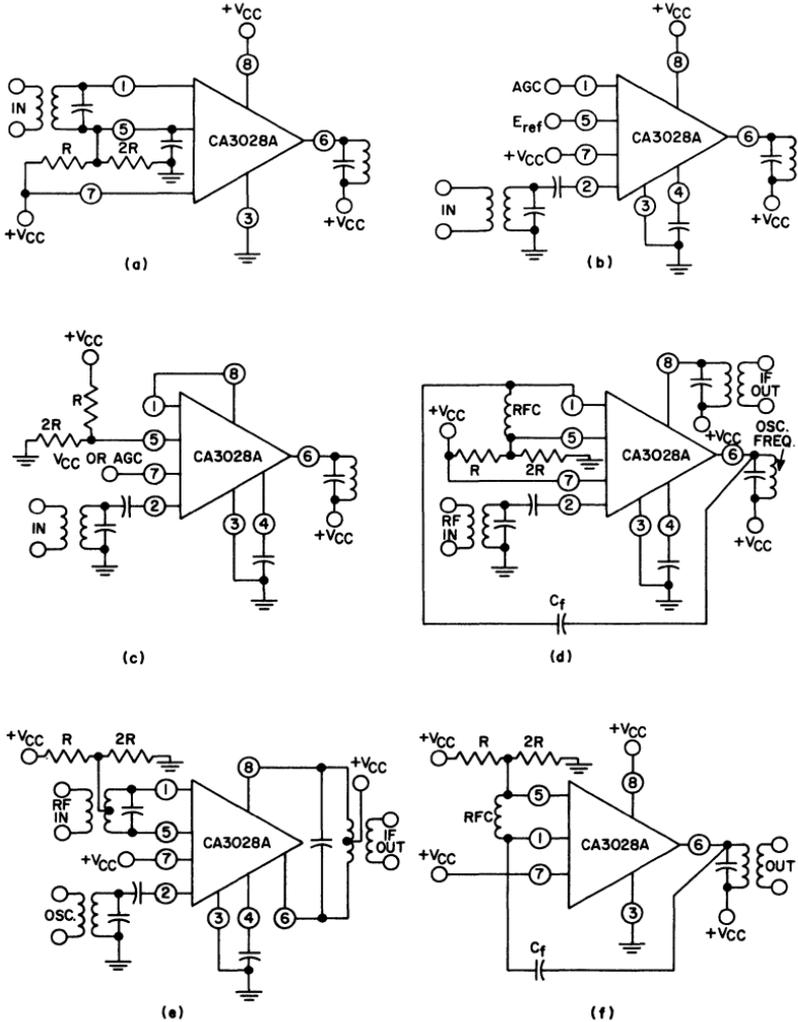
Fig. 142 — Connections for the CA3028A for use as (a) a balanced differential amplifier with a controlled constant-current-source drive and agc capability, (b) a cascode amplifier with a constant-impedance agc capability, (c) a cascode amplifier with conventional agc capability, (d) a converter, (e) a mixer, and (f) an oscillator.
