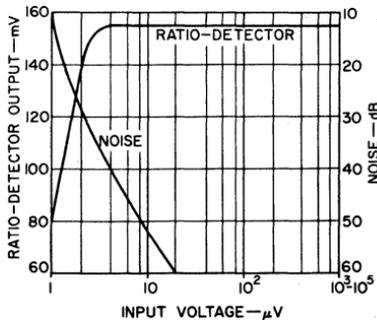
Fig. 271 — Performance curves for if-amplifier strip of Fig. 269.
