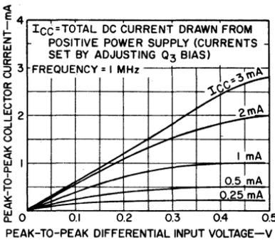
Fig. 139 — Dynamic transfer and limiting characteristics of the CA3004.
