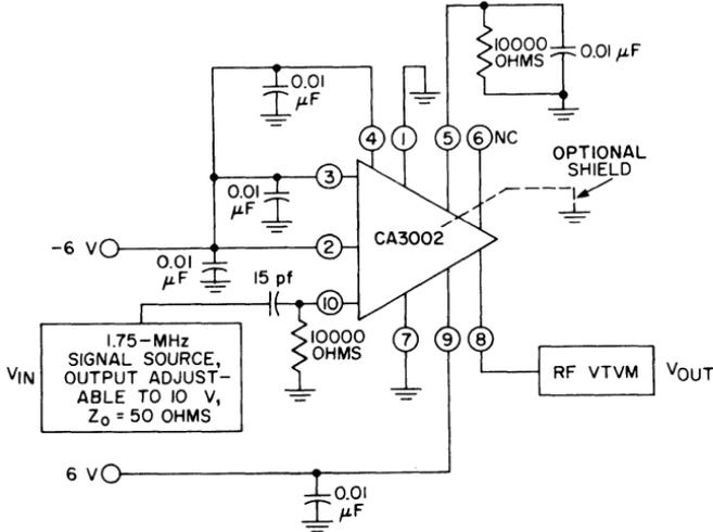
Fig. 109 — Voltage-gain test circuit.
