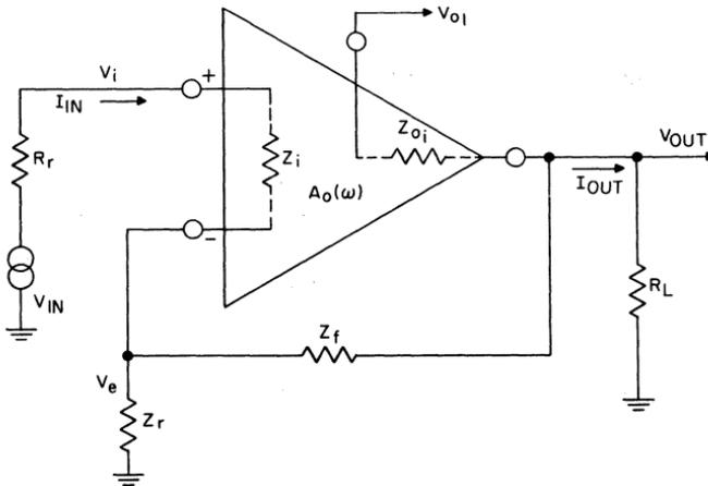
Fig. 59 — Noninverting-feedback operational-amplifier configuration.
