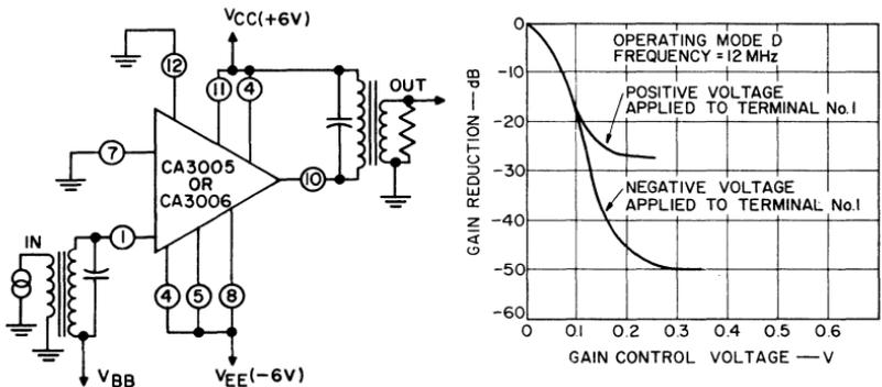
Fig. 160 — Gain control characteristics of the CA3005 or CA3006 as a function of the dc offset voltage V<sub>BB</sub> applied to the differential pair of transistors Q<sub>1</sub> and Q<sub>2</sub>.
