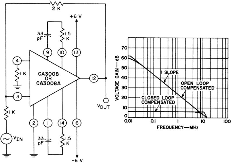
Fig. 218 — Effect of a decrease in phase-compensating capacitance from 56 picofarads to 33 picofarads on the response of the 6-dB video amplifier.
