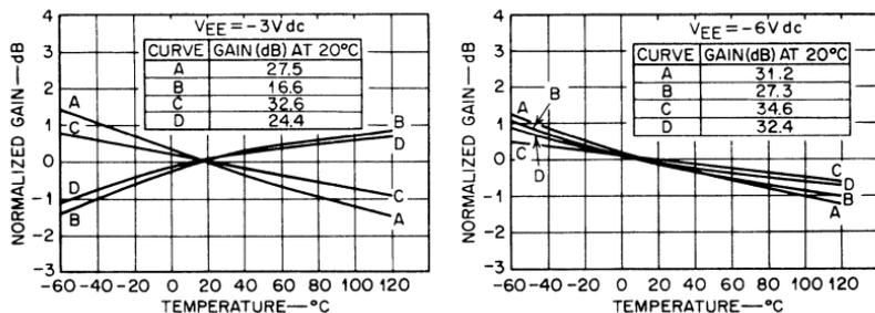
Fig. 75 — Theoretical curves of gain as a function of temperature for negative-supply voltages of  $-3$  and  $-6$  volts (calculated for  $\beta = 35$  at  $20^\circ\text{C}$ ).
