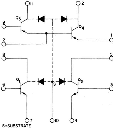
Fig. 296 — Schematic diagram for the CA3018 integrated-circuit transistor array.
