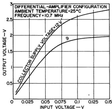
Fig. 168 — Limiting characteristics of the CA3028A operated in a differential-amplifier configuration.
