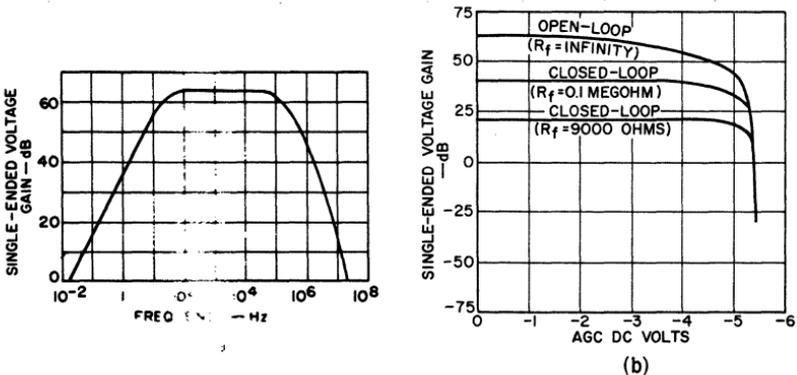
Fig. 86 — Gain frequency (a) and agc (b) characteristics of feedback amplifier shown in Fig. 85.
