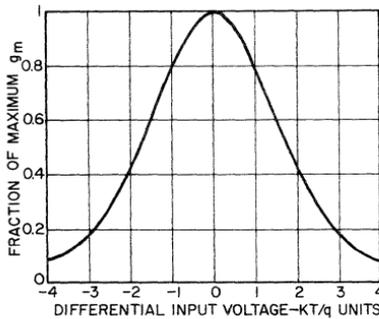
Fig. 22 — Transconductance of the basic differential amplifier as a function of the differential input voltage.
