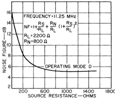
Fig. 156 — Noise figure of the CA3005 or CA3006 in a differential-amplifier configuration as a function of source resistance (operating mode D).
