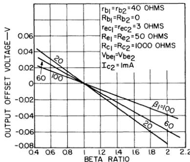
Fig. 30 — Effect of absolute values and ratios of the betas of the differential pair of transistors on the output offset voltage.
