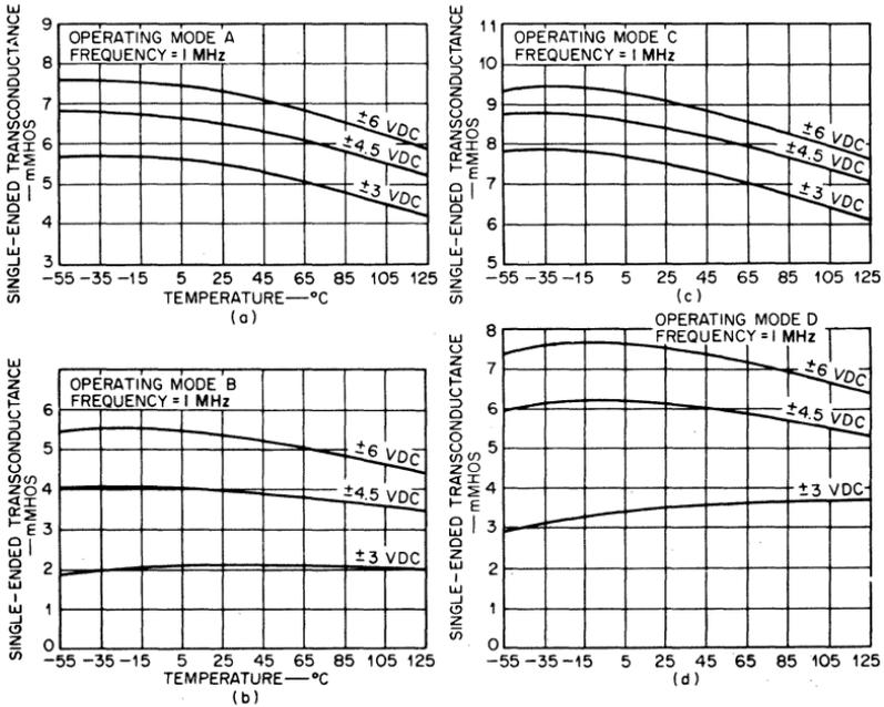
Fig. 144 — Single-ended transconductance of the CA3004 as a function of temperature for each operating mode.
