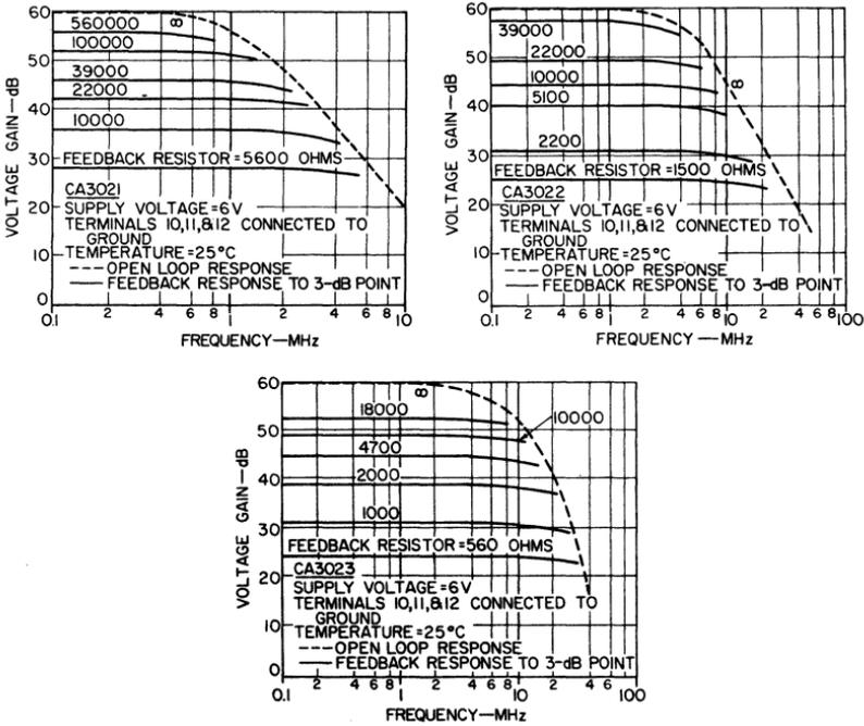
Fig. 123 — Frequency-response characteristics of the CA3021, CA3022, and CA3023.
