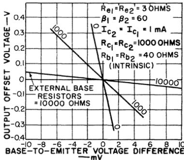
Fig. 33 — Output offset voltage as a function of the difference in the base-to-emitter voltage of the differential pair of transistors for several values of external base resistors.
