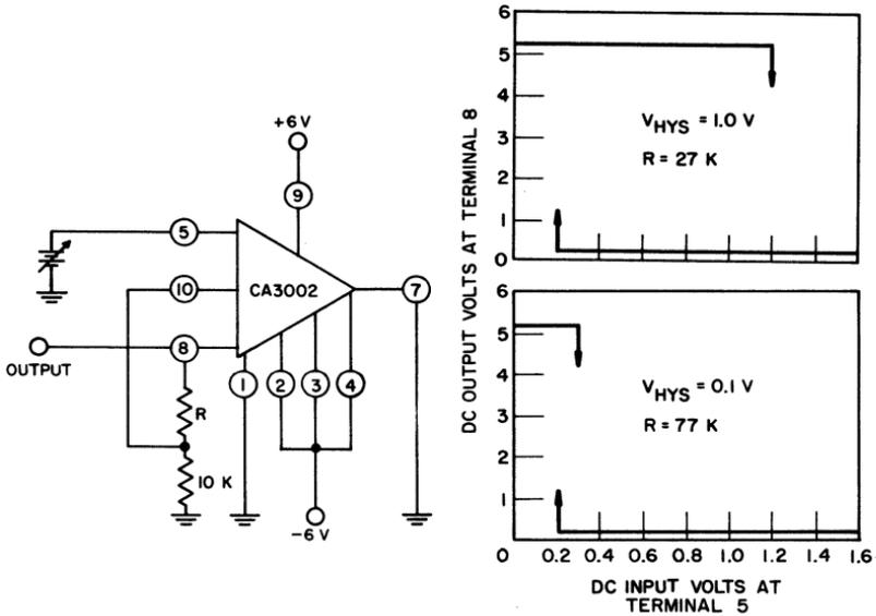
Fig. 118 — Schmitt trigger circuit using the CA3002 and the output swing and associated hysteresis for the circuit.
