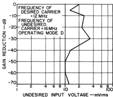
Fig. 167 — Gain control of the CA3005 or CA3006 in a cascode configuration as a function of an undesired-carrier voltage that produces cross-modulation distortion of 10 per cent when gain control is provided by a negative bias voltage applied to the base of transistor  $Q_1$ .
