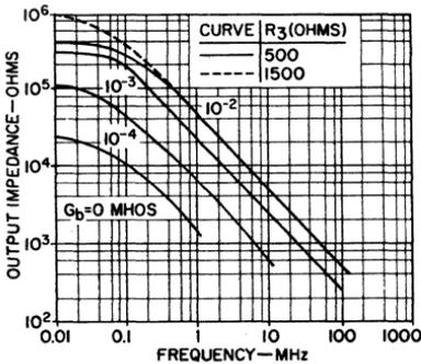
Fig. 52 — Absolute value of output impedance of the current-sink transistor as a function of frequency for several values of the base-termination conductance.
