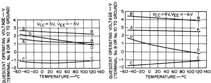
Fig. 74 — Measured curves of dc output voltage as a function of temperature for negative-supply voltages of  $-3$  and  $-6$  volts.
