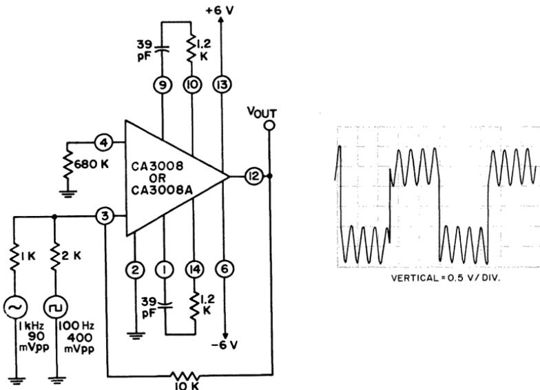
Fig. 224 — Circuit diagram and output waveform for an operational amplifier used as a scaling adder.
