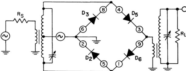
Fig. 294 — Balanced mixer with half-wave carrier switch using the CA3019.
