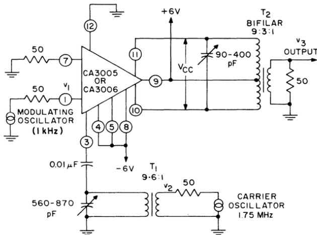
Fig. 193 — Double-sideband, suppressed-carrier modulator using the CA3005 or CA3006.
