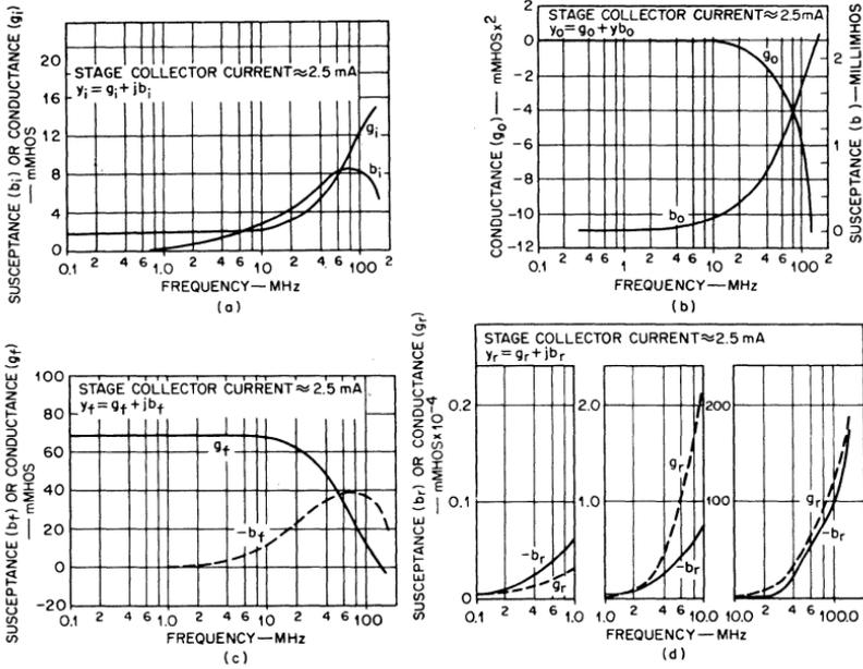
Fig. 151 — Admittance parameters of a CA3005 or CA3006 cascode amplifier as a function of frequency.
