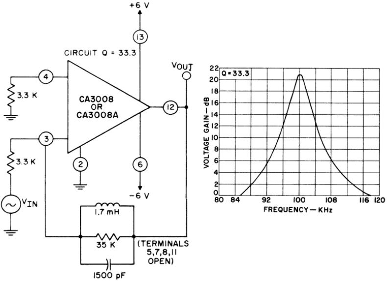
Fig. 221 — Circuit diagram and response of an inverting type of operational amplifier used as a narrow-band 100-kHz tuned amplifier.
