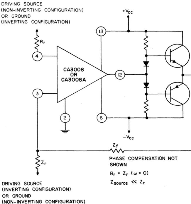
Fig. 209 — Schematic diagram showing addition of an external push-pull output stage to increase the output capability of an operational amplifier.
