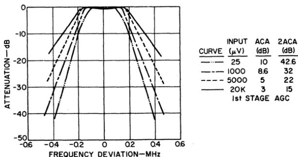
Fig. 276 — Selectivity curves for discrete-component if-amplifier strip using six double-tuned filters.
