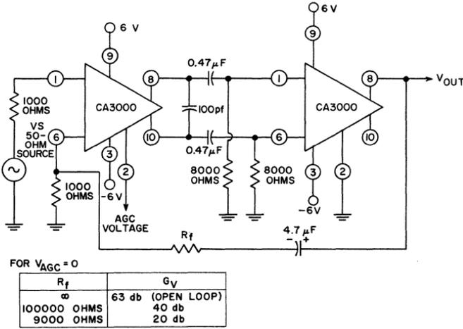
Fig. 85 — Cascaded RC-coupled feedback amplifier using two CA3000 circuits.
