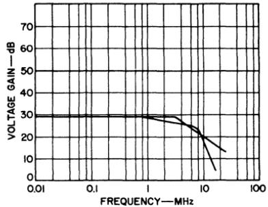
Fig. 216 — Circuit diagram and gain-frequency response of the 30-dB video amplifier when phase compensation is accomplished by addition of a capacitor in parallel with the feedback resistor.
