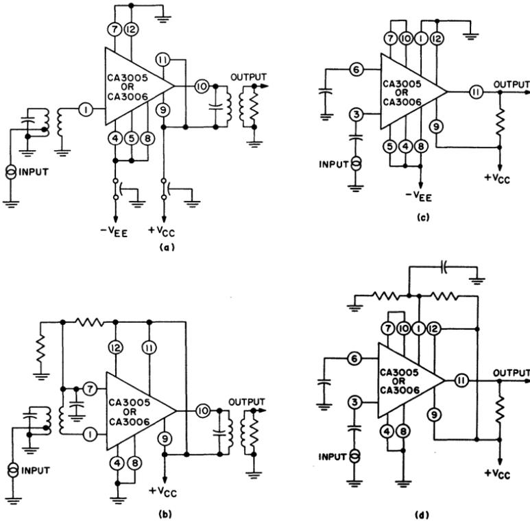
Fig. 141 — Supply-voltage connections for the CA3005 or CA3006 in (a) a differential-amplifier configuration operated from dual supplies, (b) a differential-amplifier configuration operated from a single supply, (c) a cascode configuration operated from dual supplies, and (d) a cascode configuration operation from a single supply.
