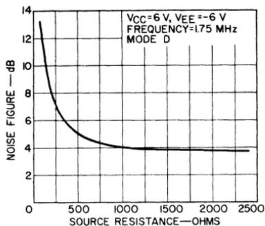
Fig. 114 — Noise figure of the CA3002 as a function of source resistance.
