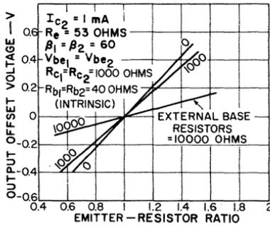
Fig. 32 — Output offset voltage as a function of the emitter-resistor ratio of the differential pair of transistors for several values of external base resistors.
