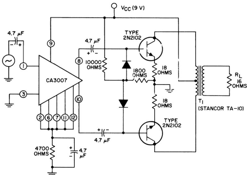
Fig. 91 — CA3007 used as an audio driver for a 30-milliwatt audio amplifier.
