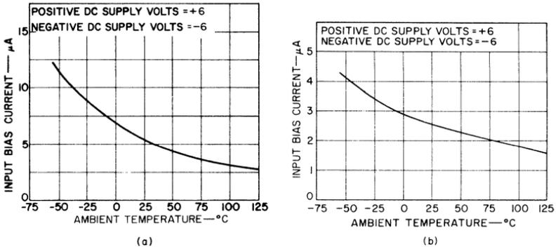
Fig. 199 — Input bias current as a function of temperature: (a) for CA3008; (b) for CA3008A.
