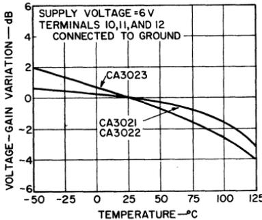
Fig. 124 — Voltage-gain variation with temperature for the CA3021, CA3022, and CA3023 (feedback adjusted to provide gain of approximately 40 dB at 25°C).
