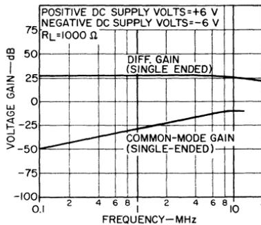
Fig. 157 — Single-ended common-mode and differential gains of the CA3004, CA3005, or CA3006 as a function of frequency.
