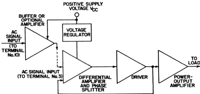
Fig. 238 — Functional block diagram of the CA3020.
