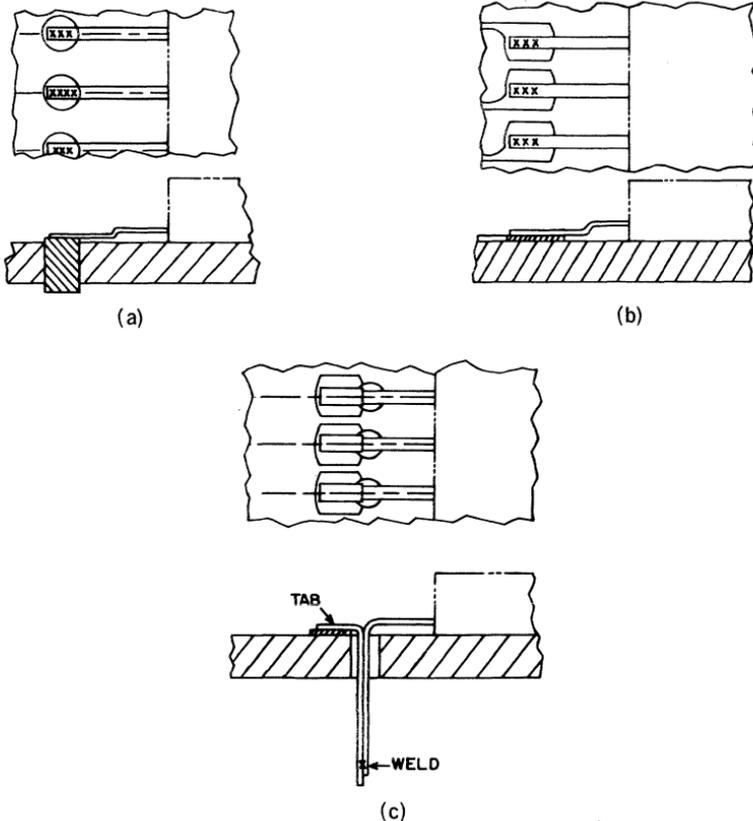
Fig. 14 — Welded connection methods for mounting RCA 14-terminal flat packs: (a) post method; (b) surface-pad method; (c) tab method.
