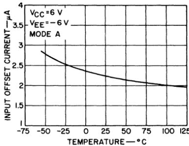
Fig. 108 — Input offset current of the CA3002 as a function of temperature.
