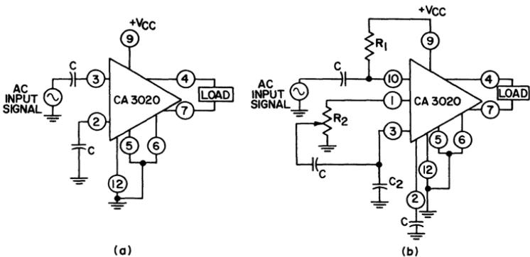
Fig. 241 — Input-impedance options for the CA3020.
