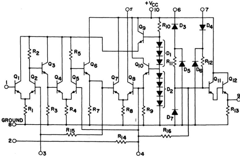
Fig. 254 — Schematic diagram of the CA3013 or CA3014 integrated-circuit amplifier-discriminator.
