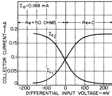
Fig. 27 — DC characteristics of the basic differential amplifier with and without emitter degeneration for a source current  $I_o$  of 0.188 milliamperes.
