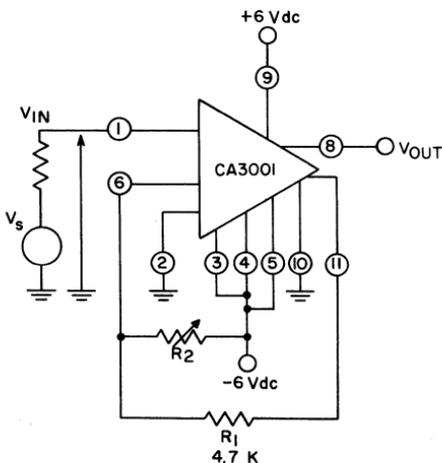
Fig. 103 — CA3001 Schmitt trigger.
