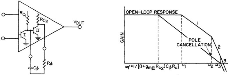
$A_o(\omega)$  = uncompensated open-loop gain
