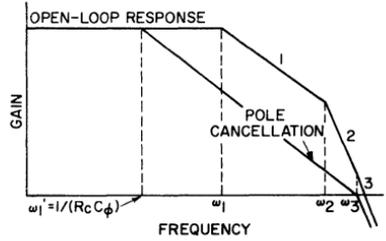
$A_o(\omega)$  = uncompensated open-loop gain
