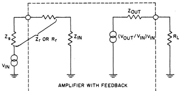
Fig. 60 — Equivalent-circuit model of a closed-loop operational amplifier.
