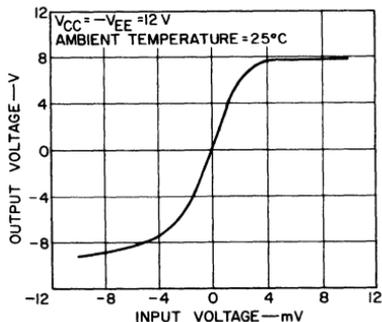
Fig. 226 — Open-loop transfer characteristics.
