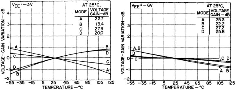
Fig. 107 — Voltage gain of the CA3002 (normalized to the 25°C voltage gain) as a function of temperature with  $V_{EE}$  supply voltages of -3 and -6 volts.
