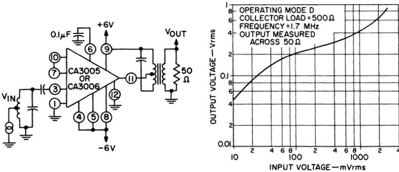
Fig. 170 — Limiting characteristics and circuit diagram of a CA3005 or CA3006 cascode limiter having a 500-ohm collector load impedance.
