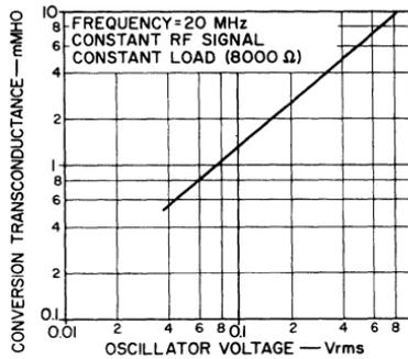
Fig. 187 — Conversion gain of a CA3005 or CA3006 mixer circuit as a function of oscillator voltage.
