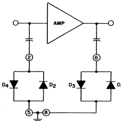
Fig. 286 — Limiters using the CA3019.
