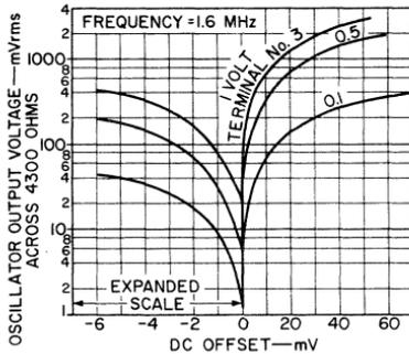
Fig. 189 — Cancellation of the oscillator signal at the output of a CA3005 or CA3006 mixer as a function of dc offset voltage.
