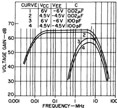
Fig. 102 — Three-stage CA3001 cascade amplifier and frequency-response characteristics.
