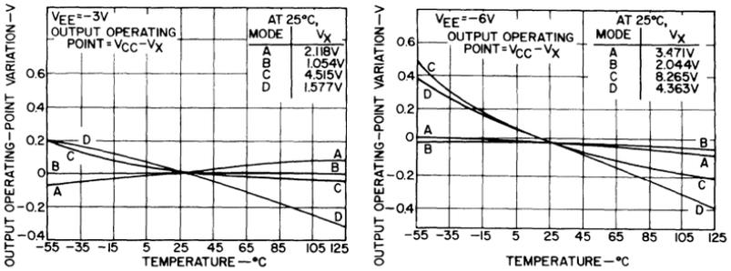
Fig. 106 — Output operating point of the CA3002 (normalized to the 25°C operating point) as a function of temperature with  $V_{EE}$  supply voltages of -3 and -6 volts.
