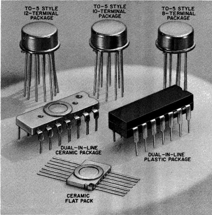
*Fig. 10 — RCA integrated-circuit packages.*
