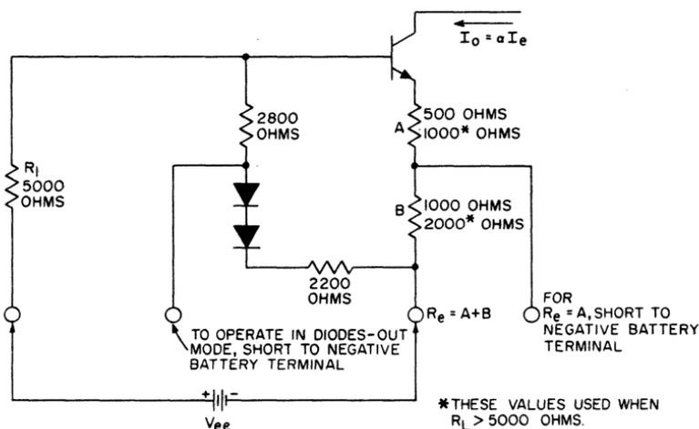
Fig. 57 — Current-sink configuration used in linear (differential-amplifier) integrated circuits.
