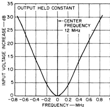
Fig. 177 — Frequency-response characteristics of the 12-MHz limiting amplifier shown in Fig. 175.
