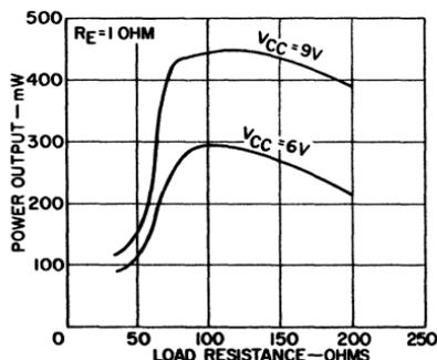
Fig. 243 — Output power as a function of load resistance.
