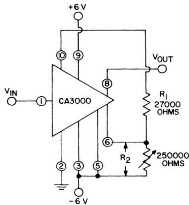
Fig. 88 — Schematic diagram of Schmitt trigger using CA3000.
