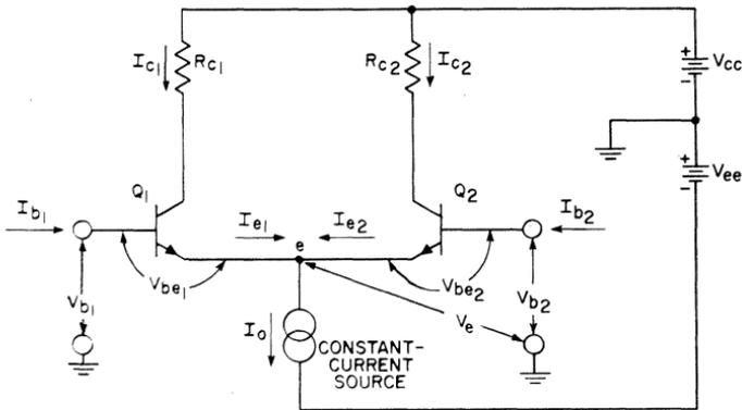
Fig. 20 — Schematic of the balanced differential amplifier used as the basic configuration for the linear integrated circuits.
