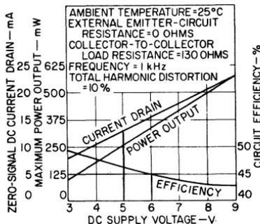
Fig. 239 — Performance characteristics of the CA3020 as a function of supply voltage.
