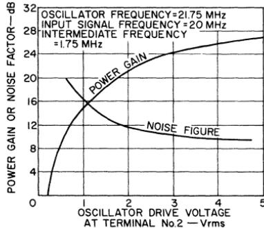
Fig. 192 — Power gain and noise figure as a function of oscillator drive voltage for the CA3004 balanced mixer.
