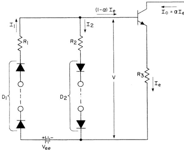
Fig. 37 — General configuration for a diode-stabilized transistor current-sink circuit.
