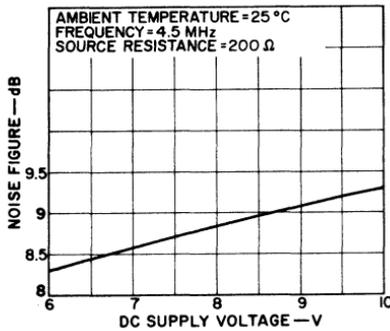
Fig. 256 — Noise figure as a function of dc supply voltage.
