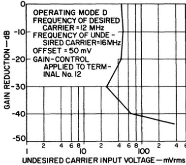
Fig. 165 — Gain control as a function of an undesired-carrier voltage that produces cross-modulation distortion of 10 per cent for a differential-amplifier configuration of the CA3005 or CA3006 having a 50-millivolt offset and with the gain-control voltage applied to the bias network of the constant-current transistor.
