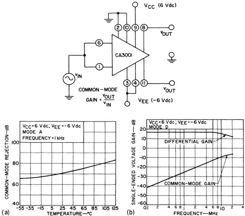
Fig. 101 — Common-mode rejection and voltage-gain characteristics of the CA3001 as a function of temperature and frequency.
