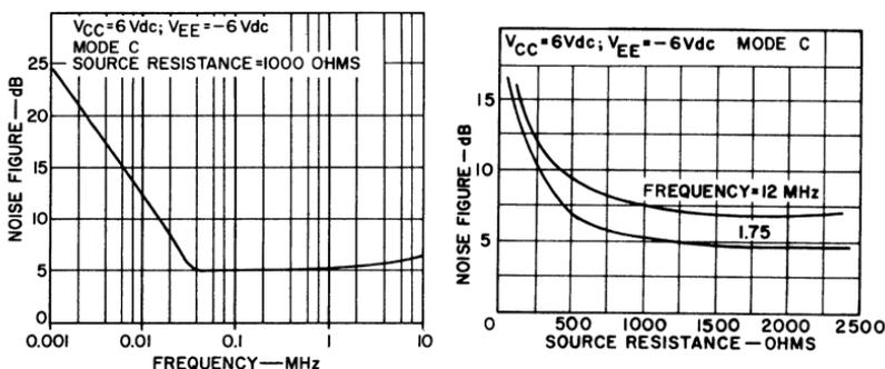
Fig. 99 — Noise figure of the CA3001 as a function of frequency and source resistance.
