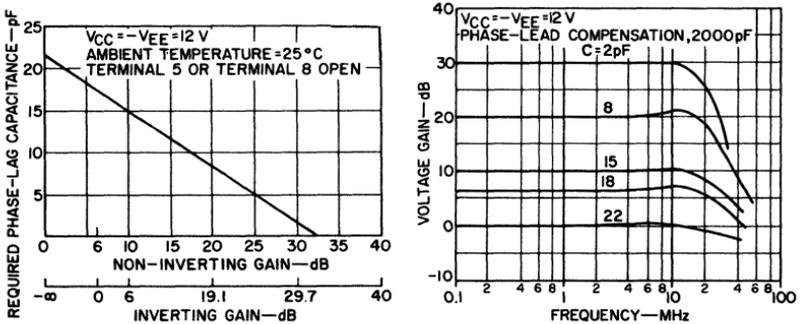
Fig. 230 — Amount of phase-lag capacitance required to obtain a flat ( $\pm 1$ -dB) response when phase-lead compensation is used, and typical response characteristics.
