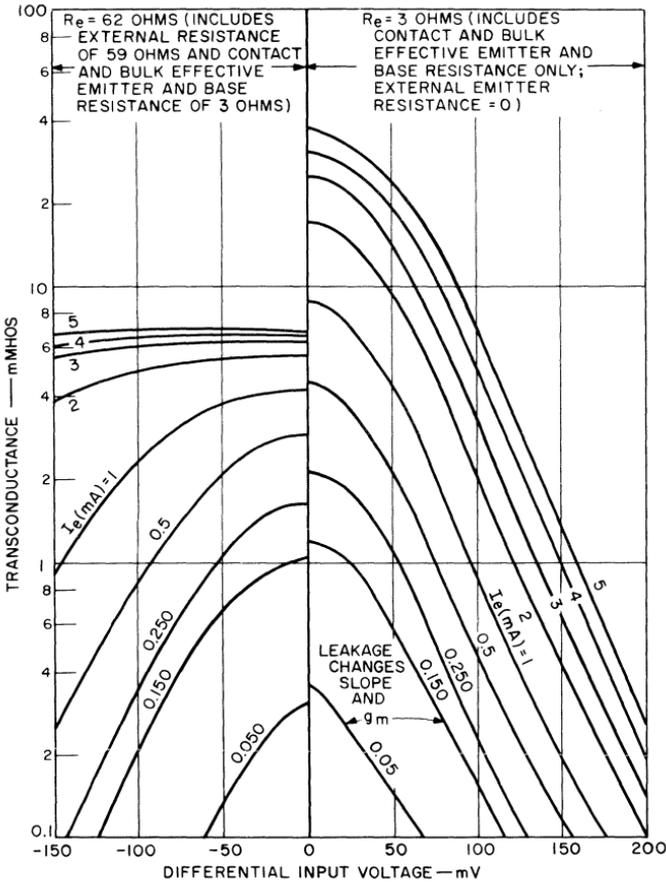
Fig. 28 — Transconductance of the basic differential amplifier as a function of differential input voltage for operation with and without emitter degeneration.
