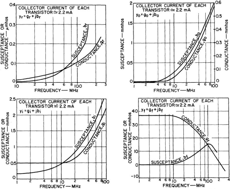
Fig. 152 — Admittance parameters of a CA3028A differential amplifier as a function of frequency.
