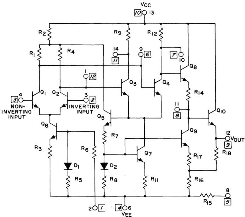
Fig. 225 — Schematic diagram for the  $\pm 12$ -volt operational amplifiers (CA3015, CA3015A, CA3016, CA3016A, CA3030, CA3030A, CA3038, and CA3038A).
