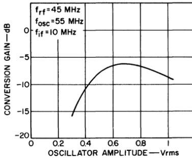
Fig. 293 — Conversion gain as a function of oscillator voltage for the balanced mixer of Fig. 292.
