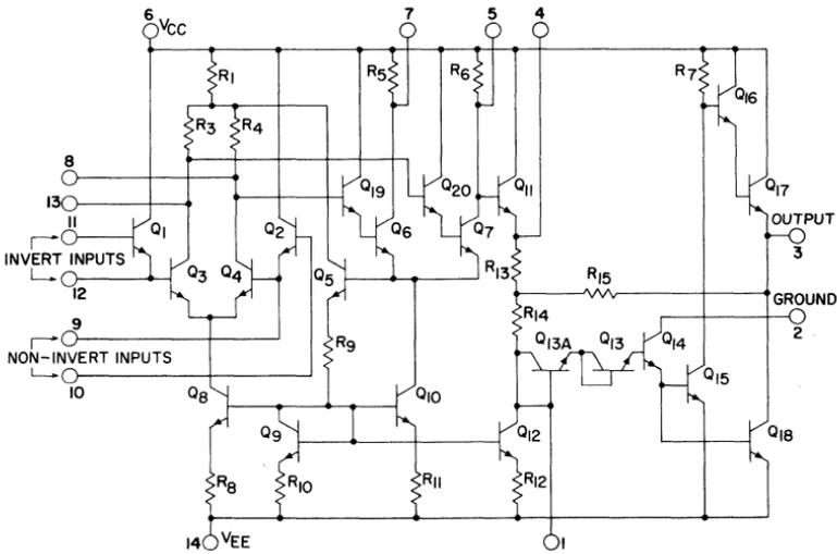
Fig. 236 — Schematic diagram of the CA3033 or CA3033A integrated-circuit operational amplifier.
