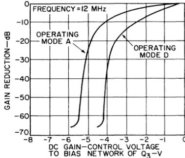
Fig. 159 — Gain-control characteristics of the CA3005 or CA3006 as a function of the dc gain-control voltage applied to the bias network of transistor Q<sub>3</sub>.
