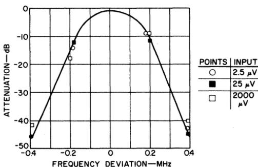
Fig. 273 — Measured over-all selectivity curve for if-amplifier strip of Fig. 269 and a given ratio detector.
