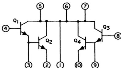
Fig. 307 — Schematic diagram of the CA3036 integrated-circuit dual Darlington array.
