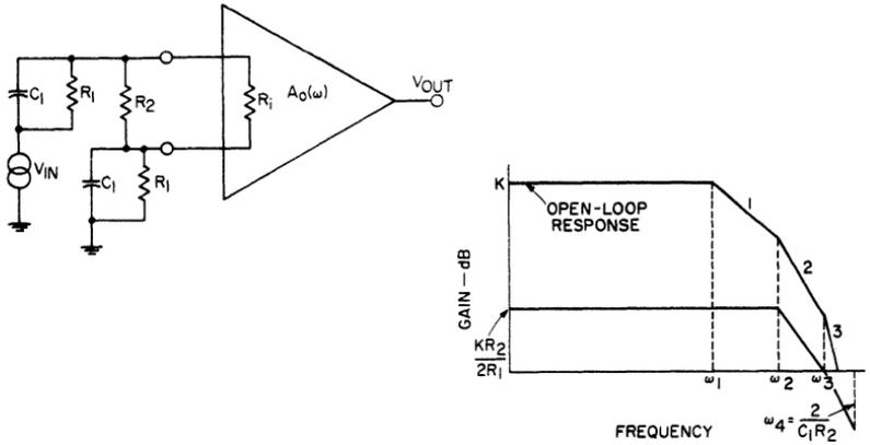
$A_o(\omega)$  = uncompensated open-loop gain
