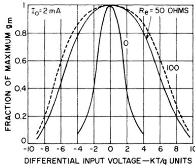
Fig. 25 — Effect of emitter degeneration on the transconductance of the basic differential amplifier.
