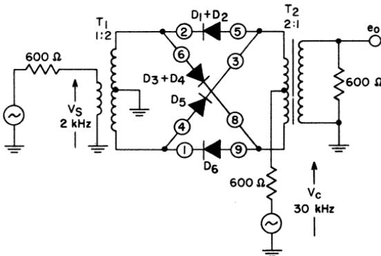
Fig. 295 — Ring modulator using the CA3019.
