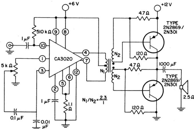
Fig. 249 — 7-watt class B single-ended audio amplifier.
