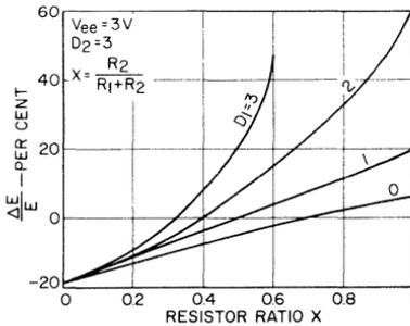
Fig. 44 — Effect of the number of diodes  $D_1$  on the variations in the voltage  $E$  as a function of the ratio  $X$  for a temperature increase of  $100^\circ\text{C}$  and a supply voltage  $V_{ee}$  of 3 volts when three diodes  $D_2$  are used.
