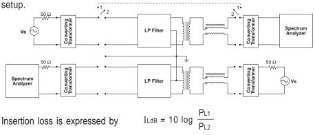
where PL1 is the power delivered to the load with both switches in position 1 with the filter by passed. PL2 is the output power with boths swithches in position 2. This expression can also be shown in terms of amplituded vol-tage ratio. The decibel unit is used to express a measure of insertion loss.
