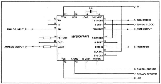
Fig.14 Simple application circuit
