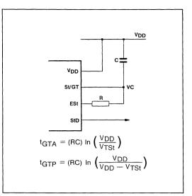
Fig.7 Basic steering circuit
