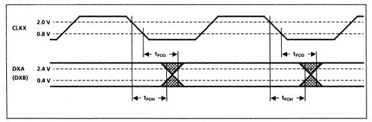
Fig. 26 Timing - PCM output changing during burst (see Fig. 4)
