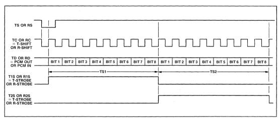
Fig.7 Signal alignment for MV3506/7/8 Codecs
