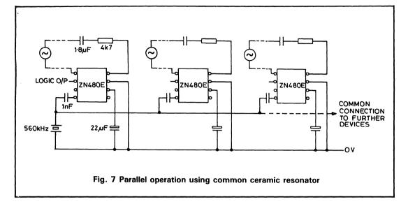
In Fig. 7 each device is powered by its separate ringing voltage and isolated individually by supply decoupling capacitors.
