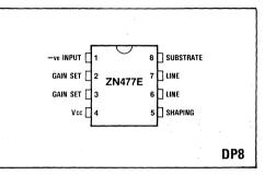
Pin connections - top view
