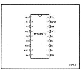
Fig.1 Pin connections - top view
