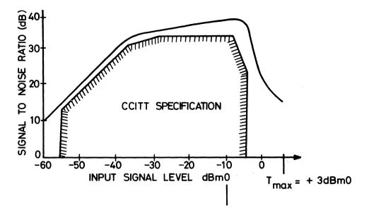
Fig. 2(a). Signal to Noise Ratio 'A Law'
