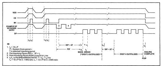
Fig.3 Keypad pulse dialer timing diagram, CE-External control
