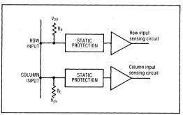
Fig.5 Row and column inputs
