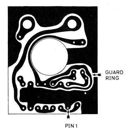
Fig. 3 Reverse Side of a PCB Indicating Guard Ring Screening on the ZN472E.
