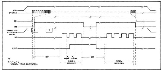
Fig.4 Keypad pulse dialer timing diagram, CE-Internal control
