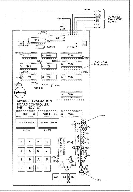
Fig.5 Controller PCB component layout
