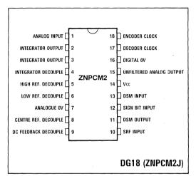
Pin connections - top view
