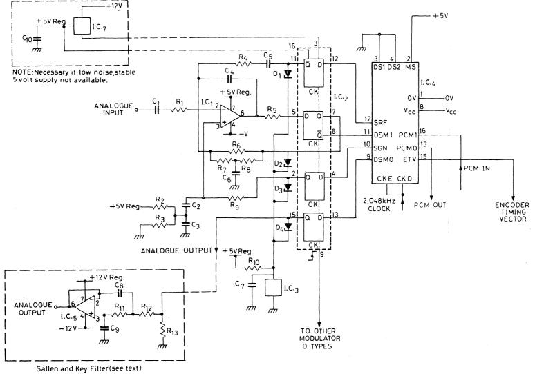
Fig. 3. Discrete Delta Sigma Modulation Circuit
