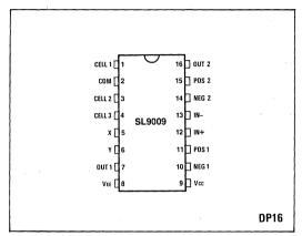
Fig.1 Pin connections - top view
