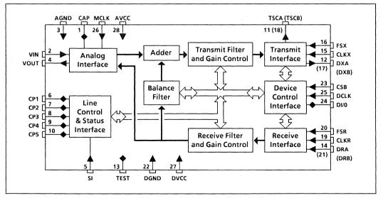
Fig. 2 Functional block diagram
