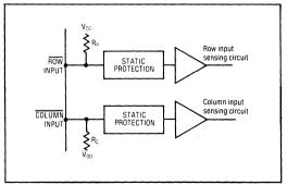
Fig.5 Row and Column inputs
