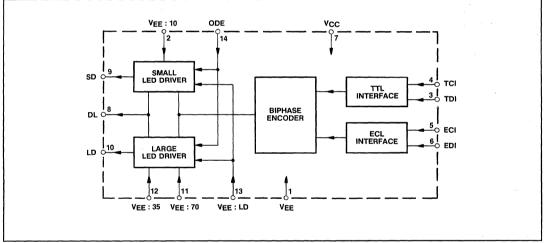
Fig.2 Functional block diagram (DG package pin out)
