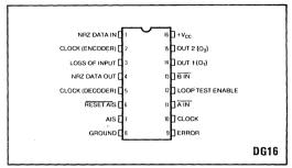
Fig. 1 Pin connections
