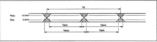
Fig.8 Timing - receive data
