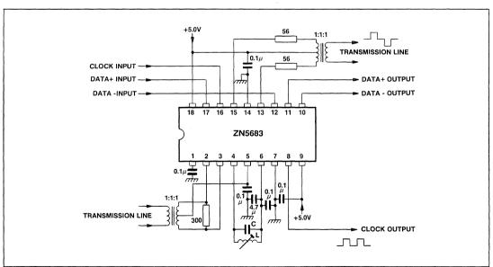
Fig.4 Recommended circuit
