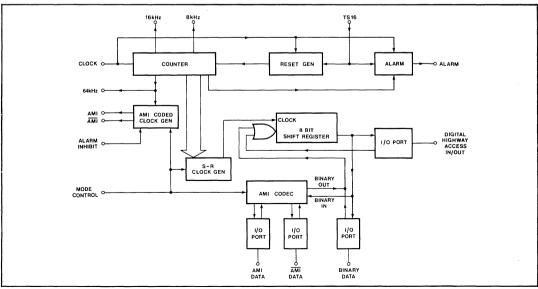
Fig.2 Block diagram
