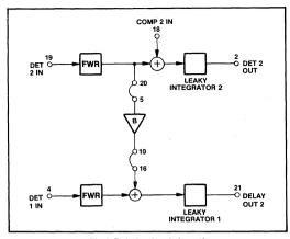
Fig.6 Relative level detection
