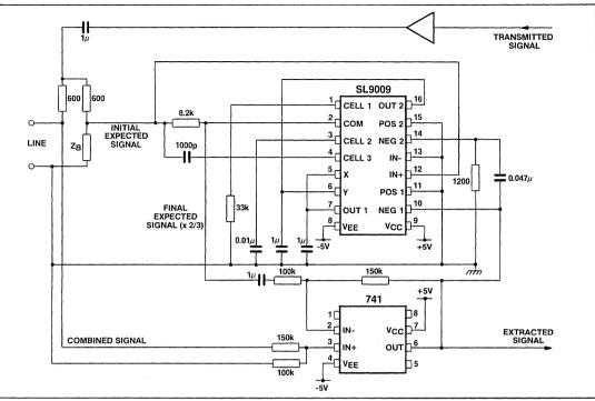
Fig.8 Circuit for improved line modelling
