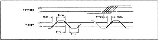
Fig.12 Timing - receive clock
