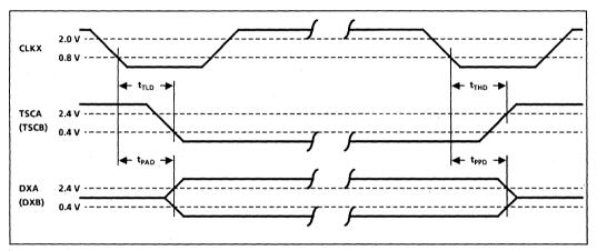
Fig. 25 Timing - PCM Output Start and Stop of Burst (see Fig. 4)
