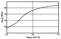
Fig.6 Typical reference VCO characteristic
