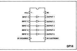
Fig.1 Pin connections (viewed from underside)
