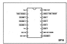
Fig.1 Pin connections - top view
