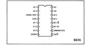
Fig.1 Pin connections
