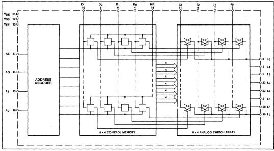
Fig.2 MV8804 functional block diagram
