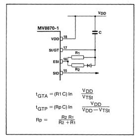
Fig.8 Guard time adjustment (tgrp>tgrA)
