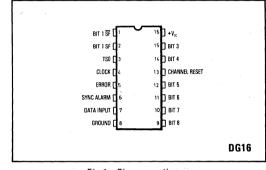
Fig.1 Pin connections
