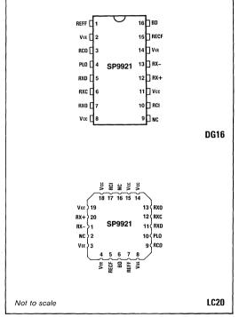
Fig.1 Pin connections - top view
