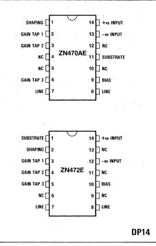
Pin connections - top view
