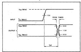
Fig. 15 Test timing definitions
