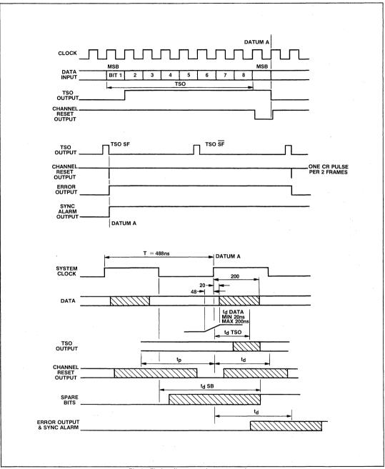
Fig.4 Timing diagram and output waveforms
