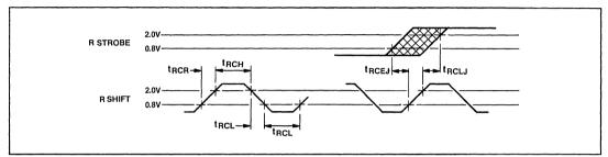
Fig.9 Timing - receive clock
