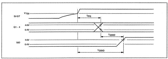
Fig.14 Timing - decoded data
