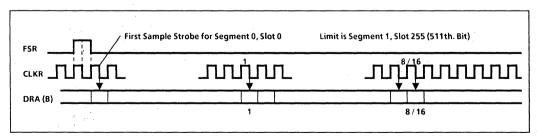
Fig. 3 Receive timing diagram
