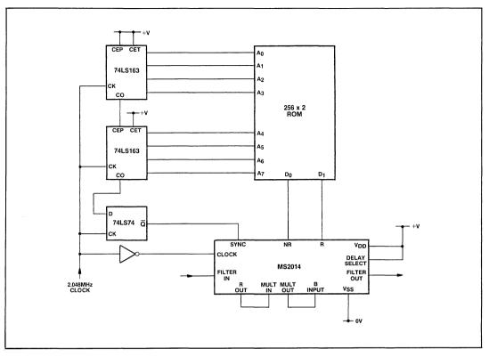
Fig.9 A 16th order 4kHz bandwidth filter
