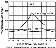
Fig.6 ON resistance vs input signal voltage
