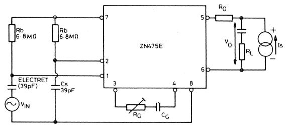
Fig. 2 Typical Electret Microphone Amplifier
