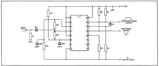
Fig.3 Functional test circuit
