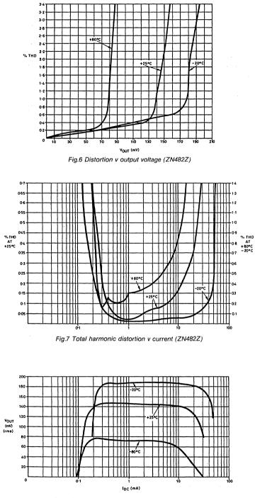
Fig.8 Output voltage v current at 2% THD (ZN482Z)
