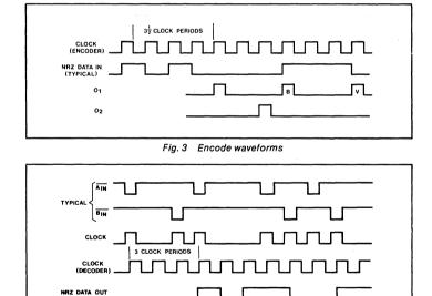
Fig. 4 Decode waveforms
