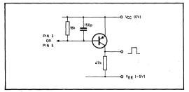
Fig.8 Interfacing with pulse fail output with CMOS
