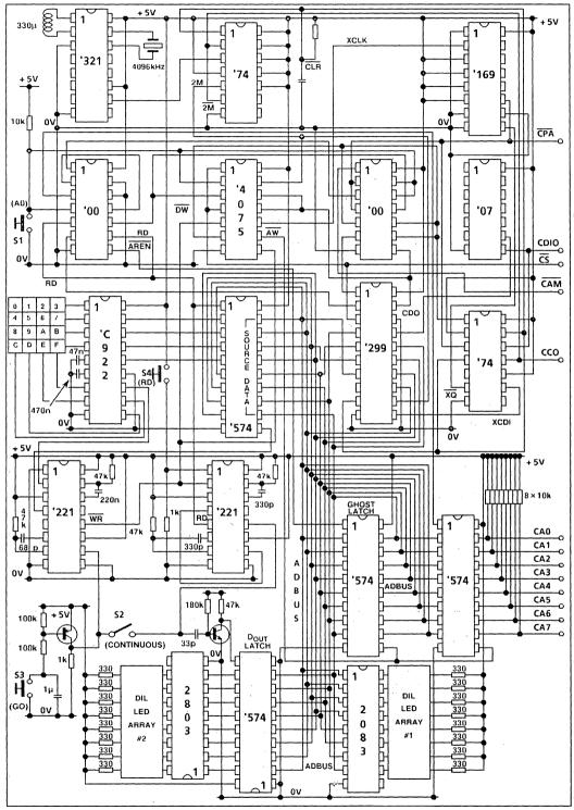
Fig.4 Controller PCB circuit diagram
