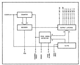
Fig.2 Block diagram MJ1445
