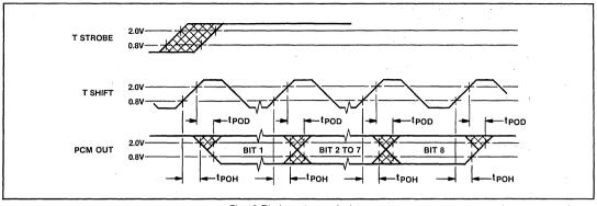
Fig.13 Timing - transmit data
