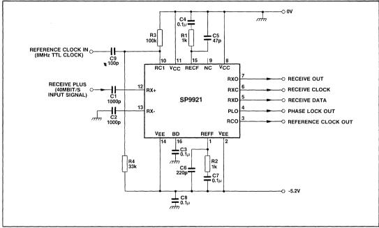
Fig.11 Typical application circuit (DG package pin out)
