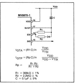
Fig.12 Non-symmetric guard time circuit
