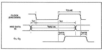
Fig.8 Encoder timing relationship
