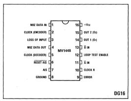
Fig.1 Pin connections - top view
