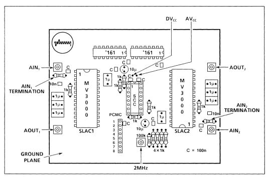
Fig.2 MV3000 evaluation board, component layout
