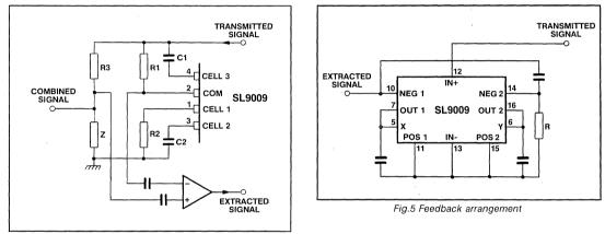
Fig.4 Simple balancing network
