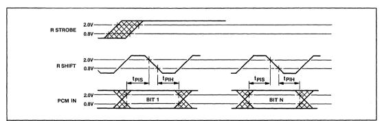
Fig.10 Timing - receive data
