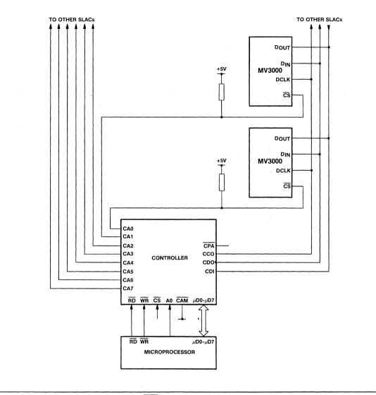
Fig.3  $\overline{CAM} = 1$  mode/line card application
