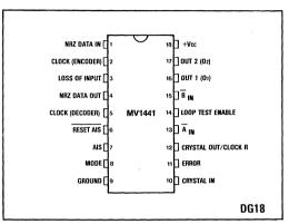
Fig.1 Pin connections - top view
