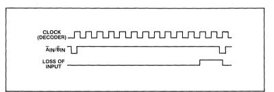
Fig.9 Loss of input waveforms
