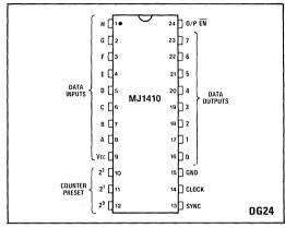
Fig.1 Pin connections
