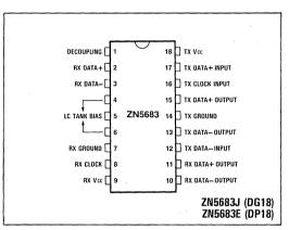
Fig.1 Pin connections - top view
