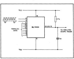
Fig.5 Test conditions (all outputs)
