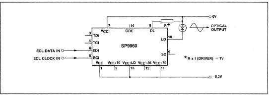
Fig.6 Typical ECL application circuit - large driver at 115mA (nominal) chosen **NB** For TTL applications the TTL inputs should be used, Vcc should be 5V and Vεε should be 0V (DG package pin out)
