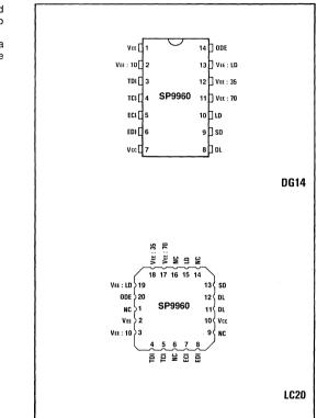
Fig.1 Pin connections - top view
