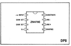
Pin connections - top view
