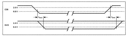
Fig. 31 Timing - data output start and stop of burst (see Fig. 9)
