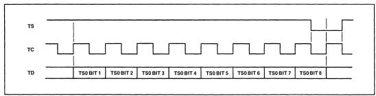
Fig.3 Transmit signal alignment
