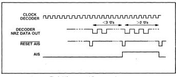
Fig.6 AIS error and Reset waveforms
