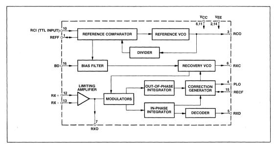
Fig.2 Functional block diagram (DG package pin out)
