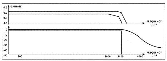
Fig. 34 Receive channel gain
