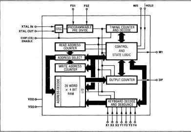
Fig.2 MV4320 functional block diagram
