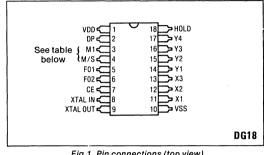
Fig.1 Pin connections (top view)
