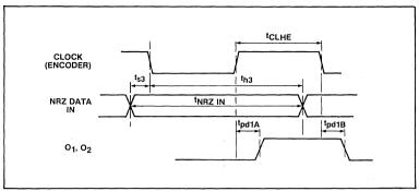
Fig.8 Encoder timing relationship
