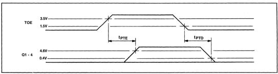
Fig.15 Timing - output enable and disable
