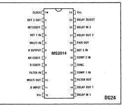
Fig.1 Pin connections - top view
