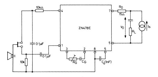
Fig. 2 Typical Application Circuit
