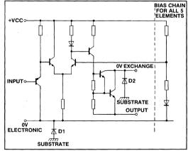
Fig.2 Circuit diagram of one element
