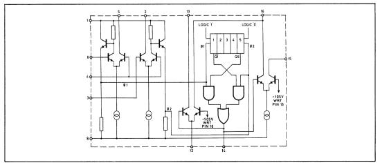
Fig.4 Circuit diagram of SP1450/SP1455
