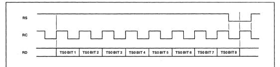
Fig.4 Receive signal alignment (RS shown for Frame-Alignment Frames)
