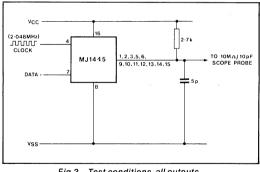
Fig.3 Test conditions, all outputs
