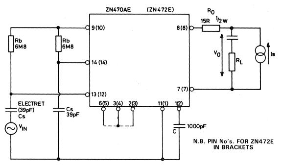
Fig. 2 Typical Electret Microphone Amplifier
