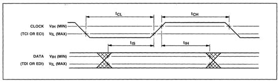
Fig.4 Digital switching characteristics - input
