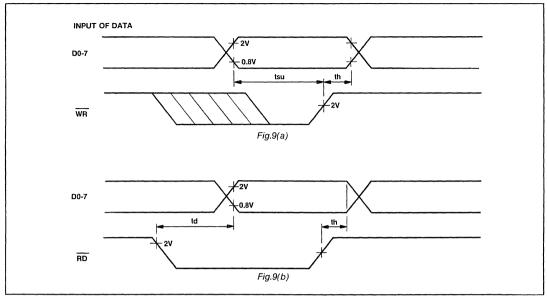
Fig.9 Register timing
