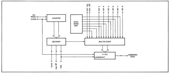
Fig.2 MJ1444 block diagram
