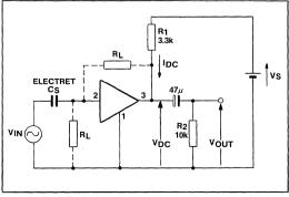
Fig.2 Typical buffer amplifier application circuit
