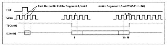
Fig. 4 Transmit timing diagram
