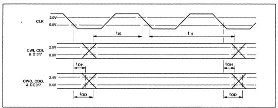
Fig.14 Timing - data and control inputs and outputs
