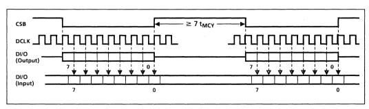
Fig. 9 Control timing diagram - normal operation
