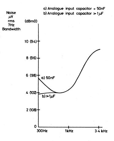
Fig. 1. Idle Channel Noise Spectrum
