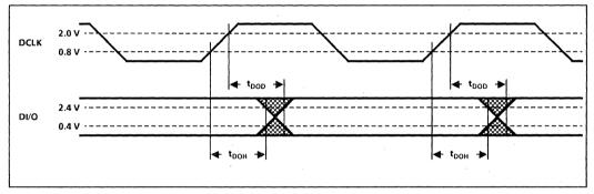
Fig. 32 Timing - data output changing during burst (see Fig. 9)
