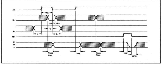
Fig.4 Timing waveforms
