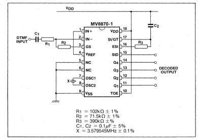
Fig.11 Single ended input configuration for BT or CEPT spec
