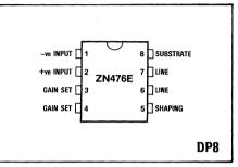
Pin connections - top view
