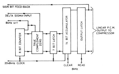
Fig. 5. Delta sigma to Linear pcm Converter
