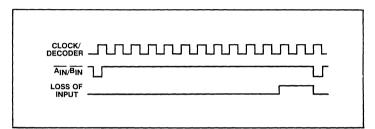
Fig.9 Loss of input waveforms
