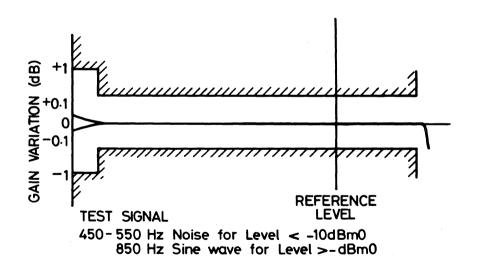
Fig. 2(b). Gain to Signal Level 'A Law'
