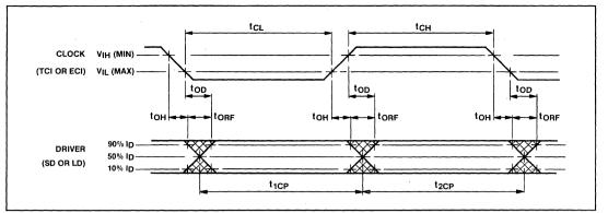
Fig.5 Digital switching characteristics - output
