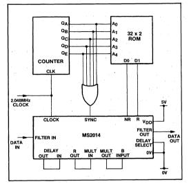
Fig.8 2nd order 32kHz bandwidth filter
