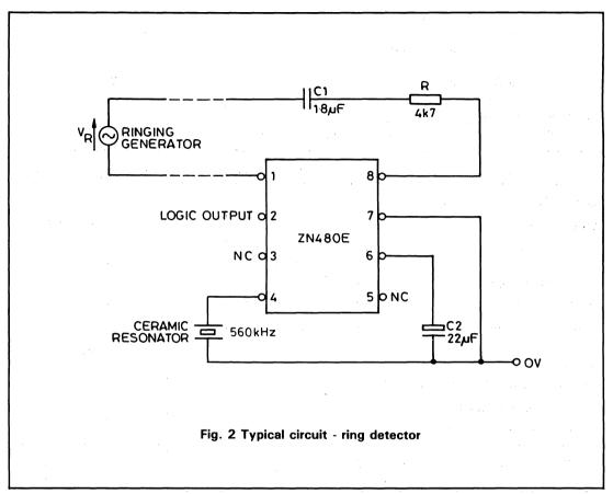
The operation of the ZN480E is most readily explained with reference to a typical circuit as shown in Fig. 2.
