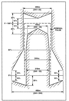
Fig.3 Input signal pulse mask
