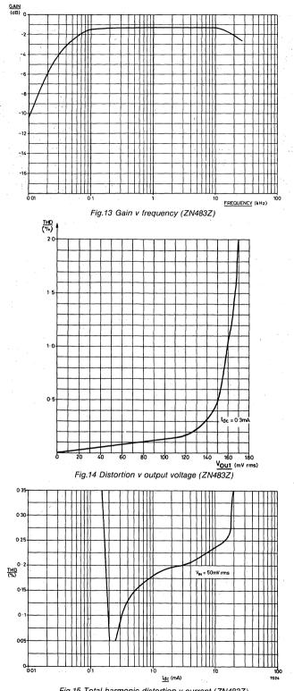
Fig.15 Total harmonic distortion v current (ZN483Z)
