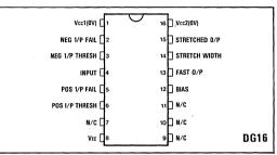
Fig.1 Pin connections (top view)
