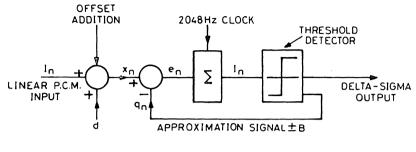
Fig. 9. The Digital DSM
