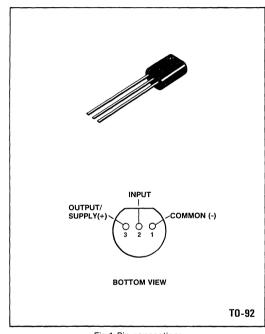
Fig.1 Pin connections
