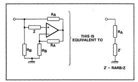
Fig.7 Gyrator circuit
