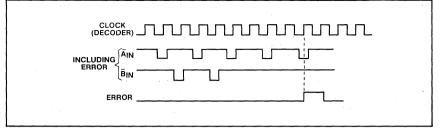
Fig.5 HDB3 error output waveforms
