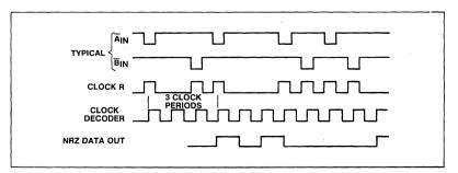
Fig.4 Decode waveforms
