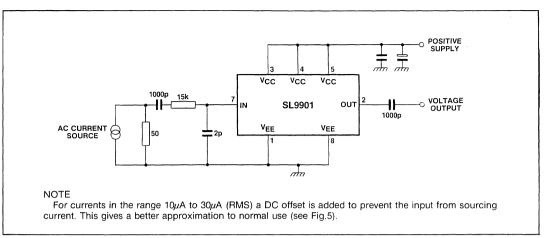
Fig.4 Test circuit
