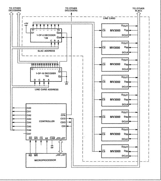
Fig.4  $\overline{CAM} = 0$  mode/PABX application
