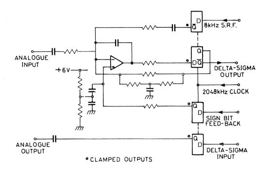
Fig. 2. Modulator/Demodulator Circuit
