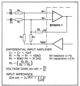
Fig.9 Differential input configuration
