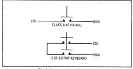
Fig.3 Keyboard configuration
