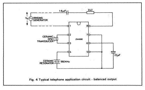
In this example pin 5 is connected to pin 7 (substrate) which selects output frequencies  $f_{H2}$  and  $f_{L2}$ . No frequency setting up procedures are called for because the clock frequency,  $f_C$ , is set by the ceramic resonator. This also ensures very good frequency stability with ambient temperature changes and life.
