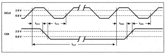
Fig. 29 Timing - chip select (see Fig. 9)
