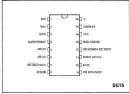
Fig.1 Pin connections
