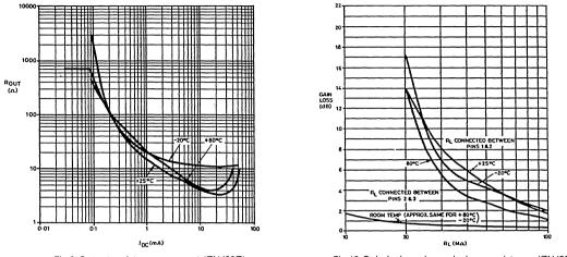
Fig.9 Output resistance v current (ZN482Z)
