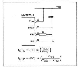
Fig.4 Basic steering circuit
