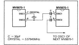
Fig.10 Oscillator circuit
