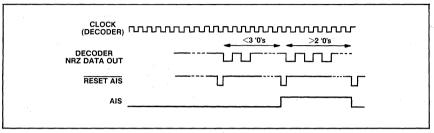
Fig.6 AIS error and Reset waveforms
