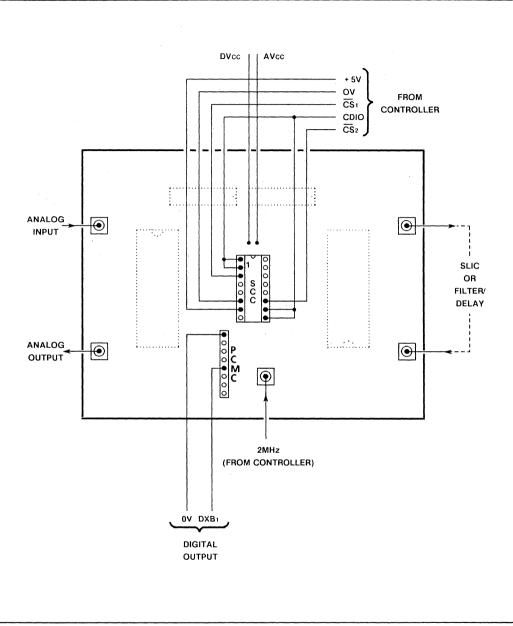
Fig.3 MV3000 evaluation board, test set-up 4
