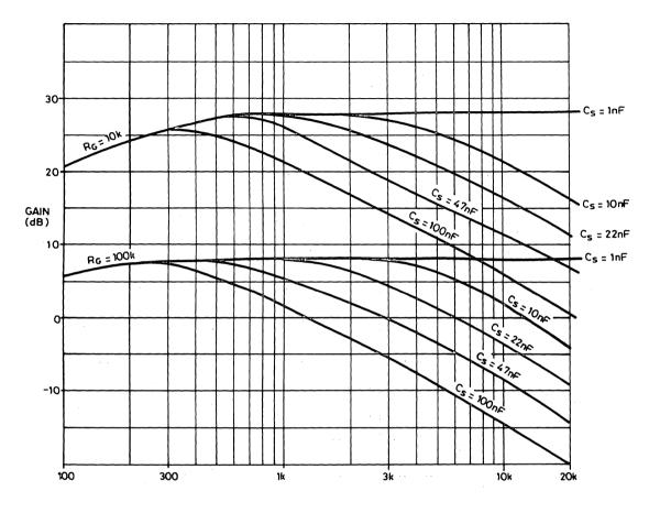
Conditions  $R_G$  = 10k and  $R_G$  = 100k  $I_C$  = 50mA  $C_G$  = 100nF
