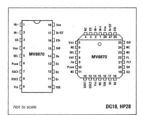
Fig.1 Pin connections (top view)
