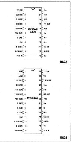
Fig.1 Pin connections - top view
