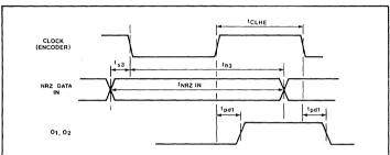
Fig. 8 Encoder timing relationship
