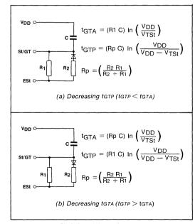
Fig.8 Guard time adjustment
