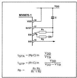
Fig.7 Guard time adjustment (tgtp < tgta)
