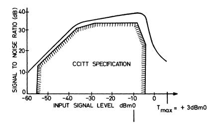
Fig. 8(a). Signal to Noise Ratio, 'A law'
