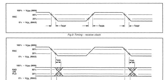
Fig.10 Timing - receive data and phase lock out
