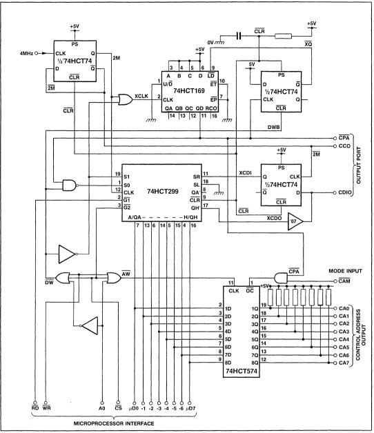
Fig.1 Line card controller logic diagram
