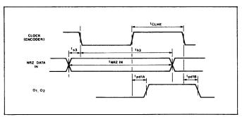
Fig. 8 Encoder timing relationship
