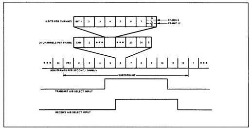
Fig.7 Signalling waveforms in a TI carrier system
