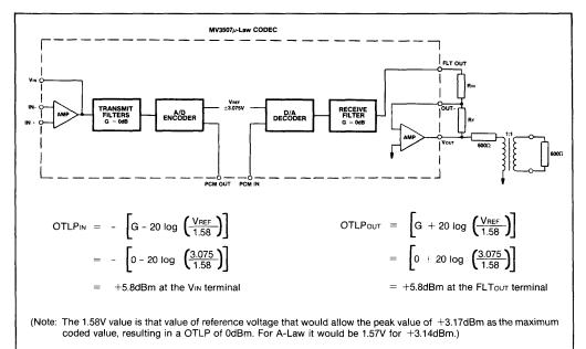
Since the output buffer amplifier is designed to drive  $1200\Omega$ , a  $600\Omega$  resistor in series with the  $600\Omega$  load divides the available voltage in half resulting in a OTLPout to the load of -0.2dBm.
