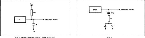
Fig.3 Propagation delay test circuits
