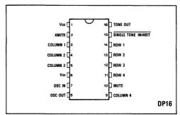
Fig.1 Pin connections - top view
