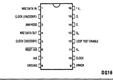
Fig.1 Pin connections
