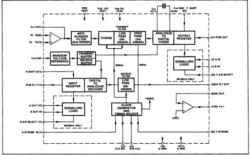
Fig.2 MV3506/MV3507/MV3507A block diagram. Pin numbers for the MV3507A are shown in brackets.
