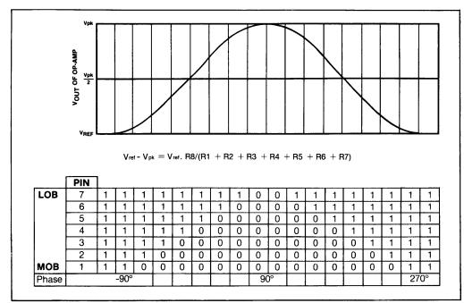
Fig.4 16 step sinewave produced by scanning 7 resistors
