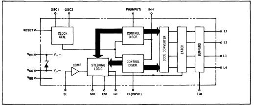
Fig.2 MV8860 functional block diagram
