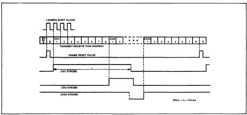
Fig.4 Waveforms in a 24 channel PCM system
