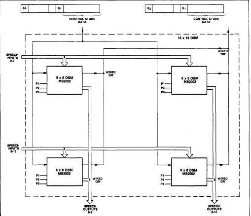
Fig.6 512 channel DSM made from four 8 x 8 DSMs
