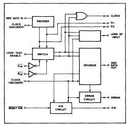
Fig. 2 Block diagram
