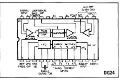
Fig.1 Pin connections (top view)
