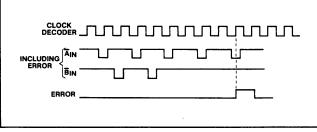
Fig.5 HDB3 error output waveforms
