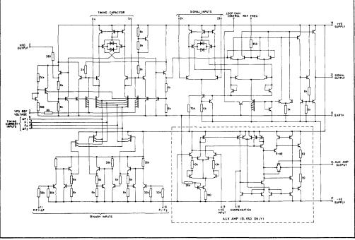
Fig. 2 Circuit diagram of SL650/SL651
