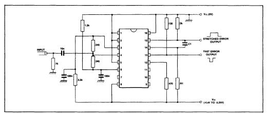
Fig.3 Functional test circuit
