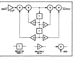
Fig.3 Basic 2nd order filter section
