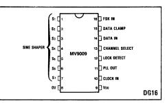
Fig.1 Pin connections - top view
