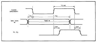
Fig. 8 Encoder timing relationship
