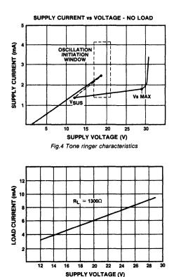
Fig.5 Typical RMS current
