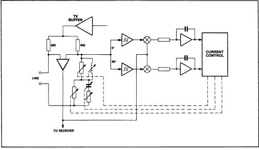
Fig.3 Simplified circuit illustrating cancellation principle
