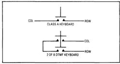
Fig.3 Keyboard configuration
