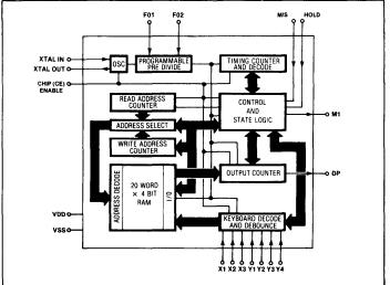
Fig.2 MV4320 functional block diagram
