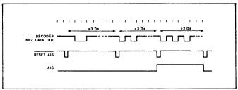
Fig.6 A/S error and reset waveforms
