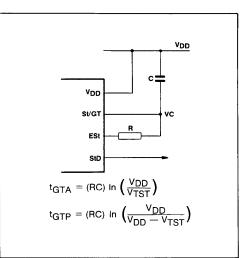
Fig.7 Basic steering circuit
