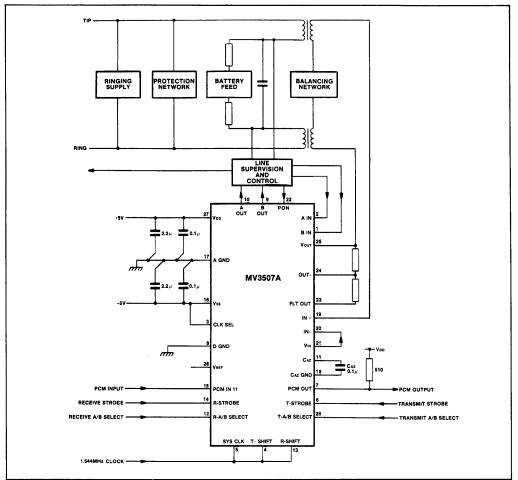
Fig.8 A subscriber line interface circuit
