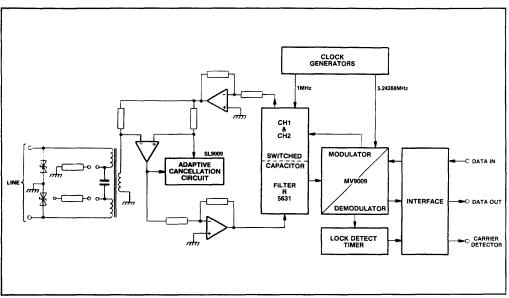
Fig.7 System block diagram
