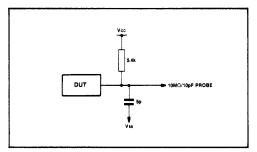
Fig.4 Propagation delay test circuit
