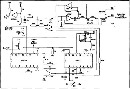
Fig.8 Basic V21 modem
