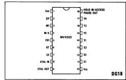
Fig.1 Pin connections (top view)
