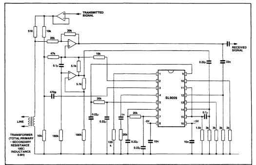
Fig.5 Typical line circuit for modem (900-3000Hz transmit frequency)
