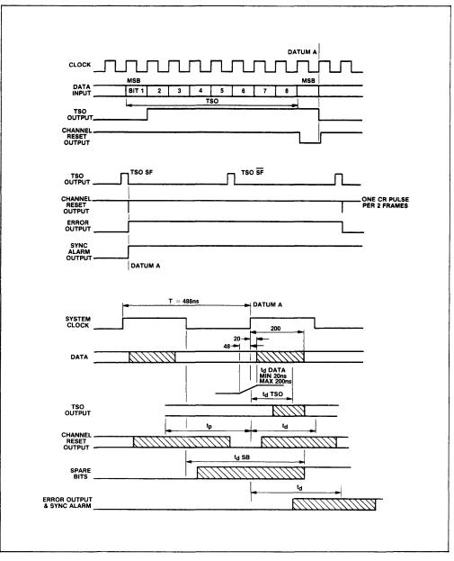
Fig.4 Timing diagram and output waveforms
