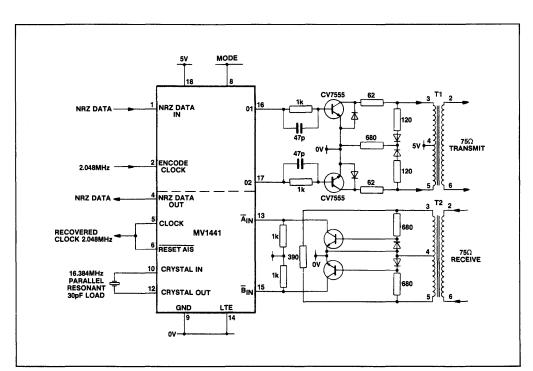
Fig.16 A typical application of the MV1441 with the interfacing to the transmission lines included
