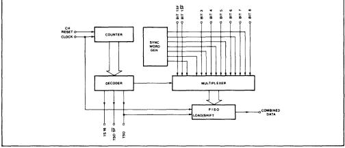
Fig.2 MJ1444 block diagram
