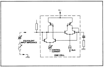
Fig.4 Conductance cell schematic
