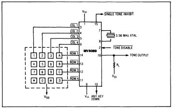
Fig.7 connection diagram
