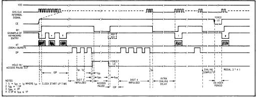
Fig.4 MV4325 timing diagram, CE Internal control
