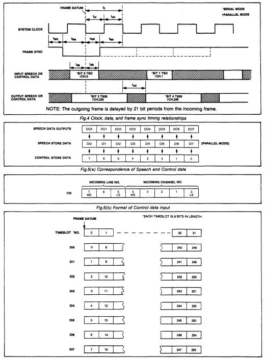
Fig.5(c) Channel numbering for incoming speech data (serial mode)
