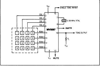
Fig.7 Connection diagram
