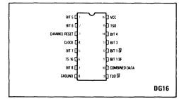
Fig.1 Pin connections
