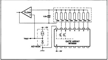
Fig.3 Output array scanning
