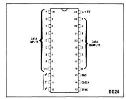
Fig.1 Pin connections
