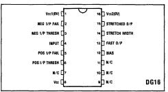
Fig.1 Pin connections (top view)
