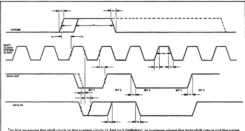
\*In this example the shift clock is the system clock (1.544 or 2.048MHz). In systems where the data shift rate is not the same the relationship of each to the strobe remains the same. The system clock and shift clock need not have coincident edges, but must relate to the strobe within the tsc, timing requirements.
