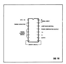
Fig. 1 Pin connections (top view)
