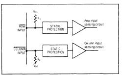
Fig.5 Row and Column inputs
