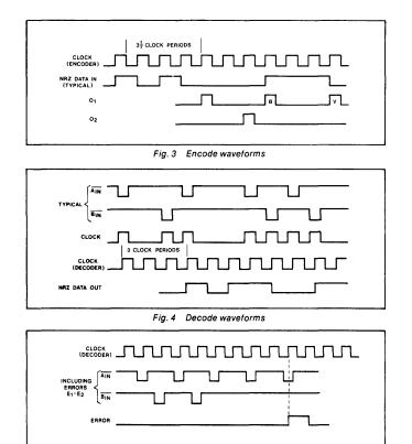
Fig. 5 HDB3 error output waveforms
