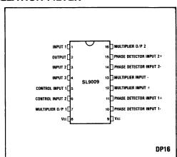
Fig.1 Pin connections - top view
