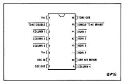
Fig.1 Pin connections - top view
