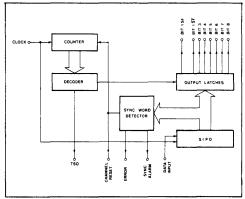
Fig.2 Block diagram MJ1445
