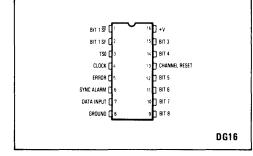
Fig.1 Pin connections
