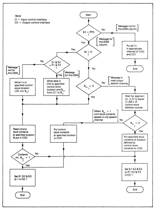
Fig.3 DSM control logic flowchart
