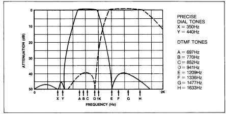
Fig.6 Typical filter characteristic
