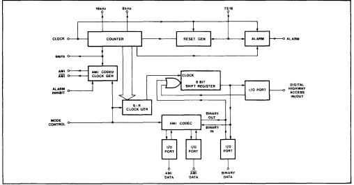
Fig.2 Block diagram
