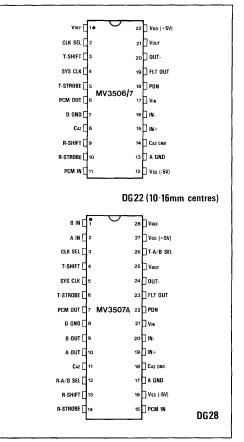
Fig.1 Pin connections - top view
