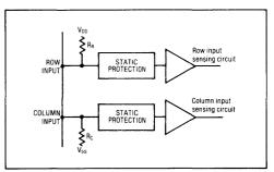
Fig.5 Row and column inputs
