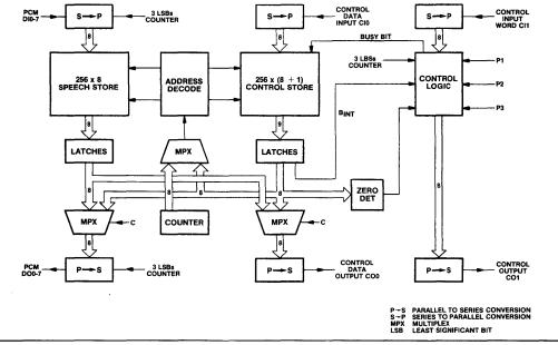
Fig.2 Block diagram of DSM
