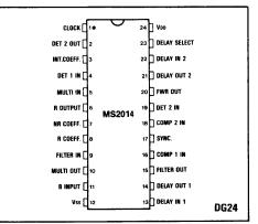
Fig.1 Pin connections - top view
