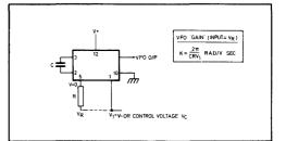
Fig. 5 VFO basic configuration
