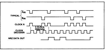
Fig.4 Decode waveforms
