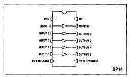
Fig. 1 Pin connections (viewed from underside)
