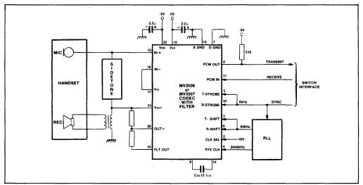
Fig.11 Voice processing in a digital telephone application
