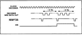
Fig.6 AIS error and Reset waveforms
