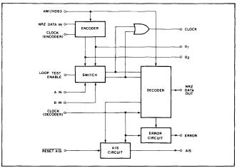
Fig. 2 MJ1471 Block diagram
