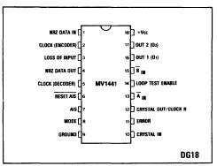
Fig.1 Pin connections - top view
