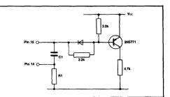
Fig.7(b) Interfacing with CMOS at the stretched output (SP1455)
