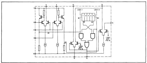
Fig.4 Circuit diagram of SP1450/SP1455
