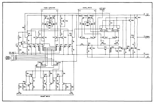
Fig. 3 Circuit diagram of SL652
