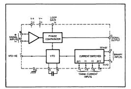
Fig. 2 SL652C block diagram
