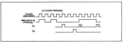
Fig.4 Encode waveforms
