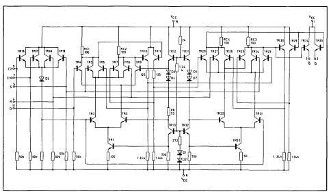
Fig. 12 SP1670 circuit diagram
