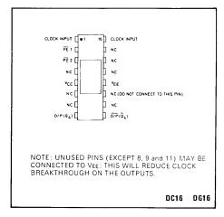
Fig. 1 Pin connections (top)
