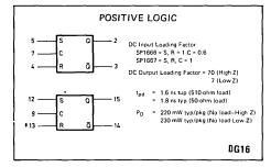
Fig. 1 Logic diagram of SP1666/1667
