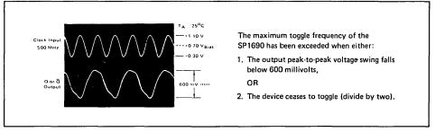
Fig. 8 Toggle frequency waveforms
