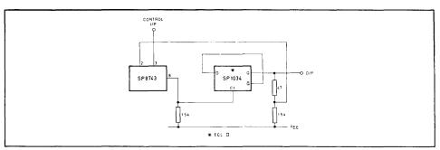
Fig.8 A-16/17 application. Control loop delay time approx. 24ns using SP1034
