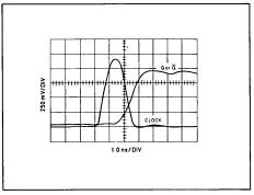
Fig. 11 Minimum 'up time' to clock output load =  $50\Omega$
