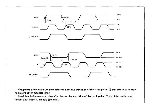
Fig. 6 Set up and hold time waveforms
