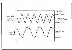
Fig. 9 Toggle frequency waveforms
