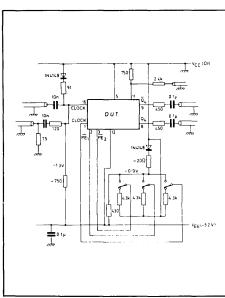
Fig. 5 Test circuit for dynamic measurements
