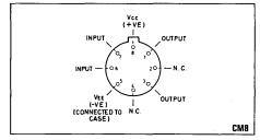
Fig. 1 Pin connections (bottom view)
