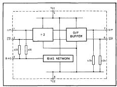
Fig. 2 SP8607 block diagram
