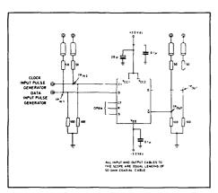
Fig. 4 Propagation delay test circuit
