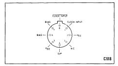
Fig. 1 Pin connections (viewed from beneath)
