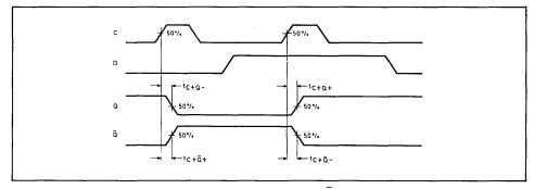
Fig. 6 Switching time waveforms (clock to  $Q/\overline{Q}$ , switch S1 in position opposite to that shown in Fig. 3
