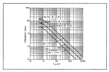
Fig. 3 Output frequency v capacitance for three values of input voltage
