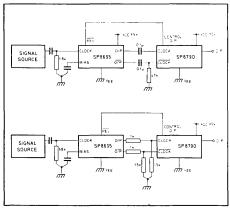
Fig. 6 Methods of preventing self-oscillation
