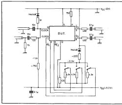
Fig. 5 Test circuit for dynamic measurements
