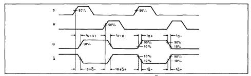
Fig. 5 Switching time waveforms (set/reset to Q/Q, switch S1 in position shown in Fig. 3)
