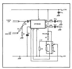
Fig.5 Test circuit for dynamic measurements
