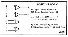
Fig. 1 Logic diagram of SP1692
