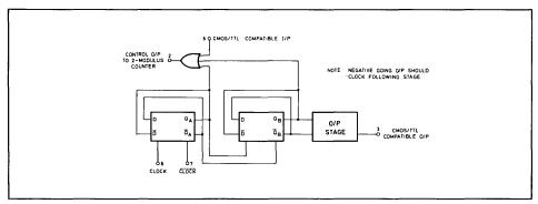
Fig. 2 Logic diagram
