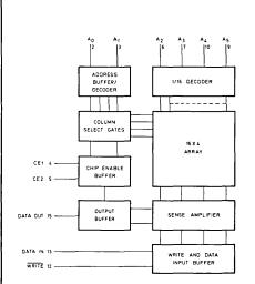
$\begin{array}{l} P_D = 420 \text{ mW typ /pkg} \\ t_{access} = 15 \text{ns (max) SP10140, SP10148} \\ = 10 \text{ns (max) SP10142} \end{array}$
