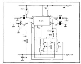
Fig. 5 Test circuit for dynamic measurements
