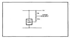
Fig.3 TTL/CMOS interface
