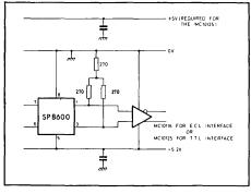
Fig. 7 ECL and Schottky TTL interfacing
