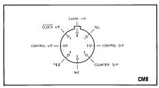
Fig. 1 Pin connections.
