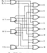
$P_D=315$ mW typ/pkg (No load)  $t_{pd}=4.0$ ns typ
