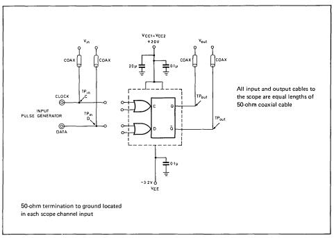
Fig. 3 Propagation delay test circuit
