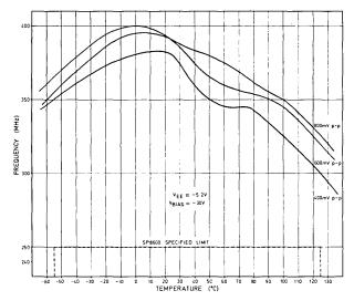
Fig. 5 Maximum input frequency v. temperature
