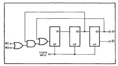
Fig. 2 Logic diagram SP8740
