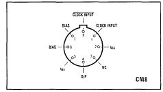
Fig. 1 Pin connections (viewed from beneath)
