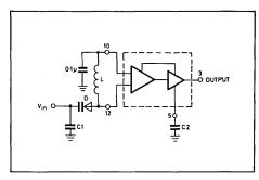
Fig. 5 The SP1648 operating in the voltage-controlled mode
