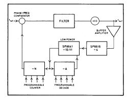
Fig. 8 A 1GHz synthesiser loop
