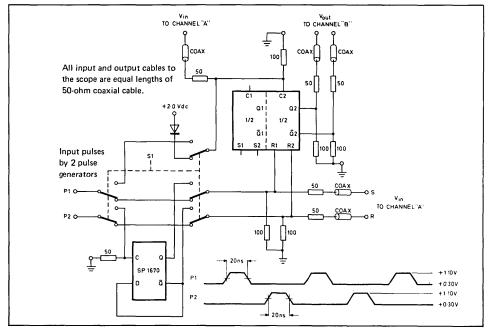
Fig. 4 Switching time test circuit
