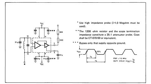
Fig. 4 Test circuit and waveforms
