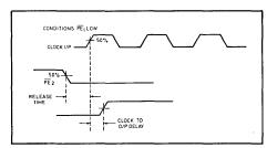
Fig. 4 Release timing diagram
