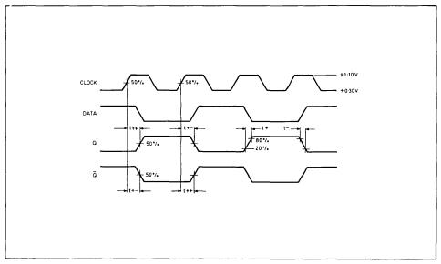
Fig. 4 Clock delay waveforms at +25°C
