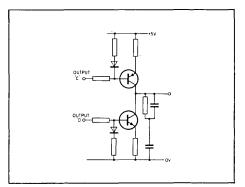
Fig. 5 Low voltage charge pump and filter
