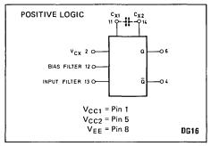
Fig. 1 Block diagram of SP1658
