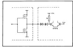
Fig. 3 CMOS and TTL compatible control I/P.
