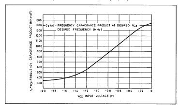
Fig. 5 Frequency-capacitance product v control voltage VCX
