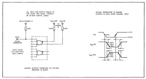
Fig. 3 Switching time test circuit and waveforms at +25°C
