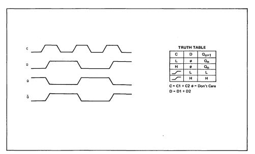
Fig. 2 Timing diagram
