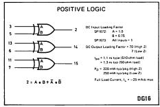
Fig. 1 Logic diagram of SP1672/1673
