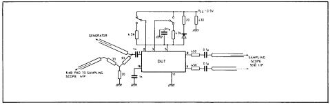
Fig. 3 Test circuit
