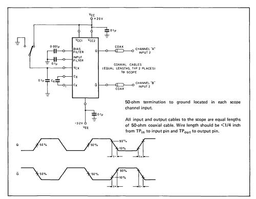
Fig. 2 AC test circuit and waveforms
