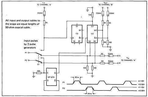
Fig. 4 Switching time test circuit
