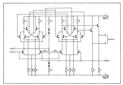
Fig. 2 Circuit diagram (all resistor values are nominal)
