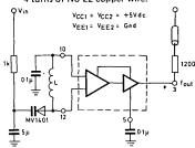
The 1200 ohm resistor and the scope termination impedance constitute a 25:1 attenuator probe. Coax shall be CT-070-50 or equivalent.
