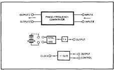
Fig. 2 SP8760 block diagram
