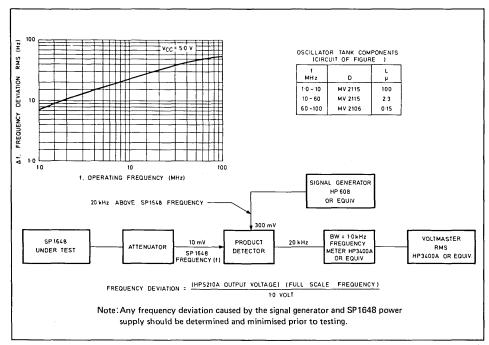
Fig. 6 Frequency deviation test circuit
