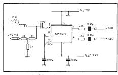
Fig. 3 Toggle frequency test circuit
