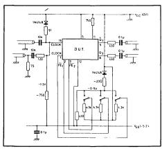
Fig. 5 Test circuit for dynamic measurements
