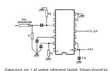
Capacitors are 1 nf unless otherwise stated. Values should be increased if operation below 10 MHz is desired. For 50 mV hysteresis  $R1=36k\Omega\,R2=\infty$  For 100 mV hysteresis  $R1=18k\Omega\,R2=18k\Omega$
