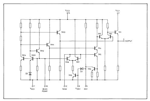
Fig. 2 Circuit diagram of SP1648
