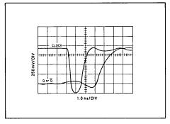
Fig. 10 Minimum 'downtime' to clock output load = 50\(\Omega\)
