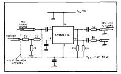
Fig. 4 Toggle frequency test circuit
