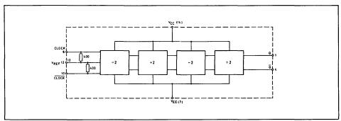
Fig. 2 Functional diagram
