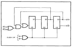
Fig. 2 Logic diagram (positive logic)
