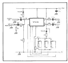
Fig.5 Test circuit for dynamic measurements
