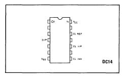
Fig. 1 Pin connections
