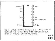
Fig. 1 Pin connections
