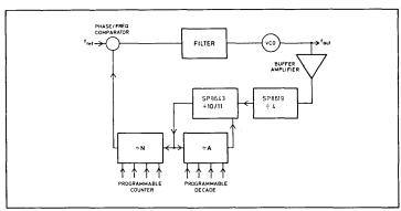
Fig. 6 A 1.5GHz synthesiser loop
