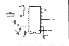
Capacitors are 1 nF unless otherwise stated. Values should be increased if operation below 10 MHz is desired. For 50mV hysteresis R1=36k $\Omega$ R2= $\infty$ For 100mV hysteresis R1 =  $18k\Omega$ R2 =  $18k\Omega$
