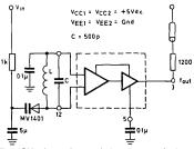
The 1200 ohm resistor and the scope termination impedance consitute a 25:1 attenuator probe. Coax shall be CT-070-50 or equivalent.
