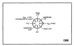
Fig. 1 Pin connections (bottom view)
