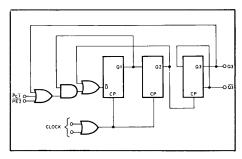
Fig. 2 Logic diagram (positive logic)
