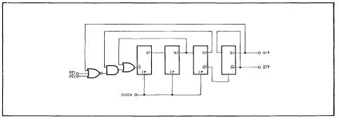
Fig. 2 SP8743 logic diagram
