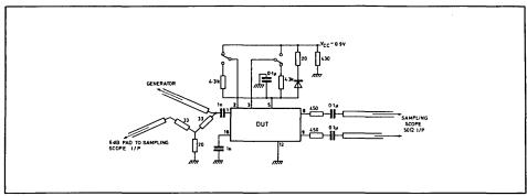
Fig. 3 Test circuit
