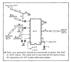
Fig. 3 AC test circuit
