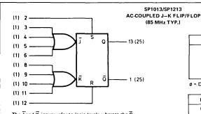
The  $\overline{J}$  and  $\overline{K}$  inputs refer to logic levels whereas the  $\overline{C}_{\underline{D}}$ input refers to dynamic logic swings. The J and K inputs should be changed to logic '1' only while  $\overline{C}_D$  is in the logic '1' state, ( $\overline{C}_D$  maximum '1' level =  $V_{CC}$ -0.6V). Clock  $\overline{C}_D$  is obtained by tying one  $\overline{J}$  and one  $\overline{K}$  input together.
