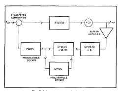
Fig. 5 A low power synthesiser loop
