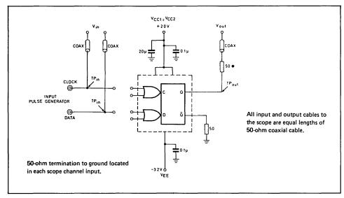
Fig. 5 Set up and hold time test circuit
