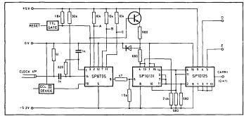
Fig.7 600MHz ÷ 32 with reset and inhibit
