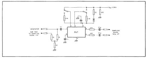
Fig. 3 Test circuit
