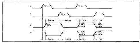
Fig. 5 Switching time waveforms (set/reset to  $Q.\overline{Q}$ , switch S1 in position shown in Fig. 4)
