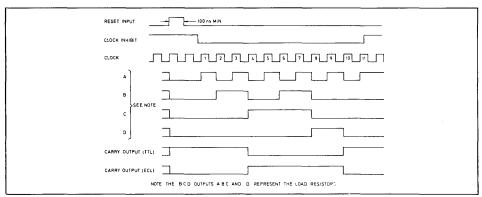
Fig. 6 Decade counter timing diagram
