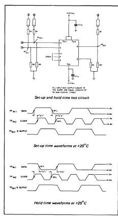
Fig. 7 Set-up and hold time test circuit
