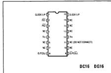
NOTE: UNUSED PINS (EXCEPT 8 AND 9) MAY BE CON-NECTED TO VEE: THIS WILL REDUCE CLOCK BREAK-THROUGH ON THE OUTPUTS. PINS 8 AND 9 SHOULD BE LEFT OPEN-CIRCUIT WHEN NOT IN USE. PIN 11 IS INTERNALLY CONNECTED AND MUST ALWAYS BE LEFT OPEN-CIRCUIT.
