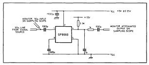
Fig. 3 Test circuit
