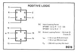
Fig. 1 Logic diagram of SP1668/1669
