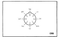
Fig., 1 Pin connections
