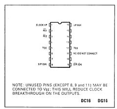
Fig. 1 Pin connections (top)
