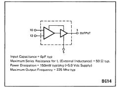
Fig. 1 Block diagram of SP1648
