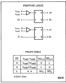
Fig. 1 Logic diagram of SP1651
