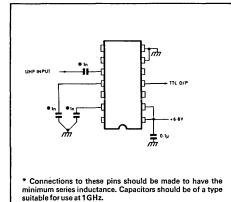
Fig. 3 Application circuit
