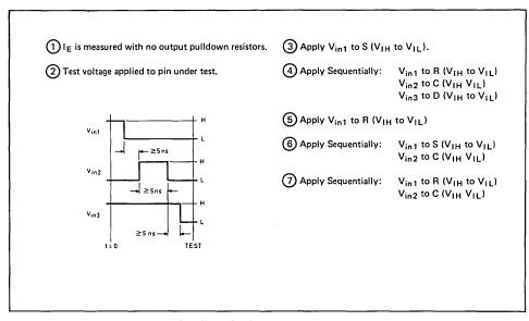
Fig. 3 Notes referred to in electrical characteristics
