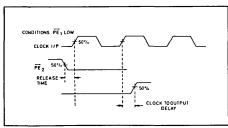
Fig. 4 Release timing diagram
