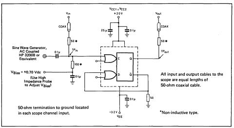
Fig. 7 Toggle frequency test circuit
