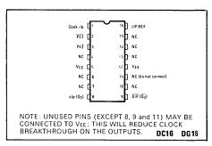
Fig. 1 Pin connections
