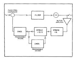
Fig. 5 A low power synthesiser loop
