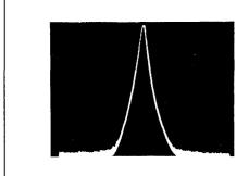
B.W. = 10kHz Scan Width = 50kHz/div Center Frequency = 100MHz Vertical Scale = 10db/div L: Micro Metal torroid #T20.13, 8 turns #30 Enameled Copper wire.
