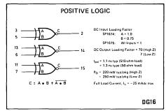
Fig. 1 Logic diagram of SP1674/1675
