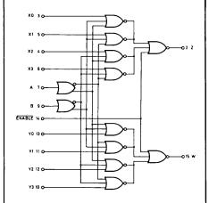
$P_D=155mW \text{ typ/pkg}$  $t_{pd}=2.5ns \text{ typ}$
