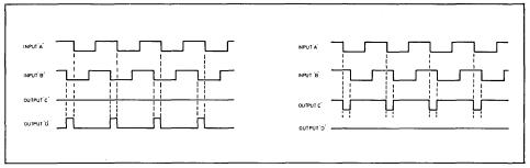
Fig. 3 Phase/frequency comparator waveforms
