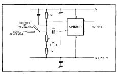
Fig. 6 Bias arrangement to prevent self-oscillation under no-signal conditions
