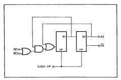
Fig. 2 Logic diagram SP8720
