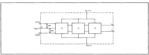
Fig. 2 Functional diagram
