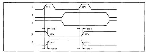
Fig. 6: Switching time waveforms (clock to  $Q/\overline{Q}$ , switch S1 in opposite position to that shown in Fig.-4)
