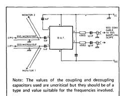
Fig. 3 Test circuit
