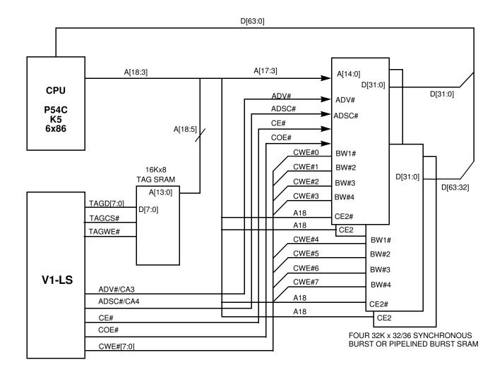
Figure 3-8. 512 Kbyte L2 Cache Using Four 32K X 32/36 Synchronous or Pipelined Burst SRAM
