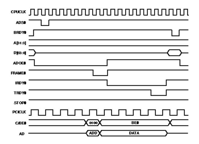
Figure 5-6. CPU-to-PCI Memory Read Cycle
