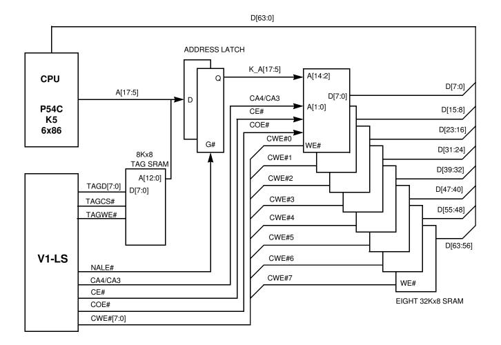
**NOTE:** TAGCS# and NALE# are multiplexed on a single pin. If NALE# function is used with asynchronous SRAM, the CS# of TAG SRAM should be connected to ground.
