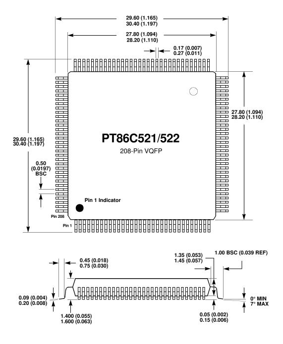
Figure A-1. 208-Pin VQFP Package Dimensions
