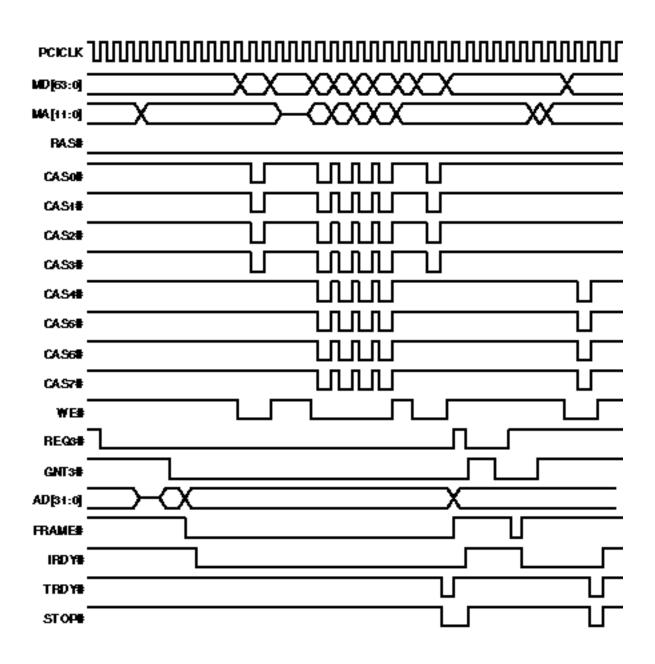
Figure 5-35. PCI Bus Master Write to 64-bit DRAM (L1 write-back)
