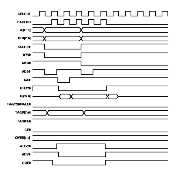
Figure 5-13. L2 Cache – Pipeline Synchronous Burst Read Hit
