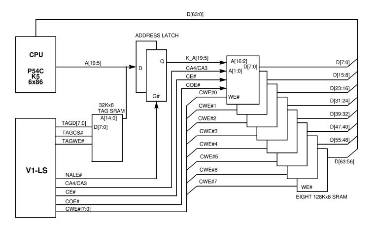
**NOTE:** TAGCS# and NALE# are multiplexed on a single pin. If NALE# function is used with asynchronous SRAM, the CS# of TAG SRAM should be connected to ground.
