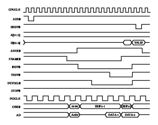
Figure 5-5. CPU-to-PCI Memory Burst Read Cycle
