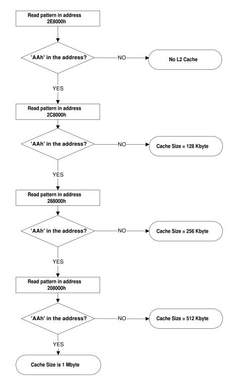
Figure D-4. Sequence for Testing Cache Size
