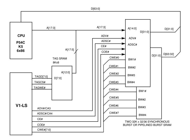
Figure 3-7. 256 Kbyte L2 Cache Using Two 32K X 32/36 Synchronous or Pipelined Burst SRAM
