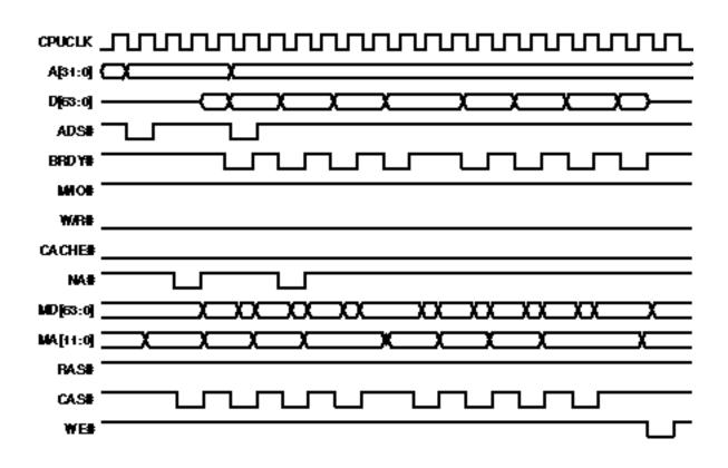
Figure 5-31. EDO Pipelined Burst Read (5-2-2-3-2-2-2)
