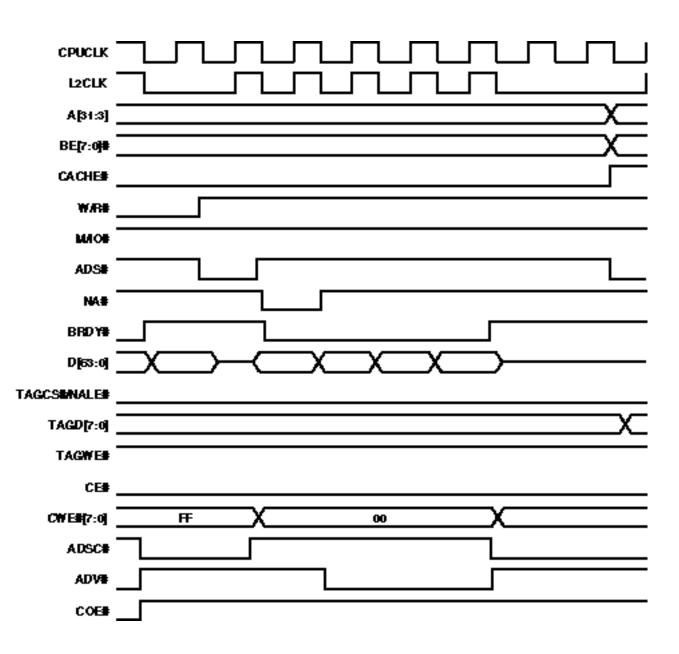
Figure 5-16. L2 Cache Write Burst Hit
