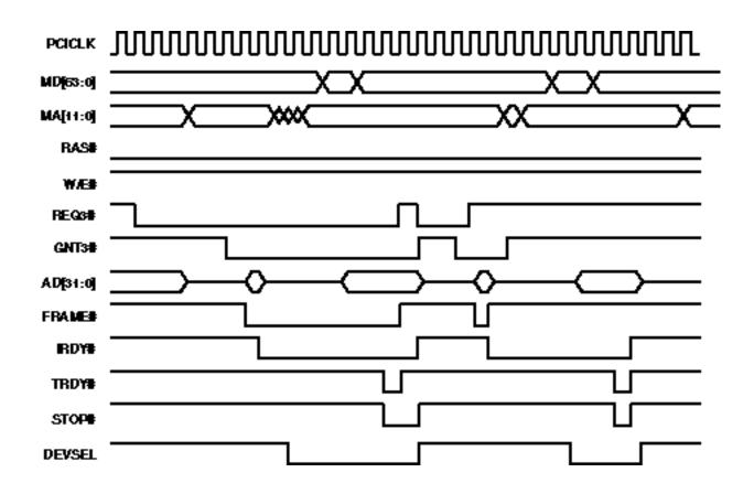
Figure 5-33. PCI Bus Master Read From 64-bit DRAM (no L1 cache hit)
