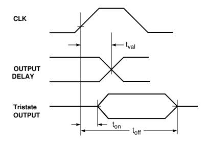
Figure 5-1. Output Timing Measurement Conditions
