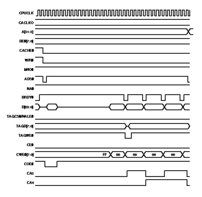
Figure 5-21. L2 Cache – Asynchronous, Burst Read Miss
