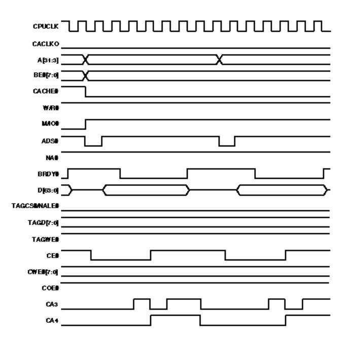
Figure 5-23. L2 Cache – Asynchronous, Burst Write Miss, Write Buffer Empty
