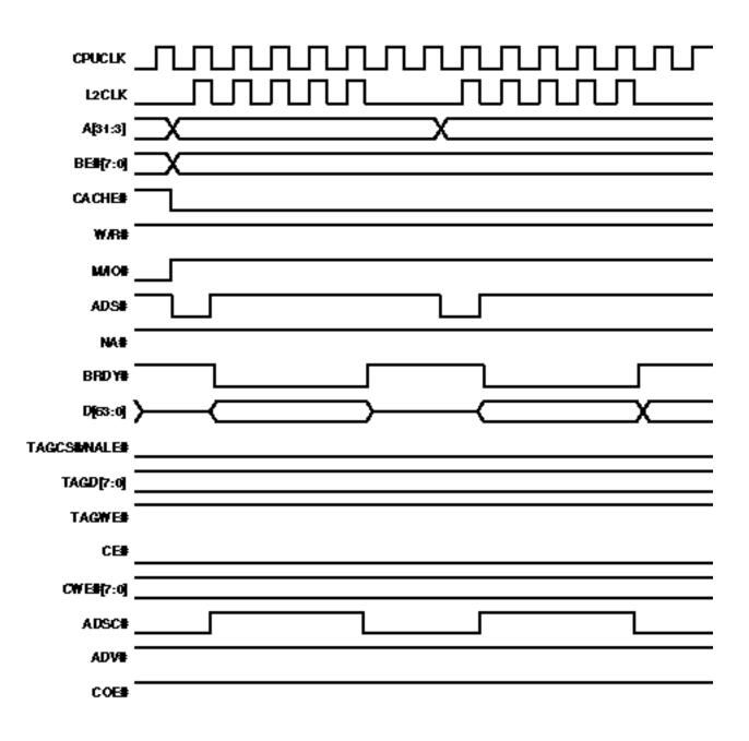
Figure 5-17. L2 Cache Write Burst Miss With Empty Write Buffer
