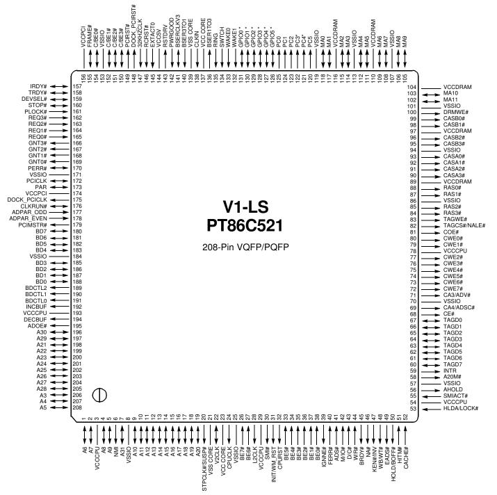
**NOTE:** Multiplexed GPIO and PC signals are shown with an asterisk (\*). Refer to Section 4.4.60 on page 1-193 for additional details on the multiplexing scheme.
