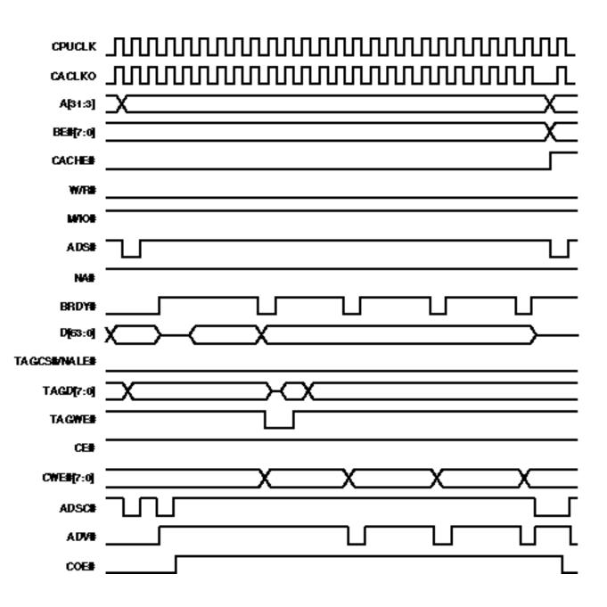
Figure 5-14. L2 Cache – Pipeline Synchronous Read Miss
