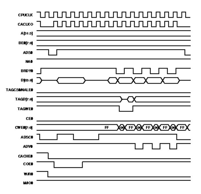
Figure 5-15. L2 Cache – Synchronous Burst Read Miss
