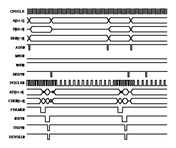
Figure 5-10. PicoPower PCICLK Control Scheme
