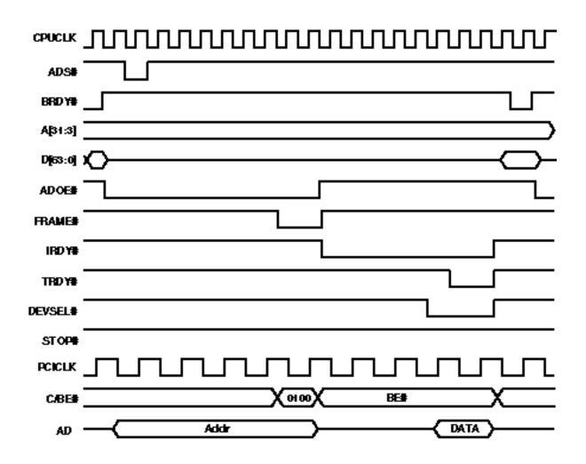
Figure 5-8. CPU-to-PCI I/O Read Cycle
