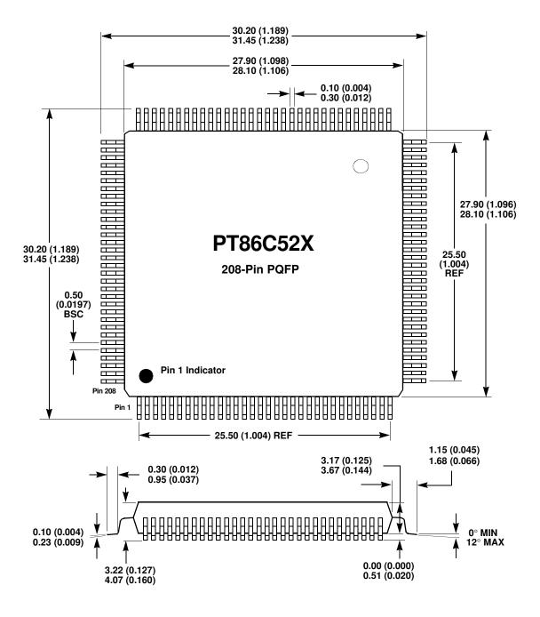
Figure A-2. 208-Pin PQFP Package Dimensions
