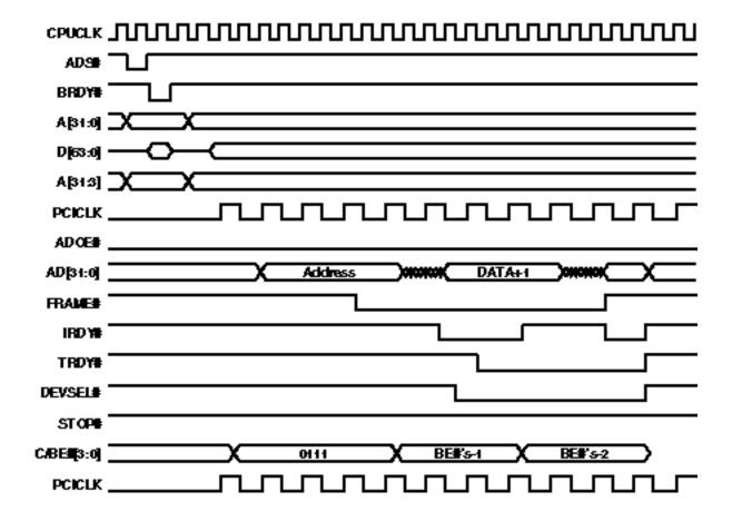
Figure 5-7. CPU-to-PCI Memory Write Cycle
