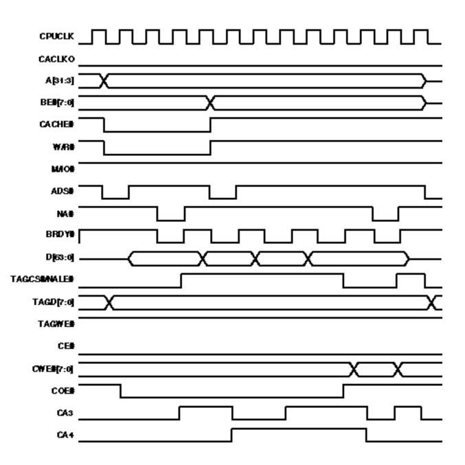
Figure 5-20. L2 Cache – Asynchronous, Burst Read 3-2-2-2 Hit
