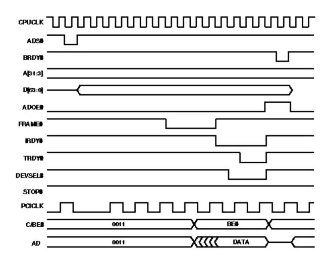
Figure 5-9. CPU-to-PCI I/O Write Cycle
