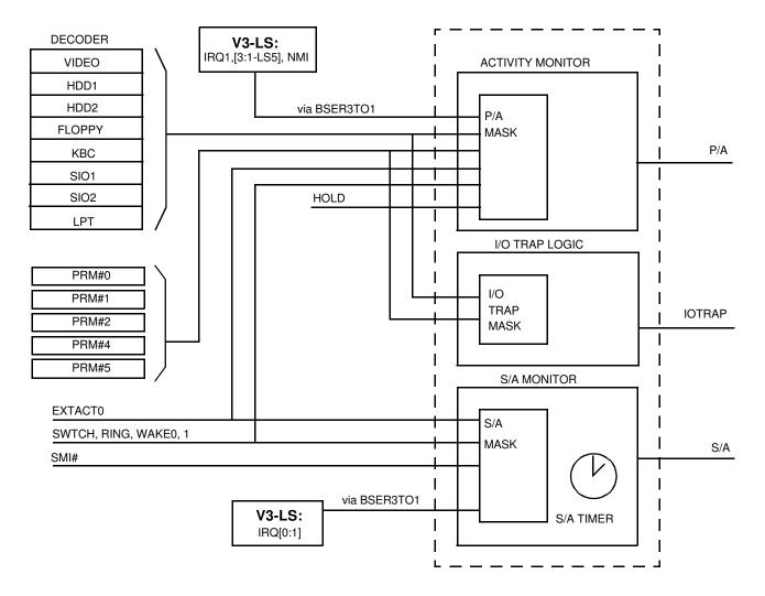
Figure 3-11. Generation of P/A, S/A, and I/O Trap
