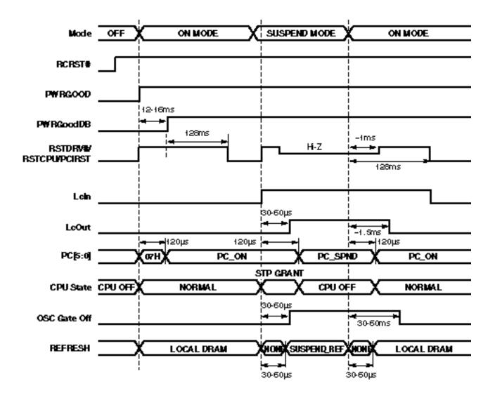
Figure 5-3. Power-On/5-V Suspend Timing Diagram
