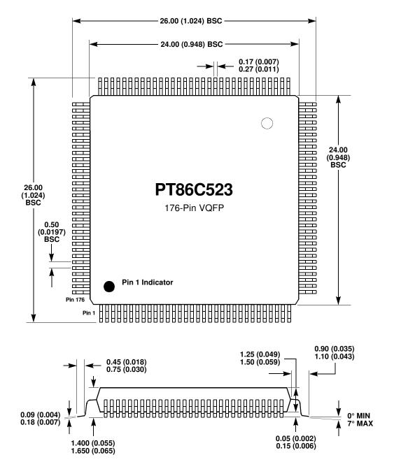
Figure A-3. 176-Pin VQFP Package Dimensions
