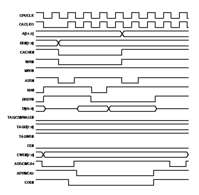
Figure 5-11. L2 Cache – Pipeline Synchronous, Single Read Hit
