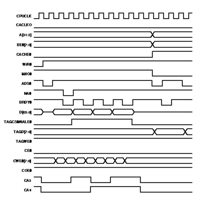
Figure 5-22. L2 Cache – Burst Write 3-2-2-2 Hit
