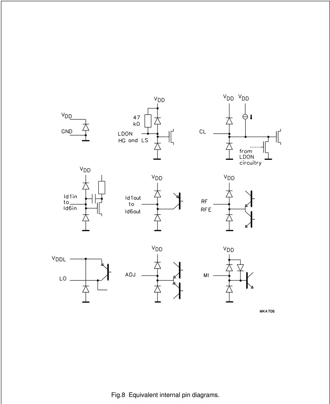
Fig.8 Equivalent internal pin diagrams.
