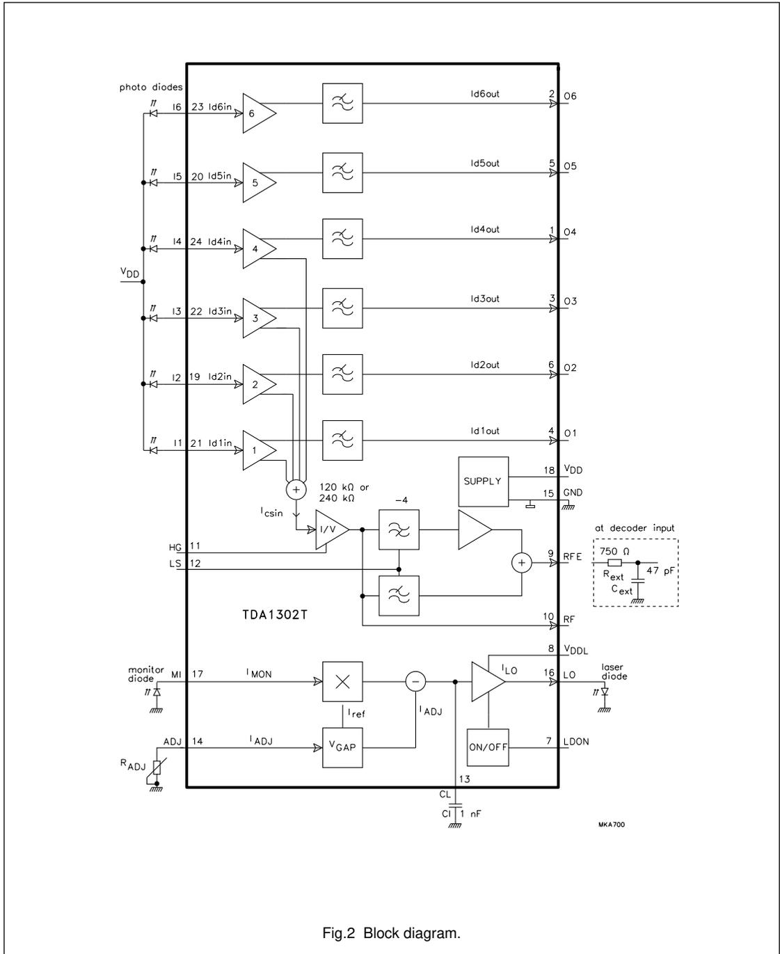
Fig.2 Block diagram.
