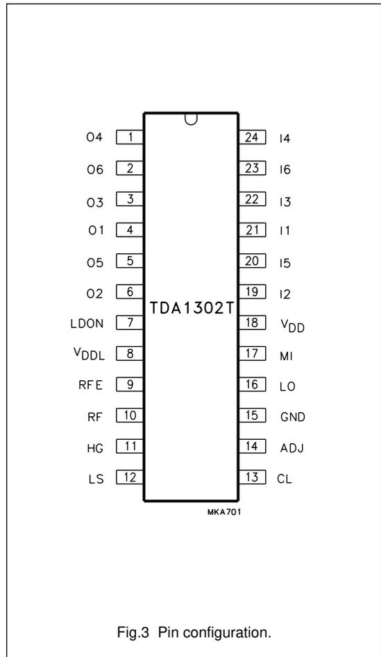
Fig.3 Pin configuration.
