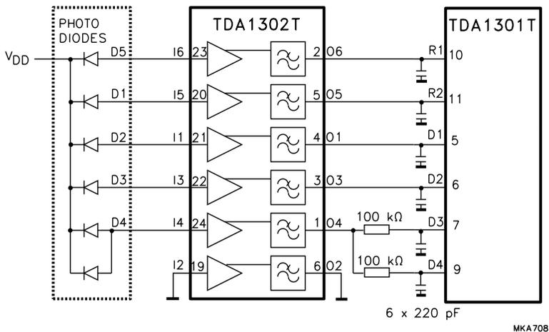
Fig.10 Application of the CDM12 pick-up unit.
