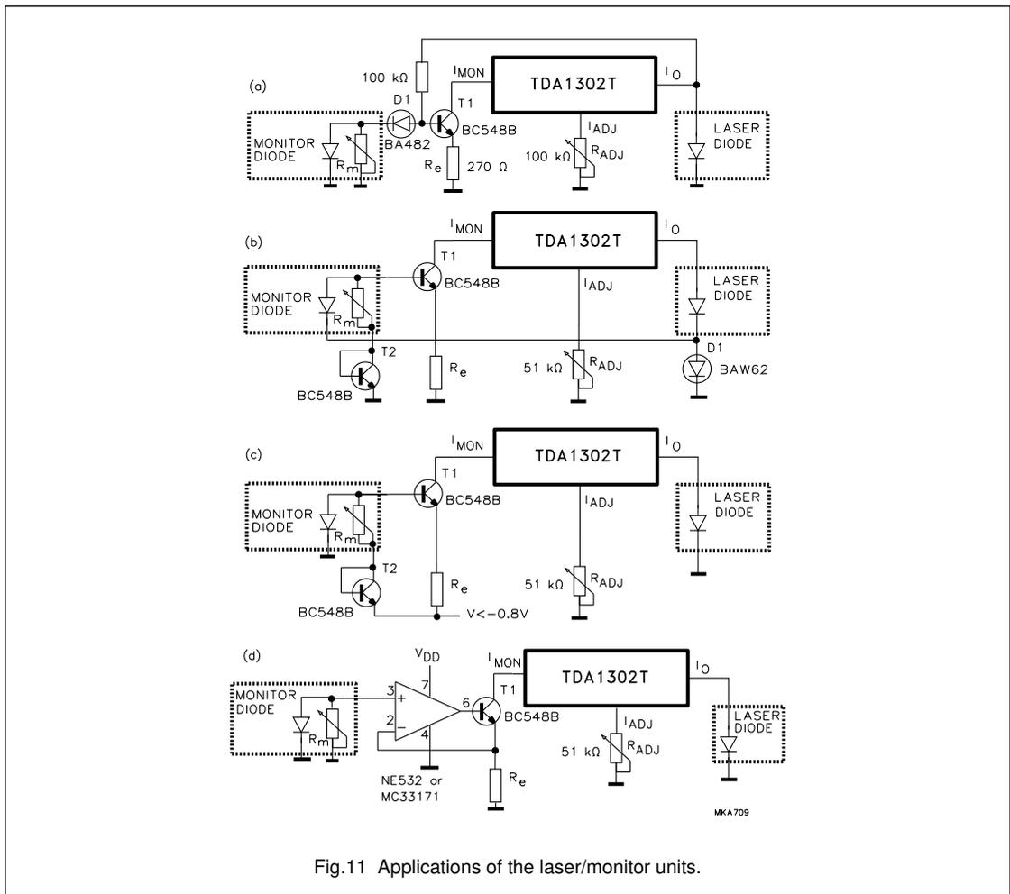
Fig.11 Applications of the laser/monitor units.
