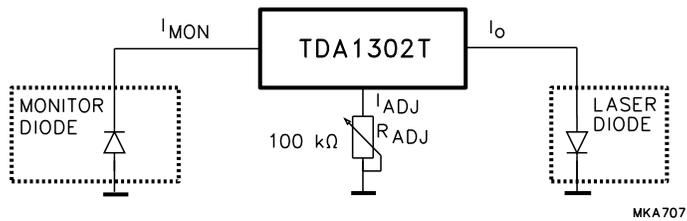
Fig.9 Application of the CDM12 laser/monitor diode unit.
