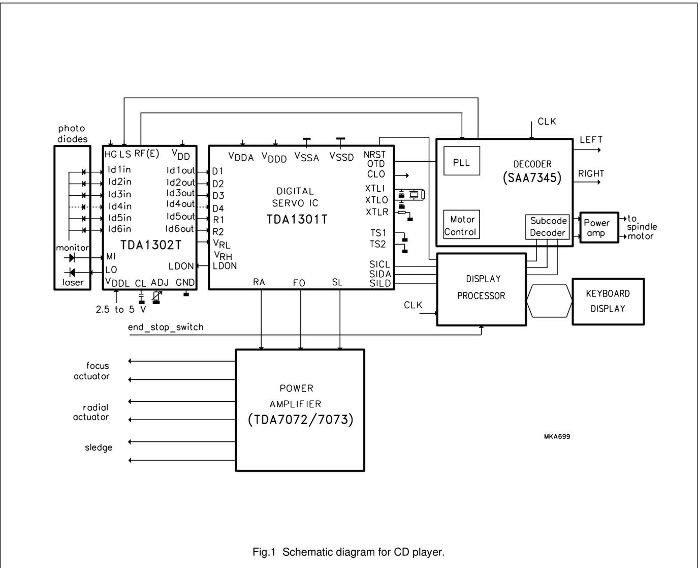
Fig.1 Schematic diagram for CD player.
