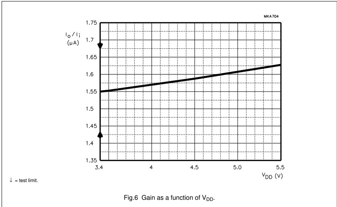
Fig.6 Gain as a function of V<sub>DD</sub>.
