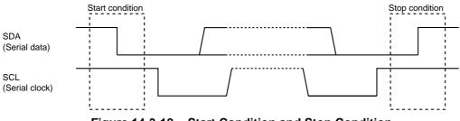
Figure 14-3-12 Start Condition and Stop Condition
