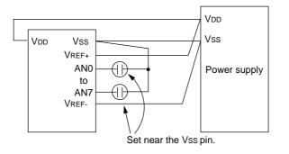
Figure 16-3-3 A/D Converter Recommended Example 2
