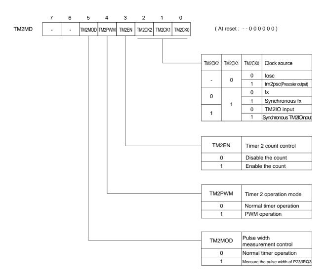
Figure 6-2-13 Timer 2 Mode Register (TM2MD : x'03F5C', R/W)
