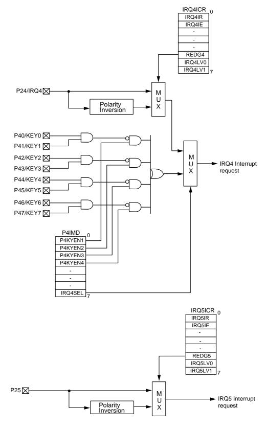
External Interrupt 4 Interface, External Interrupt 5 Interface, Block Diagram
