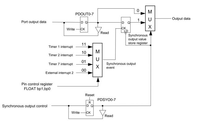
Figure 4-15-1 Synchronous Output Control Block Diagram
