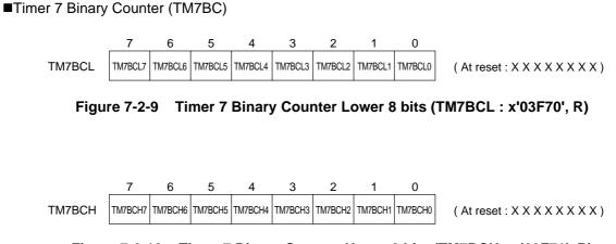
Figure 7-2-10 Timer 7 Binary Counter Upper 8 bits (TM7BCH : x'03F71', R)
