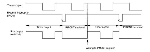
Figure 4-14-1 Real Time Output Control Timing
