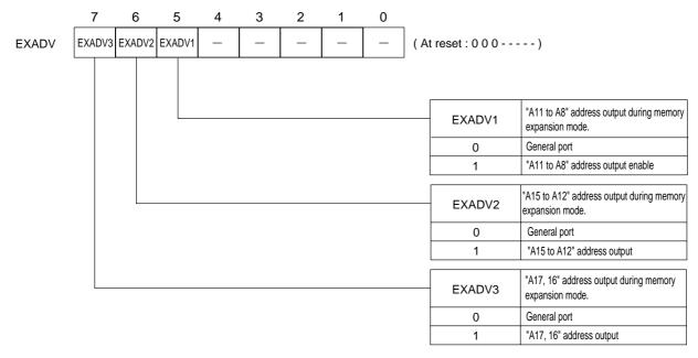
Address output control register (EXADV : x'03F0E', R/W)
