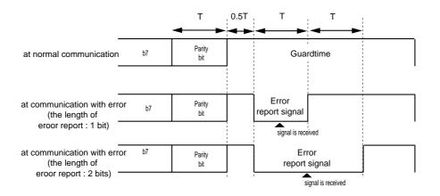
Figure 12-3-20 Report Timing of Communication Error Signal
