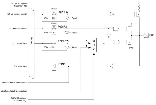
Figure 4-2-7 Block Diagram (P05)
