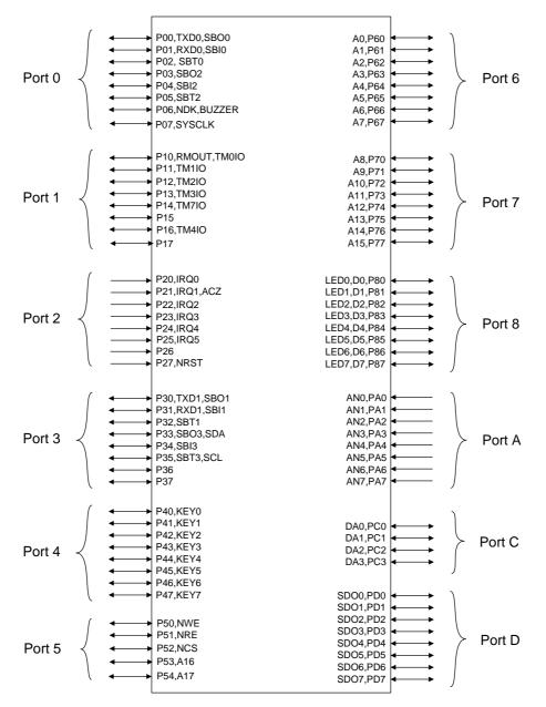
Figure 4-1-1 I/O Port Functions
