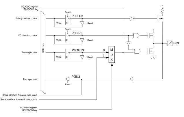
Figure 4-2-5 Block diagram (P03)
