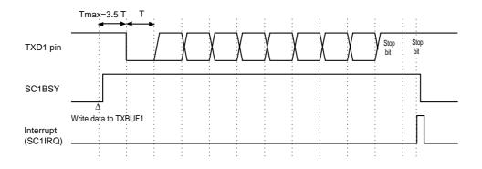
Figure 12-3-16 Transmission Timing (parity bit is disabled)
