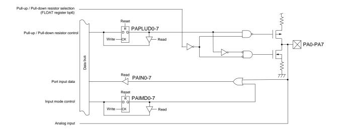
Figure 4-11-3 Block Diagram (PA0 to PA7)
