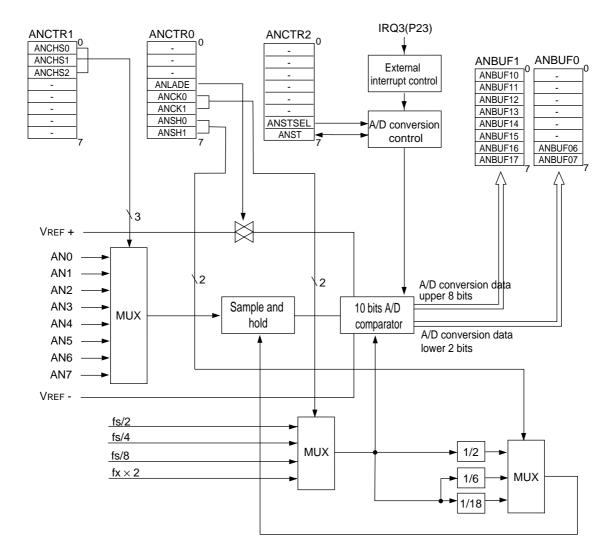
Figure 16-1-1 A/D Converter Block Diagram
