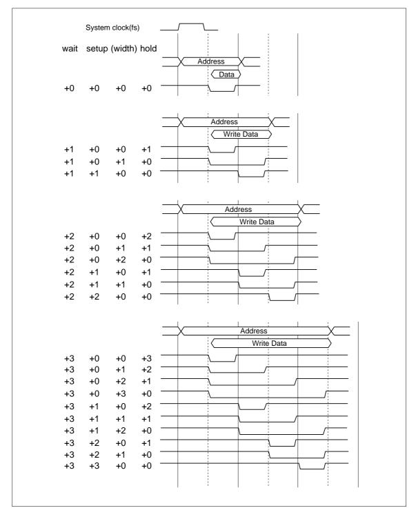
Figure 18-2-1 AC Timing Features of Data Strobe Signal
