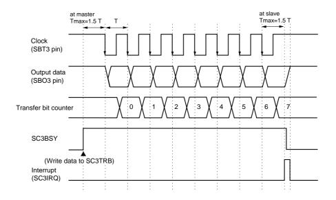
Figure 14-3-3 Transmission Timing (Falling edge, Disable Start Condition)
