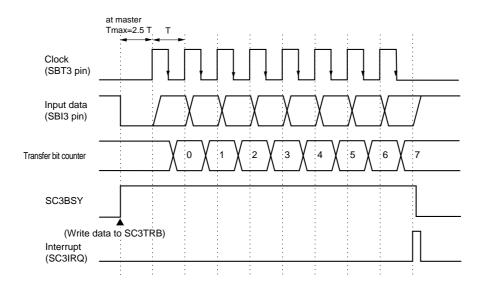
Figure 14-3-8 Reception Timing (Falling edge, Enable Start Condition)
