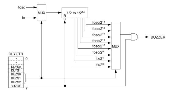
Figure 10-1-1 Block Diagram (Buzzer)
