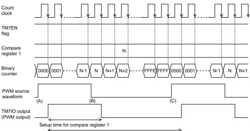
PWM basic component (overflow time of the binary counter)
