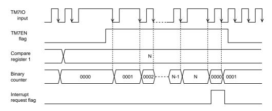
Figure 7-4-1 Count Timing TM7IO Input (Timer 7)
