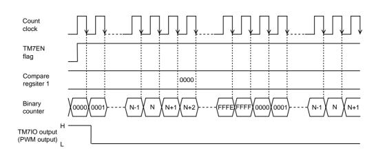
■Count Timing of Standard PWM Output (when Compare Register 1 is x'0000')(Timer 7) Here is the count timing at setting x'0000' to the compare register 1.
