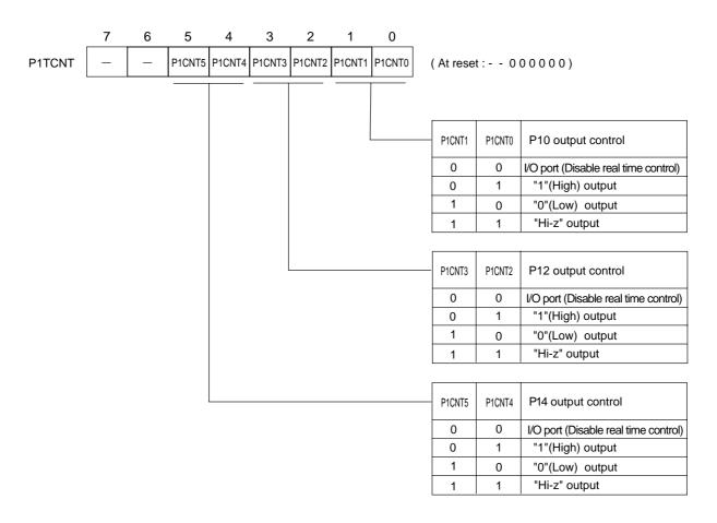
Port 1 output control register (P1TCNT : x'03F7E', R/W)
