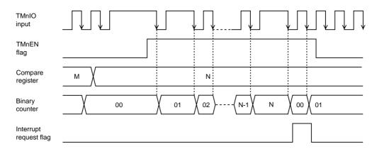
Figure 6-4-1 Count Timing of TMnIO Input (Timers 0 to 4)
