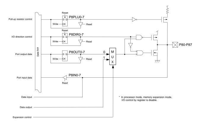
Figure 4-10-2 Block Diagram (P80 to P87)
