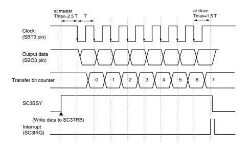
Figure 14-3-2 Transmission Timing (Falling edge, Enable Start Condition)
