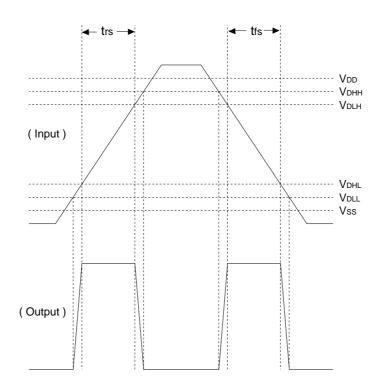
Figure 1-5-5 AC Zero-Cross Detector
