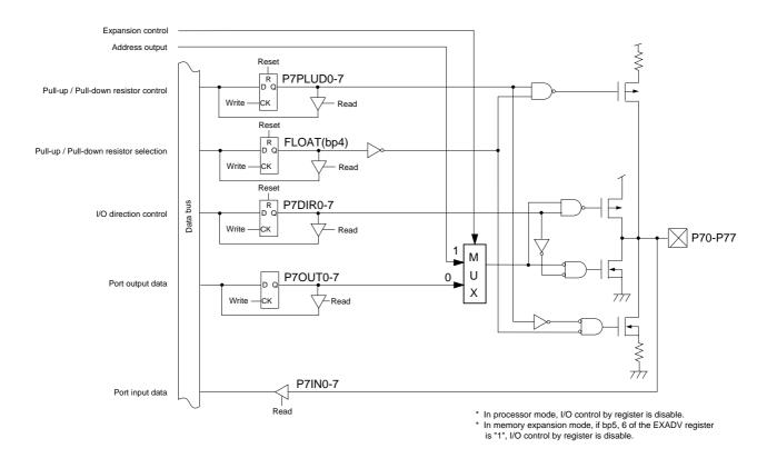
Figure 4-9-3 Block Diagram (P70 to P77)
