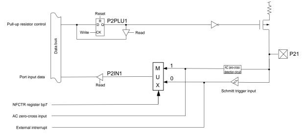
Figure 4-4-3 Block Diagram (P21)
