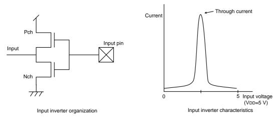
Figure 1-7-2 Input Inverter Organization and Characteristics
