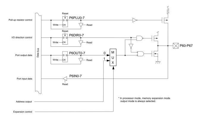
Figure 4-8-2 Block Diagram (P60 to P67)
