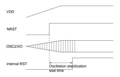
Figure 2-8-2 Reset Released Sequence
