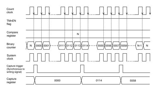
Figure 7-9-2 Capture Count Timing with a Writing Signal to Program as a Trigger (Timer 7)
