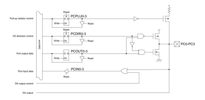
Figure 4-12-2 Block Diagram (PC0 to PC3)
