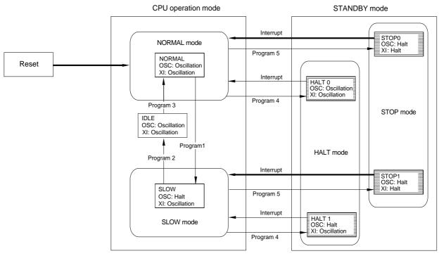
:CPU halt -: Wait period for oscillation stabilization is inserted OSC: High-frequency oscillation clock XI: Low-frequency oscillation clock (32 kHz)
