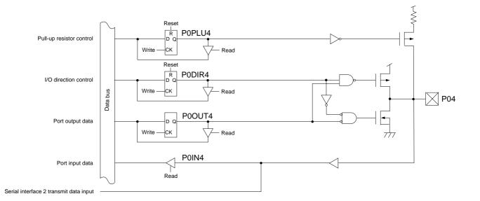
Figure 4-2-6 Block Diagram (P04)
