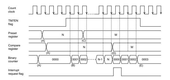
Figure 7-3-1 Count Timing of Timer Operation (Timer 7)
