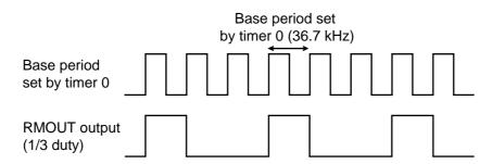
Figure 6-11-3 Output Wave Form of RMOUT Output Pin
