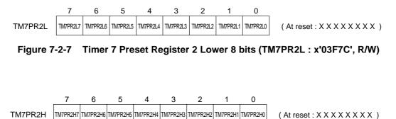
Figure 7-2-8 Timer 7 Preset Register 2 Upper 8 bits (TM7PR2H : x'03F7D', R/W)
