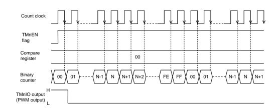
■Count Timing of PWM Output (when the compare register is x'00') (Timers 0, 2 and 4) Here is the count timing when the compare register is set to x'00';
