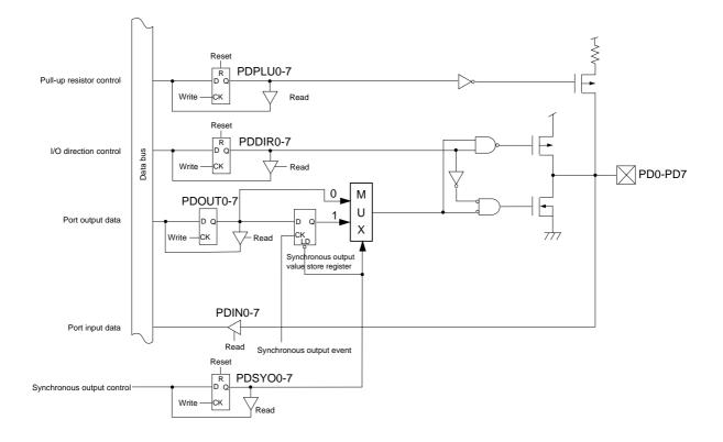
Figure 4-13-3 Block Diagram (PD0 to PD7)
