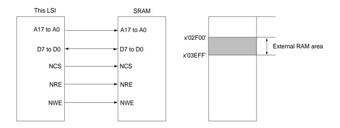
Figure 2-3-7 SRAM Connection Example
