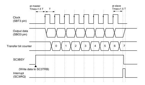
Figure 14-3-5 Transmission Timing (Rising edge, Disable Start Condition)
