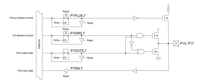
Figure 4-3-6 Block Diagram (P15, P17)
