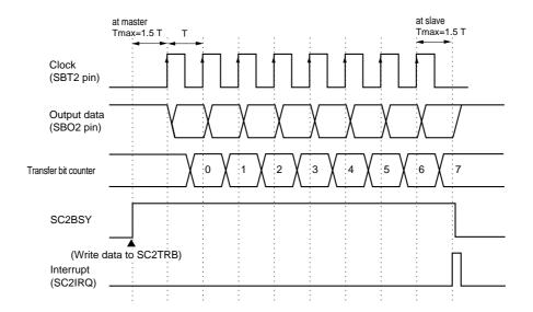
Figure 13-3-5 Transmission Timing (Rising edge, Start condition is disabled)
