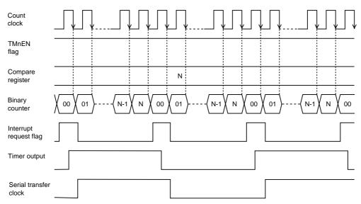
Figure 6-8-1 Timing of Serial Interface Transfer Clock (Timers 2, 3 and 4)
