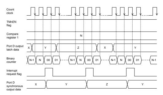
Figure 6-7-1 Count Timing of Synchronous Output (Timer 1, Timer2)
