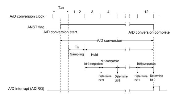
Figure 16-3-1 Operation of A/D Conversion
