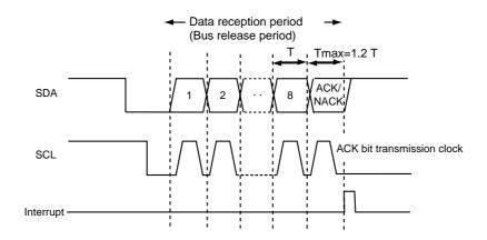
Figure 14-3-14 ACK Bit Transmission Timing after Reception of 8-bit Data
