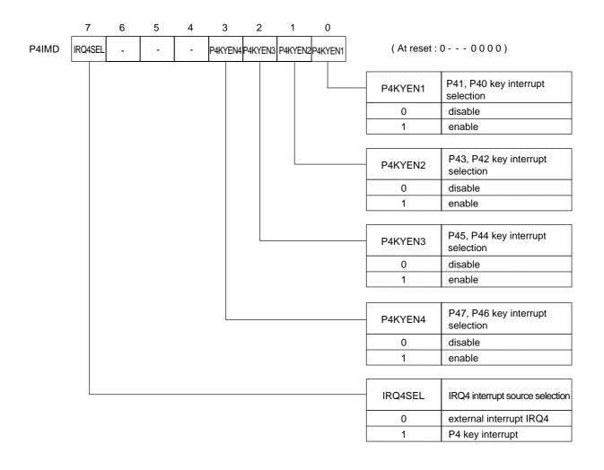
Figure 3-3-6 Port 4 Key Interrupt Control Register (P4IMD : x'03F3E', R/W)
