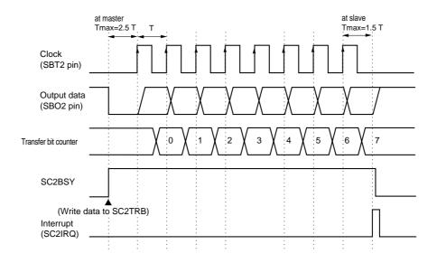
Figure 13-3-4 Transmission Timing (Rising edge, Start condition is enabled)
