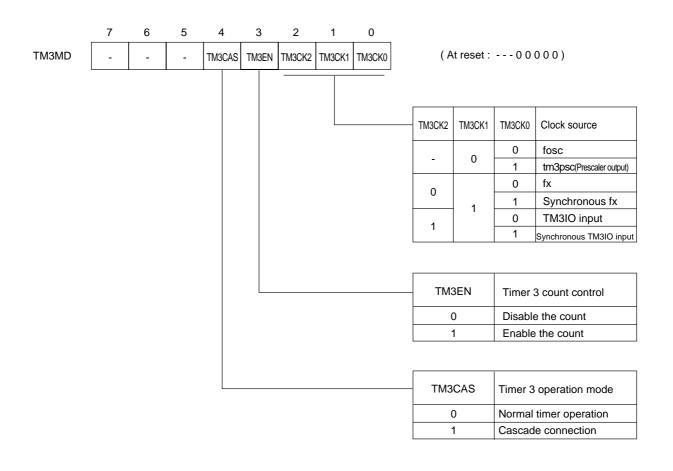
Figure 6-2-14 Timer 3 Mode Register (TM3MD : x'03F5D', R/W)
