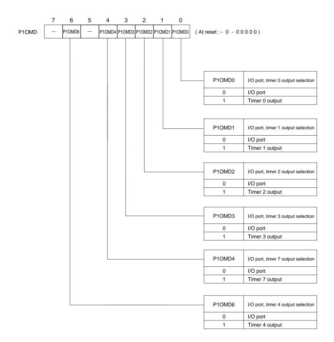
Port 1 output mode register (P1OMD : x'03F2F', R/W)
