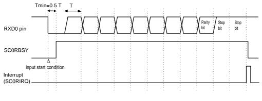
Figure 11-3-22 Reception Timing (parity bit is enabled)
