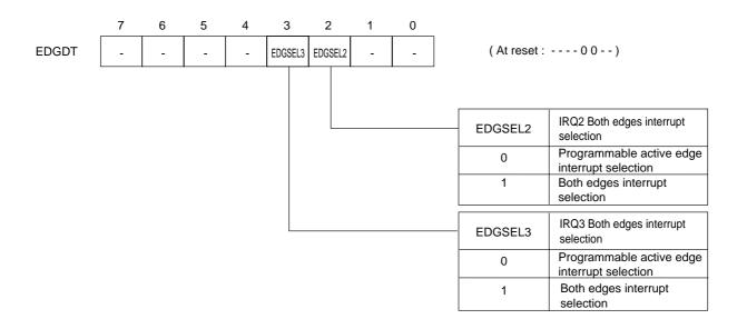
Figure 3-3-5 Both Edges Interrupt Control Register (EDGDT : x'03F8F', R/W)
