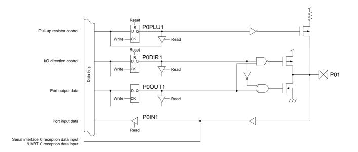
Figure 4-2-3 Block diagram (P01)
