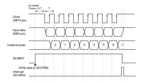
Figure 14-3-7 Reception Timing (Rising edge, Disable Start Condition)
