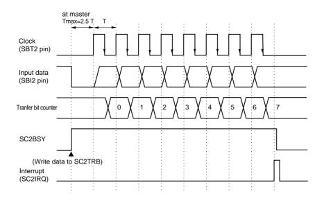
Figure 13-3-8 Reception Timing (Falling edge, Start condition is enabled)
