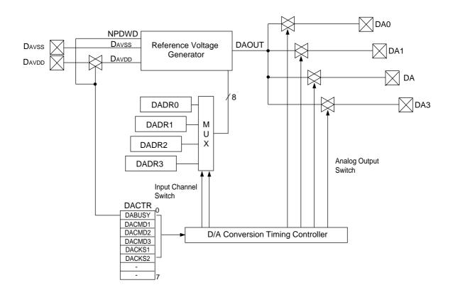
Figure 17-1-1 D/A Converter Block Diagram
