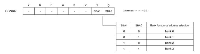
Figure 2-6-1 Bank Register for Source Address (SBNKR:x'03F0A', R/W)
