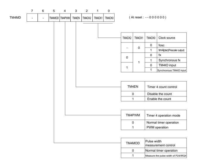
Figure 6-2-15 Timer 4 Mode Register (TM4MD : x'03F64', R/W)
