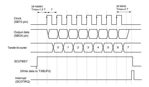
Figure 11-3-8 Transmission Timing (rising edge, start condition is disabled)
