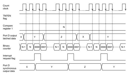
Count Timing of Synchronous Output (Timer 7)
