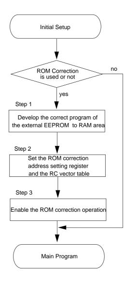
Figure 2-7-12 Initial Routine for ROM Correction
