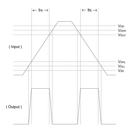
Figure 20-3-5 AC Zero-Cross Detector
