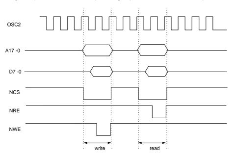
Figure 2-3-4 ROM and RAM Access Timing with No Wait Cycles
