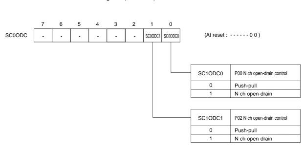
■Serial Interface 0 Port Control Register (SC0ODC)
