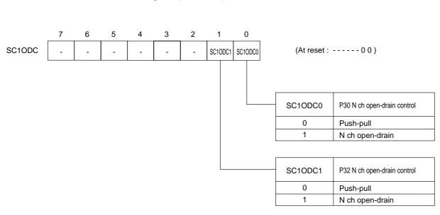
■Serial Interface 1 Port Control Register (SC1ODC)
