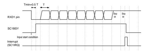
Figure 12-3-18 Reception Timing (parity bit is disabled)
