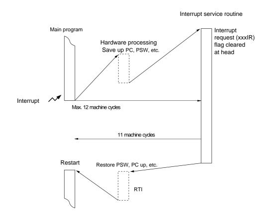
Figure 3-1-2 Interrupt Processing Sequence (maskable interrupts)
