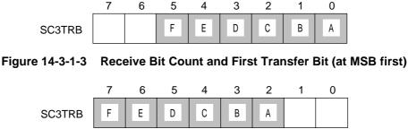
Figure 14-3-1-4 Receive Bit Count and First Transfer Bit (at LSB first)
