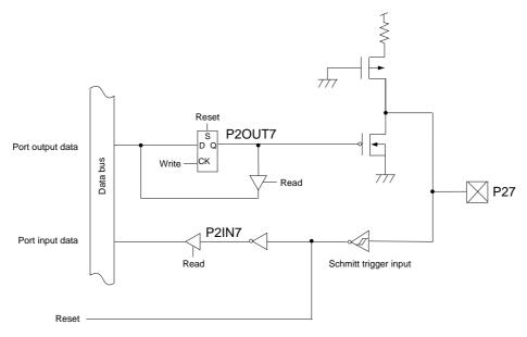
Figure 4-4-4 Block Diagram (P27)
