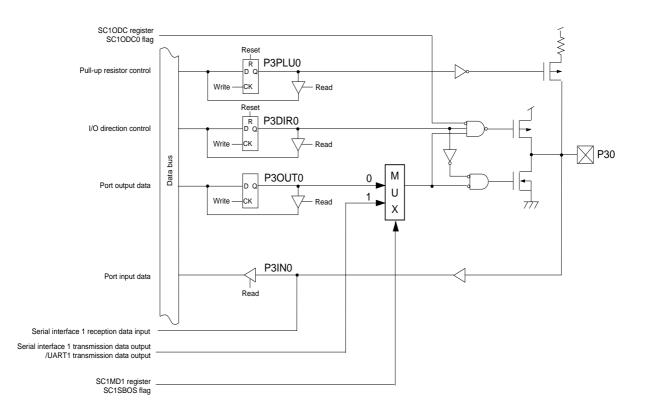
Figure 4-5-2 Block Diagram (P30)
