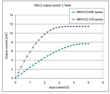
Figure 19-2-1 MN101C49K OSC2 pin's output current
