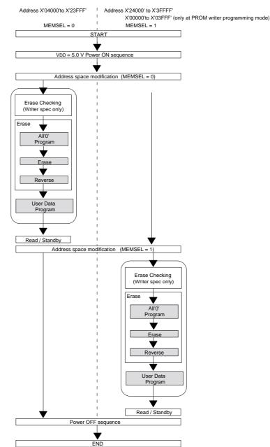
Figure 20-4-1 Reprogramming Flow of Internal Flash EEPROM
