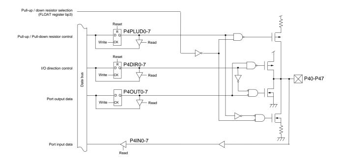
Figure 4-6-3 Block Diagram (P40 to P47)
