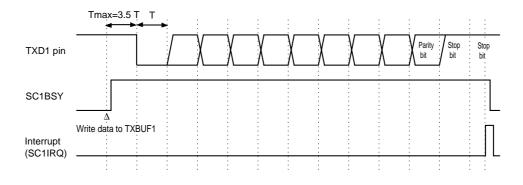
Figure 12-3-15 Transmission Timing (parity bit is enabled)
