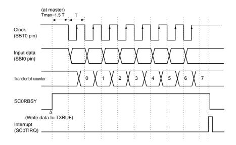
Figure 11-3-10 Reception Timing (rising edge, start condition is disabled)
