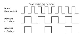
Figure 6-11-1 Duty Cycle of Remote Control Carrier Output Signal
