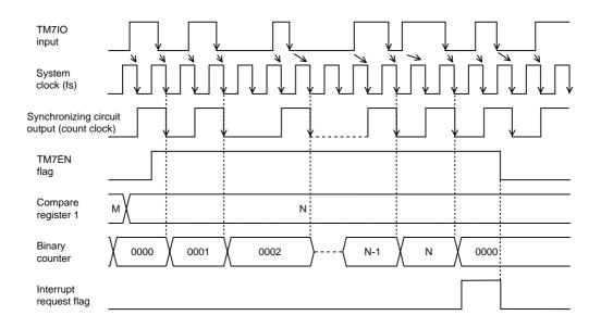
Figure 7-4-2 Count Timing of Synchronous TM7IO Input (Timer 7)
