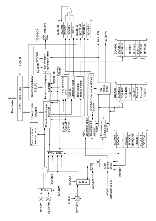
Figure 11-1-1 Serial Interface 0 Block Diagram
