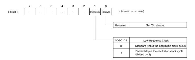
Figure 2-5-1 Oscillator Frequency Control Register (OSCMD : x'03F0D', R/W)
