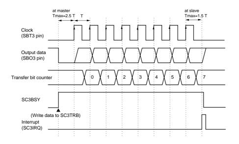
Figure 14-3-4 Transmission Timing (Rising edge, Enable Start Condition)
