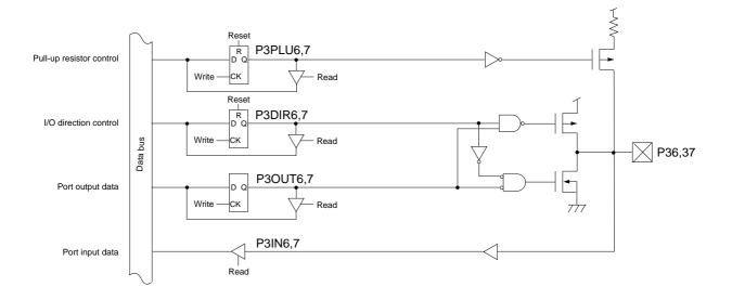
Figure 4-5-8 Block Diagram (P36,37)
