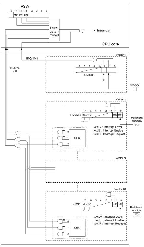
Figure 3-1-1 Interrupt Block Diagram
