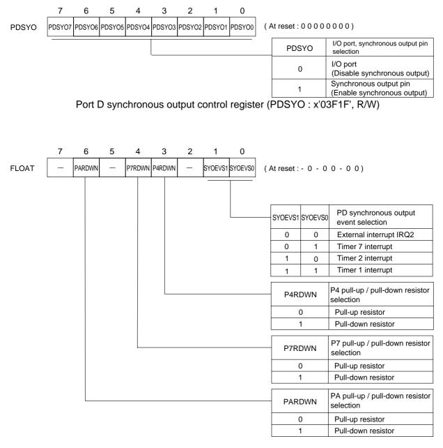
Pull-up / Pull-down resistor selection, pin control register (FLOAT : x'03F2E', R/W)
