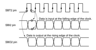
Figure 13-3-11 Transmission / Reception Timing (Reception : Falling edge, Transmission : Rising edge)
