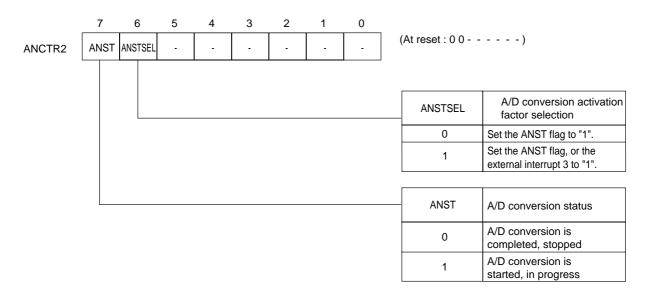
Figure 16-2-3 A/D Converter Control Register 2 (ANCTR2 : x'03FB2', R/W)
