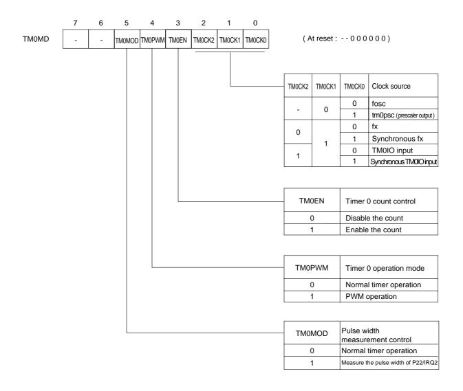
Figure 6-2-11 Timer 0 Mode Register (TM0MD : x'03F54', R/W)
