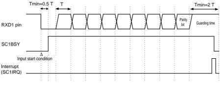
Figure 12-3-23 Reception Timing (T=0, 1 Data Communication)
