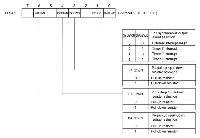
Pull-up / Pull-down resistor selection, Pin control register (FLOAT : x'03F2E', R/W)
