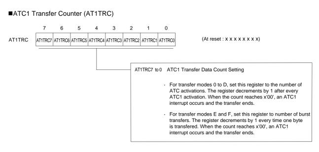
Figure 15-2-3 ATC1 Transfer Data Counter (AT1TRC : x'03FD2', R/W)
