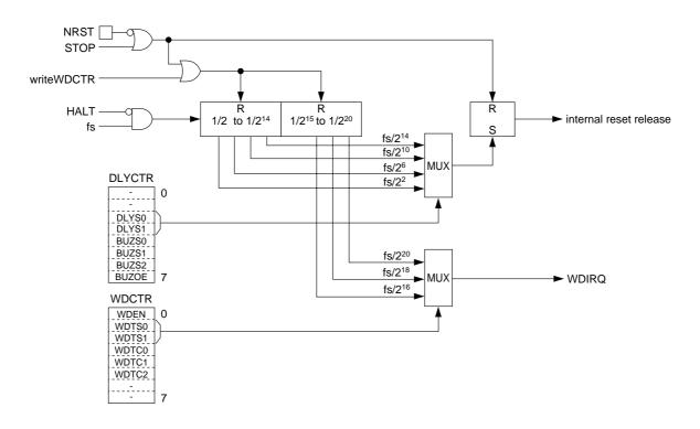
Figure 9-1-1 Block Diagram (Watchdog Timer)
