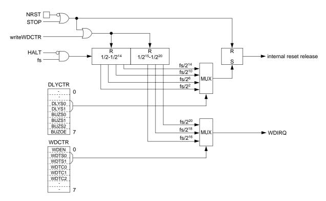
Block Diagram of Oscillation Stabilization Wait Time (watchdog timer)
