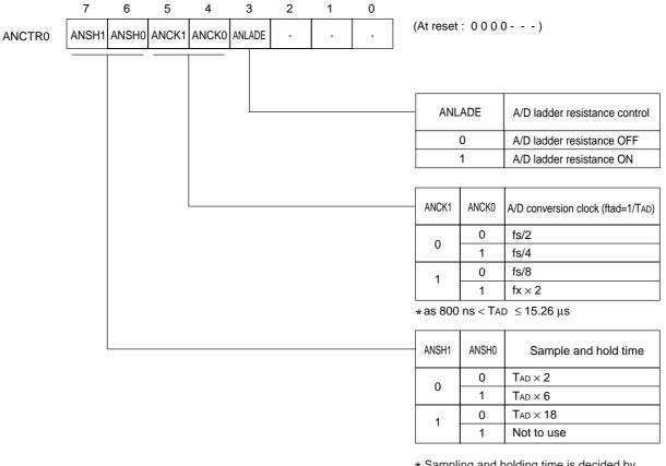
\* Sampling and holding time is decided by the input impedance at analog input.
