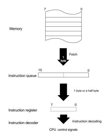
Figure 2-1-2 Instruction Execution Controller Configuration
