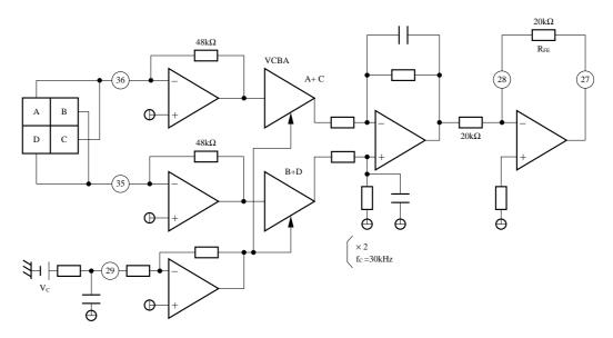
Figure 2 : Focus Error Amplifier
