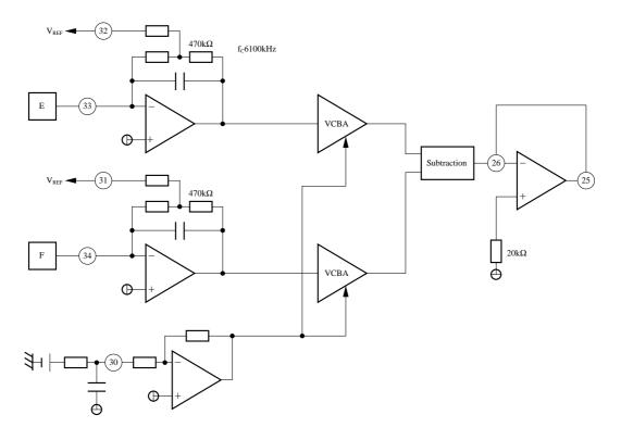
Figure 3: Tracking Error Amplifier
