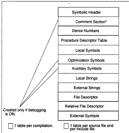
\* This section holds compacted form of relocation entries for Pixie. Currently only dynamically linked executables and shared objects have this section.
