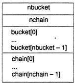
*nbucket* indicates the number of entries in the *bucket* array and *nchain* indicates the number of entries in the *chain* array. Both *bucket* and *chain* hold symbol table indexes; the entries in *chain* parallel the symbol table. The number of symbol table entries should be equal to *nchain*; symbol tables indexes also select *chain* entries.
