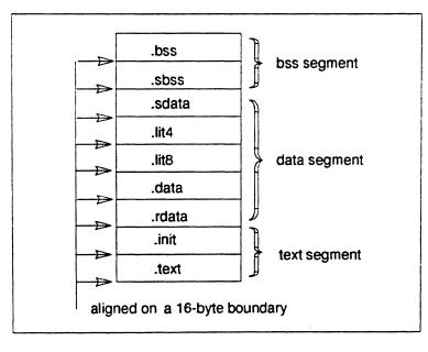
Figure 9.5: Layout of OMAGIC Files in Virtual Memory
