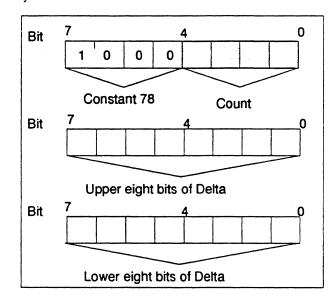
The layout of the extended field on disk is as follows:
