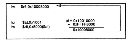
**Example 4:** Offset Reference—R\_GPREL. This example shows an assembly macro that loads a global pointer relative value *y* into Register 6:
