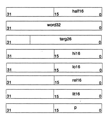
Calculations below assume the actions are transforming a relocatable file into either an executable or a shared object file. Conceptually, the linker merges one or more relocatable files to form the output. It first decides how to combine and locate the input files, then updates the symbol values, and finally performs the relocation.
