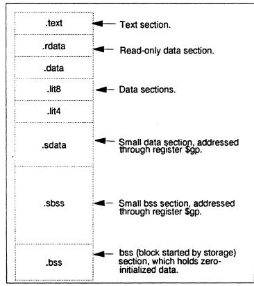
Assembled code and data fall in one of the sections shown in Figure 4.1.
