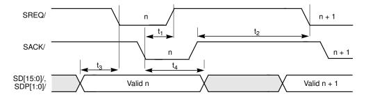
Table 7.22 Target Asynchronous Send
