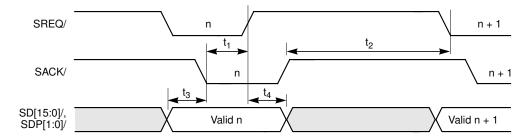
Figure 7.35 Initiator and Target Synchronous Transfer
