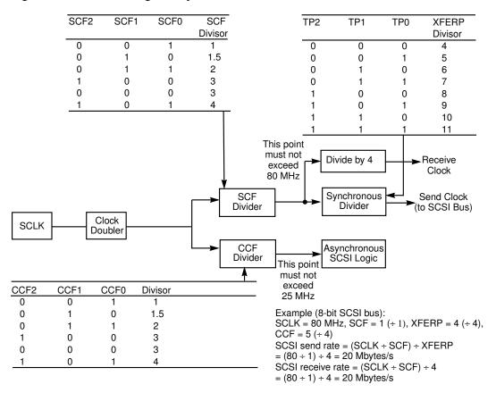
Figure 2.5 Determining the Synchronous Transfer Rate
