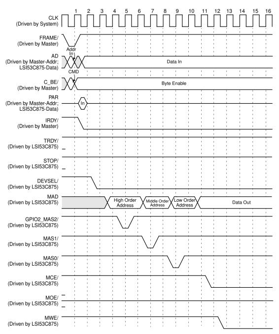
Figure 7.24 Write Cycle, Normal/Fast Memory (≥ 64 Kbyte), Multiple Byte Access (Cont.)
