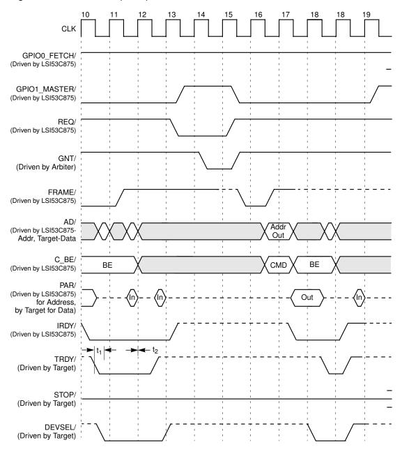
Figure 7.20 Burst Write
