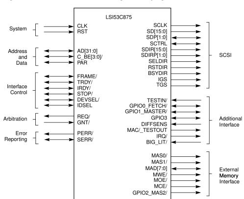
Figure 4.5 LSI53C875 Functional Signal Grouping
