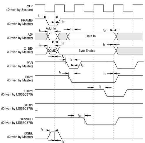
Figure 7.11 Operating Register/SCRIPTS RAM Read
