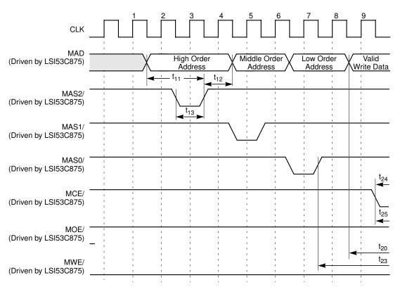
Figure 7.22 Write Cycle, Normal/Fast Memory (≥ 64 Kbytes), Single Byte Access (Cont.)
