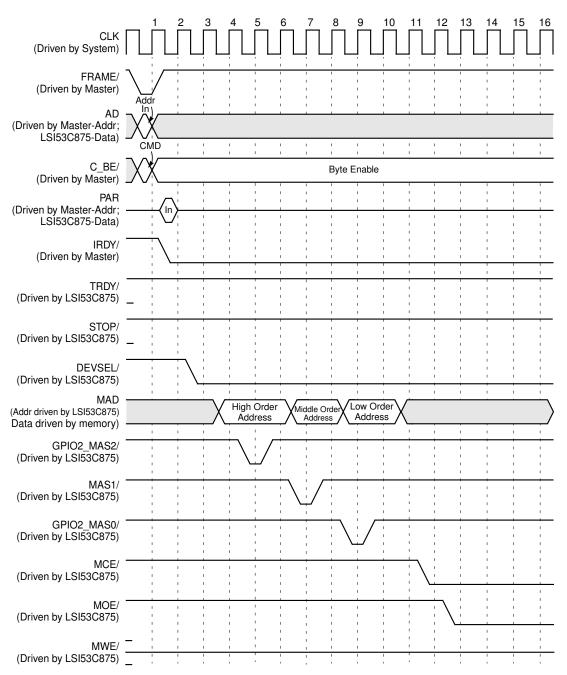
Figure 7.23 Read Cycle, Normal/Fast Memory (≥ 64 Kbyte), Multiple Byte Access (Cont.)
