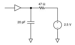
Figure 7.2 SCSI Input Filtering
