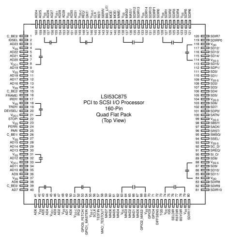
Note: The decoupling capacitor arrangement shown above is recommended to maximize the benefits of the internal split ground system. Capacitor values between 0.01 and 0.1  $\mu$ F should provide adequate noise isolation. Because of the number of high current drivers on the LSI53C875, a multilayer PC board with power and ground planes is required.
