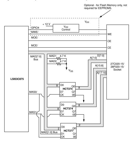
Note: MAD bus sense logic enabled for 256 Kbytes of fast memory (150 ns device @ 33 MHz). The HCT374s may be replaced with HCT377s.
