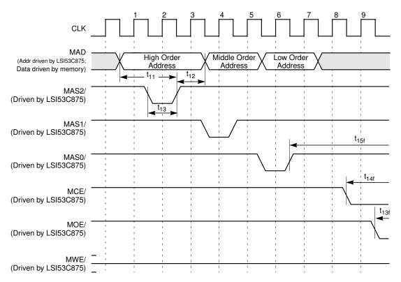
Figure 7.21 Read Cycle, Normal/Fast Memory (≥ 64 Kbytes), Single Byte Access (Cont.)
