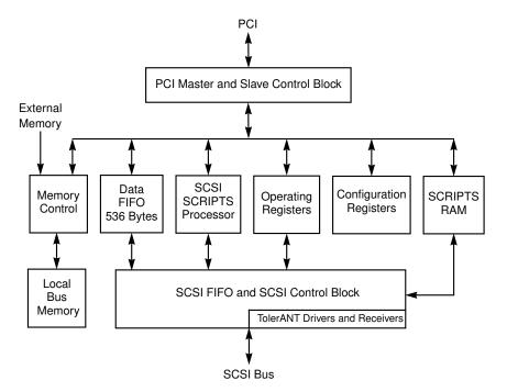
Figure 1.2 LSI53C875 Chip Block Diagram
