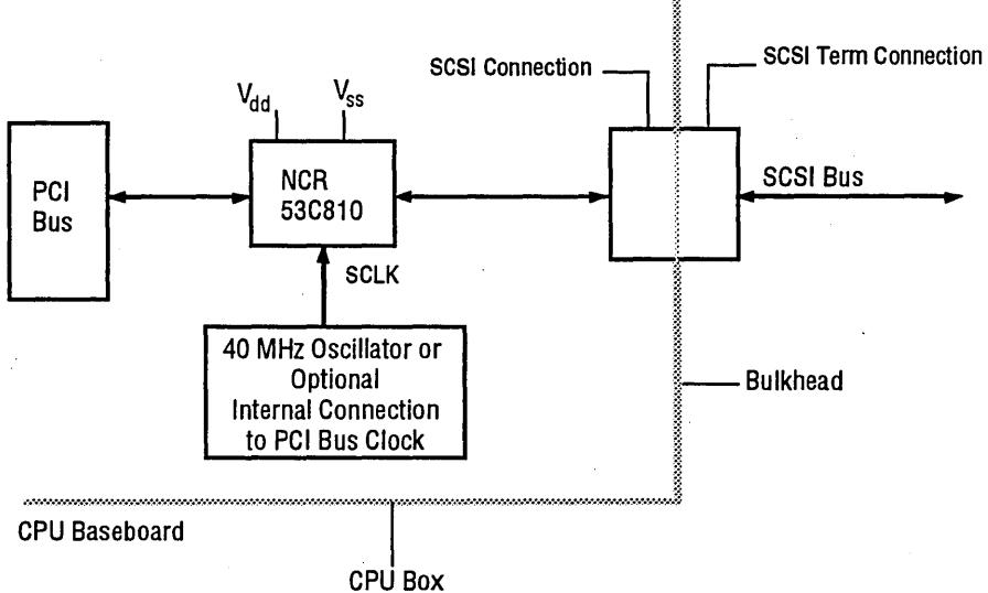
Figure 1-2. 53C810 Block Diagram
