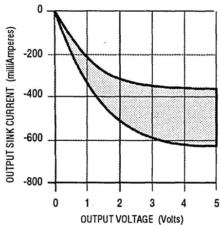
Output Source Current as a Function of Output Voltage ( $I_{OH}$ )
