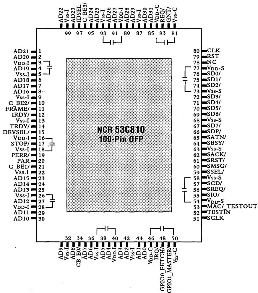
**Note:** The above decoupling capacitor arrangement shown is recommended to maximize the benefits of the internal split ground system. Capacitor values between 0.01 and 0.1 $\mu$ F should provide adequate noise isolation. Because of the number of high current drivers on the 53C810, a multi-layer PC board with power and ground planes is required.
