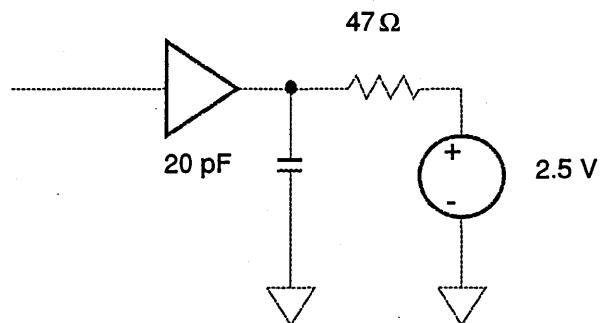
Figure 7-2. SCSI Input Filtering
