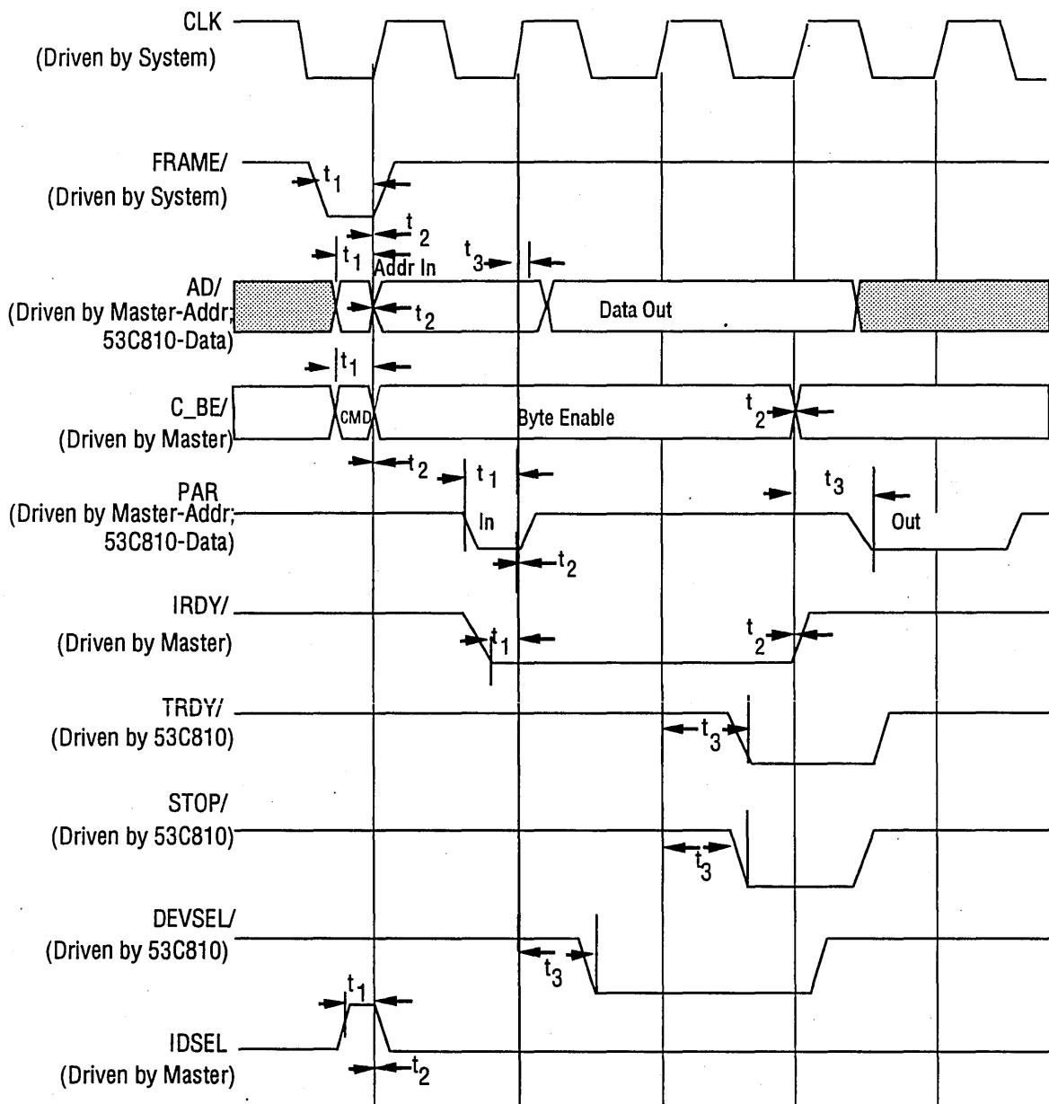
Figure 7-10. Configuration Register Write
