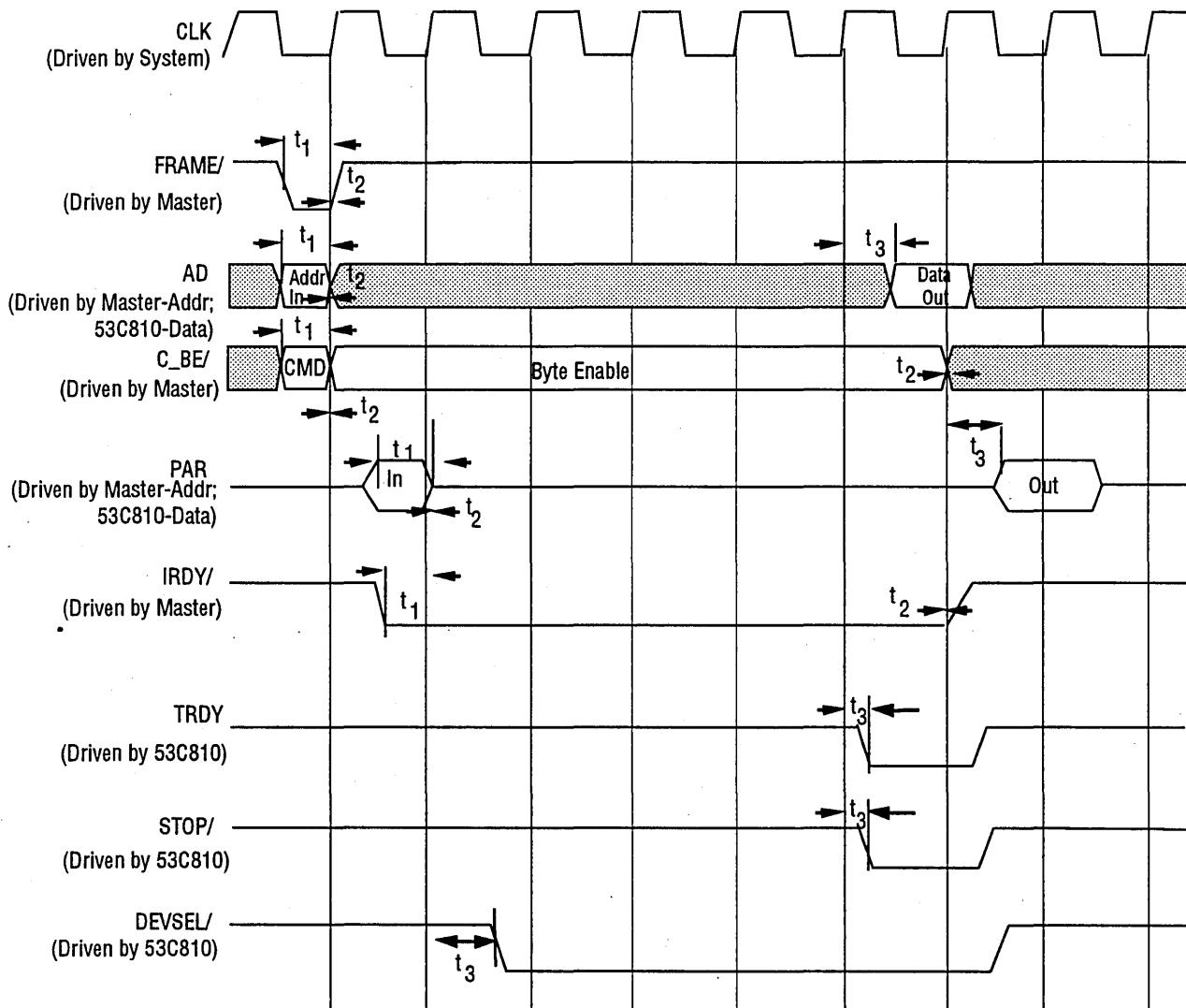
Figure 7-12. Target Write
