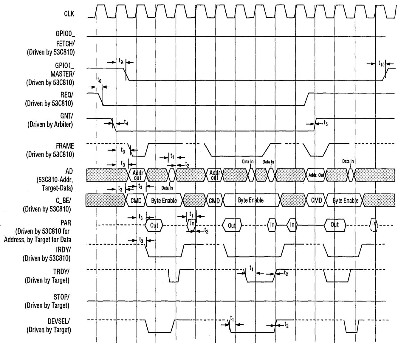
Figure 7-17. Burst Write
