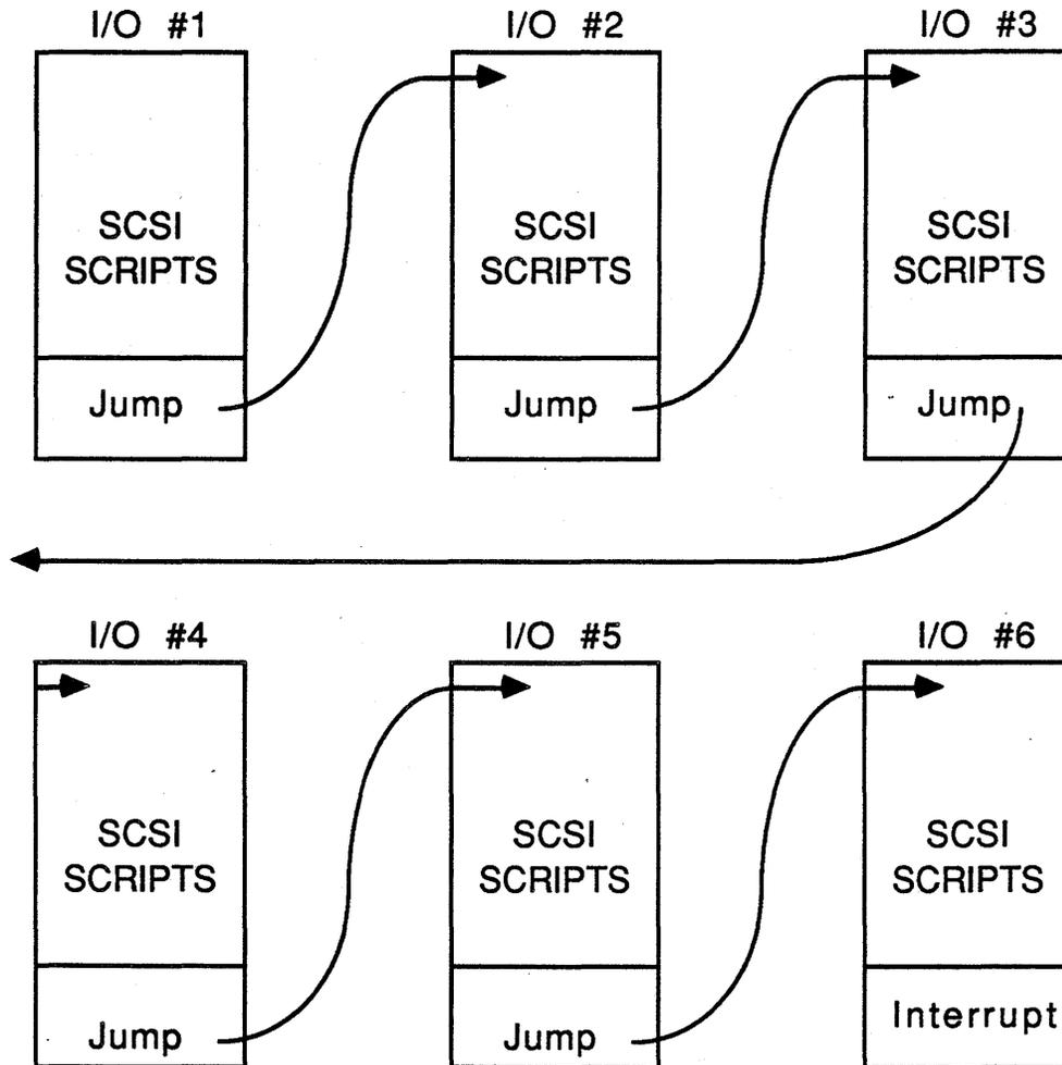
Figure 4. Using SCSI SCRIPTS to Implement Multi-Threaded I/O
