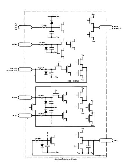
FIGURE 3. CROM Driver and Receiver Buffer
