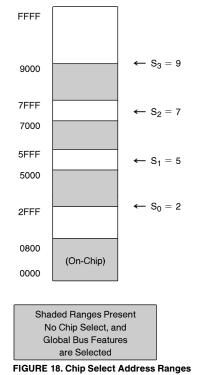
Chip Select 0 and Chip Select 3 can be programmed independently to operate with 1, 2 or 4 wait states. Chip Select 1 and 2 can be programmed independently to operate in native bus mode with 1, 2 or 4 wait states or slow peripheral bus mode.
