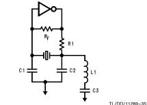
FIGURE 31. Recommended Overtone Crystal Circuit
