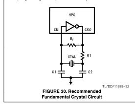
A recommended crystal oscillator circuit to be used with the HPC is shown in *Figure 30*. See table for recommended component values. The recommended values given in the table have yielded consistent results and are made to match a crystal with a 18 pF load capacitance, with some small allowance for layout capacitance.
