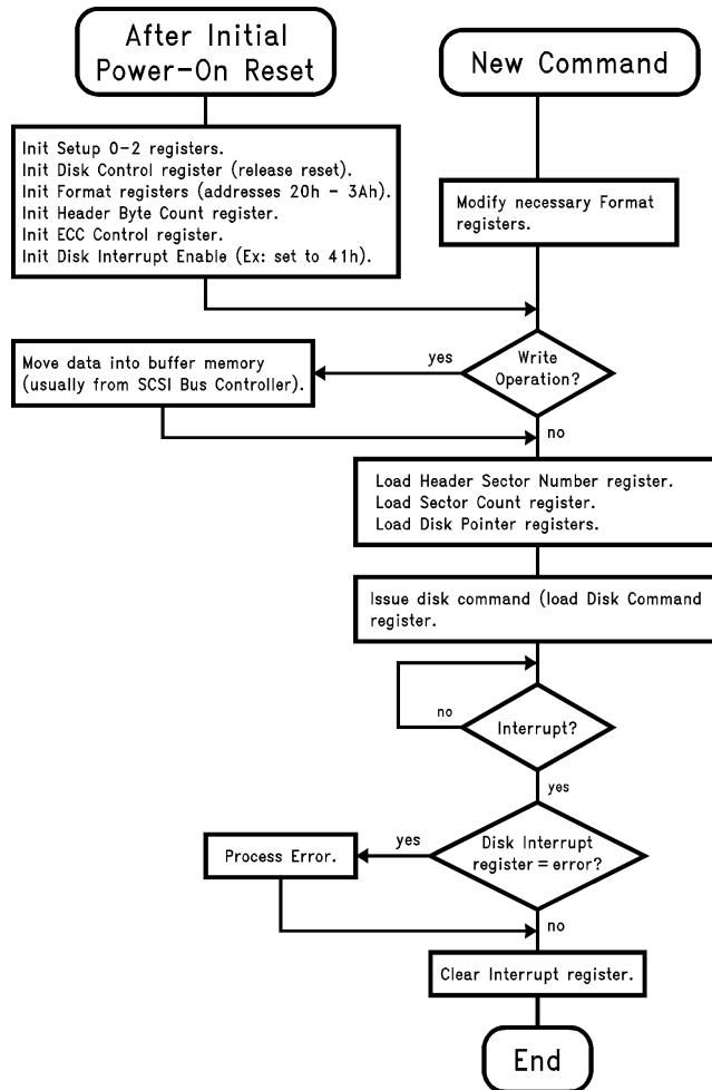
**FIGURE 4.6. Software Flowchart for Simple Disk Operations**
