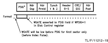
**FIGURE 4.9. RGATE and WGATE Timing during Header Segment**
