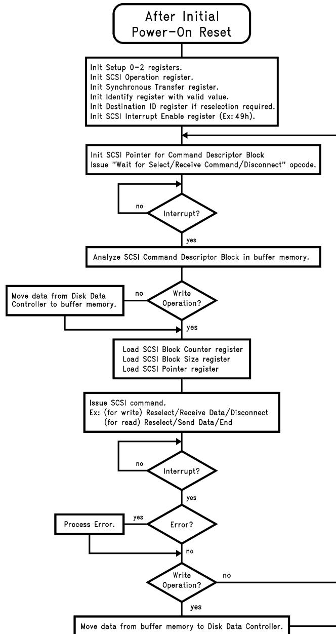
**FIGURE 4.11. Software Flowchart for Simple SCSI Operation**
