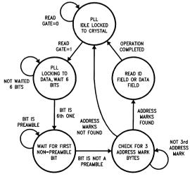
FIGURE 5. Read Algorithm-State Diagram for Data
