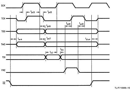
FIGURE 15. Serial Scan Interface Timing
