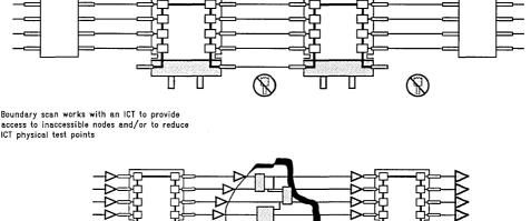
access to inaccessible nodes and/or to reduce ICT physical test points
