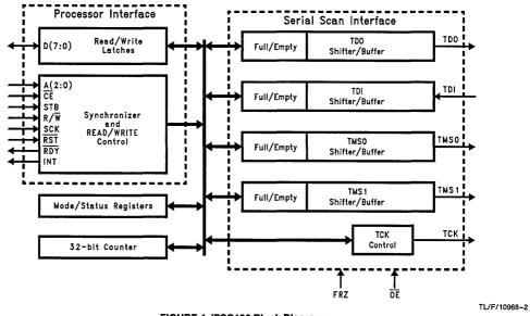
FIGURE 1. 'PSC100 Block Diagram
