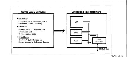
FIGURE 9. SCAN EASE Enables ATPG Test Vectors to be Embedded
