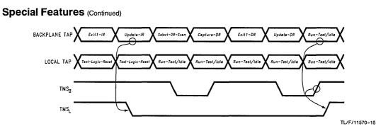
FIGURE 11. Local Scan Port Synchronization on Second Pass
