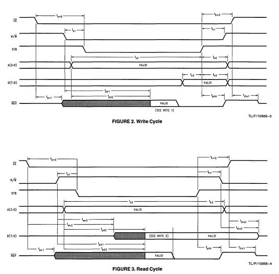
Note 1: Valid data is provided on the RDY line a t<sub>pd1</sub> after R/W is asserted low or a t<sub>pd2</sub> after valid data is decoded on A2:0. The RDY line will remain high until the addressed register is ready to participate in the write operation. This condition only applies when writing to a shifter/buffer and is eliminated (i.e., RDY will go low immediately once valid) when using shifter/buffer status polling (discussed later in this datasheet).
