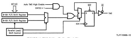
FIGURE 10. TMS Shifter/Buffer Block Diagram
