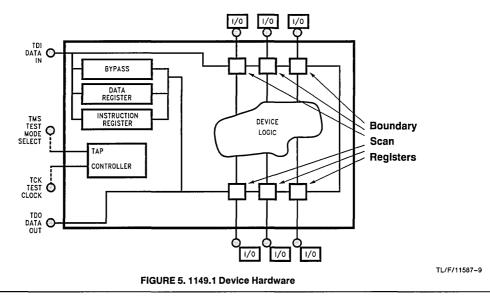
In like fashion as the chip, the boundary scan chain is extended to the board in a serial scan chain. Boards in systems can also be linked in a scan chain.
