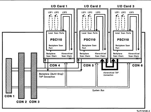
FIGURE 4. Backplane—Hierarchical Connection
