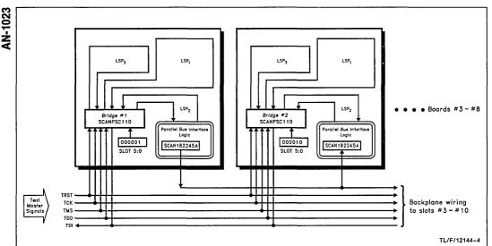
The PSC110F has 3 local scan ports. One port is connected to the backplane drivers. The other two partition the resident board. FIGURE 4. Testing the Backplane Interconnects
