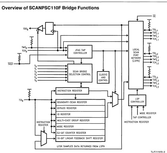
FIGURE 1. SCANPSC110F Bridge Architecture
