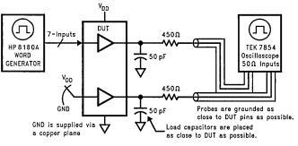
FIGURE 12. Simultaneous Switching Test Circuit
