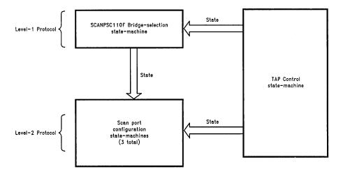
FIGURE 2. SCANPSC110F Bridge State Machines
