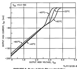
FIGURE 8. Output High Characteristics  $V_{CC} = 5V DC$
