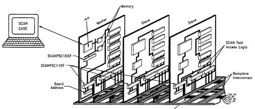
FIGURE 3. Embedding SCAN EASE for System Level Test
