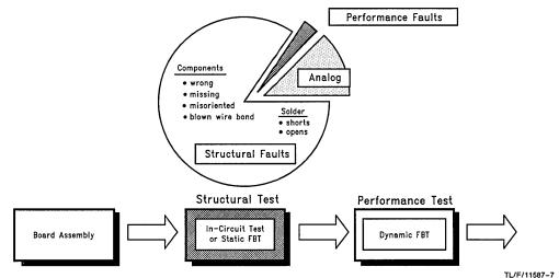
FIGURE 3. The Majority of Printed Circuit Board (PCB) Manufacturing Failures Are a Result of Structural Faults
