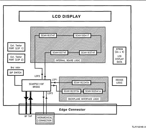
FIGURE 3. Demonstration I/O Card
