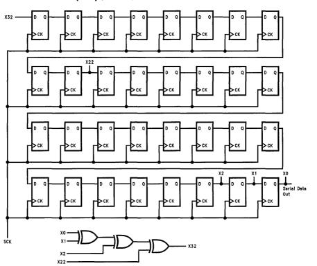
FIGURE 12. TDO PRPG Block Diagram
