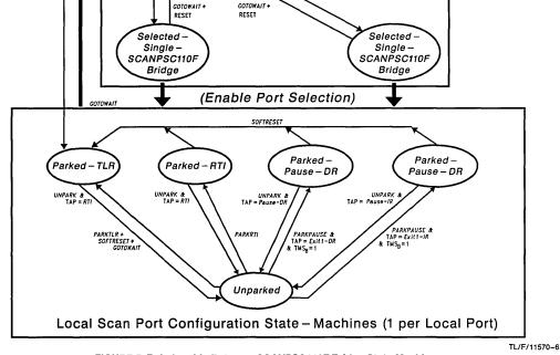
FIGURE 5. Relationship Between SCANPSC110F Bridge State Machines
