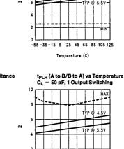
**Propagation Delay vs Temperature**
