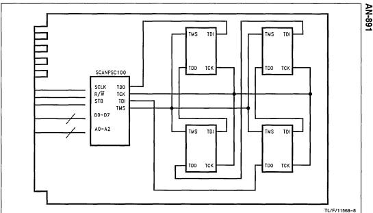
FIGURE 7. An Example of 1149.1 Applied to the Test Access of a PWB with No Spare Backplane Pins to Provide Test Access. A Typical Bus Master, SCANPSC100, Develops the Needed Test Port on the Module
