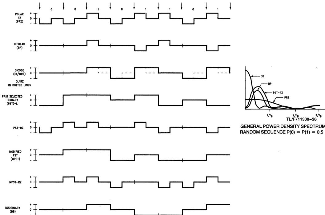
FIGURE 20. Multilevel Binary (MLB) or Pseudoternary Pulse Codes
