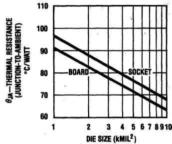
FIGURE 8. Thermal Resistance vs Board or Socket Mount
