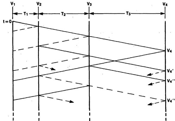
FIGURE 1-16. Lattice Diagram for Three Lines with Delay Ratios 1:2:3
