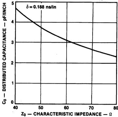
FIGURE 2-5. Stripline Distributed Capacitance Versus Impedance, G-10 Epoxy
