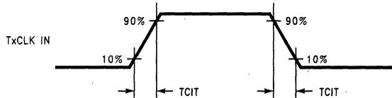
FIGURE 5. DS90CF583 (Transmitter) Input Clock Transition Time
