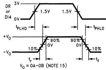
**FIGURE 4. Driver Differential Propagation Delays and Transition Times**
