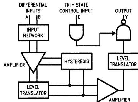
FIGURE 1. Block Diagram
