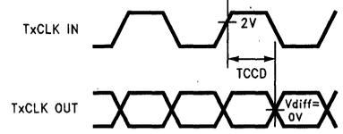
**FIGURE 9. DS90CR563 (Transmitter) Clock In to Clock Out Delay**
