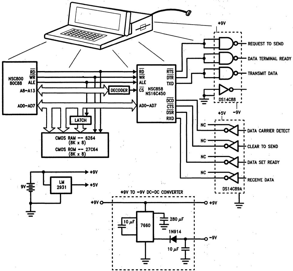
**FIGURE 5. Typical portable system application using CMOS  $\mu$ P, ROM, RAM, and UART. RS-232 Interface is shown using 7660 supply inverter and CMOS Receiver/Driver.**
