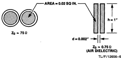
**FIGURE 3-9. Effect of Geometry on Power Bus Impedance**
