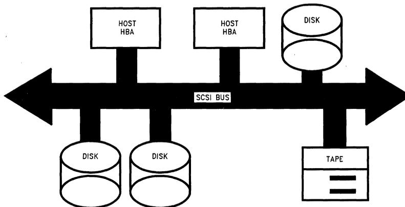
FIGURE 1. Typical SCSI Bus Configuration-Multiple Hosts/Multiple Targets
