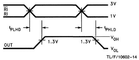
FIGURE 6. Receiver Differential Propagation Delay Timing
