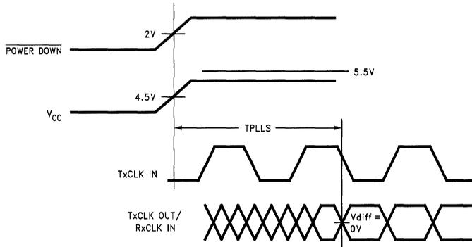
FIGURE 10. DS90CR281 (Transmitter) Phase Lock Loop Set Time
