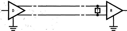
FIGURE 6. Typical TIA/EIA-422-B Point-to-Point Application
