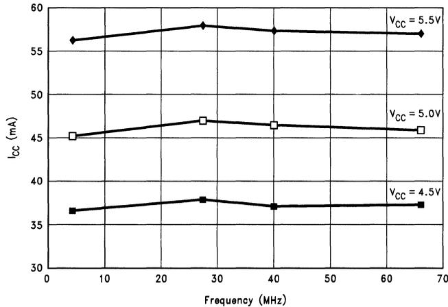
**FIGURE 7. DS3886A I<sub>CC</sub> vs Switching Frequency (A<sub>n</sub> to B<sub>n</sub>) (All Channels Switching at Room Temperature)**
