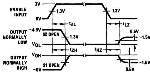
FIGURE 6. Enable and Disable Times for "LS-Type" Load (Notes 8, 9)
