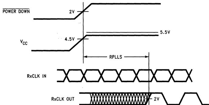
FIGURE 12. DS90CR564 (Receiver) Phase Lock Loop Set Time
