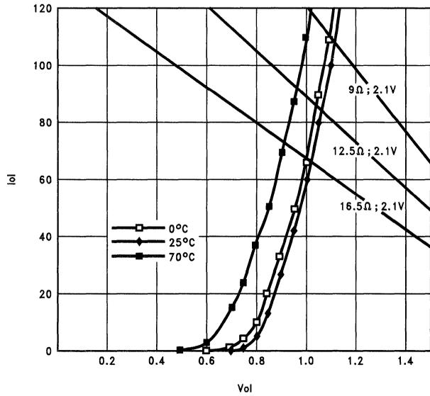
FIGURE 4.  $I_{OL}$  vs  $V_{OL}$  and Load Line
