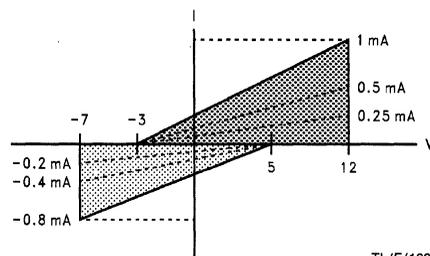
FIGURE 18. Input Current vs Input Voltage Operating Range
