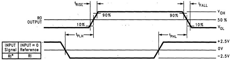
FIGURE 1. Propagation Delays
