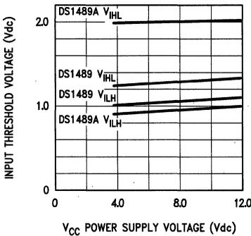
**FIGURE 6. Input Threshold vs Power Supply Voltage**
