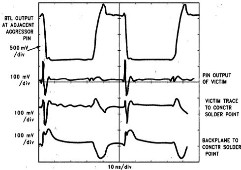
FIGURE 18. Victim Is Only Asserted, 8 Aggressor Channels Switching
