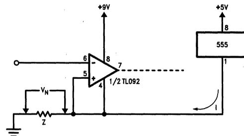
FIGURE 6. Common-Mode Impedance Coupling
