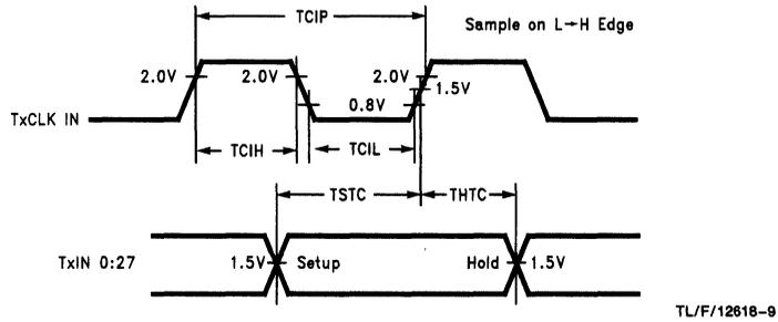
FIGURE 7. DS90CR583 (Transmitter) Setup/Hold and High/Low Times
