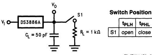
FIGURE 5. Receiver Propagation Delay Set-up
