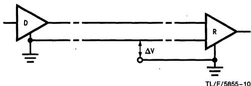
**FIGURE 11. MIL STD 188-114A Unbalanced Typical Application**
