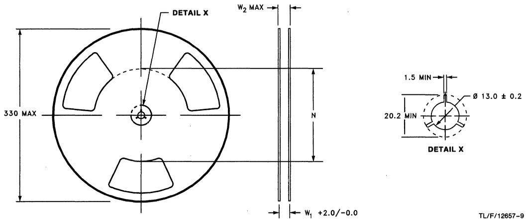
Plastic 330mm (13") Reel Dimensions for 12mm, 16mm, 24mm and 32mm Tape
