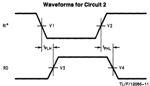
**FIGURE 6. Propagation Delay Waveforms for Circuit 1 and Circuit 2 (See Figure 5)**
