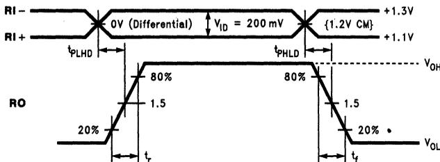
FIGURE 7. Receiver Propagation Delay and Transition Time Waveforms
