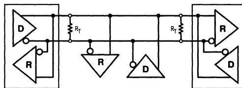
FIGURE 11. Bi-Directional Termination Configuration
