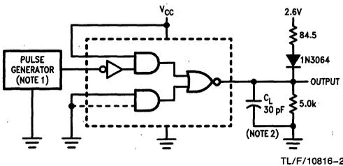
**Note 1:** The pulse generator has the following characteristics:  $Z_{OUT} \approx 50\Omega$ ,  $t_W = 200$  ns, duty cycle = 50%,  $t_r = t_f = 5.0$  ns.
