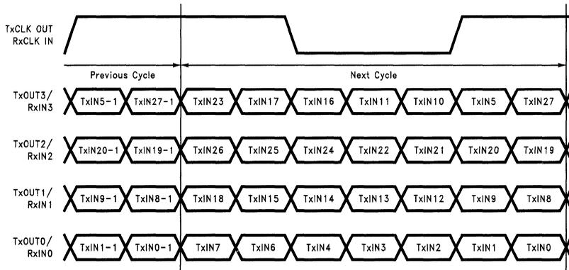
FIGURE 13. 28 Parallel TTL Data Inputs Mapped to LVDS Outputs (DS90CR281)
