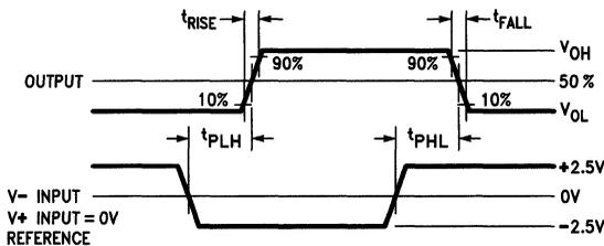
**FIGURE 1. Propagation Delays**
