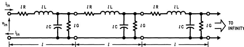
FIGURE 4. Series Connected Sections to Approximate a Distributed Transmission Line
