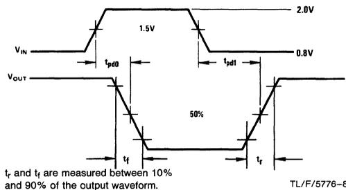
t<sub>r</sub> and t<sub>f</sub> are measured between 10% and 90% of the output waveform.
