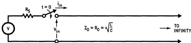
FIGURE 1a. Generator Driving an Infinite Transmission Line
