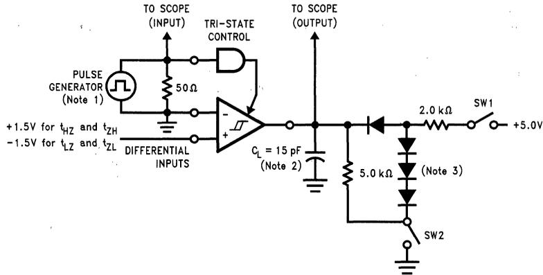
FIGURE 3. Propagation Delay TRI-STATE Control Input to Output
