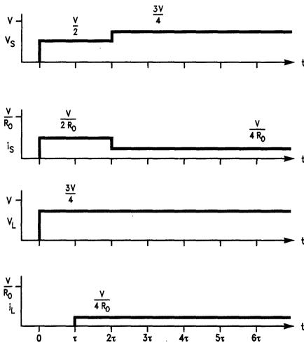
FIGURE 6.  $R_S = R_0, R_L = 3R_0$
