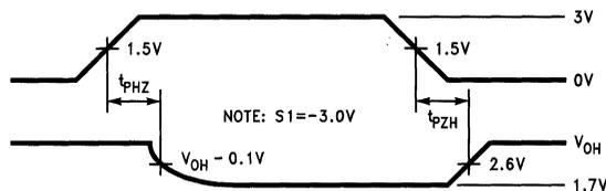
FIGURE 6. Receiver TRI-STATE® Delay Timing ( $t_{PHZ}$ ,  $t_{PZH}$ )
