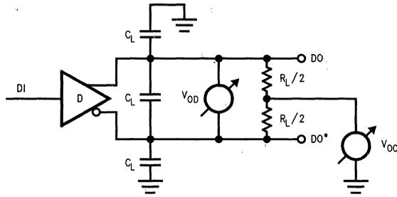
FIGURE 1.  $V_{OD}$  and  $V_{OC}$  Test Circuit
