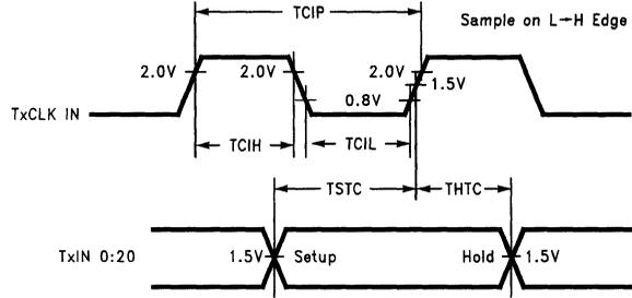
**FIGURE 7. DS90CR563 (Transmitter) Setup/Hold and High/Low Times**
