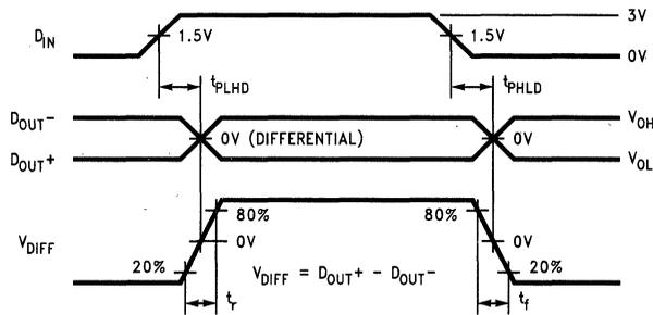
FIGURE 4. Differential Driver Propagation Delay and Transition Time Waveforms
