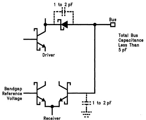
**FIGURE 4. Typical BTL Input/Output Structure**
