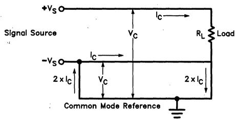
FIGURE 3. Common-Mode Interference
