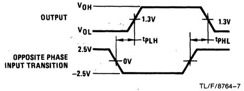
FIGURE 5. Propagation Delay for "LS-Type" Load (Notes 7, 9)
