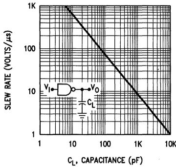
**FIGURE 3. Output Slew Rate vs Load Capacitance**
