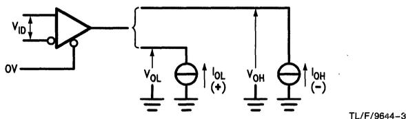
FIGURE 3. Receiver  $V_{OH}$  and  $V_{OL}$
