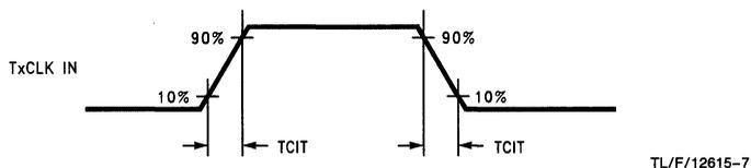
FIGURE 5. DS90CF563 (Transmitter) Input Clock Transition Time
