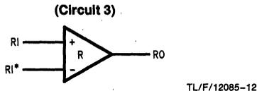
**FIGURE 7. Circuit for Measuring Differential Propagation Delays (See Figure 8)**
