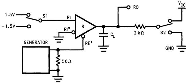
FIGURE 14. Receiver TRI-STATE and Sleep Mode Test Circuit
