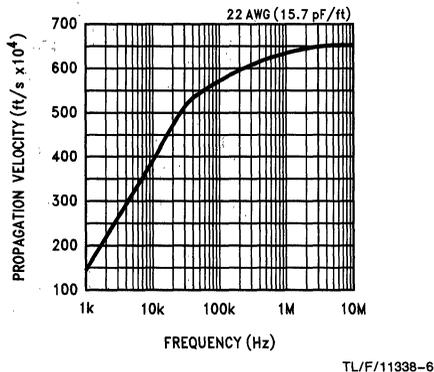
FIGURE 5. Propagation Velocity vs Frequency
