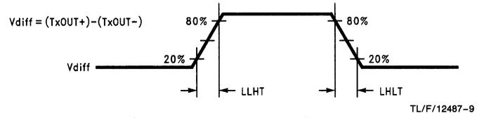
FIGURE 3. DS90CR581 (Transmitter) LVDS Output Load and Transition Timing
