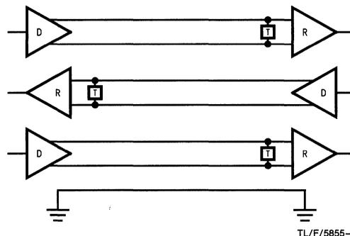
**FIGURE 2. Balanced Data Transmission-3 Channel, 7 Line and Ground**
