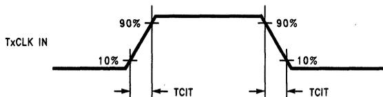
FIGURE 5. DS90CR583 (Transmitter) Input Clock Transition Time
