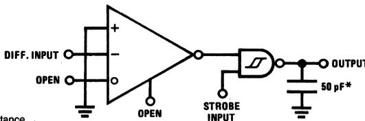
\*Includes probe and test fixture capacitance
