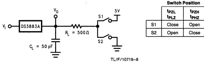
**FIGURE 6. Receiver Enable/Disable Set-Up**
