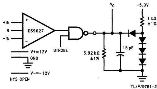
15 pF includes jig capacitance. All diodes are FD777 or equivalent.
