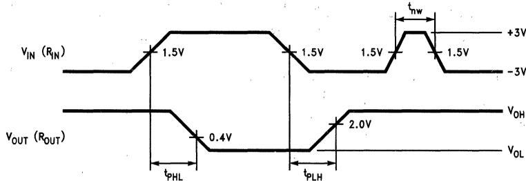
FIGURE 4. Receiver Propagation Delays and Noise Rejection
