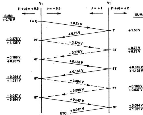
FIGURE 1-5. Lattice Diagram for the Circuit of Figure 1-3
