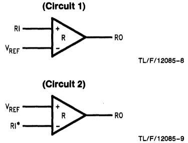
**FIGURE 5. Circuits for Measuring Single-Ended Propagation Delays (See Figure 6)**
