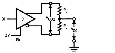
FIGURE 1. Driver V<sub>OD2</sub> and V<sub>OC</sub>
