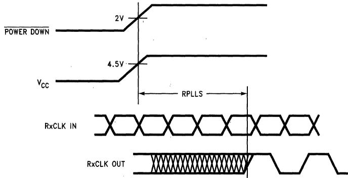
FIGURE 12. DS90CF582 (Receiver) Phase Lock Loop Set Time
