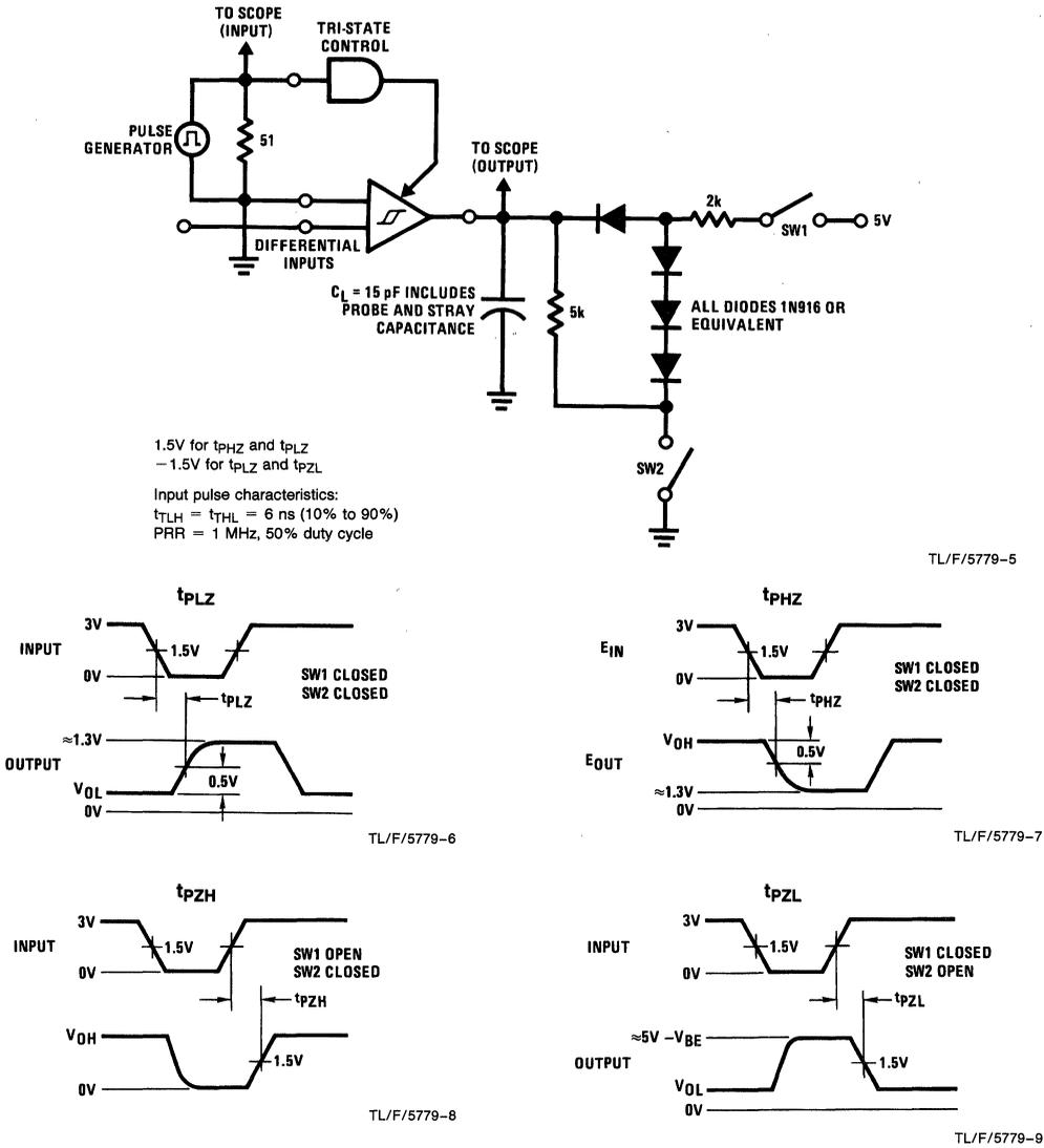
FIGURE 2. Propagation Delay TRI-STATE Control Input to Output
