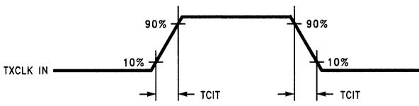
FIGURE 5. DS90CR581 (Transmitter) Input Clock Transition Time
