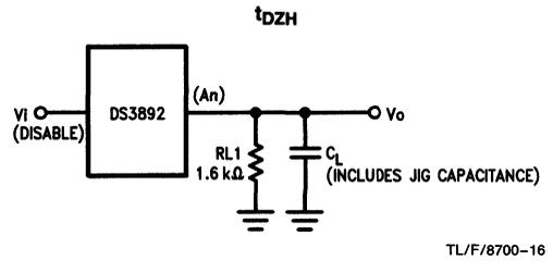
FIGURE 3. Propagation Delay from Disable Pin to An
