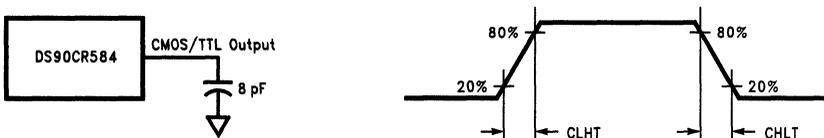
FIGURE 4. DS90CR584 (Receiver) CMOS/TTL Output Load and Transition Times
