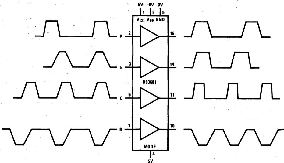
FIGURE 9. DS3691 Connected for Unbalanced Mode Operation (Non-inverting)
