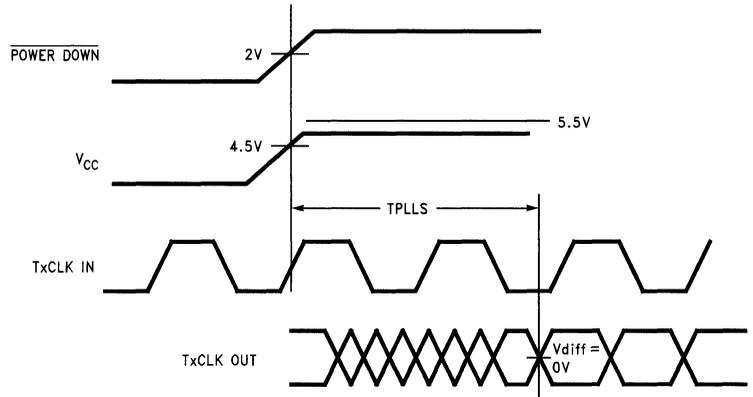
FIGURE 11. DS90CF563 (Transmitter) Phase Lock Loop Set Time
