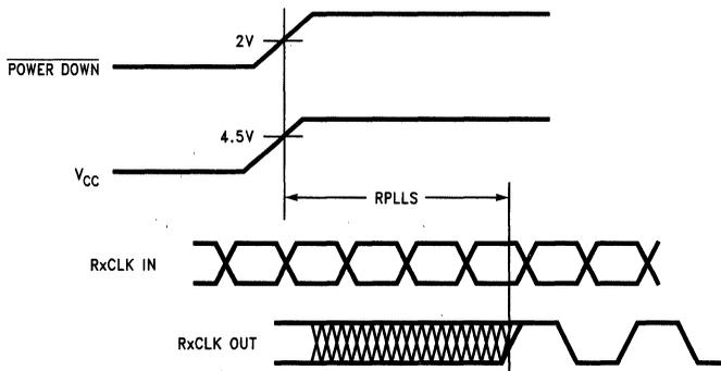
FIGURE 11. DS90CR212 (Receiver) Phase Lock Loop Set Time
