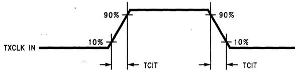
FIGURE 5. DS90CF581 (Transmitter) Input Clock Transition Time
