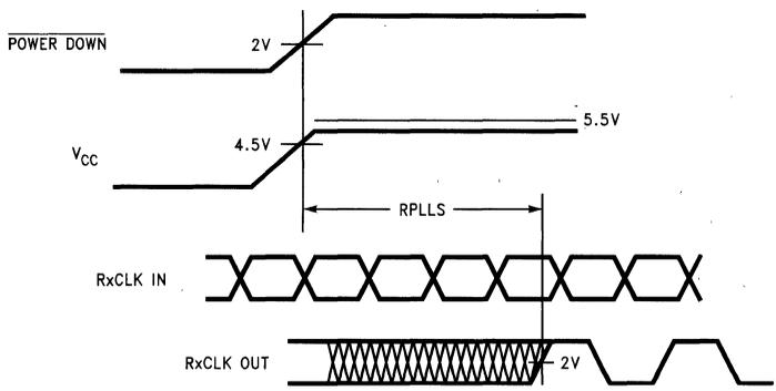
FIGURE 12. DS90CF564 (Receiver) Phase Lock Loop Set Time
