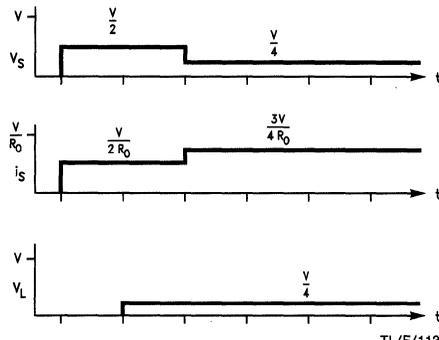
FIGURE 7.  $R_L = \frac{R_0}{3}$
