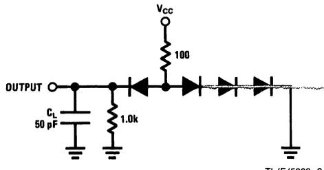
**FIGURE 1. Driver Output Load**
