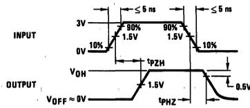
FIGURE 2.  $t_{PZH}$  and  $t_{PHZ}$
