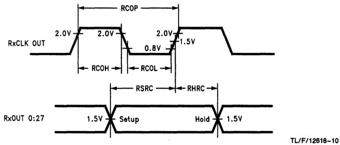
FIGURE 8. DS90CR584 (Receiver) Setup/Hold and High/Low Times
