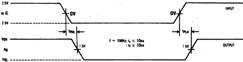
Note: Differential input voltage may be realized by grounding  $\bar{R}I$  and pulsing  $R_I$  between +2.5V and -2.5V.
