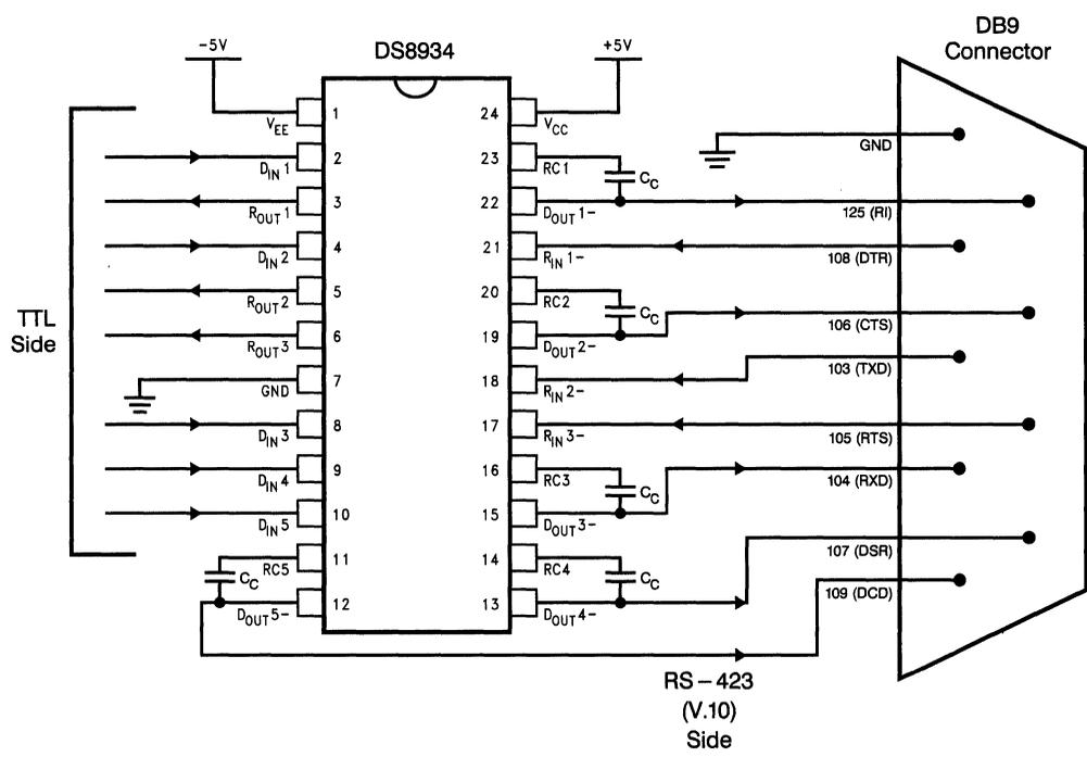
FIGURE 1. Asynchronous Application
