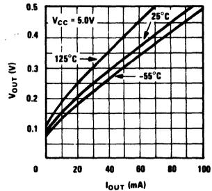
Iout vs Vout High Impedance Output State
