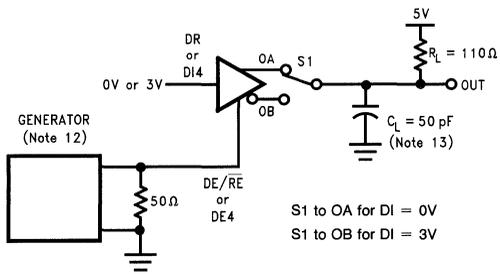
**FIGURE 6. Driver Enable and Disable Timing ( $t_{pZL}$ ,  $t_{pLZ}$ )**
