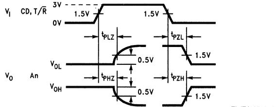
**FIGURE 7. Receiver: CD to An, T/R to An ( $t_{pHZ}$  and  $t_{pZH}$  only)**
