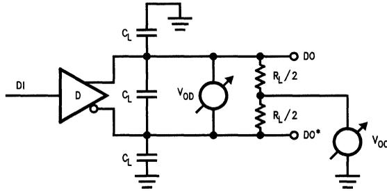
FIGURE 1.  $V_{OD}$  and  $V_{OC}$  Test Circuit
