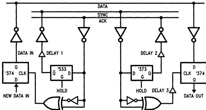
FIGURE 5. Asynchronous Bus Logic for Burst Data Transfers
