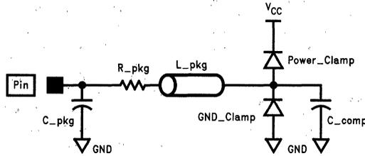
FIGURE 2. Input/Enable Structure Model
