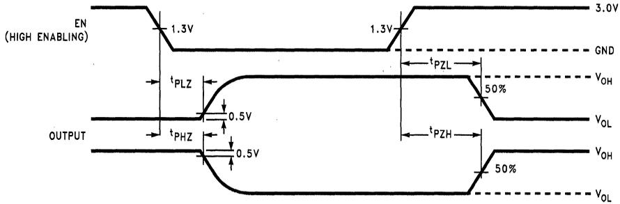
FIGURE 3. TRI-STATE Output Enable and Disable Waveforms
