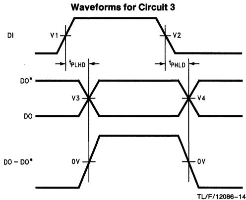
**FIGURE 9. Propagation Delay Waveforms for Circuit 3 (See *Figure 8*)**
