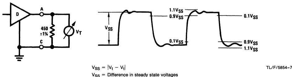
FIGURE 4. Unbalanced Driver Output Signal Waveform
