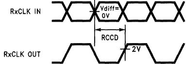
**FIGURE 10. DS90CR564 (Receiver) Clock In to Clock Out Delay**
