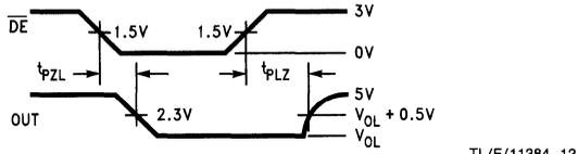
**FIGURE 11. Driver TRI-STATE Delays ( $t_{pZL}$ ,  $t_{PLZ}$ )**
