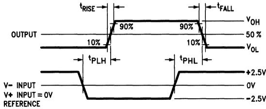
FIGURE 1. Propagation Delay
