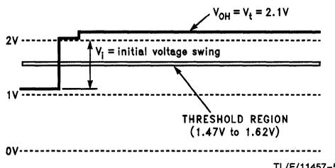
**FIGURE 5. BTL Bus Waveforms—IEEE 896 Electrical Environment**
