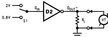
FIGURE 2. Single Ended Driver DC Test Circuit
