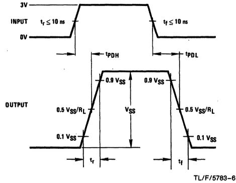
AC Test Circuits and Switching Time Waveforms (Continued)
