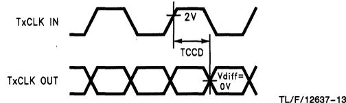
FIGURE 8. DS90CR211 (Transmitter) Clock In to Clock Out Delay
