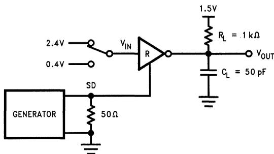
FIGURE 7. Receiver SHUTDOWN (SD) Delay Test Circuit
