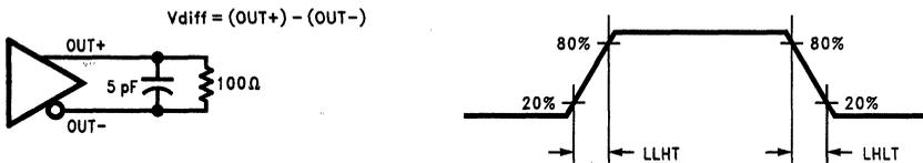
FIGURE 3. DS90CR583 (Transmitter) LVDS Output Load and Transition Times
