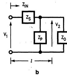
**FIGURE 5. Cascaded Network to Model Transmission Line**
