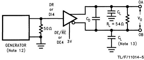
**FIGURE 3. Driver Differential Propagation Delay Load Circuit**
