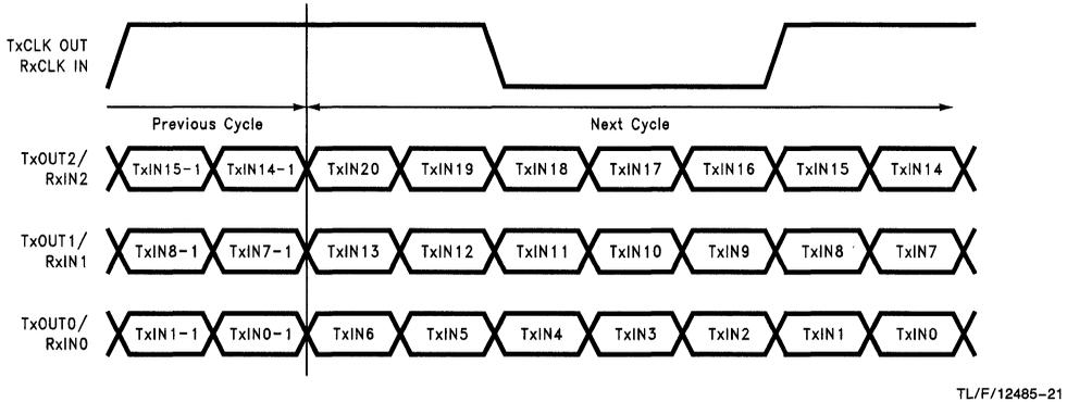
**FIGURE 14. 21 Parallel TTL Data Inputs Mapped to LVDS Outputs (DS90CF561)**
