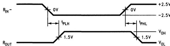
FIGURE 10. Receiver Propagation Delay Waveform
