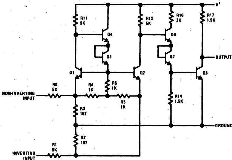
FIGURE 9. Simplified Schematic of the Line Receiver
