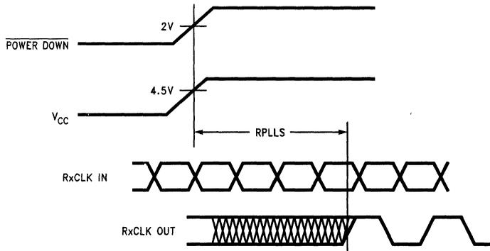
FIGURE 12. DS90CR562 (Receiver) Phase Lock Loop Set Time
