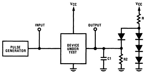
**Note:** C1 includes test fixture capacitance.
