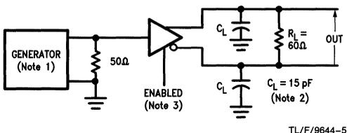
FIGURE 4. Driver Differential Output Delay and Transition Times
