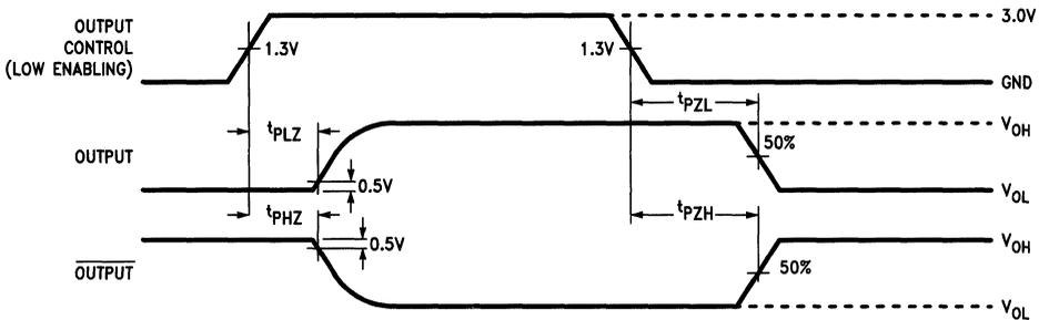
FIGURE 3. TRI-STATE Output Enable and Disable Waveforms
