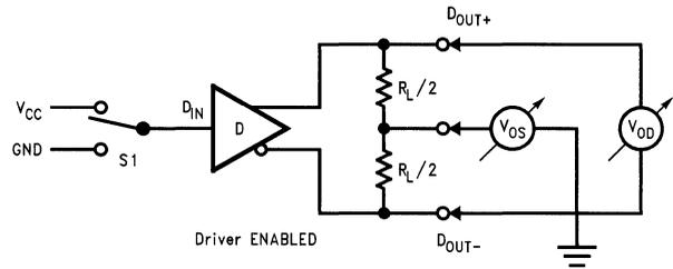
FIGURE 1. Driver  $V_{OD}$  and  $V_{OS}$  Test Circuit
