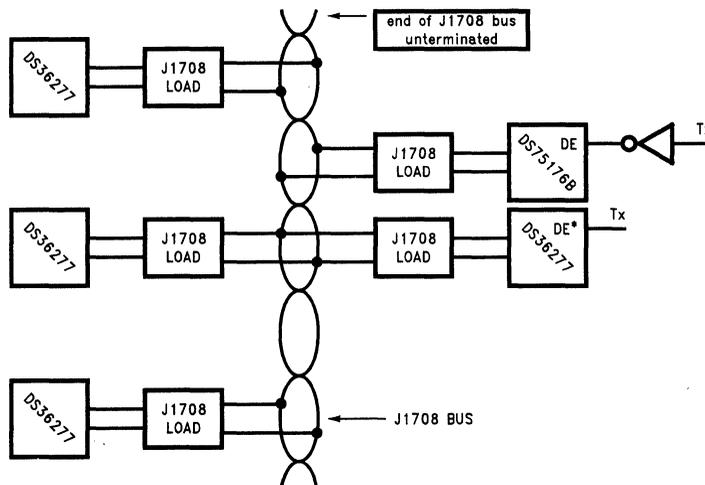
FIGURE 7. SAE J1708 Typical Bus Configuration and Loading
