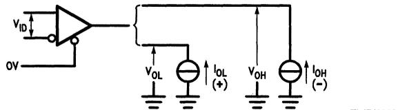
FIGURE 3. Receiver  $V_{OH}$  and  $V_{OL}$
