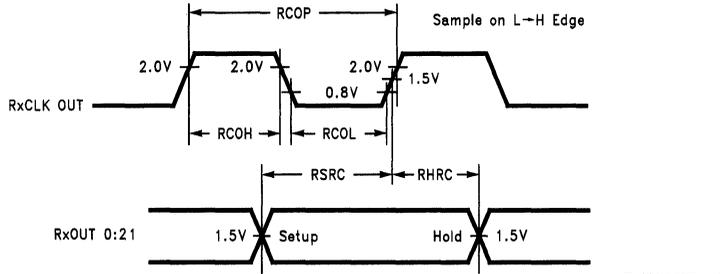
FIGURE 7. DS90CR212 Setup/Hold and High/Low Times
