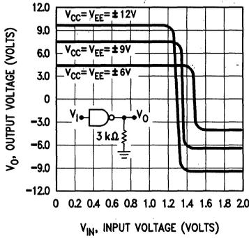
**FIGURE 1. Transfer Characteristics vs Power Supply Voltage**
