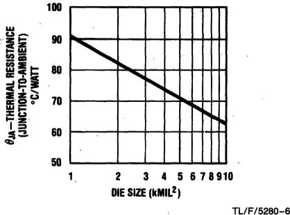
FIGURE 6. Thermal Resistance vs Die Size
