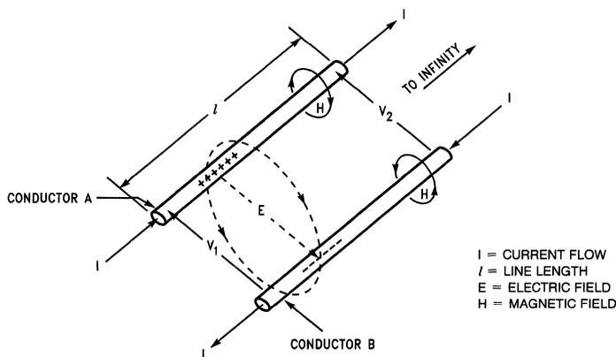
FIGURE 1. Infinite Length Parallel Wire Transmission Line
