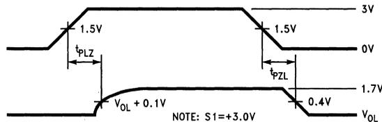
FIGURE 7. Receiver TRI-STATE® Delay Timing ( $t_{PLZ}$ ,  $t_{PZL}$ )
