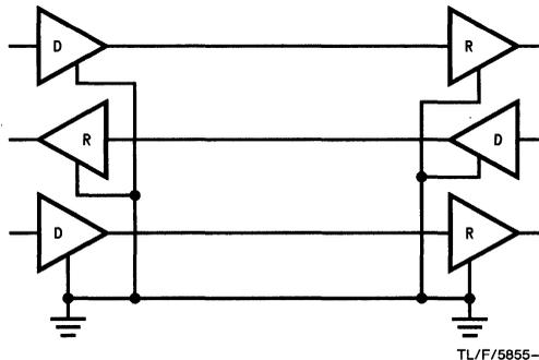
**FIGURE 1. Unbalanced Data Transmission-3 Channel, 4 Line**
