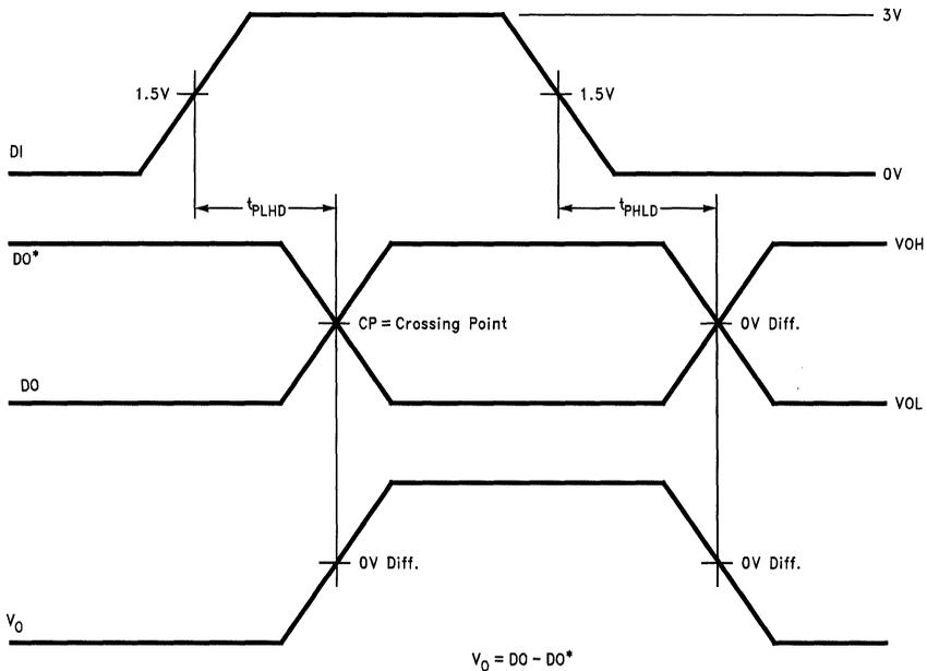
FIGURE 12. Typical Curve Driver Differential Propagation Delay Timing
