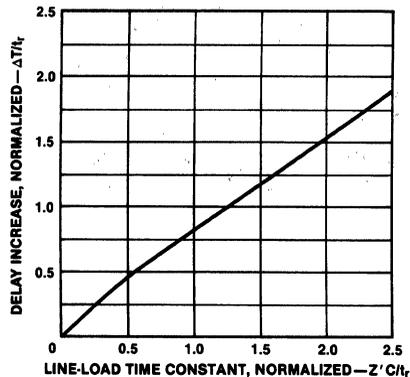
**FIGURE 1-11. Increase in 50% Point Delay Due to Capacitive Loading at the End of the Line, Normalized to  $T_r$**
