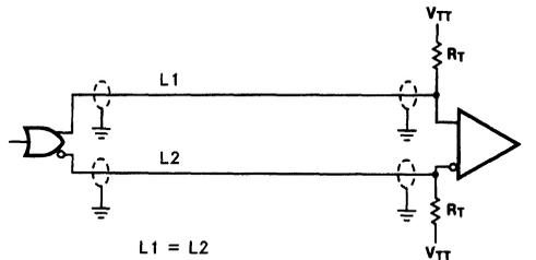
c. Differential Transmission with Grounded Shields
