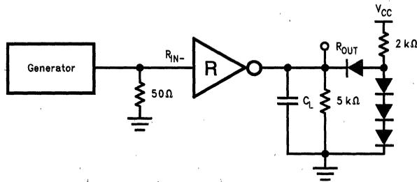
FIGURE 4. Receiver Propagation Delay Test Circuit (Note 6)
