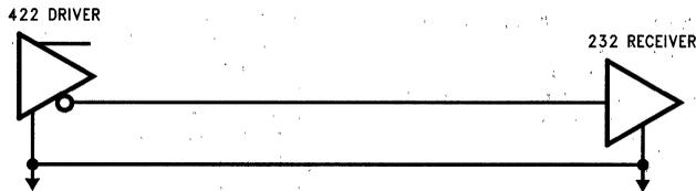
FIGURE 4. RS-422 to RS-232—Direct Connection
