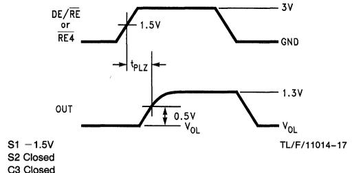
FIGURE 8. Receiver Enable and Disable Timing
