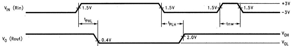
FIGURE 4. Receiver Propagation Delays and Noise Rejection (Note 4)
