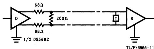
**FIGURE 12. MIL STD 188-114A Balanced, Type 1 Typical Application**
