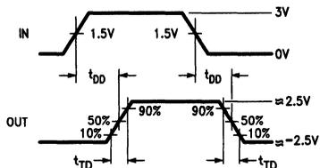
FIGURE 4. Driver Differential Output Delay and Transition Times
