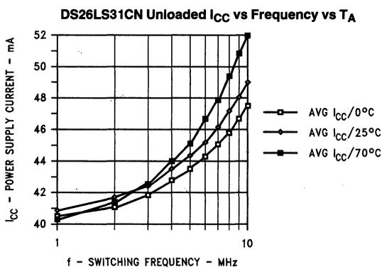
FIGURE 1. Supply Current vs Switching Frequency vs Temperature
