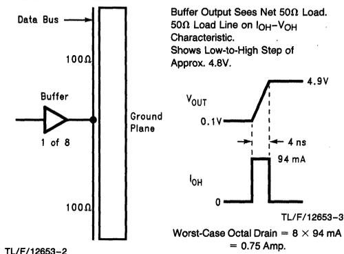
**FIGURE 4-2. Octal Buffer Driving a  $100\Omega$  Bus**
