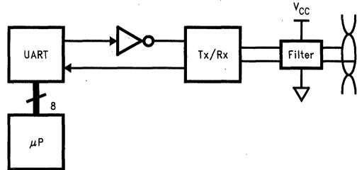
**FIGURE 6. Typical SAE J1708 System Block Diagram**
