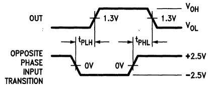
FIGURE 3. Propagation Delay (Notes 1, 2 and 3)
