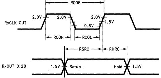
**FIGURE 8. DS90CR564 (Receiver) Setup/Hold and High/Low Times**
