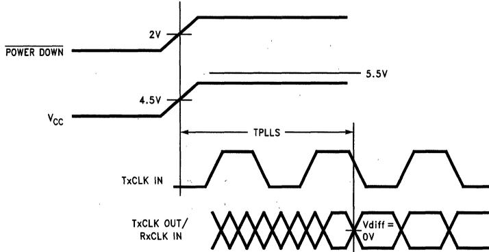
FIGURE 10. DS90CR211 (Transmitter) Phase Lock Loop Set Time
