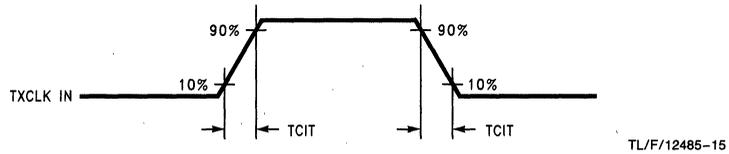
FIGURE 5. DS90CF561 (Transmitter) Input Clock Transition Time
