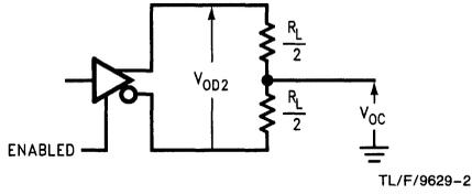
FIGURE 1. Driver  $V_{OD}$  and  $V_{OC}$  (Note 13)
