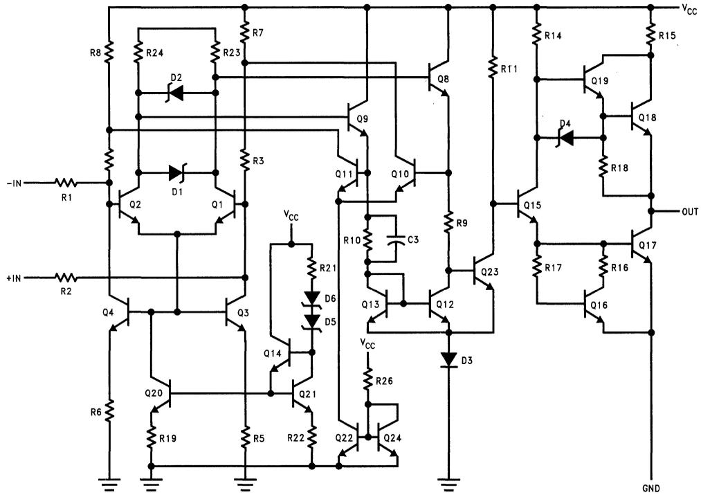
FIGURE 1. Equivalent Circuit
