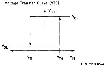
FIGURE 3. Threshold Voltages
