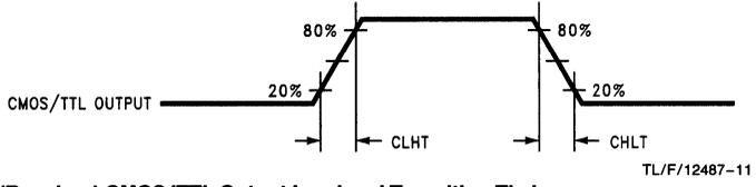
FIGURE 4. DS90CR582 (Receiver) CMOS/TTL Output Load and Transition Timing
