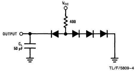
FIGURE 2. Receiver Output Load
