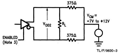
FIGURE 2. Driver  $V_{OD}$  with Varying Common Mode Voltage
