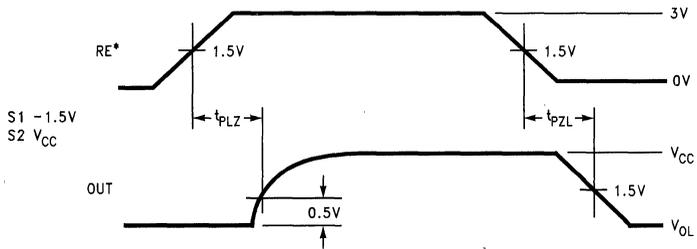
FIGURE 15. Receiver Enable and Disable Waveforms ( $t_{PLZ}$ ,  $t_{PZL}$ )
