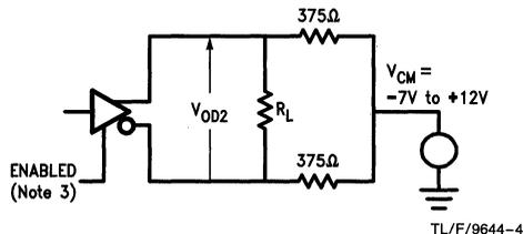
FIGURE 2. Driver  $V_{OD2}$  with Varying Common Mode Voltage
