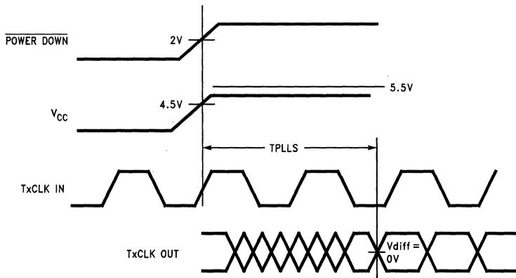
FIGURE 11. DS90CR563 (Transmitter) Phase Lock Loop Set Time
