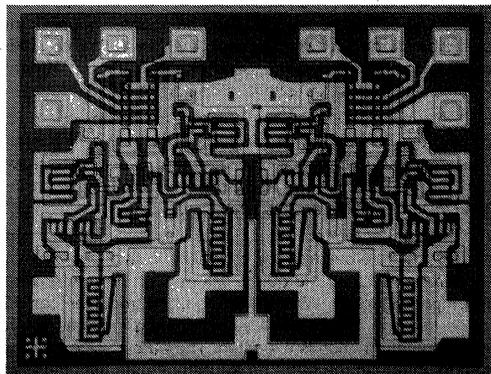
FIGURE 8. Photomicrograph of the DS7830 Dual Line Driver
