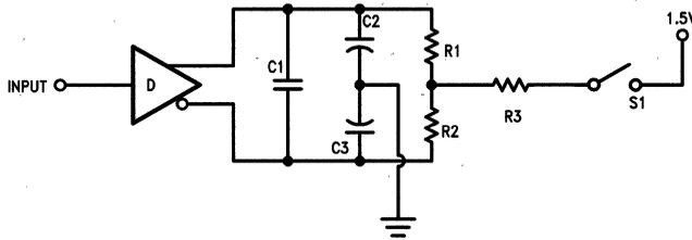
Note: C1 = C2 = C3 = 40 pF (Including Probe and Jig Capacitance), R1 = R2 = 50Ω, R3 = 500Ω.
