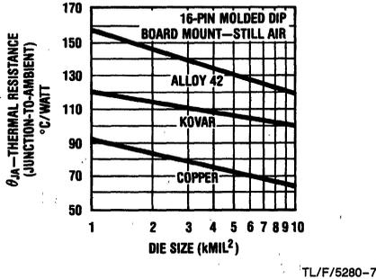
FIGURE 7. Thermal Resistance vs Lead Frame Material
