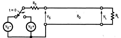
**FIGURE 11. Model Used for Lattice Diagram Method**
