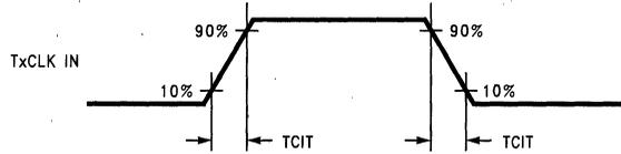
FIGURE 5. DS90CR563 (Transmitter) Input Clock Transition Time
