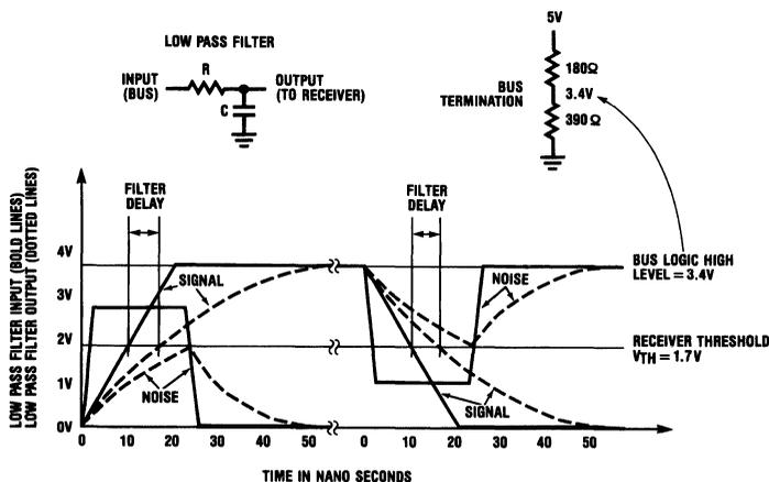
FIGURE 2. Ideal Receiver Low Pass Filter Response
