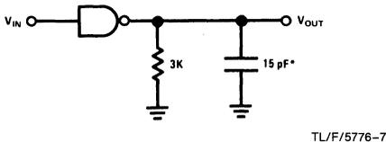
\*C<sub>L</sub> includes probe and jig capacitance.
