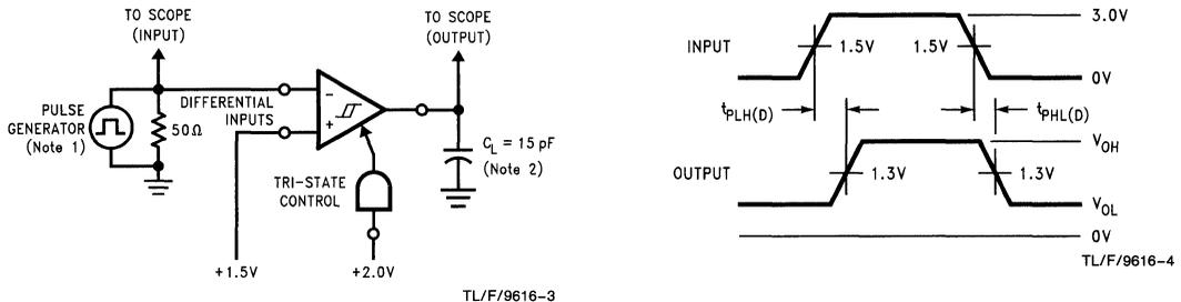
**FIGURE 2. Propagation Delay Differential Input to Output**
