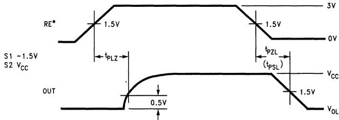
FIGURE 15. Receiver Enable and Disable Waveforms ( $t_{PLZ}$ ,  $t_{PZL}$ , ( $t_{PSL}$ ))
