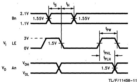
FIGURE 7. Receiver Enable/Disable Set-up
