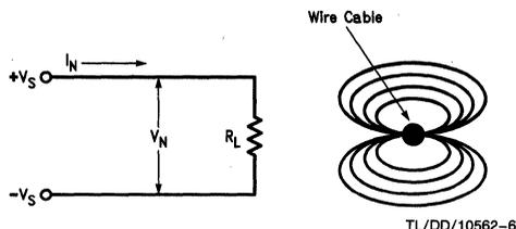
FIGURE 4. Field-to-Cable Coupling
