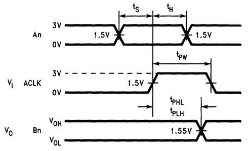
FIGURE 4. Driver: ACKL to Bn,  $t_s$ ,  $t_h$ ,  $t_{PW}$
