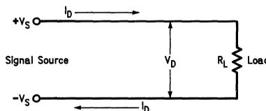
FIGURE 2. Differential-Mode Interference
