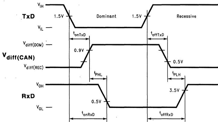
FIGURE 9. Propagation Delays
