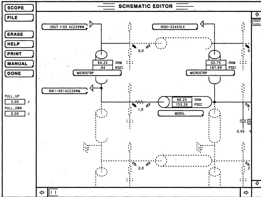
FIGURE 5. Schematic Editor of LineSim PRO
