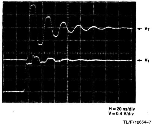
**FIGURE 1-4. Extended Ringing when  $R_S$  of *Figure 1-3* is Reduced to  $13\Omega$**
