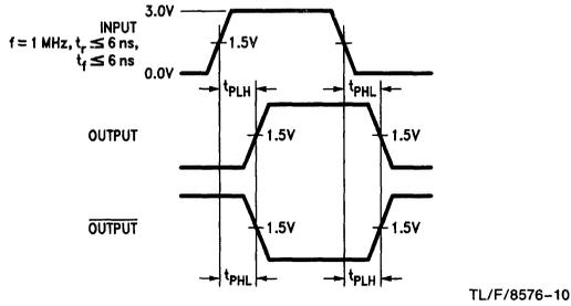
**FIGURE 8. Load Propagation Delays for "LS-Type" Load**
