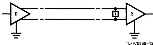
**FIGURE 13. MIL STD 188-114A Balanced, Type 2 Typical Application**
