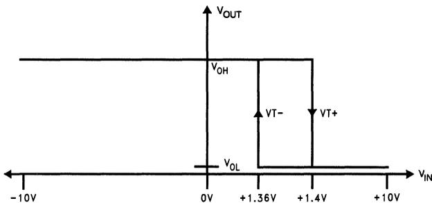
FIGURE 7. Receiver Threshold Voltage Transfer Curve (VTC)
