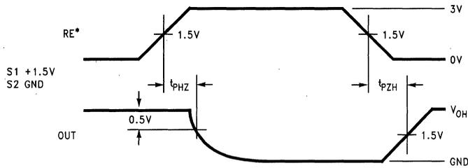
FIGURE 16. Receiver Enable and Disable Waveforms ( $t_{PHZ}$ ,  $t_{PZH}$ )
