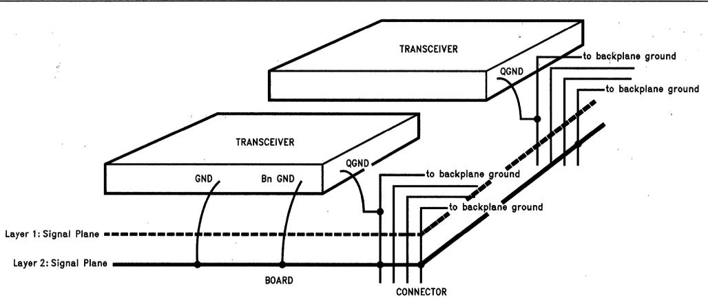
**FIGURE 2. Ground Structure with One Ground Plane**
