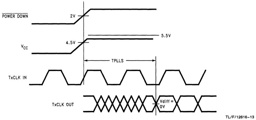
FIGURE 11. DS90CF583 (Transmitter) Phase Lock Loop Set Time
