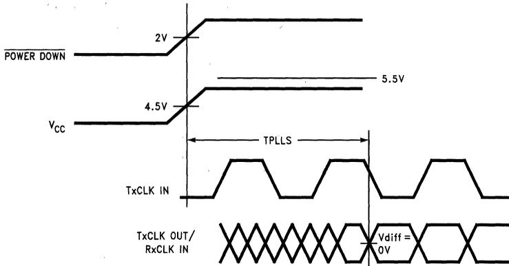
FIGURE 11. DS90CF581 (Transmitter) Phase Lock Loop Set Time
