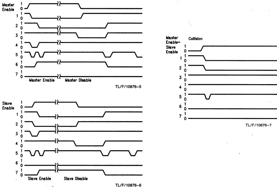
**FIGURE 5. Signals at different points in the circuit vary according to the data line conditions. There are five possible cases: Master Enable, Master Disable, Slave Enable, Slave Disable, and Collision (master and slave attempting to enable simultaneously).**
