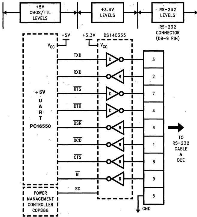
FIGURE 2. Typical Mixed Supply (3V/5V) DTE Application
