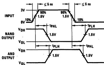
FIGURE 1.  $t_{PLH}$  and  $t_{PHL}$
