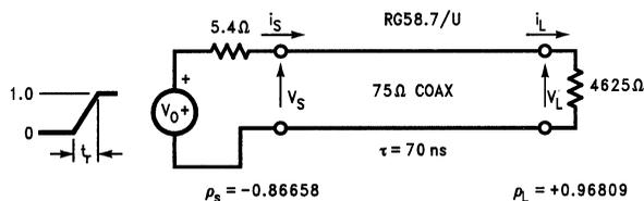
FIGURE 16. Transmission Line Model and Its Lattice Diagram
