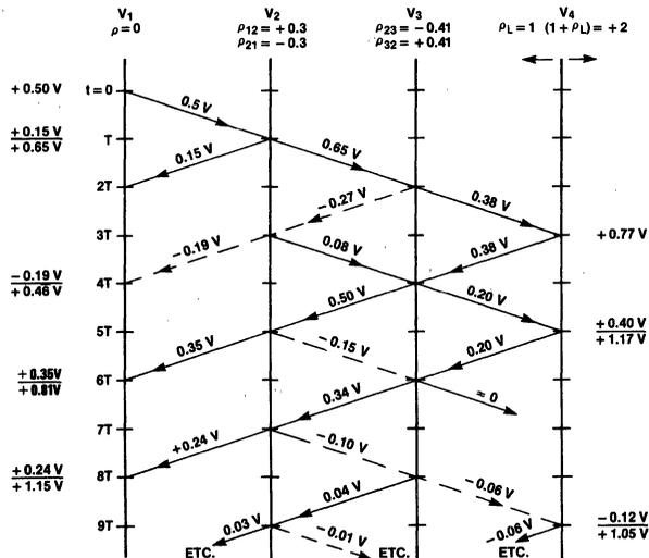
FIGURE 1-15. Lattice Diagram for the Circuit of *Figure 1-14*
