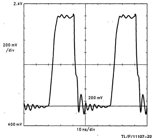
FIGURE 13. Backplane Probed at Driver = Slot 5, 12 pF Loads in Slots 0 and 6
