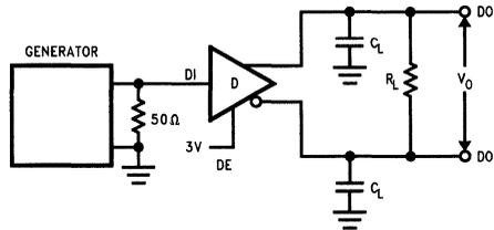
FIGURE 5. Driver Differential Propagation Delay Test Circuit
