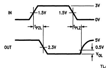
FIGURE 7. Driver Enable and Disable Times ( $t_{PZL}$ ,  $t_{PLZ}$ )
