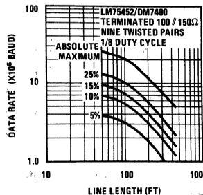
FIGURE 21. Data Rate vs Distortion of LM75452, DM7400
