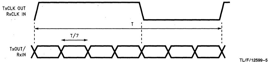
**FIGURE 5. Seven Bits of LVDS in One Clock Cycle**
