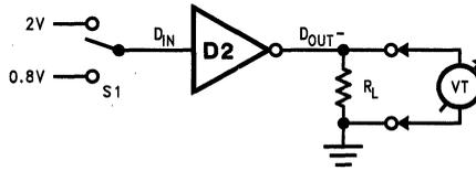
FIGURE 2. Single Ended Driver DC Test Circuit
