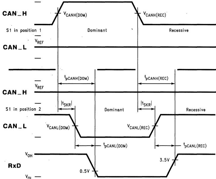
FIGURE 8. Receiver Skew Timing
