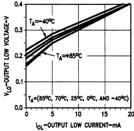
**Receiver VOL vs IOL vs VCC**
