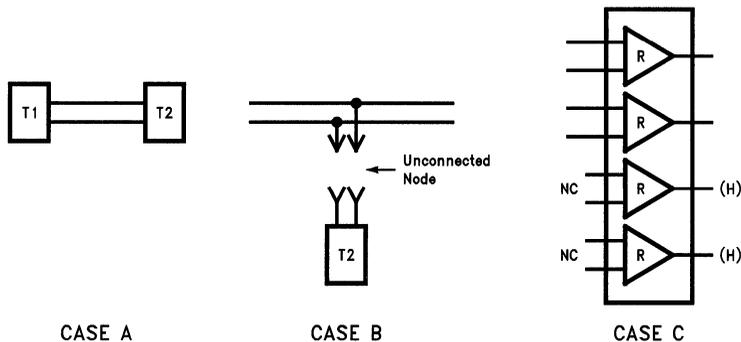
FIGURE 8. Applications of OPEN INPUT FAILSAFE Feature
