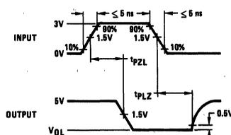
FIGURE 3.  $t_{PZL}$  and  $t_{PLZ}$
