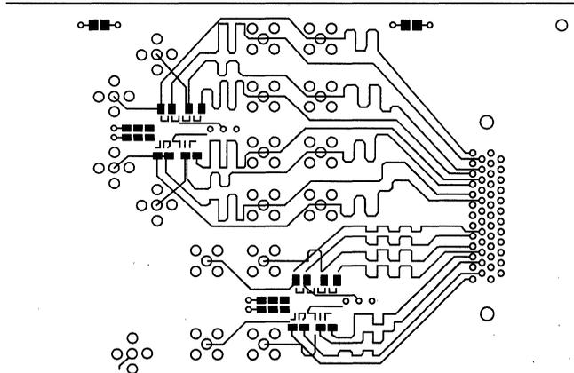
FIGURE 3. Trace Mitering on LVDS Lines
