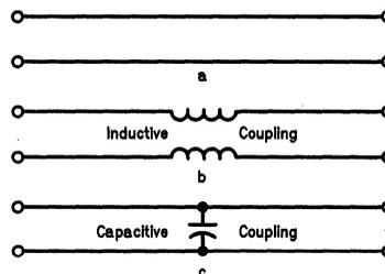
FIGURE 5. Cable-to-Cable Coupling
