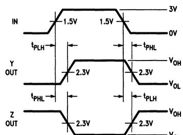
FIGURE 5. Driver Propagation Times
