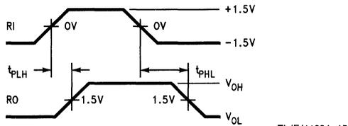
**FIGURE 14. Receiver Propagation Delays**
