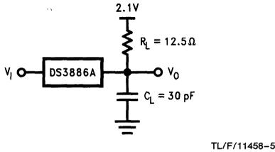
FIGURE 1. Driver Propagation Delay Set-up
