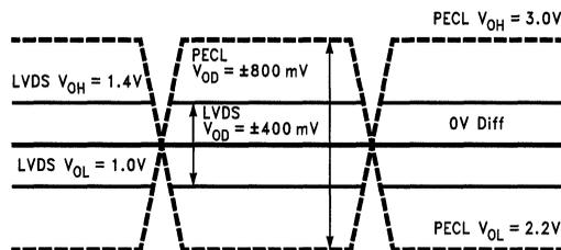
FIGURE 1. PECL vs LVDS Signal Swing
