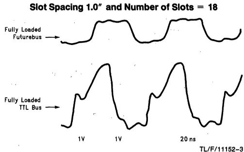
**FIGURE 3. Actual BTL vs TTL Waveforms**
