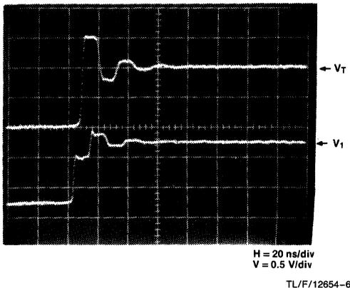
**FIGURE 1-3. Multiple Reflections Due to Mismatch at Load and Source**
