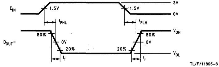
FIGURE 6. Single Ended Driver Propagation Delay and Transition Time Waveform
