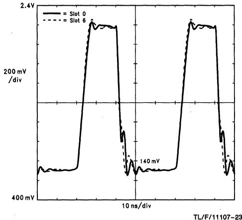
FIGURE 14. Backplane Probed at Driver = Slot 5
