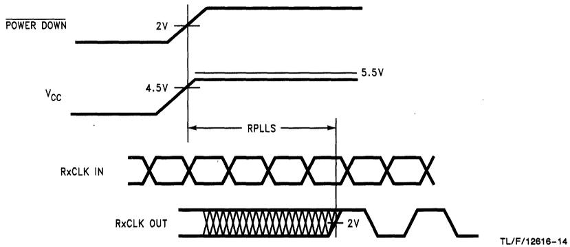
FIGURE 12. DS90CF584 (Receiver) Phase Lock Loop Set Time
