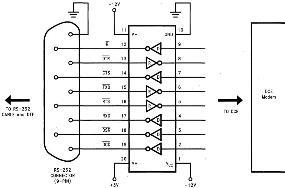
FIGURE 5. Typical DCE Application
