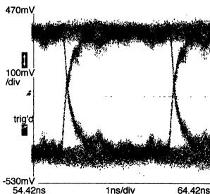
FIGURE 10a. Eye Pattern at Driver Output
