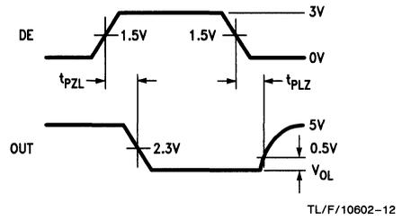
FIGURE 5. Driver Enable and Disable Timing ( $t_{PZL}$ ,  $t_{PLZ}$ )
