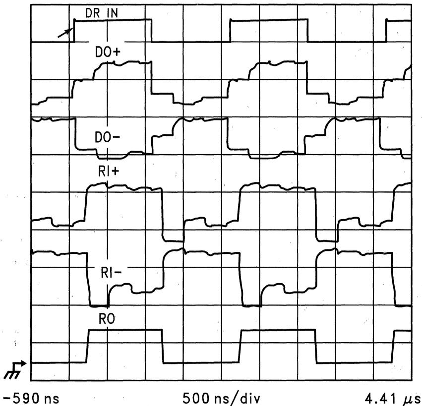
FIGURE 2. Underterminated Waveforms
