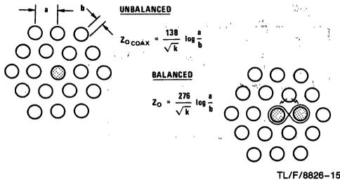
FIGURE 15.  $Z_0$  Unbalanced <  $Z_0$  Balanced
