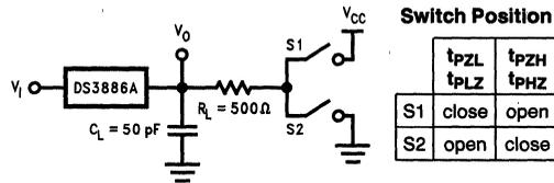
FIGURE 8. Receiver: Enable/Disable Set-up
