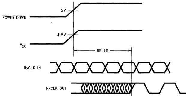
FIGURE 11. DS90CR282 (Receiver) Phase Lock Loop Set Time
