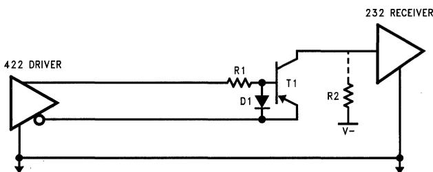
FIGURE 3. RS-422 to RS-232—with Active Device
