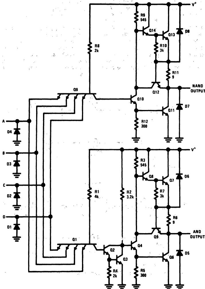
FIGURE 2. Schematic Diagram of the DS7830 Line Driver
