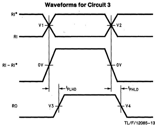
**FIGURE 8. Propagation Delay Waveforms for Circuit 3 (see Figure 7)**
