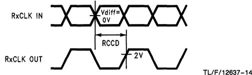
FIGURE 9. DS90CR212 (Receiver) Clock In to Clock Out Delay
