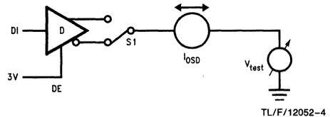
V<sub>test</sub> = -7V to +12V
