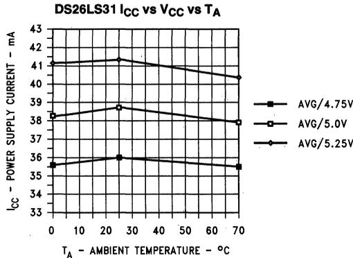
FIGURE 2. Supply Current vs Supply Voltage vs Temperature
