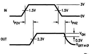
FIGURE 6. Driver Enable and Disable Times ( $t_{PZH}$ ,  $t_{PHZ}$ )
