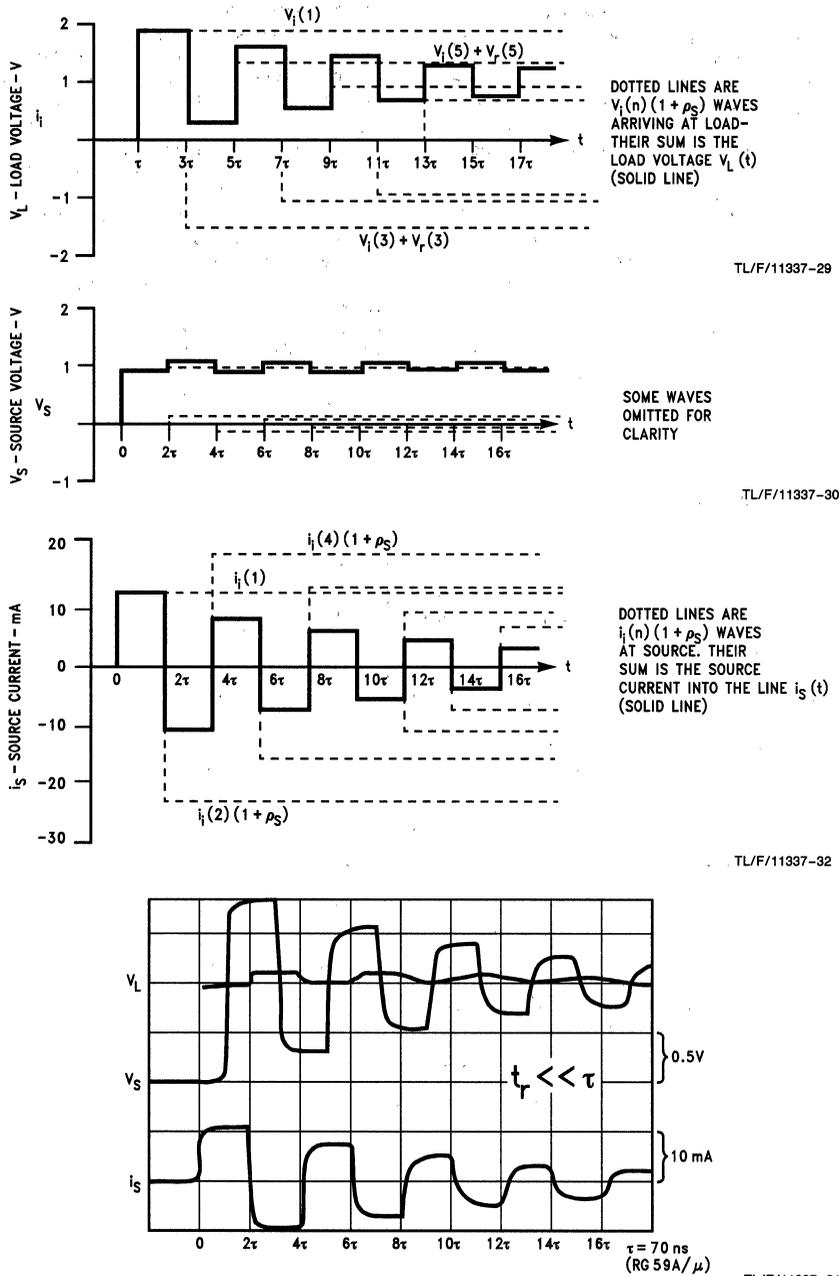
FIGURE 17. Waveforms for  $t_r = 2 \leq \tau$
