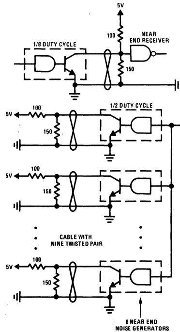
FIGURE 23. Signal Cross Talk Experiment Using DM75452, DM7400
