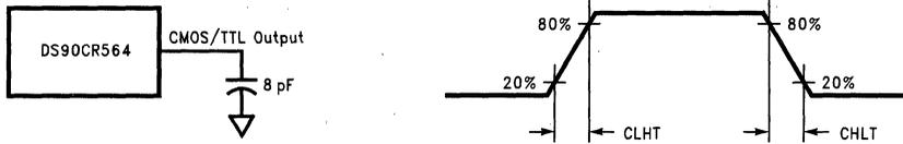
FIGURE 4. DS90CR564 (Receiver) CMOS/TTL Output Load and Transition Times
