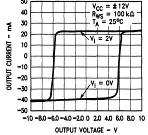
**Output Current vs Output Voltage (Power Off)**
