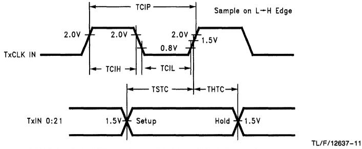
FIGURE 6. DS90CR211 Setup/Hold and High/Low Times
