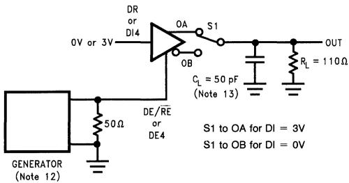
**FIGURE 5. Driver Enable and Disable Timing ( $t_{pZH}$ ,  $t_{pHZ}$ )**
