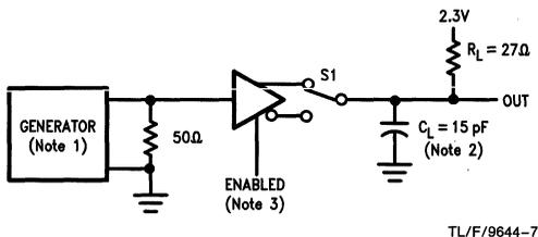
FIGURE 5. Drive Propagation Times
