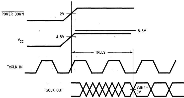
**FIGURE 11. DS90CR583 (Transmitter) Phase Lock Loop Set Time**
