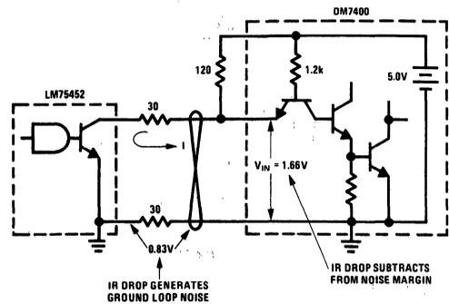
FIGURE 9. Unbalanced Method
