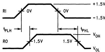
**FIGURE 14. Receiver Propagation Delays**
