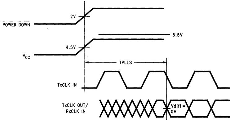
FIGURE 11. DS90CR561 (Transmitter) Phase Lock Loop Set Time
