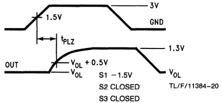
FIGURE 16. Receiver Enable and Disable Timing
