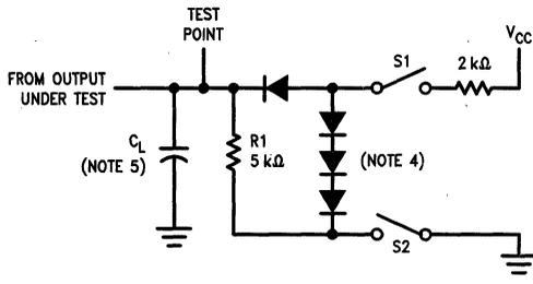
FIGURE 2. Load Test Circuit for Three-State Outputs
