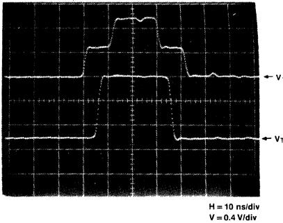
**FIGURE 1-7. Series Terminated Line and Waveforms**
