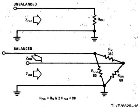
FIGURE 16. Impedance Measurement
