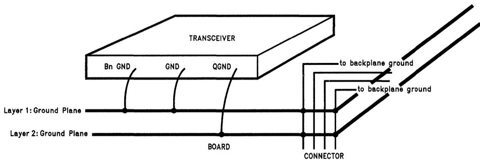
FIGURE 1. Ground Structure with Two Ground Planes
