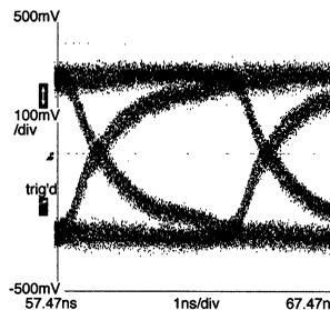
FIGURE 10b. Eye Pattern at Receiver Inputs
