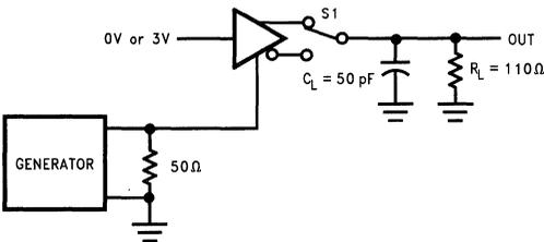
FIGURE 5. Driver Enable and Disable Times ( $t_{ZH}$ ,  $t_{HZ}$ ) (Notes 10, 11, 12)
