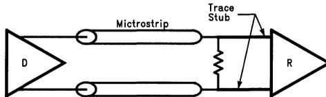
FIGURE 7. A Point-to-Point Configuration Using LVDS
