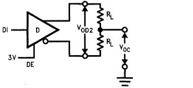
FIGURE 1. Driver  $V_{OD2}$  and  $V_{OC}$
