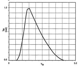
FIGURE 3-20. IDD versus Input Voltage for 'ACT Devices
