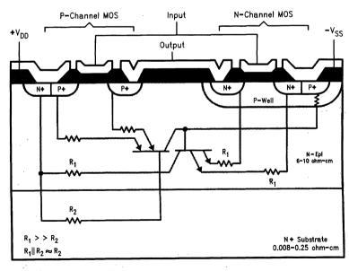
FIGURE 1-16. FACT EPI Process Cross Section with Latch-up Circuit Model
