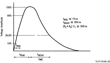
FIGURE 1-18. ESD Pulse Waveform
