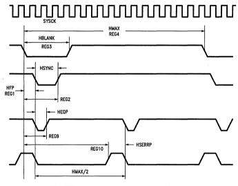
FIGURE 1. Horizontal Waveform Specification
