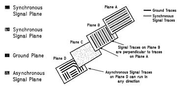
FIGURE 3-11a. Recommended Crosstalk—Avoidance Structure
