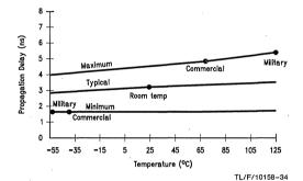
FIGURE 1-11i. t<sub>PHL</sub>, 'FCT244A, with Voltage and Process Variation
