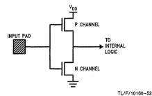
FIGURE 3-19. CMOS Input Structure
