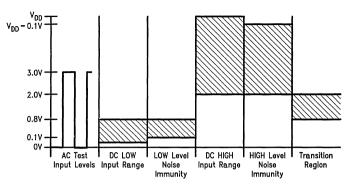
FIGURE 2b. Test Input Signal Levels
