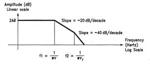
FIGURE 3-17. Time Domain to Frequency Domain Conversion
