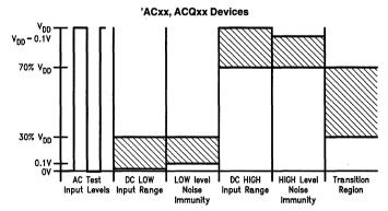
FIGURE 2a. Test Input Signal Levels
