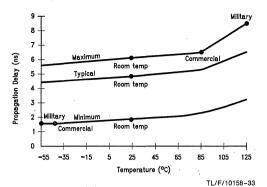
FIGURE 1-11h. t<sub>PHL</sub>, 'ACQ244, with Voltage and Process Variation
