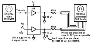
FIGURE 13. Simultaneous Switching Test Circuit
