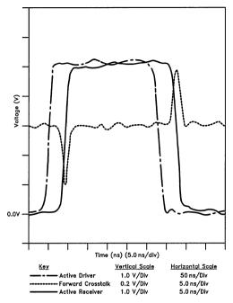
This figure shows traces taken on a test fixture designed to exaggerate the amplitude of crosstalk pulses.
