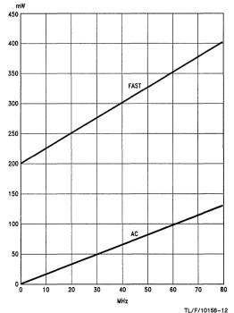
FIGURE 1-10. FACT vs FAST Circuit Power
