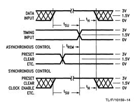
FIGURE 10. Set-Up, Hold and Release Times for FCT, FCTA
