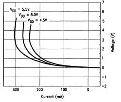
FIGURE 1-5c. Output Characteristics V<sub>OL</sub>/I<sub>OL</sub>, 'FCT244A
