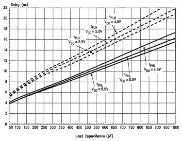
FIGURE 1-13a. Propagation Delay vs C<sub>L</sub> ('AC00)
