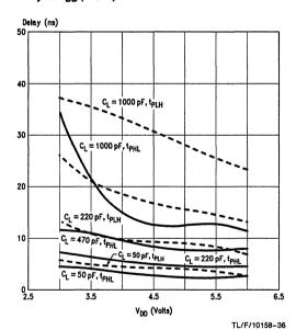
FIGURE 1-12c. Propagation Delay vs V<sub>DD</sub> ('FCT244A)
