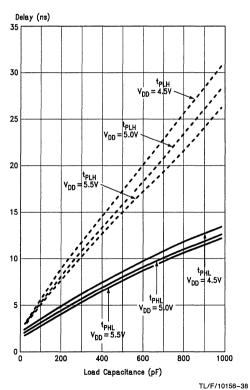
FIGURE 1-13c. Propagation Delay vs C<sub>L</sub> ('FCT244A)
