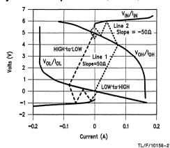
FIGURE 1-2. Gate Driving 50Ω Line Reflection Diagram
