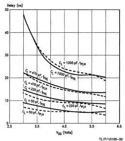
FIGURE 1-12b. Propagation Delay vs V<sub>DD</sub> ('ACTQ244)
