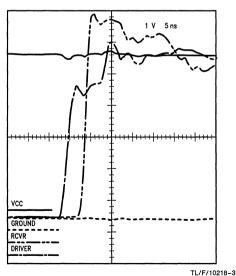
FIGURE 3. Effects of Input Clamp Diodes
