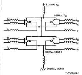
FIGURE 1. A Typical "00" 2-Input Quad NAND Gate
