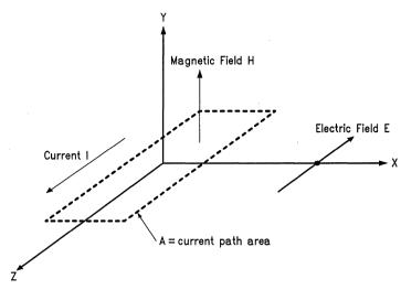
FIGURE 3-16. EMI is Generated by a Current Flowing along Some Path (Loop)
