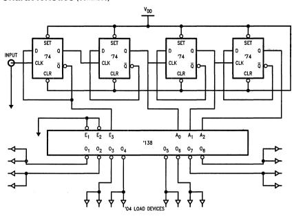
FIGURE 1-9. Power Demonstration Circuit Schematic
