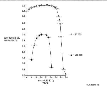
FIGURE 11. 'FCT534A Data/Clock  $V_{IH}$  Noise Margin IDT #5 (PDIP) vs NSC #2 (CDIP) 5.0V  $V_{DD}$  @ Room
