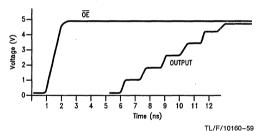
FIGURE 3-26. Typical ATE TRI-STATE Waveform
