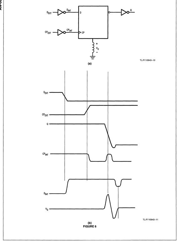
The most rigorous test for the non-inverting flop will be to have clock held at  $V_{IHD}$ , data at a hard HIGH, and all outputs are transitioning ZL.
