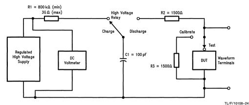
FIGURE 1-17. ESD Test Circuit
