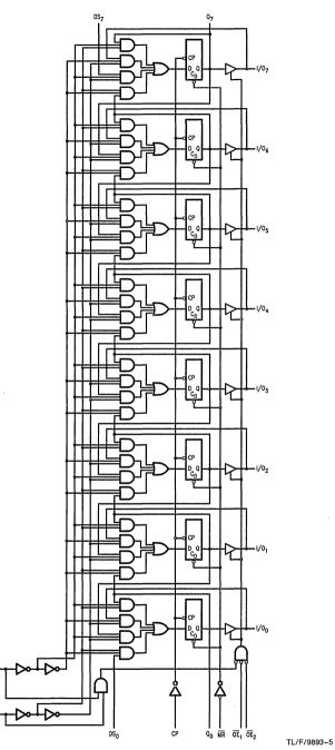
Please note that this diagram is provided only for the understanding of logic operations and should not be used to estimate propagation delays.
