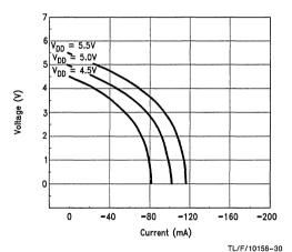
FIGURE 1-4c. Output Characteristics V<sub>OH</sub>/I<sub>OH</sub>, 'FCT244A
