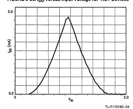
FIGURE 3-21. I<sub>DD</sub> versus I<sub>IN</sub> for 'AC Devices
