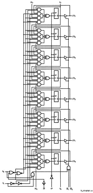
Please note that this diagram is provided only for the understanding of logic operations and should not be used to estimate propagation delays.
