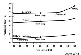
FIGURE 1-11g. t<sub>PHL</sub>, 'AC244, with Voltage and Process Variation
