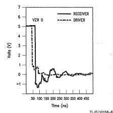
FIGURE 1-3d. Resultant Waveforms Driving 50Ω Line—Actual
