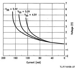
FIGURE 1-5b. Output Characteristics
