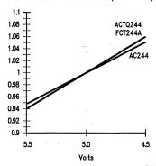
TL/F/10158-16 FIGURE 1-11e. Voltage Effects on Delay Times
