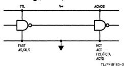
FIGURE 3-3. TTL Interfacing to 'ACT
