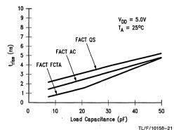
FIGURE 1-14. t<sub>rise</sub> vs Capacitance
