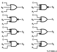
FIGURE a. Gate Functions (Each Half)
