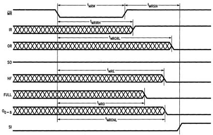
FIGURE 2. Mode of Operation Mode 2
