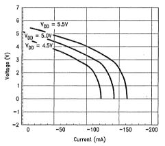
FIGURE 1-4a. Output Characteristics
