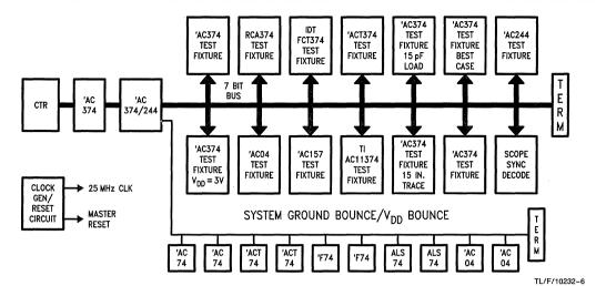
FIGURE 3. Ground Bounce Demonstration Board Block Diagram
