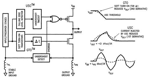
FIGURE 9. National Semiconductor's Proprietary Noise Control Circuitry
