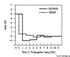
FIGURE 1-3c. Resultant Waveforms Driving 50Ω Line—Theoretical
