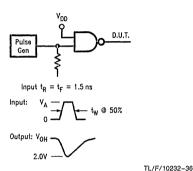
FIGURE 31. AC Noise Thresholds
