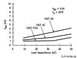
FIGURE 1-15. tfall vs Capacitance
