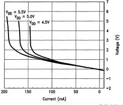
TL/F/10158-8 FIGURE 1-5a. Output Characteristics V<sub>OL</sub>/I<sub>OL</sub>, 'AC00
