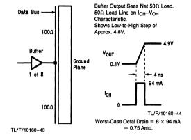
FIGURE 3-13. Octal Buffer Driving a  $100\Omega$  Bus
