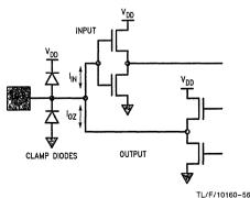
FIGURE 3-23. I/O Pin Internal Structure
