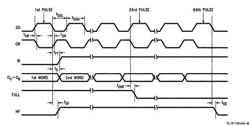
Note: SI and  $\overline{OE}$  are LOW;  $\overline{MR}$  is HIGH; D<sub>0</sub>-D<sub>8</sub> are immaterial.
