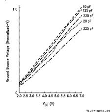
FIGURE 20. Quiet Output Noise vs Power Supply
