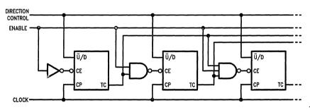
FIGURE C. Synchronous N-Stage Counter with Parallel Gated Carry/Borrow
