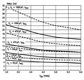
FIGURE 1-12a. Propagation Delay vs V<sub>DD</sub> ('AC00)
