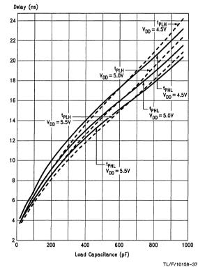
FIGURE 1-13b. Propagation Delay vs C<sub>L</sub> ('ACTQ244)
