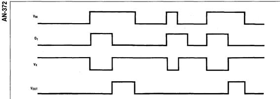
FIGURE 14. Pulse Width Detector (Continued)
