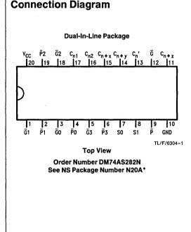
The carry functions (inputs, outputs, generate and propagate) of the look-ahead generator are implemented in compatible forms for direct connection to the 'AS881 ALU. The carry inputs are selectable in either active high or active low.
