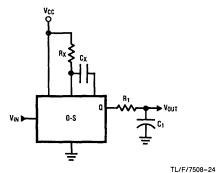
stant width for each triggering transition on its input. The output pulse train is integrated by  $R_1$  and  $C_1$  to yield a waveform whose amplitude is proportional to the input frequency. (Retriggerable device required.)
