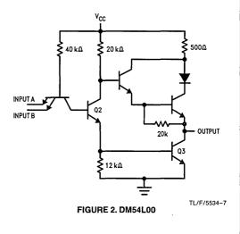
yield a symmetrical transfer characteristic (squaring network). This family achieves circuit performance exceeding the standard TTL family at fractions of its power consumption. The typical device power dissipation is 2 mW per gate and typical propagation delay is 10 ns while driving a 15 pF/ 2 k $\Omega$  load.
