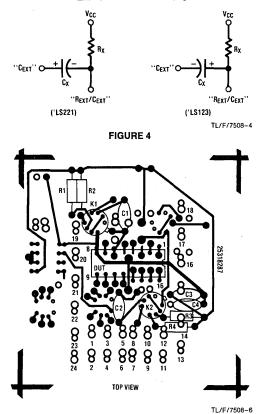
FIGURE 6a. AC Test Adapter
