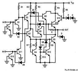
FIGURE 5. AS00 Schematic
