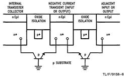
FIGURE 6. Parasitic Failures Modes
