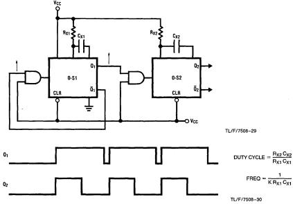
FIGURE 11. Pulse Generator (Retriggerable Device Required)
