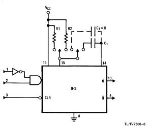
FIGURE 7a. Timing Components and I/O connections to D.U.T.
