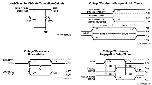
Note: All input pulses are supplied by generators having the following characteristics: frequency = 1 MHz,  $Z_{OUT} = 50\Omega$ ,  $t_r = t_f = 2$  ns.
