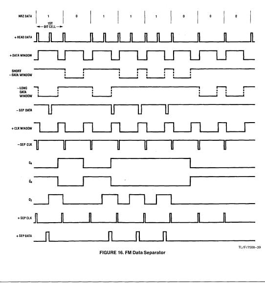
The next clock pulse (the second bit cell) is ANDed with +CLK WINDOW and becomes the next —SEP CLK, which will reset the R–S FF and trigger O–S1. As O–S1 becomes active, the +DATA WINDOW becomes active, enabling the first AND gate. With no data bit in the second bit cell, the R–S FF will remain reset, enabling the D–FF to be clocked off when +DATA WINDOW falls. When the D–FF is clocked off, Q<sub>4</sub> will hold O–S1 reset and allow O–S2 to be triggered.
