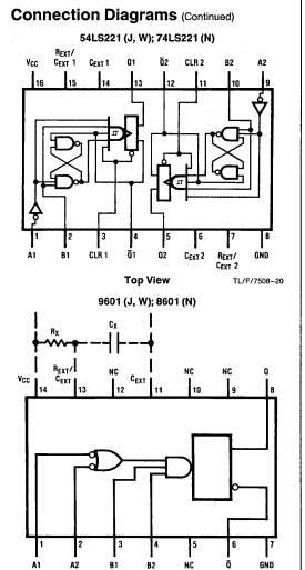
will follow the desired input pulse, with the leading edge delayed by the predetermined time constant. The output pulse width is also reduced by the amount of the time constant from  $R_X$  and  $C_X$ .
