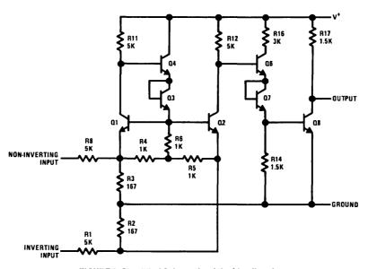
FIGURE 9. Simplified Schematic of the Line Receiver
