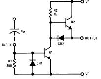
FIGURE 7. DS0025 Schematic (One-Half Circuit)
