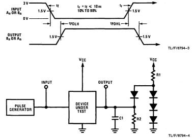
Note: C1 includes test fixture capacitance.
