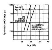
$$^{\rm TL/F/5219-7}$$  FIGURE 5. tpLH Measured to 2.7V on Output vs. CL
