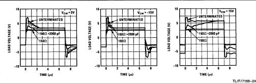
a.  $V_{CM}=0V$  b.  $V_{CM}=-15V$  c.  $V_{CM}=15V$  FIGURE 23. Line Response With Different Terminations and Common Mode Input Voltages
