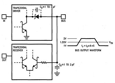
FIGURE 4. The Futurebus Trapezoidal Transceiver
