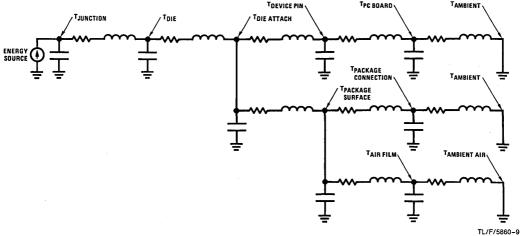
FIGURE 9. Thermal Reactance from Junction to Ambient
