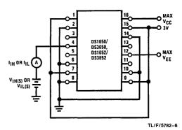
FIGURE 3.  $I_{IH(S)}$  and  $I_{IL(S)}$
