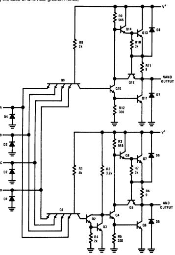
FIGURE 2. Schematic Diagram of the DS7830 Line Driver
