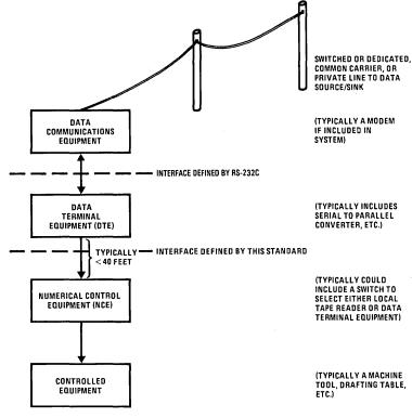
FIGURE 14. EIA RS-408 Interface Applications
