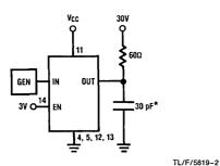
\*Includes probe and jig capacitance
