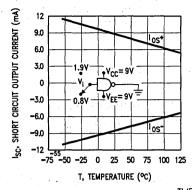
TL/F/5776-10 FIGURE 2. Short-Circuit Output **Current vs Temperature**
