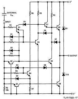
FIGURE 17. DS0026 Schematic (One-Half Circuit)
