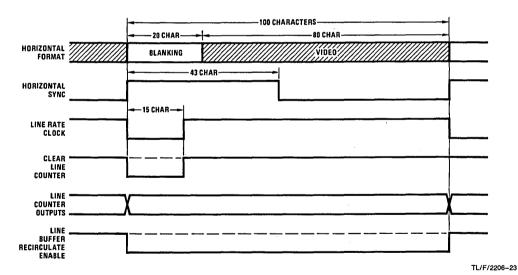
Note: Dashed lines in waveforms denote inactive state logic levels.
