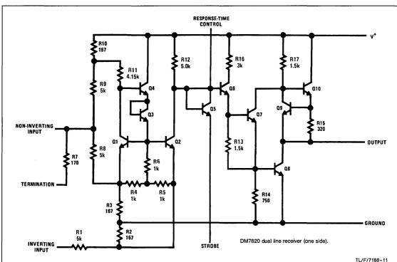
FIGURE 10. Complete Schematic of One Half of the DS7820 Line Receiver
