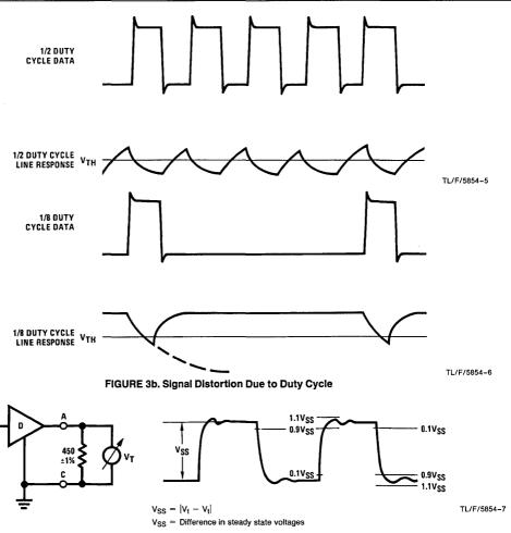
FIGURE 4. Unbalanced Driver Output Signal Waveform
