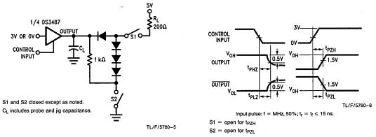
FIGURE 2. TRI-STATE Enable and Disable Delays
