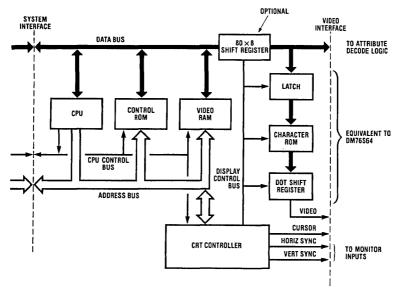
FIGURE 16. General System Block Diagram
