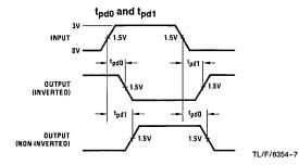
Input Characteristics: f = 1 MHz,  $t_R=t_F \leq 5$  ns (10% to 90% points), duty cycle = 50%,  $Z_{OUT}=50~\Omega$
