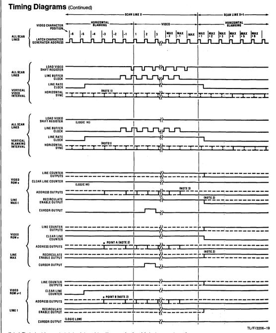
Note 1: The horizontal sync output start and stop point positions are a function of device type or custom option.
