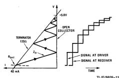
FIGURE 11. Line Reflection Diagram of Rise Timer
