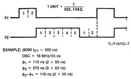
FIGURE B. DP8224 Clock Generator Waveforms
