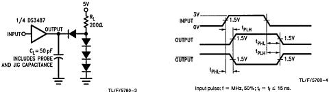
FIGURE 1. Propagation Delays
