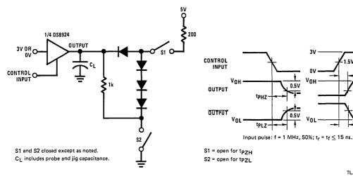
FIGURE 2. TRI-STATE Enable and Disable Delays
