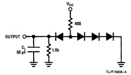
FIGURE 2. Receiver Output Load
