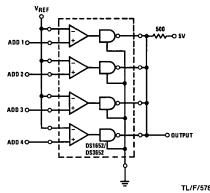
Wired "OR" Data Selecting Using TRI-STATE Logic
