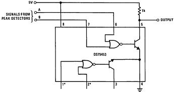
\*If inputs are unused, they should be connected to  $\pm 5V$  through a 1k resistor.
