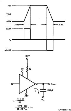
FIGURE 8. Clock Waveforms (Voltage and Current)
