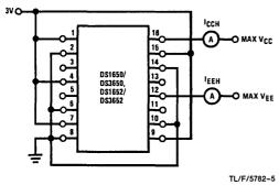
FIGURE 2. I<sub>CCH</sub> and I<sub>EEH</sub>
