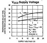
Propagation Delay Time, **High-to-Low Level Output** vs V<sub>CC2</sub> Supply Voltage
