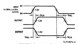
FIGURE 2. Propagation Delays
