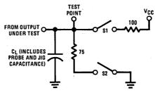
Note: S1 and S2 of load circuit are closed except where shown.
