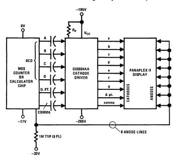
Note: Capacitive coupling between the logic and the segment drivers may be used only when the segment drivers are turned "OFF" during digit-to-digit transistions.
