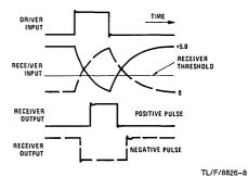
FIGURE 8. Slicing Level Distortion
