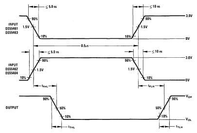
FIGURE 6. Switching Times of Complete Drivers
