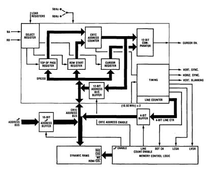
FIGURE 9. 8350 Block Diagram
