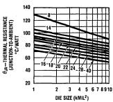
\*Packages from 8- to 20-pin 0.3 mil width 22-pin 0.4 mil width TL/F/5280-11
