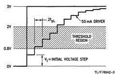
FIGURE 3. TTL Bus Waveforms—50 mA Driver
