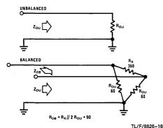
FIGURE 16. Impedance Measurement
