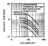
FIGURE 19. Data Rate vs Duty Cycle
