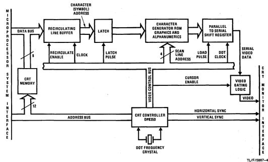
FIGURE 5. Character Generator Graphics (with line buffer)
