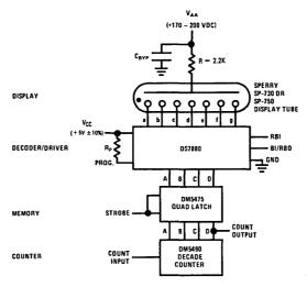
FIGURE 2. DC Operation From TTL
