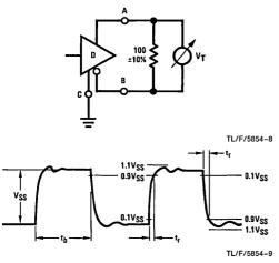
$t_{\mbox{\scriptsize b}}=$  Time duration of the unit interval at the applicable modulation rate.
