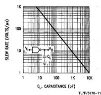
FIGURE 3. Output Siew Rate vs **Load Capacitance**
