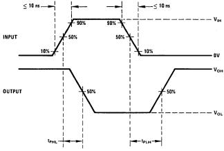
TL/F/5839-4 Note 1: The pulse generator has the following characteristics:  $Z_{OUT} = 50\Omega$ , PRR = 100 KHz,  $t_W = 1\mu s$ .
