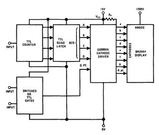
FIGURE 3. Interfacing Directly With TTL Output
