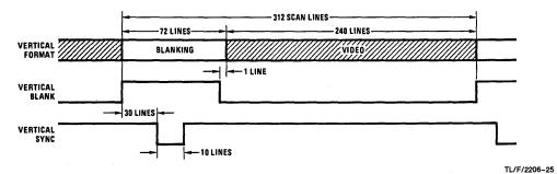
FIGURE 21. DP8350 50 Hz Refresh Rate Frame Signals
