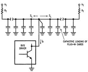
FIGURE 2. The Loaded Bus—Each Driver Sees Two Loaded Line Impedances in Parallel ( $Z_L || Z_L = Z_{L/2}$ ).
