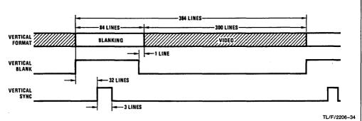
FIGURE 30. DP8353 50 Hz Refresh Rate Frame Signals
