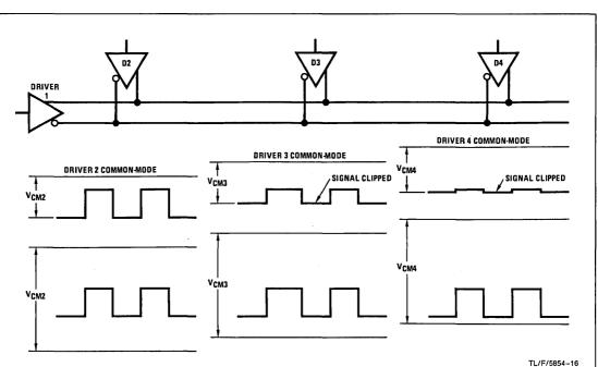
FIGURE 12. Comparison of Drivers without TRI-STATE Common-Mode Output Range (top waveforms) to DS3691 (bottom waveforms)
