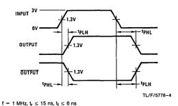
FIGURE 2. Propagation Delays
