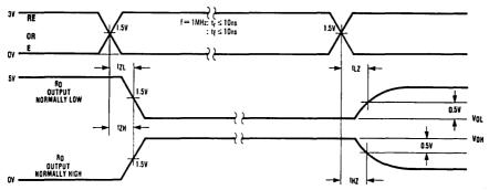
FIGURE 8. Receiver Enable and Disable Times
