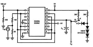
Note:  $E_{IN}$  waveform characteristics:  $t_{TLH}$  and  $t_{THL} \le 10$  ns measured 10% to 90% PRR = 1 MHz Duty Cycle = 50%
