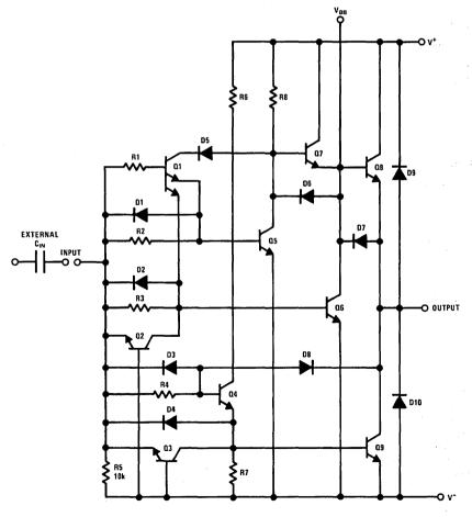
FIGURE 7. Schematic of 1/2 DS0056
