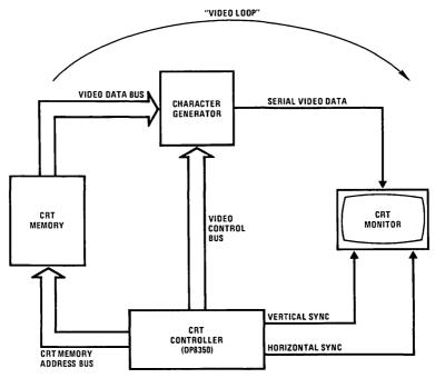
FIGURE 1. Elements of the "Video Loop"
