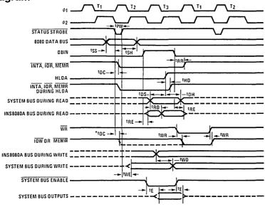
VOLTAGE MEASUREMENT POINTS: D<sub>0</sub>-D<sub>7</sub> (when outputs) Logic "0" = 0.8V, Logic "0" = 0.8V, Logic "1" = 3.0V. All other signals measured at 1.5V. \*Advanced |\overline{I/OW} MEMW for 8238 only.
