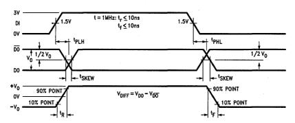
FIGURE 5. Driver Propagation Delays
