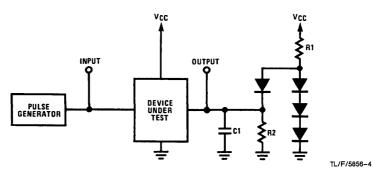
Note: C1 includes test fixture capacitance.
