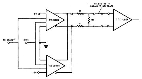
FIGURE 6. MIL-STD-188-114 (Balanced Applications)
