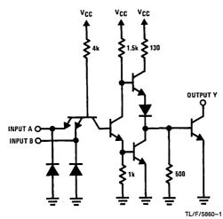
FIGURE 1. Typical Peripheral Driver DS75451
