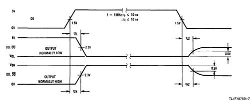
FIGURE 6. Driver Enable and Disable Times
