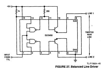
Termination is made at the receiving end as follows: Line 1 is terminated to ground through Z<sub>O</sub>/Z; Line 2 is terminated to +5V through Z<sub>O</sub>/Z;
