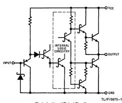
(Equivalent Input/Output Circuit)
