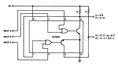
FIGURE 34. Multifunction Logic-Signal Comparator
