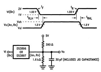
**Note:**  $t_{R} = t_{F} \le 10 \text{ ns from } 10\% \text{ to } 90\%$
