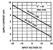
TL/F/7188-18 FIGURE 17. Power Supply Current as a Function of Common Mode Input Voltage
