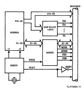
FIGURE 11. 8080 System Model for the Basic Microbus Interface
