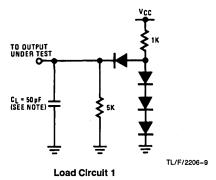
Note: C<sub>L</sub> includes probe and jig capacitance. All diodes are 1N914 or equivalent.
