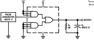
Note 1: The pulse generators have the following characteristics:  $Z_{OUT} \approx 50\Omega$ ,  $t_W = 200$  ns, duty cycle
