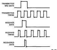
**FIGURE 4. Effect of Distortion**
