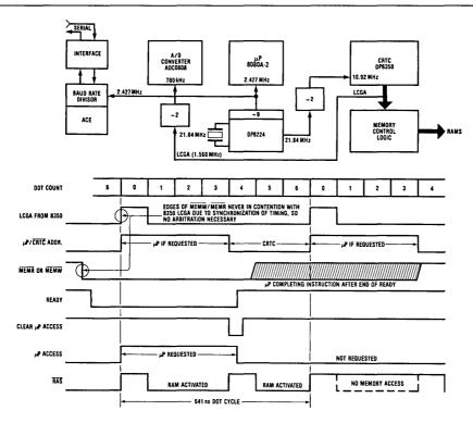
FIGURE 10. System Timing Control Circuit and Diagram
