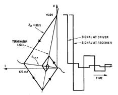
TL/F/8826-12 FIGURE 12. Line Reflection Diagram of Fall Time
