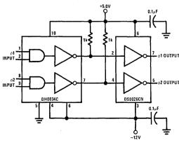
FIGURE 24. Transistor Coupled MOS Clock Driver
