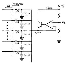
FIGURE 6. The Futurebus Termination Circuit
