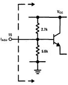
I<sub>ADJ</sub> may be programmed by a voltage source or by resistors.
