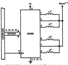
\*L1, L2, L3, L4 are the windings of a bifilar stepping motor.
