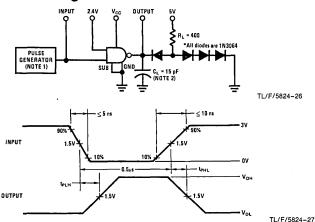
Note 1: The pulse generator has the following characteristics: PRR = 1 MHz,  $Z_{OUT} \approx 50\Omega$ .
