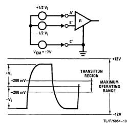
FIGURE 6. Receiver Input Sensitivity Measurement
