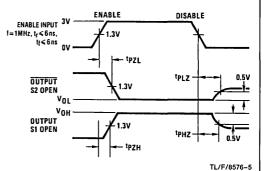
FIGURE 3. Enable and Disable Times
