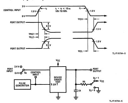
Note: C4 includes test fixture capacitance. Port input is in a fixed logical condition. See AC Table.
