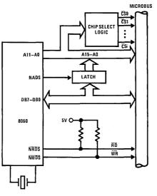
FIGURE 10.8060 SC/MP II System Moldel
