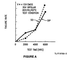
In order to achieve reliability performance comparable to DIPS—SO packages are designed and built with materials and processes that effectively compensate for their small size
