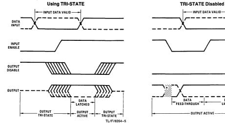
\*When the Input Enable makes a negative transition, the output will be indeterminate for a short duration. The negative transition of the Input Enable normally occurs during a don't-care timing state at the output.
