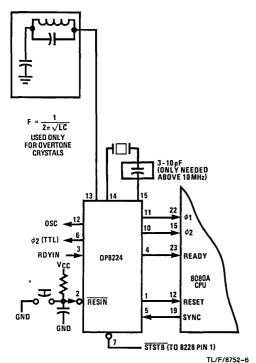
FIGURE A. DP8224 Connection Diagram
