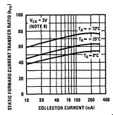
FIGURE 17. DS75450 Transistor Static Forward Current
