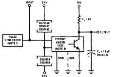
Note 1: The pulse generator has the following characteristics: PRR =  $^{0.4V}_{1.0}$  MHz,  $Z_{OUT} \approx 50\Omega$ .
