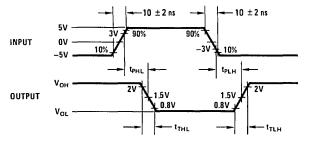
Note 1: The pulse generator has the following characteristics:  $Z_{OUT} = 50\Omega$ ,  $t_W = 200$  ns, duty cycle  $\leq 20\%$ . Note 2:  $C_L$  includes probe and jig capacitance.
