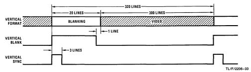
FIGURE 29, DP8353 60 Hz Refresh Rate Frame Signals
