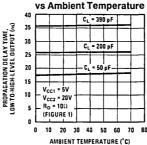
Propagation Delay Time, High-to-Low Level Output vs Ambient Temperature
