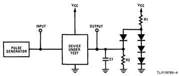
Note: C1 includes test fixture capacitance.
