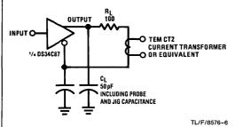
FIGURE 4. Differential Rise and Fall Times
