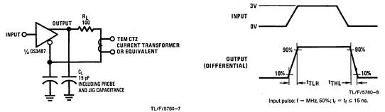
FIGURE 3. Differential Rise and Fall Times
