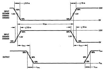
**FIGURE 14. Switching Times of Complete Drivers**
