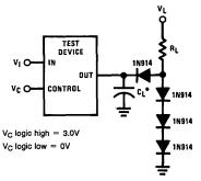
\*CL includes jig and probe capacitance
