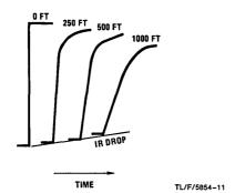
FIGURE 7. Signal Rise Time on Transmission Line vs Line Length
