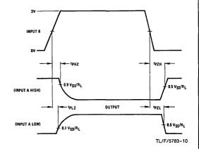
FIGURE 4. TRI-STATE Delays
