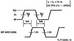
FIGURE 8. X1 Input to Dot Rate Clock
