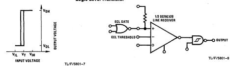
The DS78C120/DS88C120 may be used as a level transistor to interface between ±12V MOS, ECL, TTL and CMOS. To configure, bias either input to a voltage equal to ½ the voltage of the input signal, and the other input to the driving gate.
