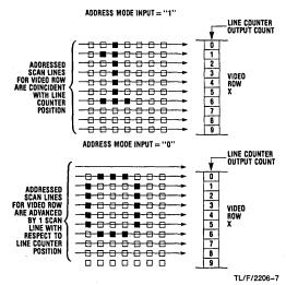
FIGURE 5. Address Mode Functionality
