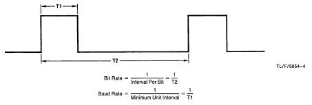
FIGURE 3a. Definition of Baud Rate
