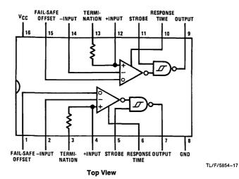
FIGURE 13. DS78LS120/DS88LS120 Dual Differential Line Receiver
