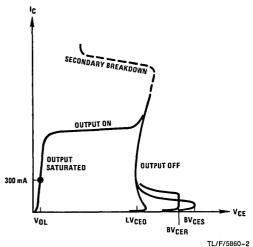
FIGURE 2. Output Characteristics ON and OFF
