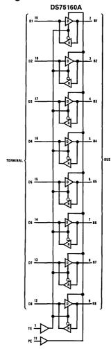
Note 3: Driver and receiver outputs are totem-pole configurations Note 4: The driver outputs of DS75160A can have their active pull-ups disabled by switching the PE input (pin 11) to the logic low state. This mode configures the outputs as open collector.
