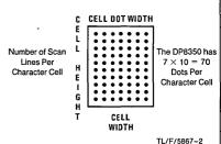
FIGURE 3. The DP8350 Character Cell is 7 Dots Wide and 10 Dots High
