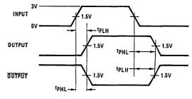
Input pulse: f = 1 MHz, 50%;  $t_r = t_f \le 15$  ns.
