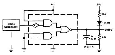
Note 1: The pulse generator has the following characteristics:  $Z_{OUT} \approx 50\Omega$ ,  $t_W = 200$  ns, duty cycle = 50% Note 2:  $C_L$  includes probe and jig capacitance.
