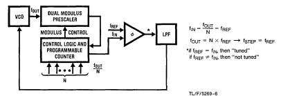
FIGURE 6. Basic Dual-Modulus Frequency Synthesizer
