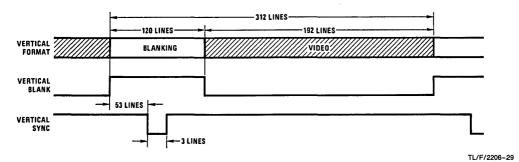
FIGURE 25. DP8352 50 Hz Refresh Rate Frame Signals
