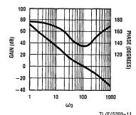
VHF loop, running at 100 MHz, ref = 10 kHz  $K_V = 2.5 \text{ MHz/V} = 15.7 \text{ Mrad/sec/V}$  $K_D = \frac{400 \, \mu A}{4\pi} = 31.8 \, \mu A/radian$  $\frac{100 \text{ MHz}}{100 \text{ MHz}} = 10,000, \, \omega_{\text{O}} = 2\pi \times 100 \, \text{Hz}$ 10 kHz  $\theta = 45^{\circ}$  (desired phase margin)  $T2 = 6.6 \times 10^{-4} \text{ sec}$  $T1 = 3.84 \times 10^{-3} \text{ sec}$  $C1 = 0.3 \mu F$ so R1 = T1/C1 = 13 k $\Omega$  $C2 = T2/R1 = 0.05 \mu F$
