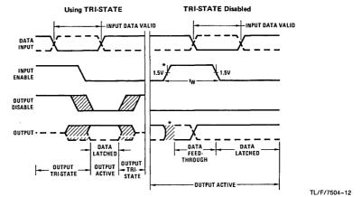
\*When the Input Enable makes a positive transition the output will be indeterminate for a short duration. The positive transition of the Input Enable normally occurs during a don't care timing state at the output.
