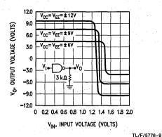
FIGURE 1. Transfer Characteristics vs Power Supply Voltage
