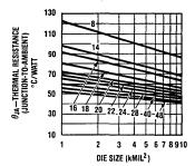
\*Packages from 8- to 20-pin 0.3 mil width 22-pin 0.4 mil width TL/F/5280-10
