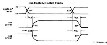
\*Input signal: f = 1.0 MHz, 50% duty cycle,  $t_f = t_f \le 5 \text{ ns}$
