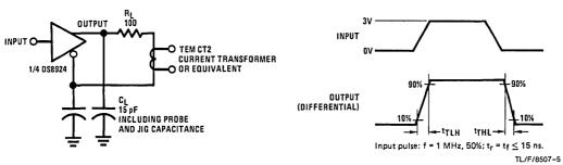
FIGURE 3. Differential Rise and Fall Times
