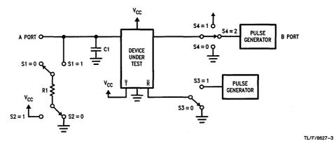
FIGURE A. A Port Test Load
