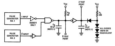
Note 1: Includes probe and jig capacitance.
