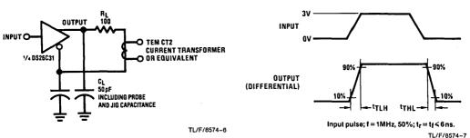
FIGURE 4. Differential Rise and Fall Times
