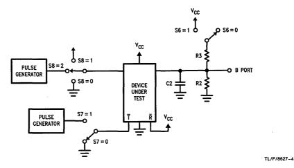
FIGURE B. B Port Test Load
