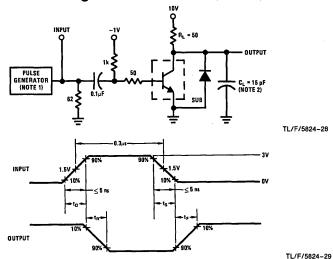
Note 1: The pulse generator has the following characteristics: duty cycle  $\leq$  1%, Z<sub>OUT</sub>  $\approx$  50 $\Omega$ .
