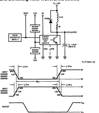
Note 1: The pulse generator has the following characteristics: PRR = 12.5 kHz,  $Z_{OUT} \approx 50\Omega$ .
