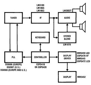
FIGURE 12. AM-FM Digitally Tuned Radio System
