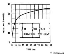
FIGURE 19. Transient Response of an Incandescent Lamp
