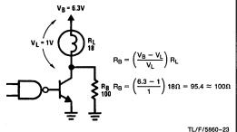
FIGURE 23. Circuit Used to Reduce Peak
