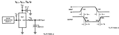
Note 1: The pulse generator has the following characteristics:  $Z_{OUT} = 50\Omega$  and PRR  $\leq 1$  MHz. Rise and fall times between 10% and 90% points  $\leq 5$  ns. Note 2:  $C_L$  includes probe and jig capacitance.
