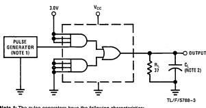
Note 1: The pulse generators have the following characteristics:  $Z_{OUT} \approx 50\Omega$ ,  $t_W = 200$  ns, duty cycle = 50%,  $t_r$ , =  $t_f$  = 5.0 ns.
