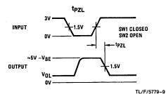
FIGURE 2. Propagation Delay TRI-STATE Control Input to Output
