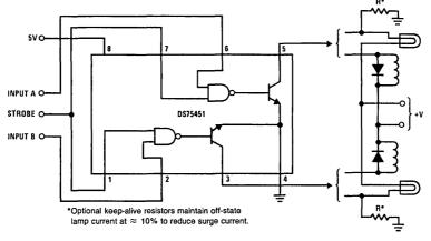
FIGURE 28. Dual Lamp or Relay Driver
