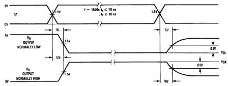
FIGURE 8. Receiver Enable and Disable Times
