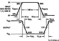
Note 1: Input pulses are supplied by a generator having the following characteristics:  $Z_0 = 50\Omega$ , PRR = 5 MHz.
