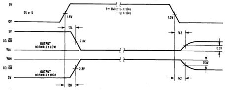
FIGURE 6. Driver Enable and Disable Times
