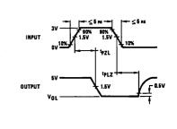
FIGURE 3.  $t_{PZL}$  and  $t_{PLZ}$
