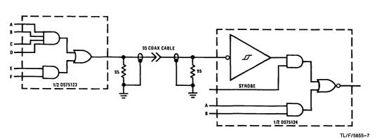
FIGURE 7. IBM 360/370 I/O Application
