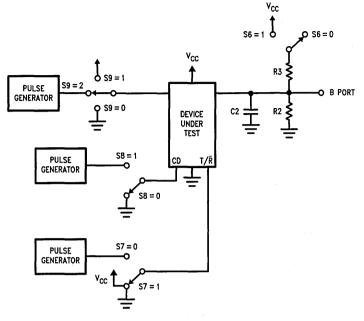
FIGURE B. B Port Test Load
