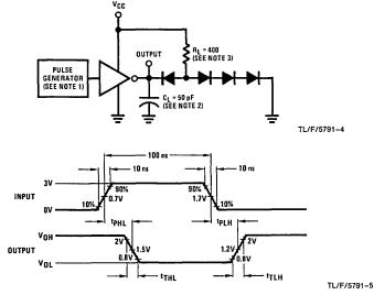
Note 1: The pulse generator has the following characteristics:  $Z_{OUT}=50\Omega$ , PRR = 5 MHz.
