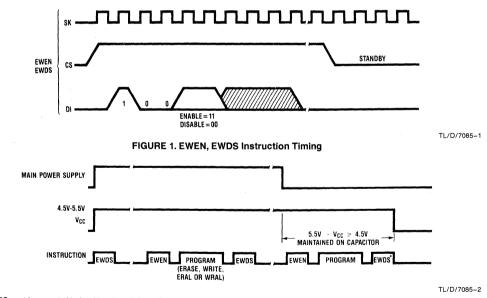
\*EWDS must be executed before V<sub>CC</sub> drops below 4.5V to prevent accidental data loss during subsequent power down and/or power up transients.
