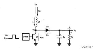
FIGURE 1. Basic Step-Up Switching Regulator
