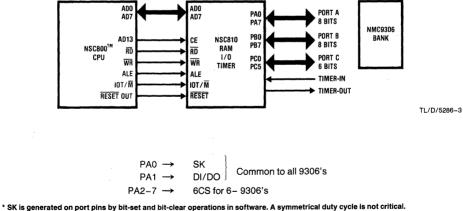
\* CS is set in software. To generate 10–30 ms write/erase the timer/counter is used. During write/erase. SK may be turned off.
