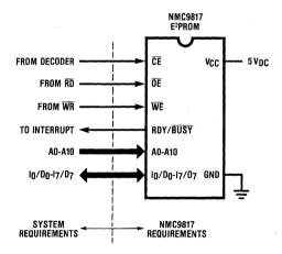
FIGURE 4. Simple NMC9817 Interface Requirements
