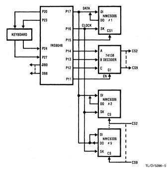
\* SK and DI are generated by software. It should be noted that at 2.72 μs/instruction. The minimum SK period achievable will be 10.88 μs or 92 kHz, well within the NMC9306 frequency range.
