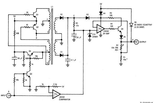
FIGURE 8. VPP Pulse Generator Circuit
