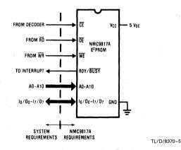
FIGURE 3. Simple NMC9817A Interface Requirements
