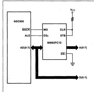
FIGURE 8-5. System Bus Separation
