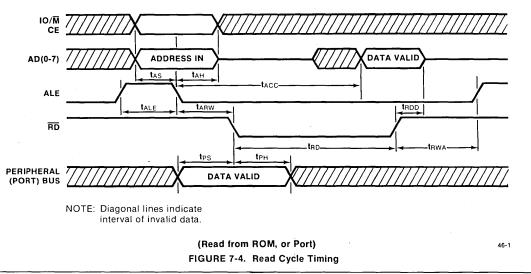
When a read occurs, the information is latched from the peripheral (port) bus during the leading (falling) edge of the  $\overline{RD}$  strobe. When a write occurs, the port bus is modified after the trailing (rising) edge of the  $\overline{WR}$  strobe with data from the AD bus. Port output data remains valid at the output pin from one trailing edge of  $\overline{WR}$  strobe to the trailing edge of the next  $\overline{WR}$  strobe, which then modifies that port.
