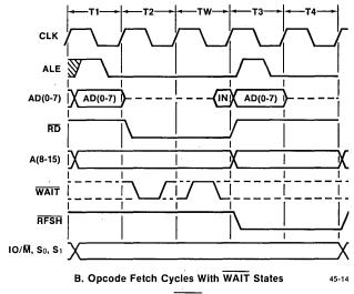
FIGURE 4-18. Effect of WAIT on Machine Cycles
