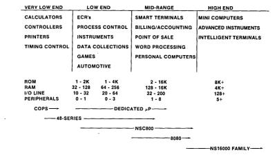
FIGURE 2-1. National Semiconductor Microprocessors Performance Spectrum
