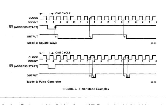
Prescale The timer output is affected by the prescale selection. The output responds to the timer clock, not the incoming clock (TIN); so, TOUT will be prescaled by the same value as the timer. Although the 16-bit prescaled count of the timer may be read, the internal value of the prescaler cannot be read by the user. A "00" for either timer represents ÷ 1 (no prescale). Timer 0 has the two possibilities of ÷ 2 or ÷ 64:
