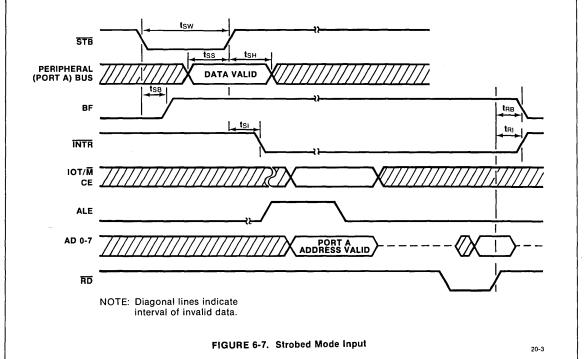
to accept the data in Port A it pulses the STB signal. STB will reset BF with its rising edge and also activates the INTR signal.
