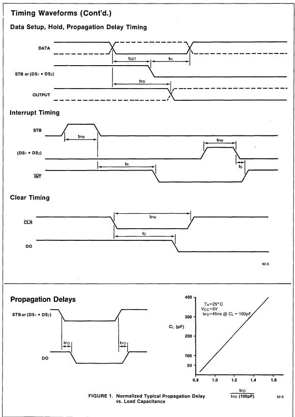
Figure 1 illustrates the calculations of a more useful propagation delay. The figure uses a 5-volt supply with a tolerance of  $\pm 10\%$ , ambient temperature of  $\pm 25^{\circ}$  C, and a load capacitance of 100pF. The AC Characteristics table depicts trp, at 5 volts, 25^{\circ} C, equalling 25ns. Use the graph in *Figure 1* to get the degradation multiple for 150pF. The number shown is 1.09. The adjusted propagation delay is, therefore 25 x 1.09 or 27ns.
