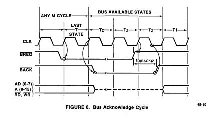
T<sub>Z</sub> = Time states Bus and control signals are in high impedance mode.
