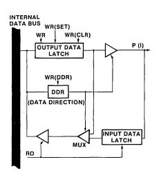
FIGURE 6-3. Block Diagram for Port Bit (i)
