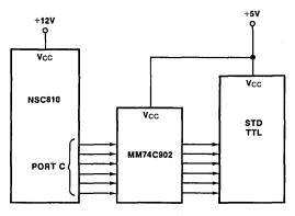
FIGURE 8-14. P<sup>2</sup>CMOS at High Voltage to Standard TTL 72-15
