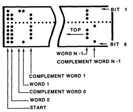
NOTE 1: Tape must be blank except for the data words. NOTE 2: Tape must start with a rubout character.
