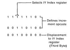
The indexed addressing mode uses the contents of index register IY as a base address from which a pointer is formed to where the data is incremented.
