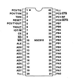
FIGURE 6-2. NSC810 Pin Configuration
