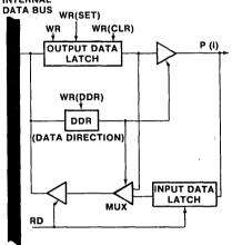
FIGURE 2. Block Diagram for Port Bit (i)
