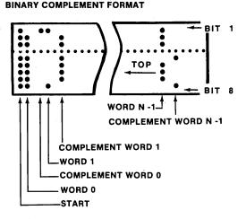
NOTE 1: Tape must be blank except for the data words. NOTE 2: Tape must start with a rubout character.
