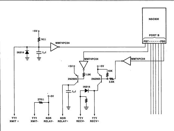
FIGURE 8-17. Serial I/O Via Port I/O Pins
