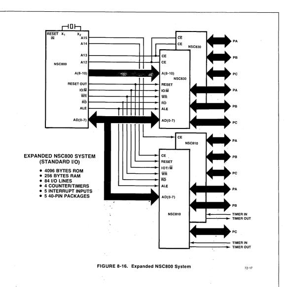
NSC830 can also be used, or if the NSC830 is configured in the memory-mapped I/O technique, the bit set and reset instructions of the NSC800 could also be used.
