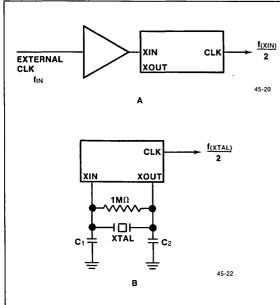
FIGURE 8-2. External Clock Circuits
