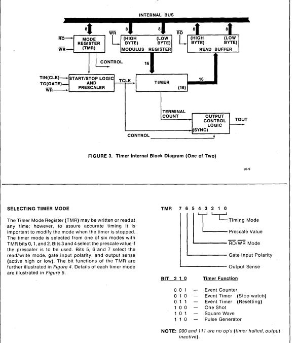
FIGURE 4. Timer Mode Register (Mode Selection)
