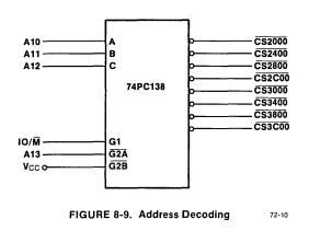
process, and are speed and bus compatible with the NSC800. *Figure 8-10* shows an expanded system using the NMC6514 to provide 4K of R/W memory. Since the NMC6514 has on-chip address latches, it is not necessary to demultiplex the address/data bus for interfacing. An MM74PC138 is used to decode the address space for the RAM.
