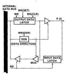
FIGURE 7-3. Block Diagram for Port Bit (i)
