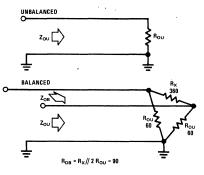
FIGURE 16. Impedance Measurement
