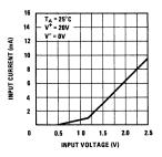
FIGURE All-4. Input Current vs Input Voltage
