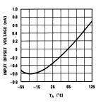
FIGURE 3. Offset Temperature Coefficient
