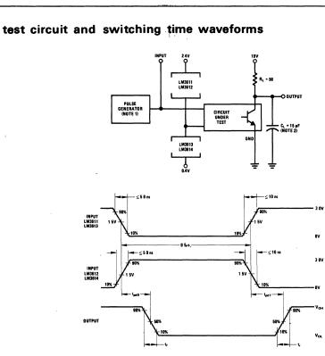
NOTE 1 THE PULSE GENERATOR HAS THE FOLLOWING CHARACTERISTICS PRR = 1 0 MHz,  $z_{OUT} \approx 50 \Omega$  Note 2  $c_L$  includes probe and Jig Capacitance
