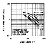
FIGURE 22. Data Rate vs Distorion of DM7820A, DM7830
