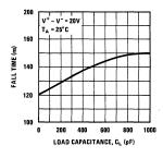
FIGURE AI-5. MH0025 Fall Time vs CL
