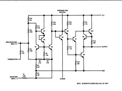
FIGURE 18. DM7820 Schematic
