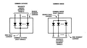
FIGURE 1. 7-Segment LED Construction
