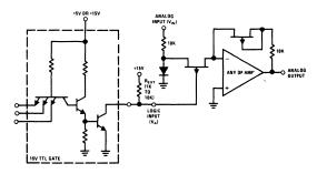
FIGURE 5. Interfacing with +15V Open Collector Logic
