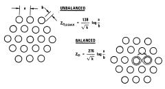
FIGURE 15. Z<sub>O</sub> Unbalanced < Z<sub>O</sub> Balanced
