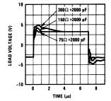
FIGURE 21. Line Response for Various Termination Resistances With a DC Isolation Capacitor
