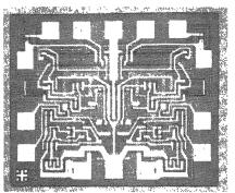
FIGURE 11. Photomicrograph of the DM7820 Dual Line Receiver
