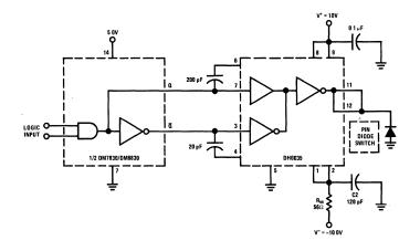
FIGURE 5. Anode Grounded Driver
