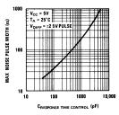
FIGURE 20. Noise Rejection in the DM7820A
