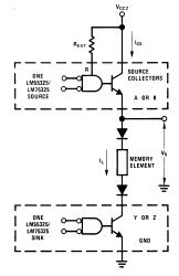
Note 1 For clarity, partial logic diagrams of two LM55325's are shown Note 2 Source and sink shown are in different packages
