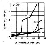
FIGURE 4. Low-State Output Current as a Function of Output Current
