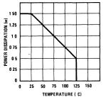
FIGURE 2. Maximum Power Dissipation
