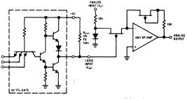
FIGURE 4. Interfacing with +5V Logic
