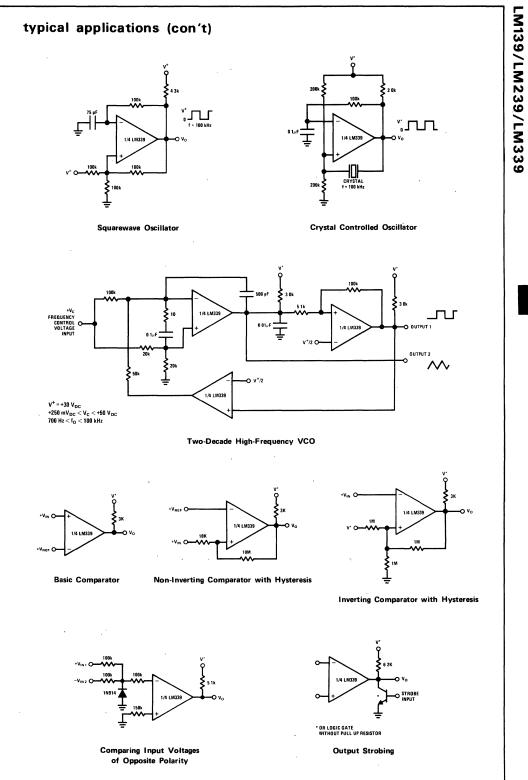
Voltage Comparators LM139A/LM239A/LM339A low offset voltage quad comparators
