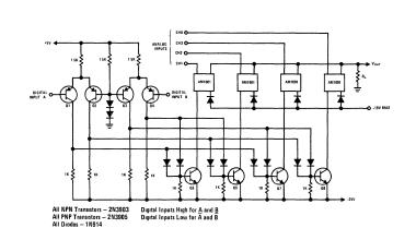
FIGURE 9. Binary Controlled Four Channel Multiplexer
