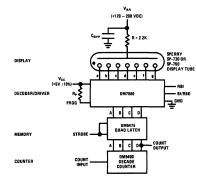
FIGURE 2. DC Operation From TTL
