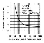
FIGURE 1. Delay vs Overdrive
