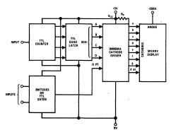
FIGURE 3. Interfacing Directly With TTL Output
