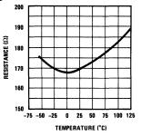
FIGURE 18. Variation of Termination Resistance With Temperature
