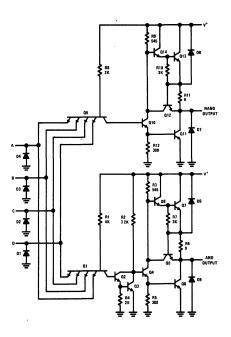
FIGURE 2. Schematic Diagram of the DM7830 Line Driver
