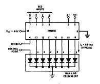
FIGURE 7. Nonmultiplex Application of the DM8856
