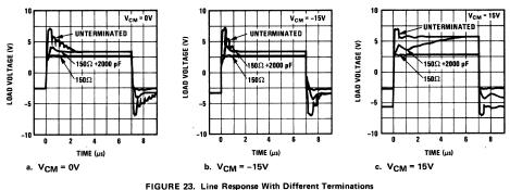
URE 23. Line Response With Different Terminatio and Common Mode Input Voltages
