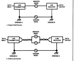
FIGURE 1. Comparing Differential and Single-Ended Data Transmission
