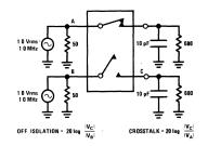
FIGURE 3. tON, tOFF, Test
