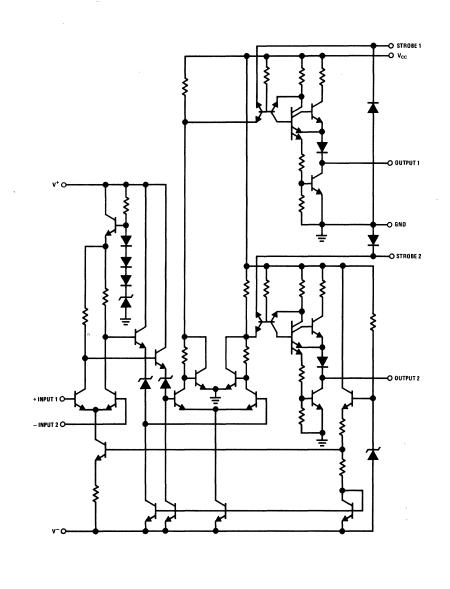
FIGURE 5. LM161 Schematic Diagram
