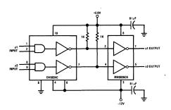
FIGURE All-8. Transistor Coupled MOS Clock Driver
