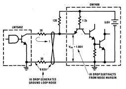
FIGURE 9. Unbalanced Method
