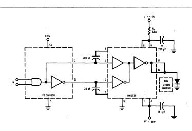
FIGURE 6. Cathode Grounded Design
