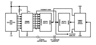
FIGURE 6. Fully Decoded MOS Cathode Outputs
