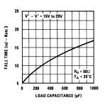
FIGURE All-3. Fall Time vs Load Capacitance
