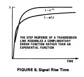
The rise time in a transmission line is not an exponential function but a complementary error function. The high frequency components of the step input are attenuated and delayed more than the low frequency components. This attenuation is inversely proportional to the frequency. Notice in *Figure 6* particularly that the signal takes much longer to reach its final dc value. This effect is more significant for fast risetimes.
