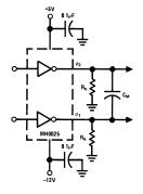
FIGURE 6. Use of Bleed Resistors to Minimize Clock-Line Crosstalk
