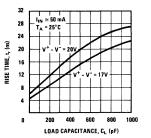
FIGURE AI-3. Rise Time vs CL for the MH0025
