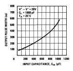
FIGURE All-6. Optimum Input Capacitance vs Output Pulse Width
