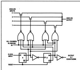
FIGURE 12. Logic Diagram of MM454F Four-Channel MOS Multiplexer. Switches and Control Circuitry Are Fabricated in the Same Monolithic Chip.
