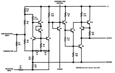
FIGURE 10. Complete Schematic of the Line Receiver
