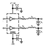
FIGURE 3. Use of Damping Resistor to Eliminate Clock Overshoot
