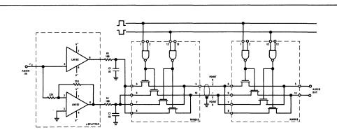
FIGURE 7. Double Sideband Modulator-Demodulator
