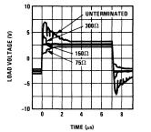
FIGURE 20. Transmission Line Response With Various Termination Resistances
