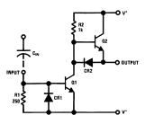
FIGURE AI-1. MH0026 Schematic (One-Half Circuit)
