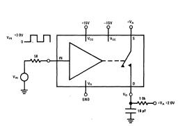
FIGURE 4. tON, tOFF Test Circuit
