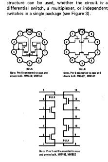
FIGURE 3. Connection Diagrams of Dual Differential Switch, Four-Channel Switch and Quad MOS Transistor.
