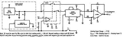
Note S1 must be open for 50, $\mu$ s min to take first reading with  $l_{\perp} = 50$  mA Second reading is taken with S2 closed. With S1 and other set-up forong functions under computer control, system will measure line and load regulation on voltage regulatory voltage gain, diffect current, CMR and PSR on on gains as well as other circuits requiring measurement of the change of a parameter with the change of a forcing function
