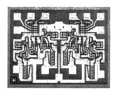
FIGURE 8. Photomicrograph of the DM7830 Dual Line Driver
