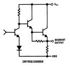
FIGURE 4d. Output Stage
