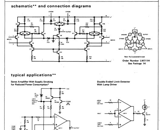
\*\*Pin connections shown are for metal can
