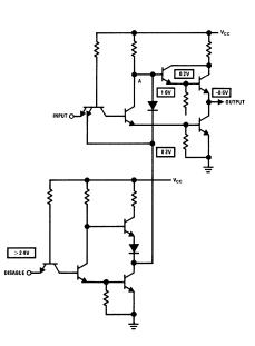
FIGURE 9. DC Levels in a Disabled TRI-STATE Element
