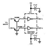
FIGURE AI-10, Transistor Coupled MH0025 Clock Driver.
