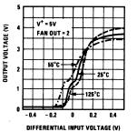
FIGURE 14. Voltage Transfer Function
