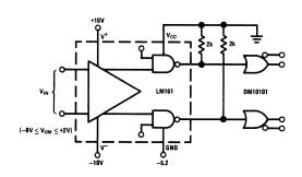
FIGURE 9. Direct Interfacing to ECL
