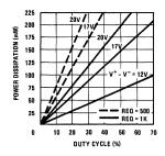
FIGURE 1. PDC vs Duty Cycle
