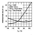
FIGURE 2. Delay vs Temperature
