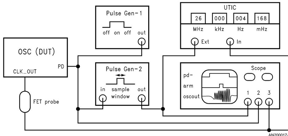
FIGURE 1. Sample Measurement Setup
