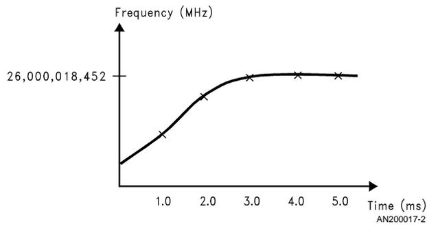
FIGURE 2. Plot of a Xtal Oscillator Startup Time Profile
