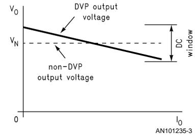
**FIGURE 3. DVP Converter Output Characteristics**
